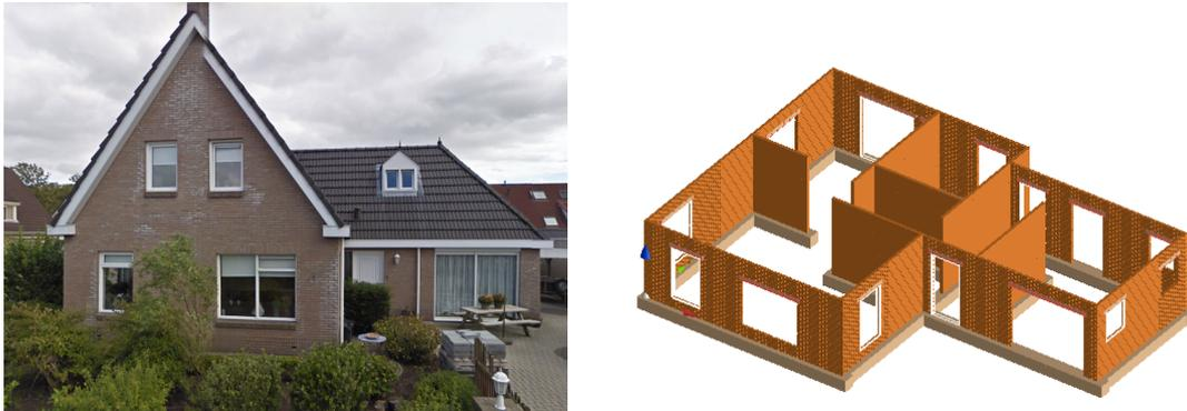
Figure 3.1. URM detached building and associated Extreme Loading for Structures (ELS) model (where the concrete slab is not shown and the gable walls and roof are applied as line loads to the appropriate ground floor bearing walls)
