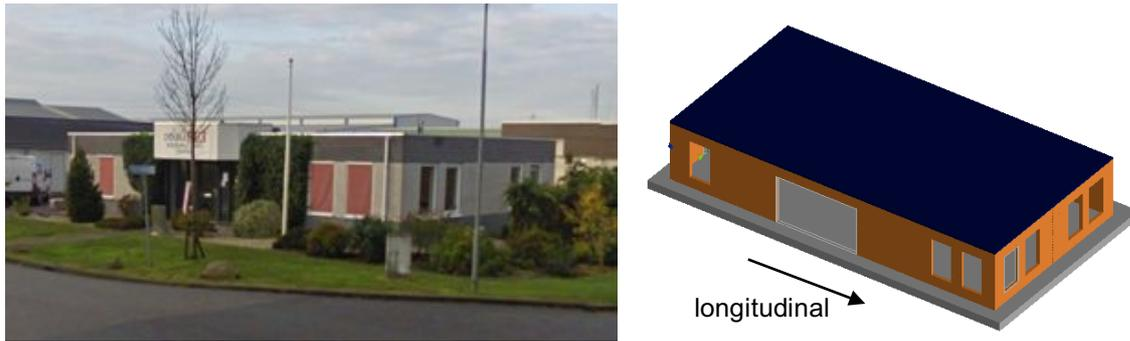
Figure 3.13. A typical industrial/commercial URM building (left) and ELS prototype structure (right)
