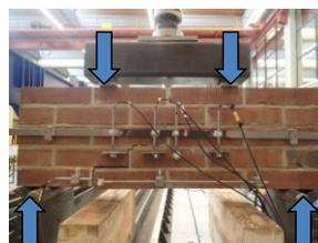
Figure 7.12 Material tests on small walls samples.
