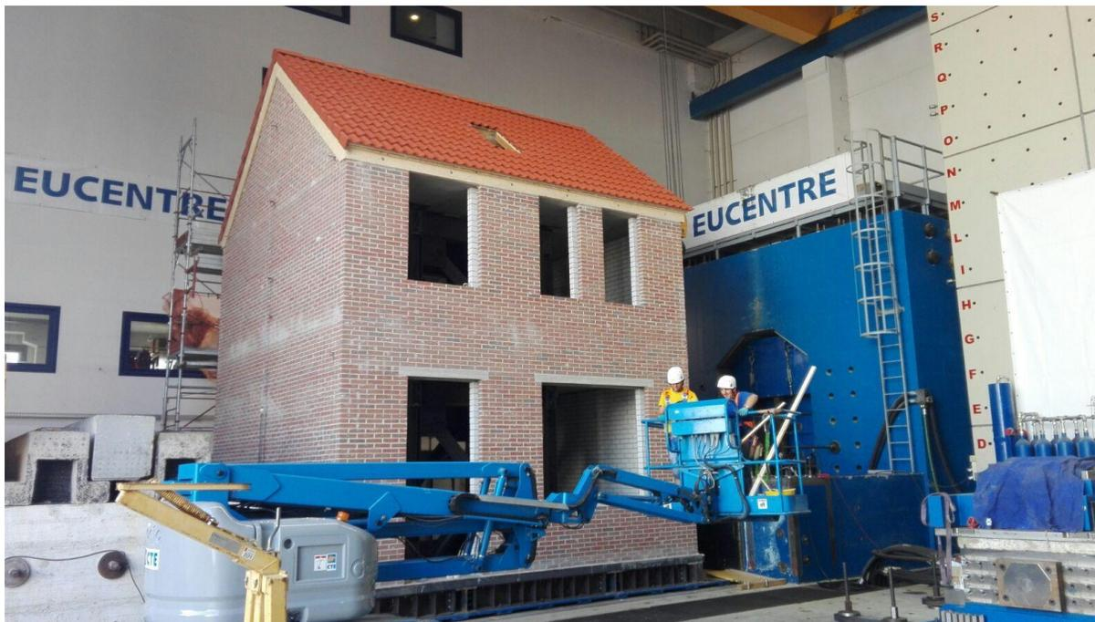
Figure 7.16 Full-scale terraced house building on the shaking table
