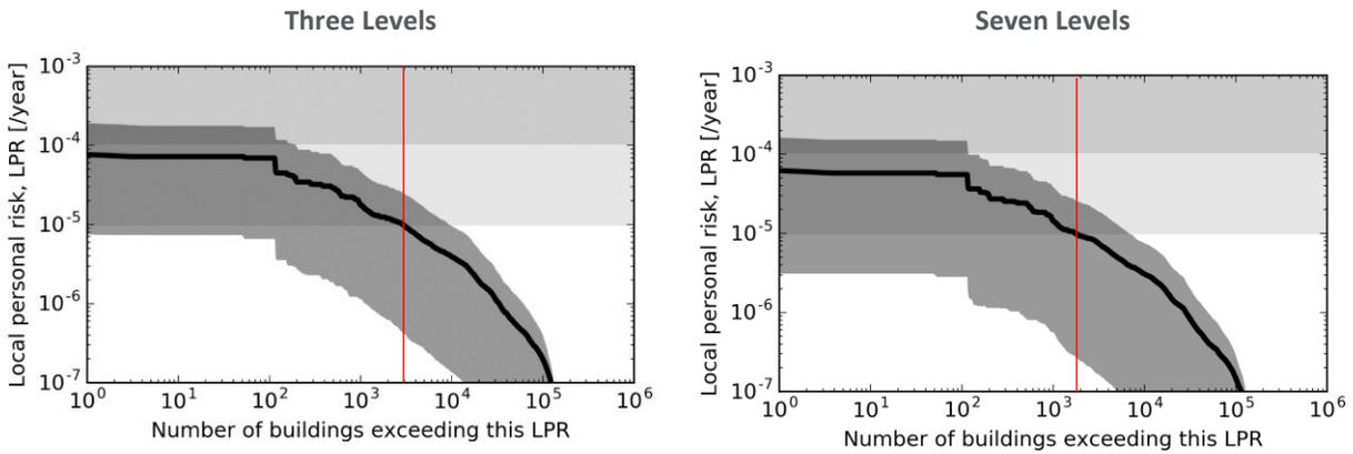
Figure C.5 LPR distributions under the 24 Bcm/year production scenario for the 3-point (left) and 7-point (right) discrete  $M_{max}$  distributions.
