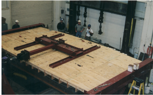
Figure 127 General diaphragm test setup
