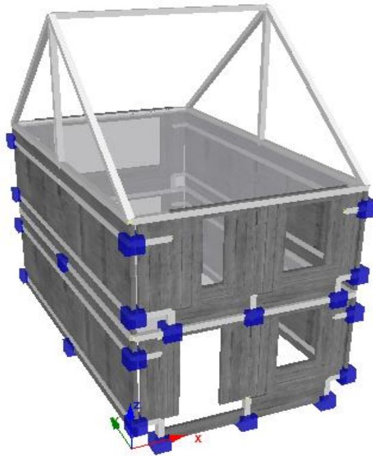
Figure 2.25: Screenshot of the SeismoStruct model of the calibrated one-unit REST-RC-B index building with nonlinear springs at the base of the wall panels and between adjacent panels
