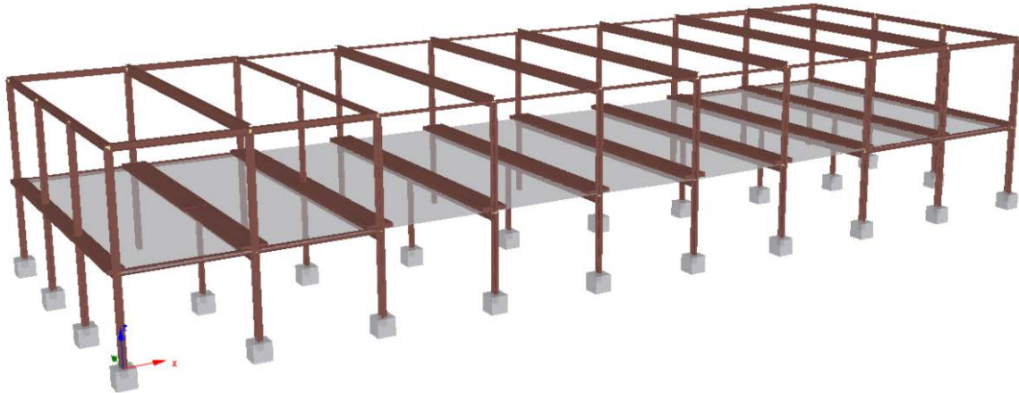
Figure 11.6: Screenshot of the SeismoStruct model of the COMO-S-B-L4S index building
