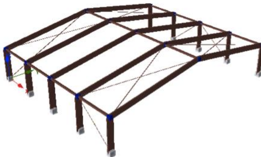
Figure 7.4: AGRI/INDU/COML-W-B1 index building - Screenshot of the SeismoStruct model
