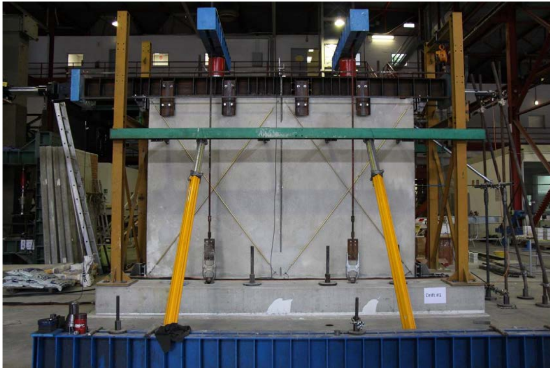
Figure 2.22: Example of specimen of precast panel tested at the Eucentre laboratory of Pavia (Italy)
