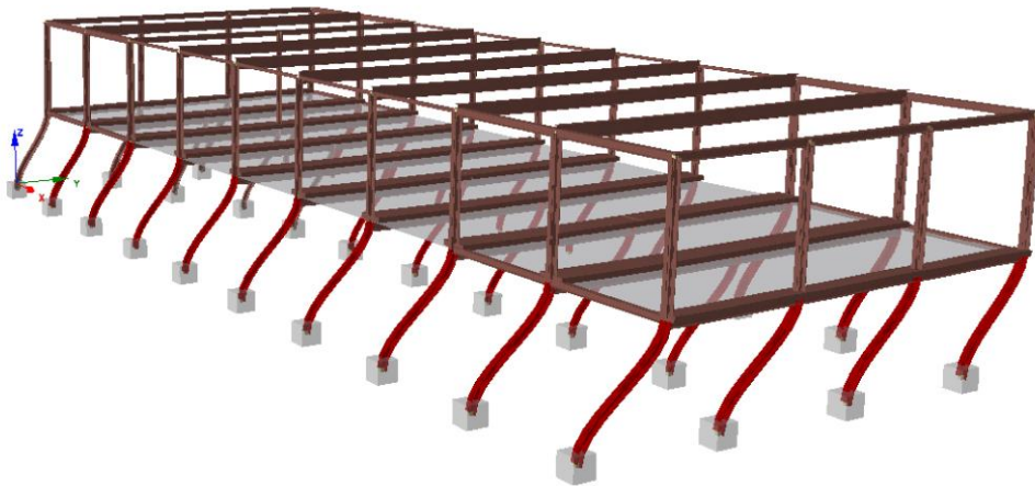
Figure 11.10: Deformed shape (trans. direction) at ultimate displacement, showing the elements (in red) that reach their rotational capacity
