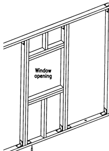
Figure 4.4: Timber Frame Residential Detached House –Detail of studs adjacent to a window opening
