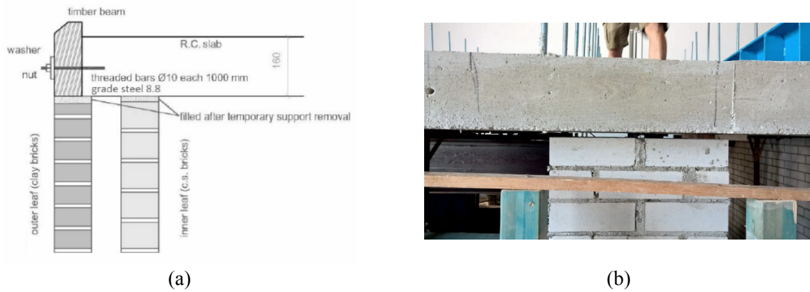
Figure A.6 Constructional details of the gap between CL walls/timber beam (a) and CS walls/RC slab (b) (Graziotti et al., 2015)
