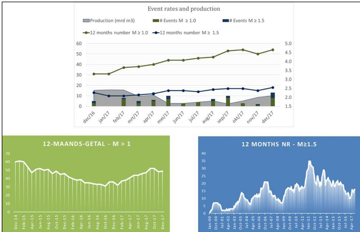
Figure 41 Temporal evolution of the activity rate for the last 12 months. The activity rate has increased somewhat in the first part of 2017 and fluctuated around the alertness level (NAM, 2017a). Lower right panel shows development of activity rate over a much longer time-period (from 2000 to 2017). The green line and the lower left panel show the development of  $M \geq 1$  earthquakes.
