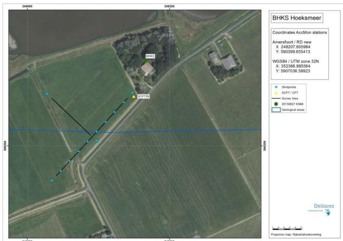
Figure 4.83 Map of location BHKS, showing the KNMI accelerograph station, SCPT location and MASW survey lines and shot locations.
