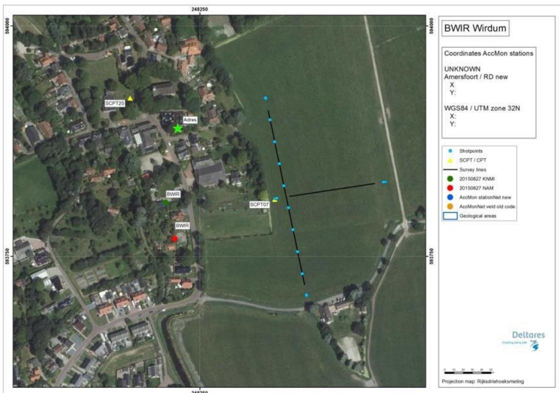
Figure 4.181 Map of location BWIR, showing the KNMI accelerograph station (exact location ambiguous), SCPT location and MASW survey lines and shot locations.
