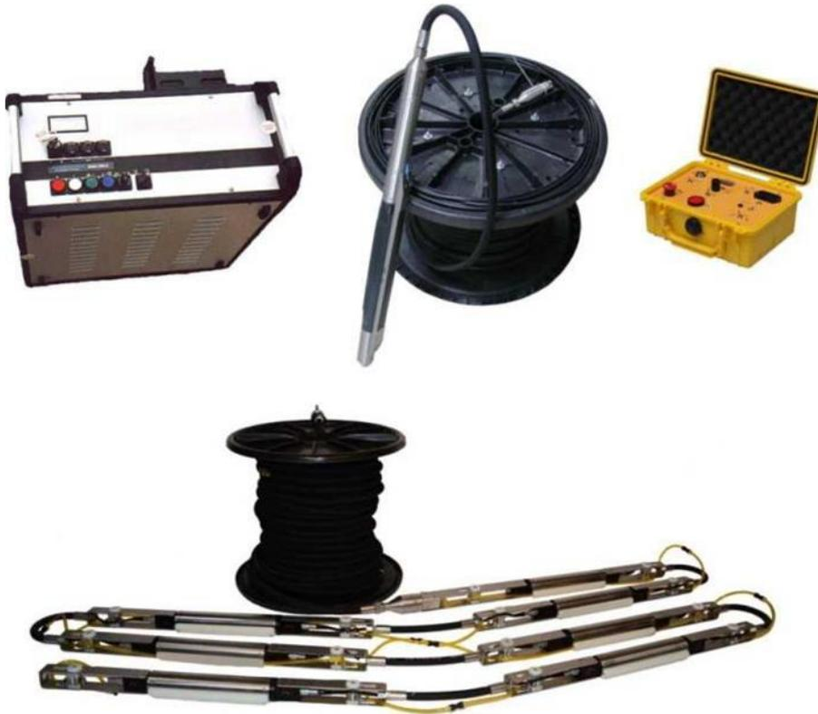
Figure 2.15 SH-wave equipment with 5 kV HV unit (upper left), down-hole probe BIS-SH (upper middle), remote control unit (upper right) and MBAS receiver (lower middle)
