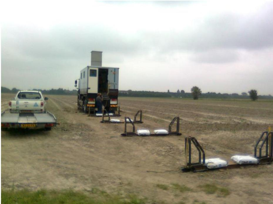
Figure 2.7 The field setup for the OSCP acquisition. A standard CPT truck with 4 additional S-wave sources (beams) with on left and right hammers. The beams have been weight down for improved coupling. Later on in the project the coupling of largest offset has been improved by adding even more weight.
