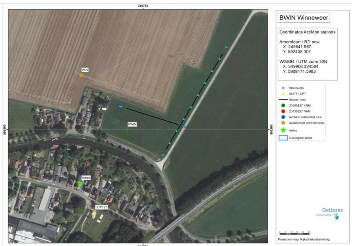
Figure 4.171 Map of location BWIN, showing the KNMI accelerograph station (exact location ambiguous), SCPT location and MASW survey lines and shot locations.
