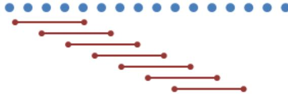
Figure 3.3 Schematic representation of CMPcc sampling, blue dots are geophones and red lined are groups of 24 channels used for each individual CMPcc. By virtually shifting the array (i.e. selecting a different group of geophones and source signals) a different section of the survey line is sampled.
