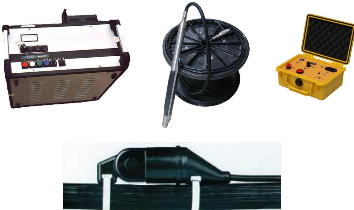
Fig. 3: P-wave tomography equipment with 5 kV HV unit (upper left), downhole probe BIS-SH (upper middle), remote control unit (upper right) and hydrophone (lower middle)
