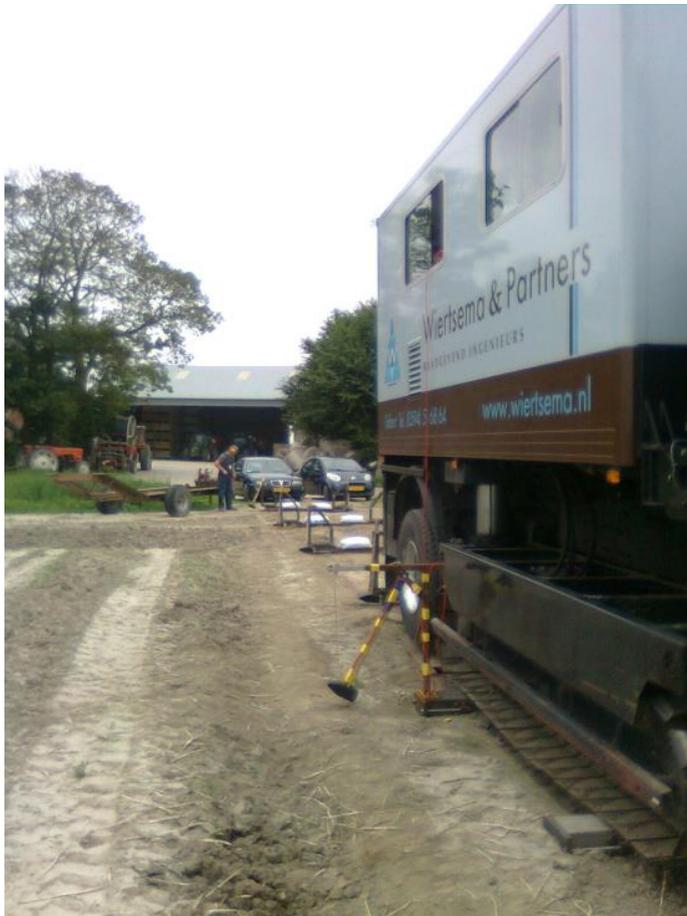
Figure 2.4 The SCPT truck with the hammer source on the side, the beam is locked under the tracks guaranteeing sufficient coupling between soil and seismic source.
