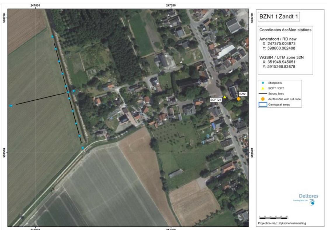
Figure 4.194 Map of location BZN1, showing the KNMI accelerograph station, SCPT location and MASW survey lines and shot locations.
