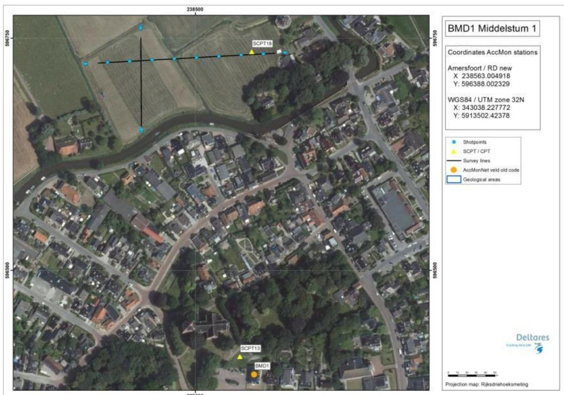
Figure 4.115 Map of location BMD1, showing the KNMI accelerograph station, SCPT location and MASW survey lines and shot locations.
