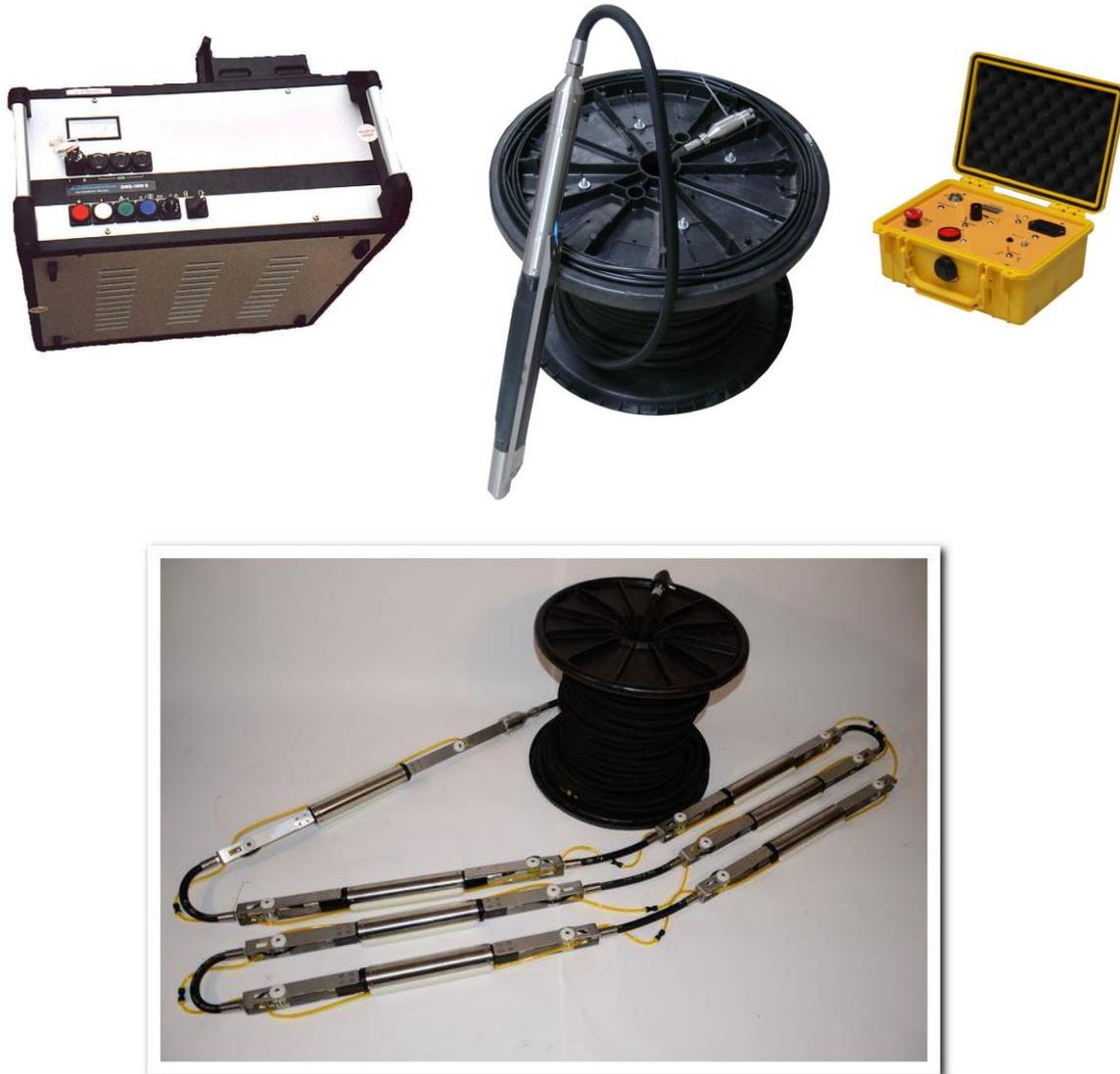
Fig. 4: SH-wave equipment with 5 kV HV unit (upper left), downhole probe BIS-SH (upper middle), remote control unit (upper right) and MBAS receiver (lower middle)
