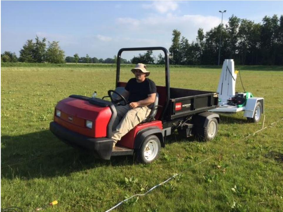
Figure 2.8 Impactor source behind towing vehicle as used in the field
