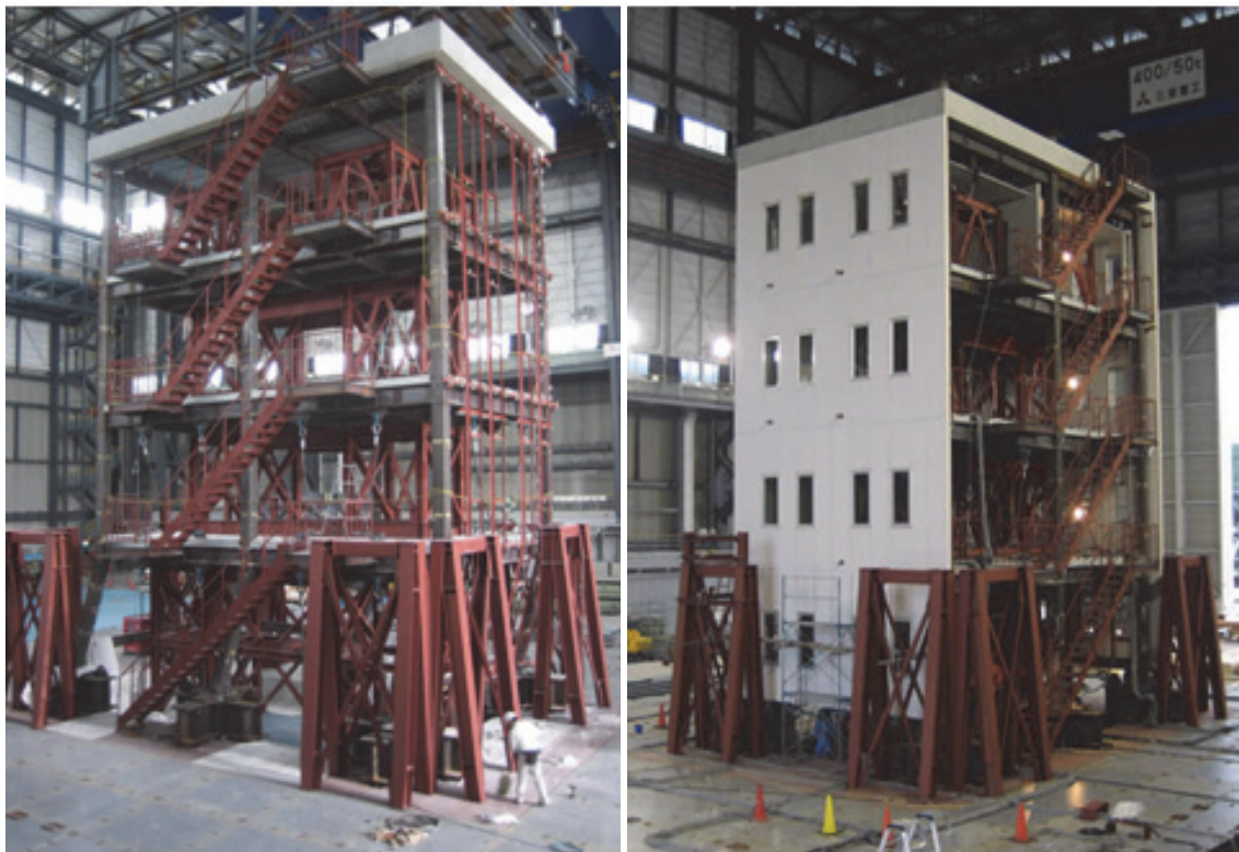
Figure 61: Four-storey 3D steel moment resisting frame (NRIESDP, 2007)
