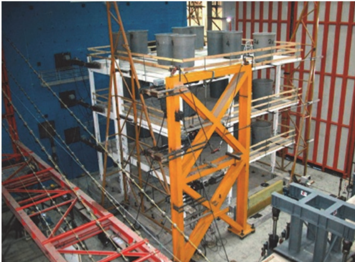
Figure 37: Three-storey full-scale RC irregular building tested at the ELSA laboratory of Ispra (Italy)
