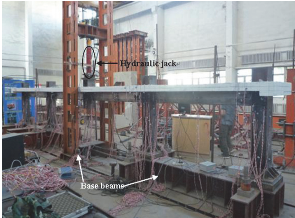
Figure 70: 1/3-scale one-storey composite frame
