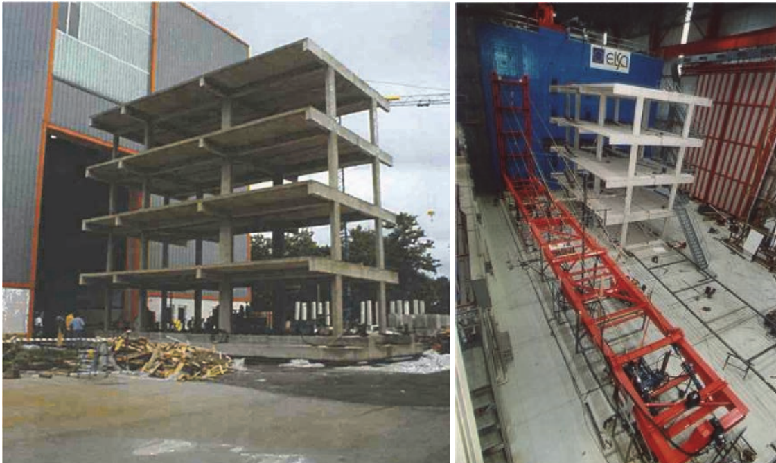
Figure 28: Full-scale four-storey RC frame tested at the ELSA laboratory of Ispra (Italy)
