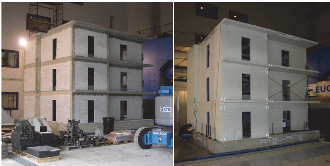
Figure 21: Half-scale three-storey RC irregular building with infill panels tested at the EUCENTRE of Pavia (Italy)
