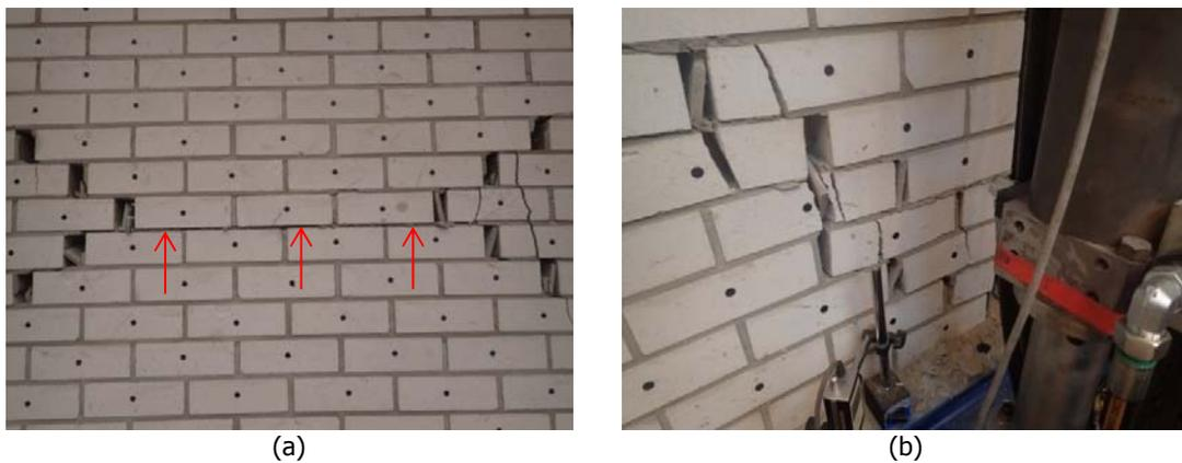
Figure 28. TUD\_COMP-4: details of the crack pattern at end stage. Crushing of the mortar bed joint at the centre of the wall (a); shearing out of the loose triangle at the bottom corner (b).
