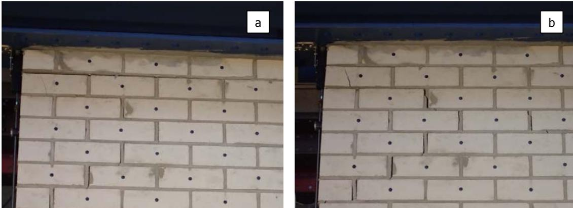
Figure 22. TUD\_COMP-3: Evolution of the crack pattern in the top portion of the wall for positive drifts: cycle 10 (horizontal crack along the bed joint - a) and cycle 11 (diagonal cracks - b).
