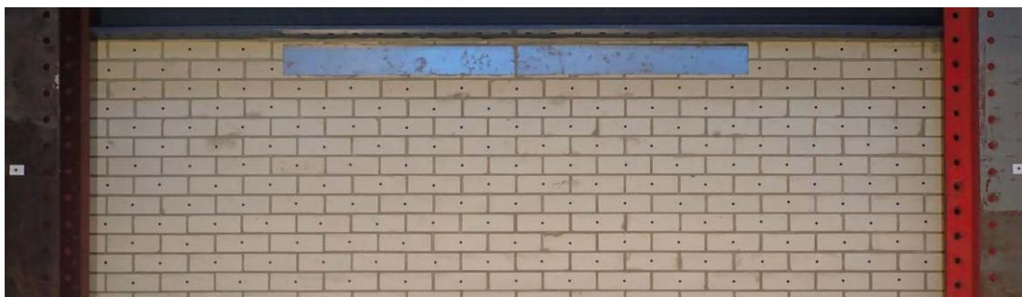
Figure 29. Detail of the repaired top bricklayer of TUD\_COMP-5.
