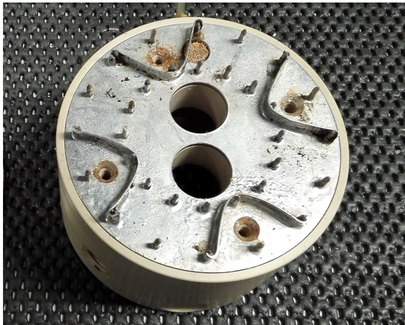
Figure 2.12: Photograph of modified top cap to improve the interlocking or contact between top cap and sample using nails and wings, test on sample Bus-13-2
