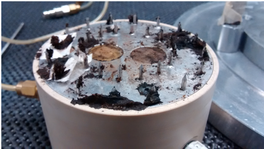
Figure 2.7: Photo of modified top cap to improve the interlocking or contact between top cap and sample using nails, after test on sample Bus-13-1
