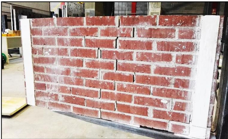
**Out-of-plane Flexural Strength Test**
