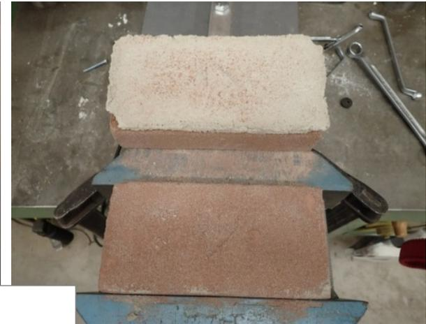
Bondwrench Test - clay brick masonry
