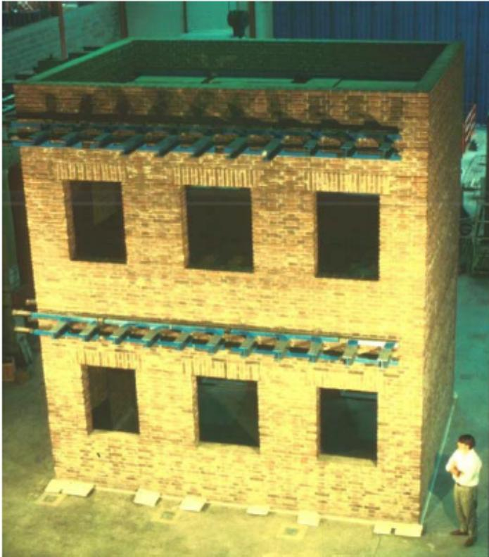
Cyclic testing in longitudinal direction
