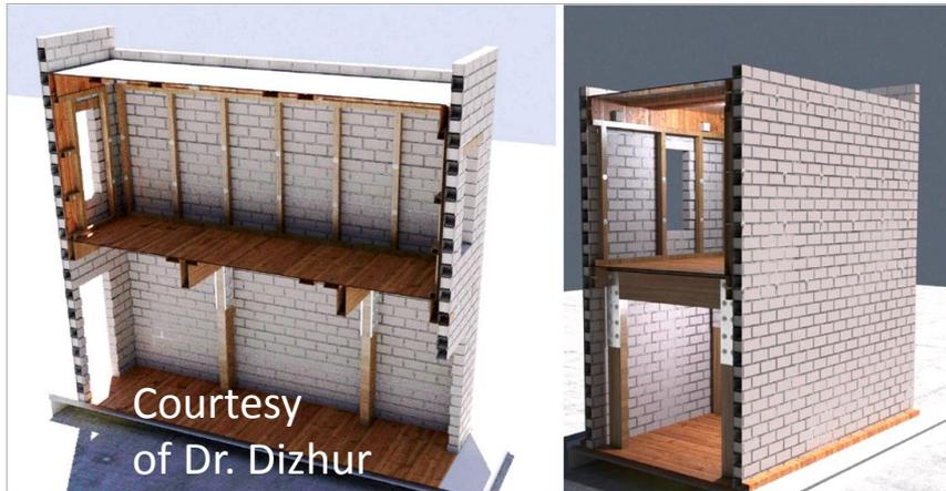
Seismic behaviour of 'light-retrofitted' terrace house
