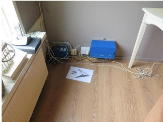
Figure VI.2 Sensors installed on the walls at: crawl space level (top), basement level (middle) and ground floor level (bottom). The large blue box of the lowermost figure is the recorder.
