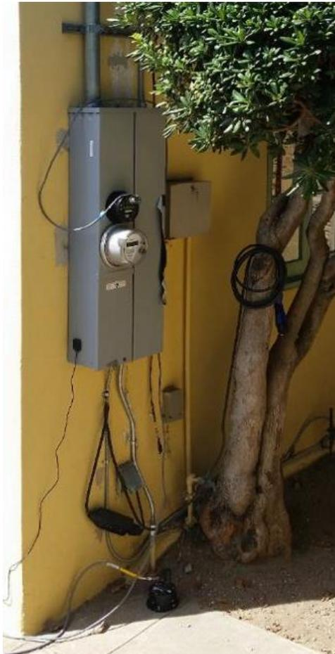
Figure VI.14. Installation of an EpiSensor accelerograph (*black*) at smart meter height and on the ground below (*image courtesy of Professor Norm Abrahamson and Professor Richard Nigbor*)
