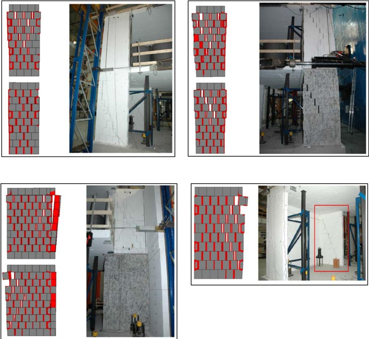
Figure 2.4.6: Crack pattern after successive loadings of 0.02g–0.20g PGAs, i.e. after final laboratory test .
