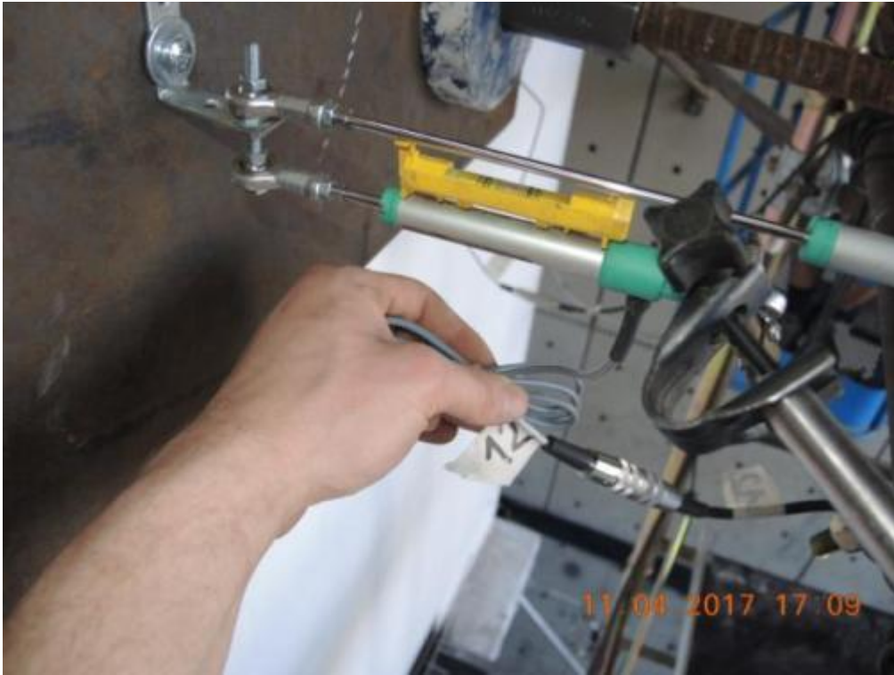
Figure 103. Detail of short and long stroke potentiometers for global displacement of the second storey.
