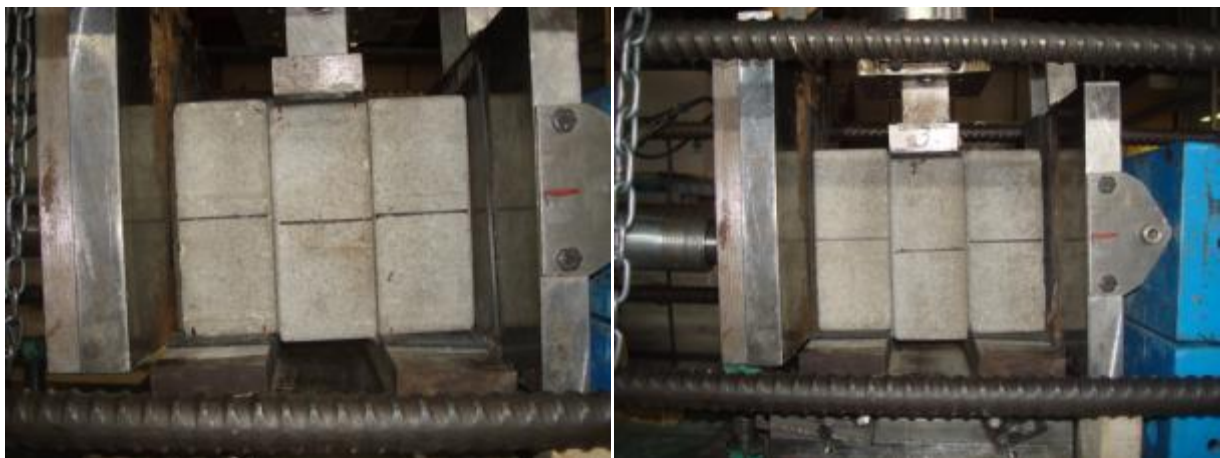
Figure 8. Examples of relative block-to-block sliding mechanism during one of the triplet test.
