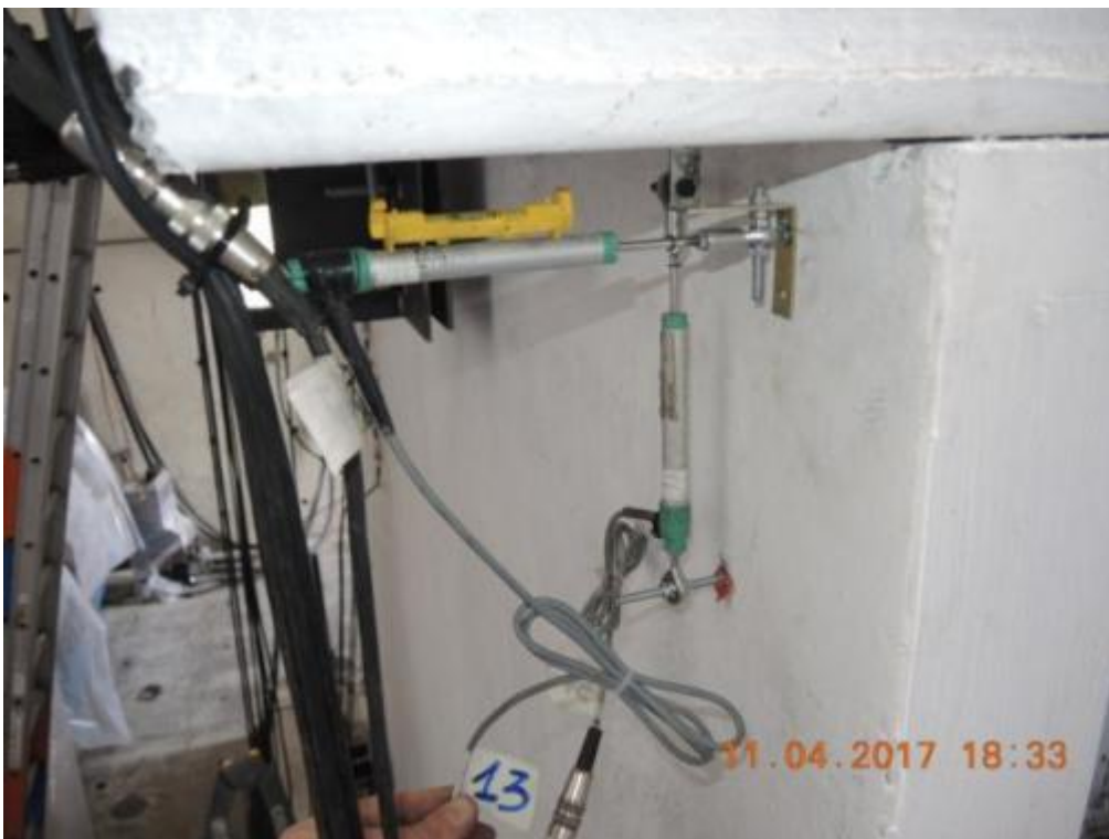
Figure 104. Instrumentation installed onto lateral walls – top of the wall.
