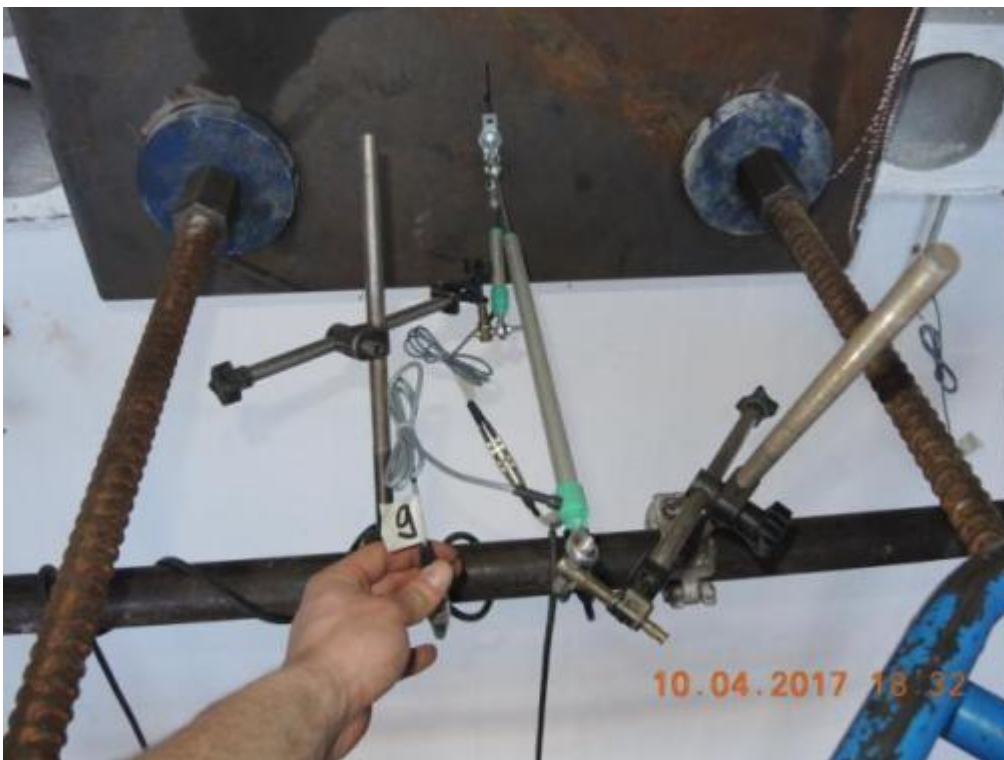
Figure 100. Instruments for global displacement of the second storey – Central slab panel.
