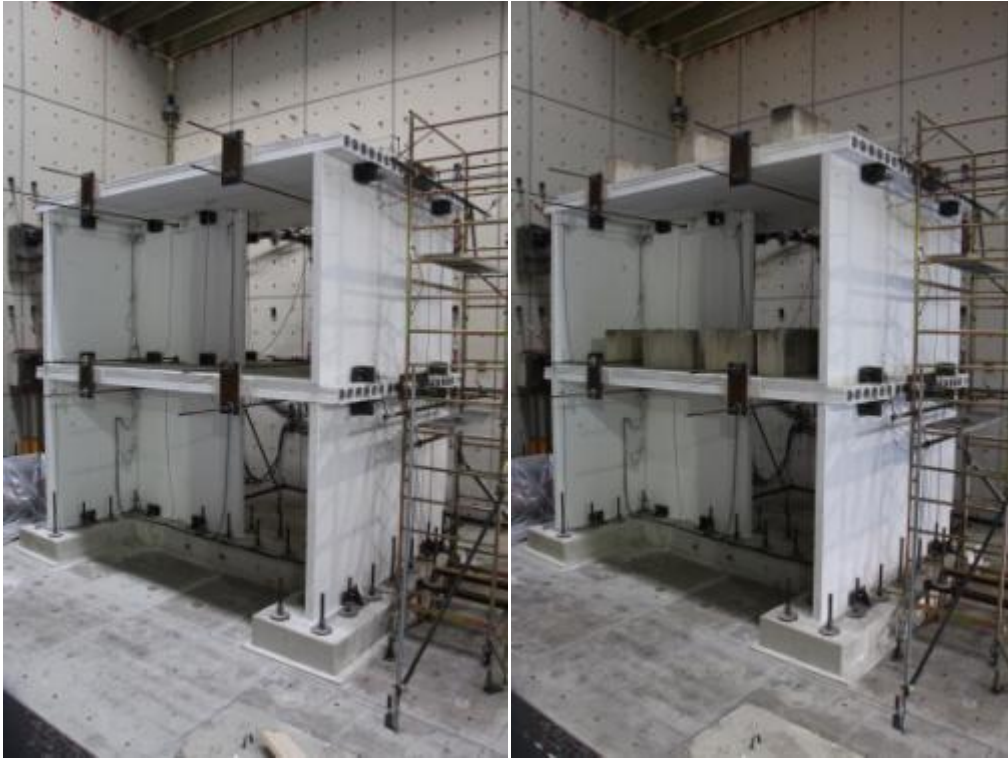
Figure 72. Photographs of the experimental set-up mounted before testing the as-built configuration.
