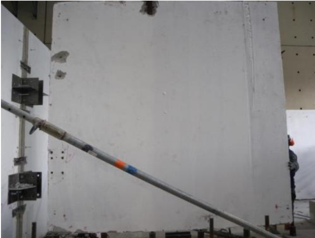
Figure 354. Uplift of dismantled ground-floor stability wall panel.
