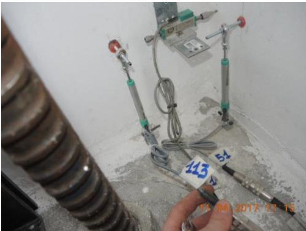
Figure 124. First-storey stability wall – Instrumentation for in-plane rocking at the base of the wall.
