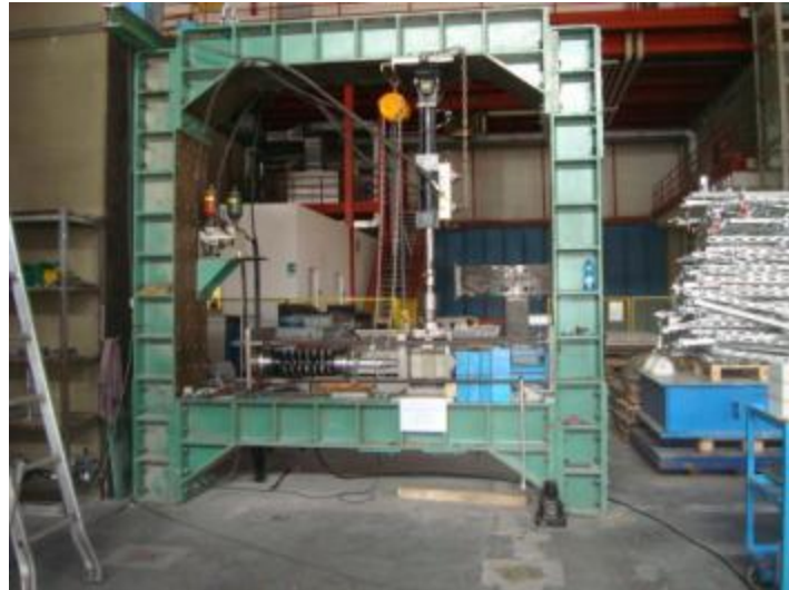
Figure 6. Experimental setup for friction testing of felt material.
