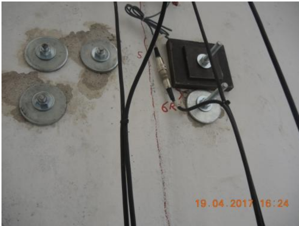
Figure 271. Evolution of crack pattern in correspondence to the implemented retrofitting intervention – Top.
