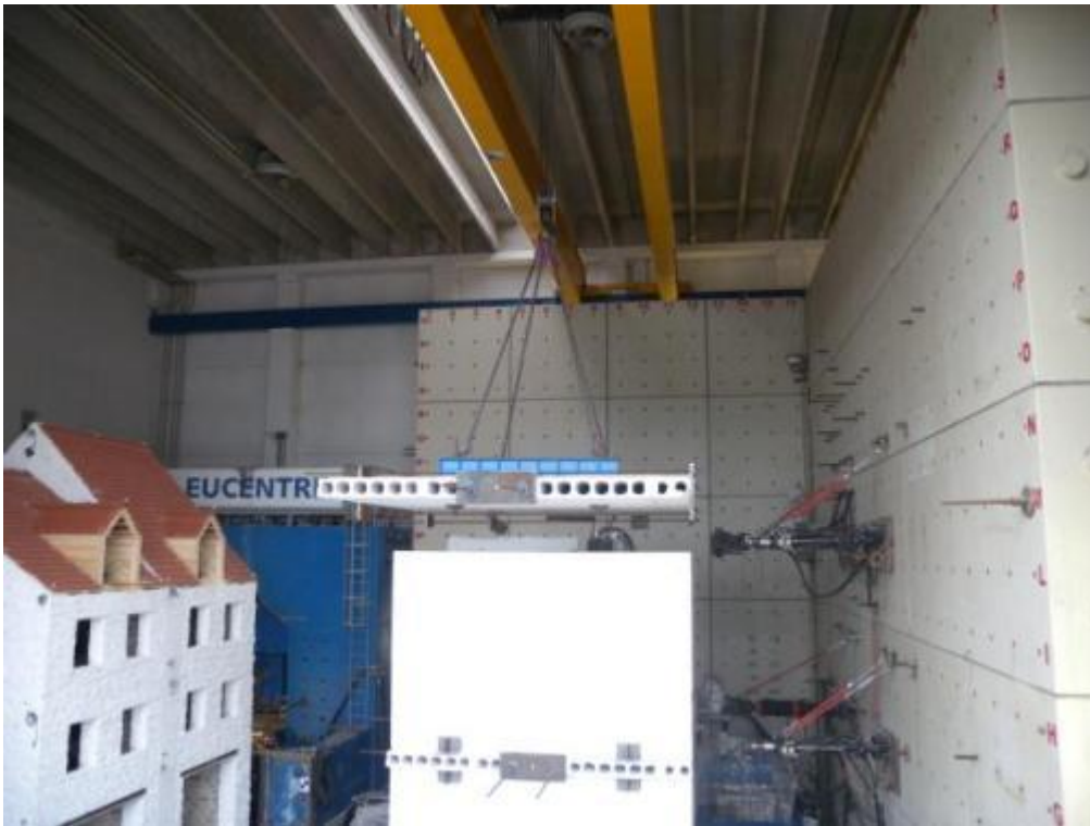
Figure 330. Uplift of second-storey flooring system without disassemblage of screed and precast panels.
