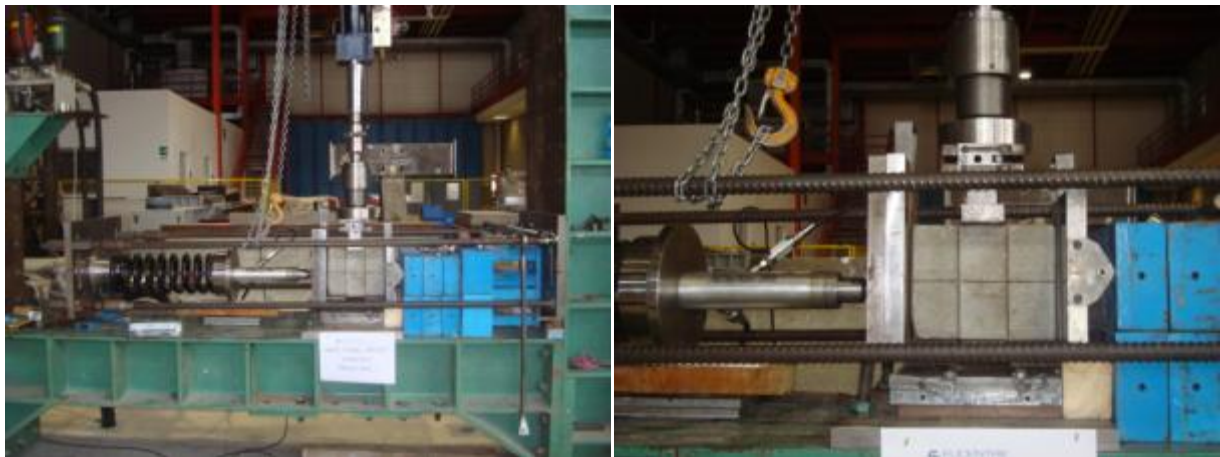
Figure 7. Testing apparatus and installed/assembled triplet specimen.
