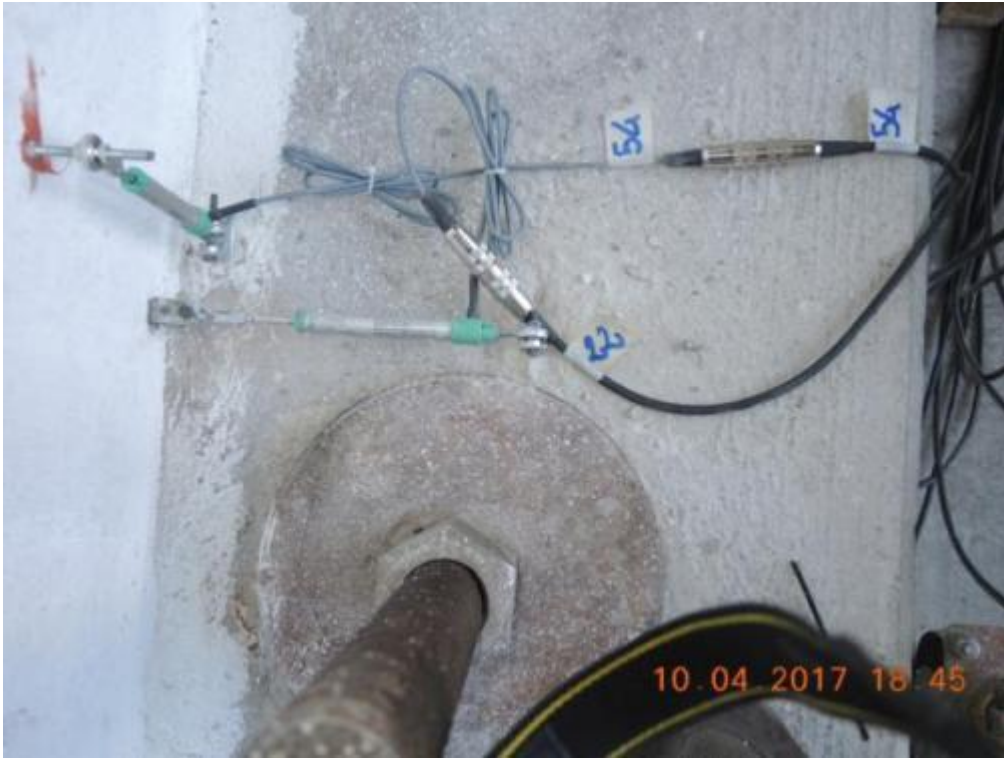
Figure 109. Instrumentation at the base of lateral walls – Opposite side of the specimen.
