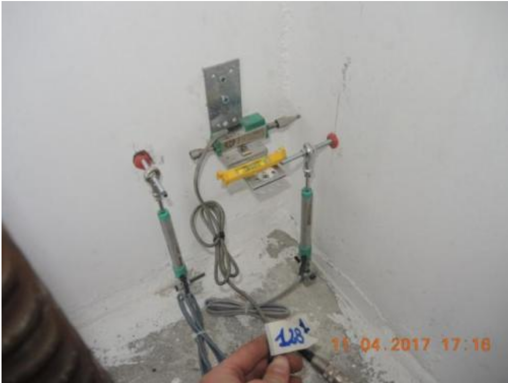
Figure 125. First-storey stability wall – Instrumentation for out-of-plane displacement at the wall base.
