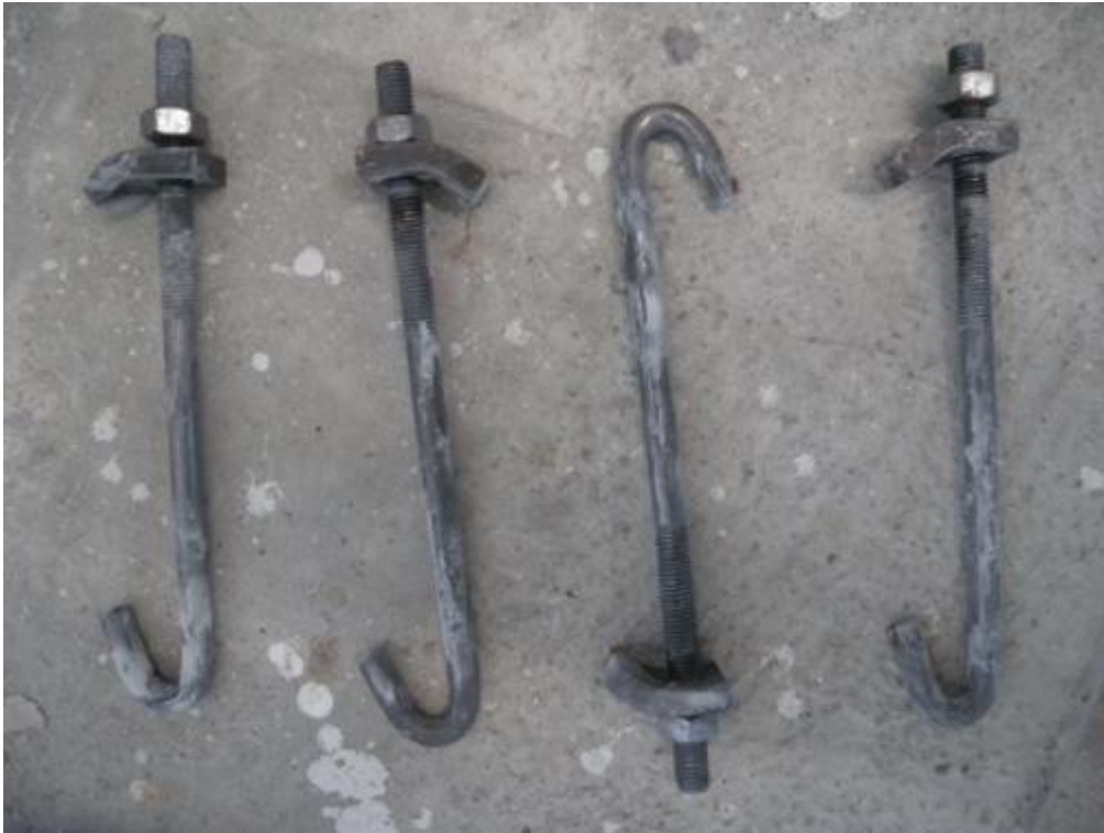
Figure 346. Detail of the four anchors for panel-to-panel connections – Lateral walls, first storey.
