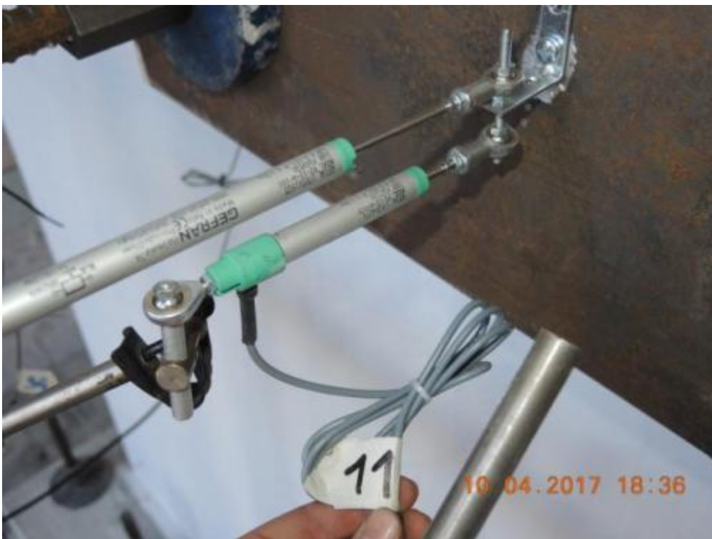
Figure 102. Global displacement of the second storey – short and long stroke potentiometers.
