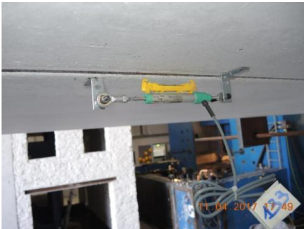
Figure 128. Detail of a 25 mm-stroke for monitoring relative displacements between slab panels.
