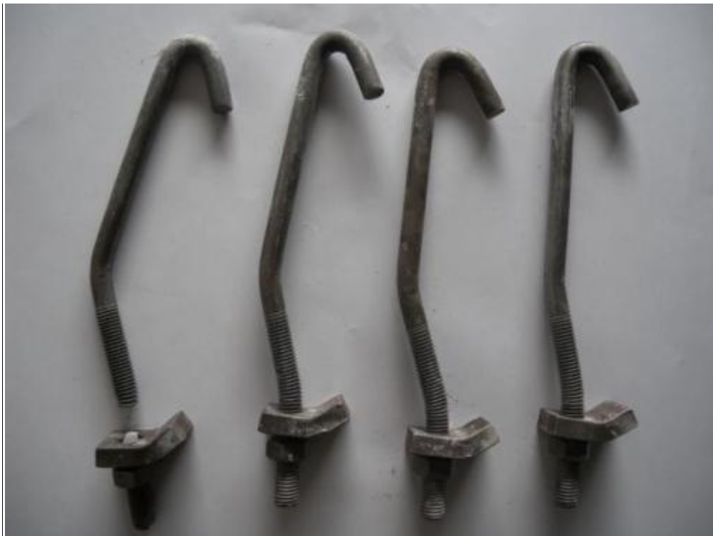
Figure 370. Permanent bending of transversal connectors in each of the four three-way joints.
