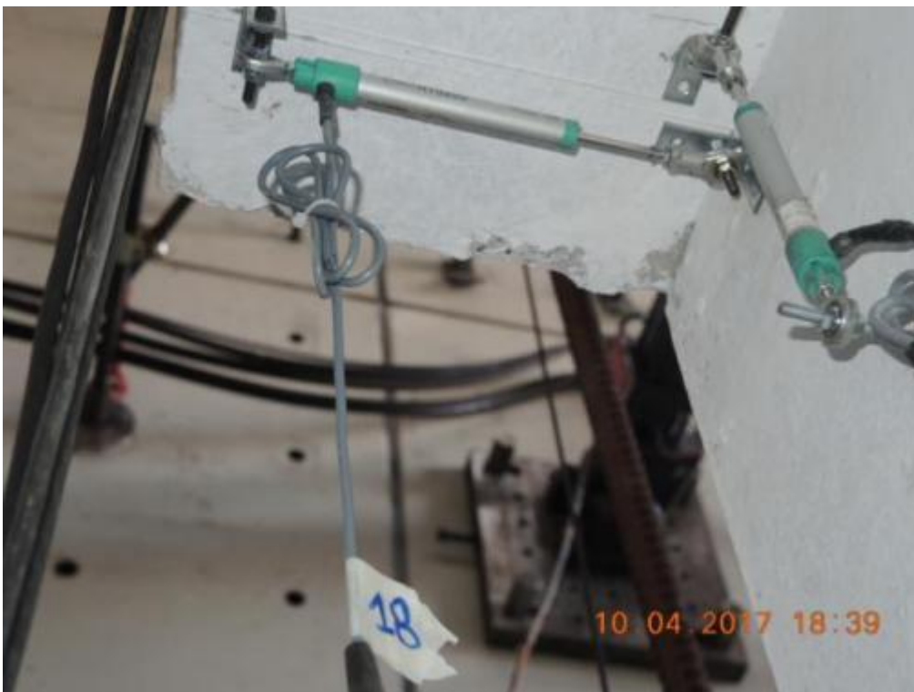
Figure 108. Instrumentation installed onto lateral walls – top of the wall, opposite side.
