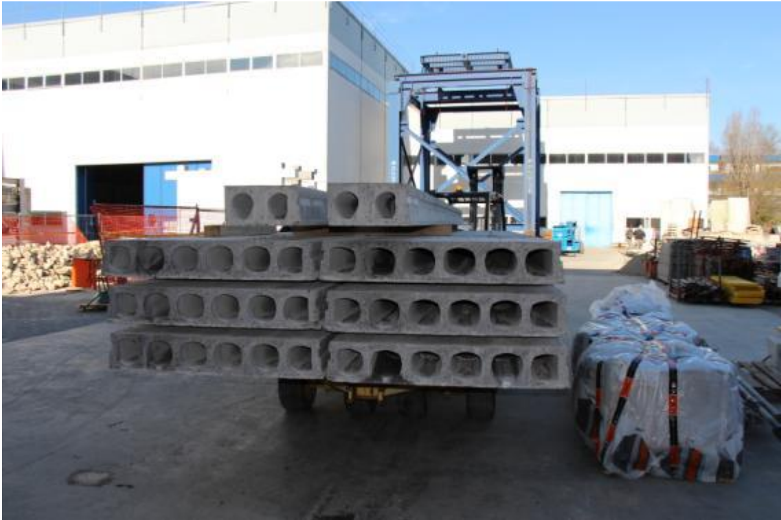
Figure 22. Examples of the two typologies of precast hollow core slabs.
