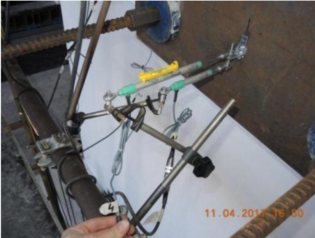
Figure 95. Detail of instrumentation for global displacement of the first storey – Central slab panel.
