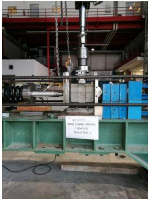
Figure 1. Triplet test for friction testing of felt material.
