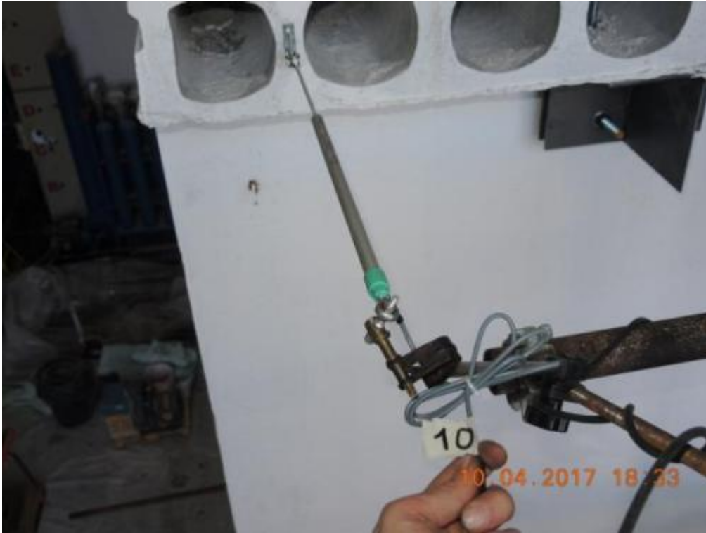
Figure 101. Instrumentation for global displacement of the second storey – Opposite lateral slab panel.
