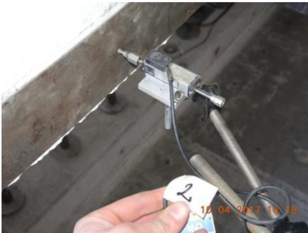
Figure 98. Detail of the instrumentation installed for uneven displacement in the transverse direction.
