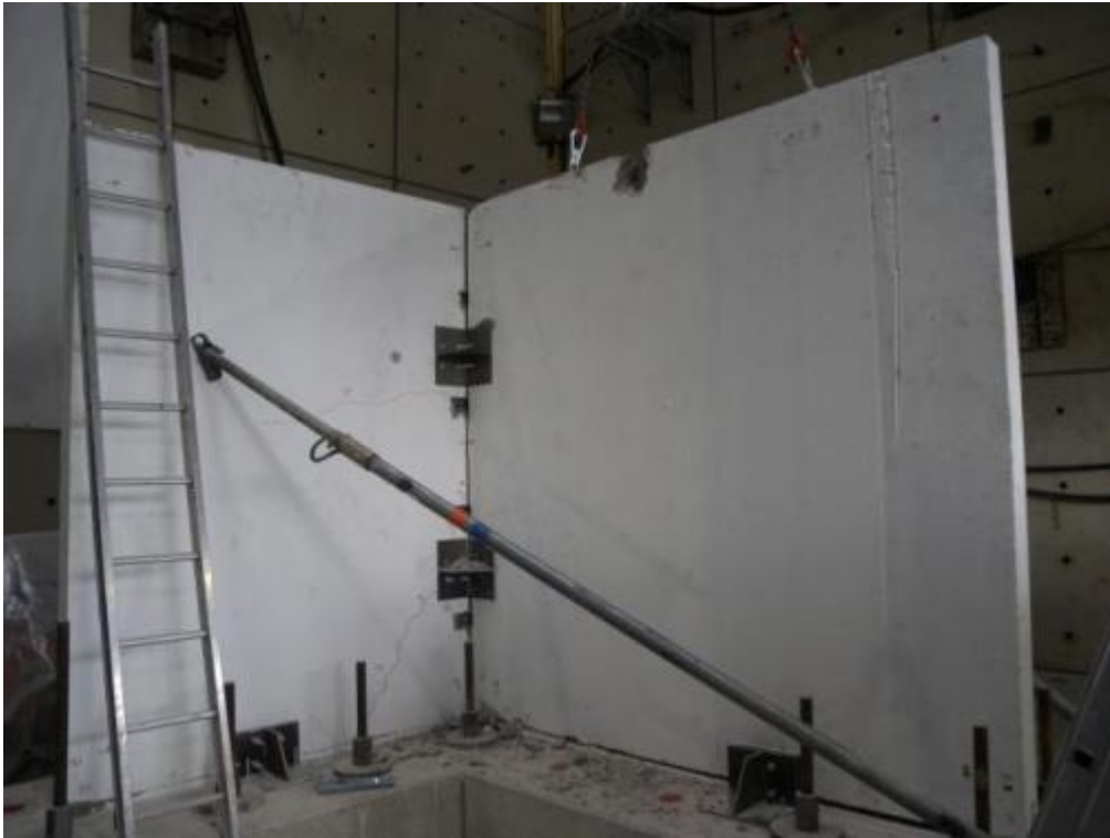
Figure 350. Ground-floor stability wall and corresponding lateral wall panel before dismantling of clip angles.
