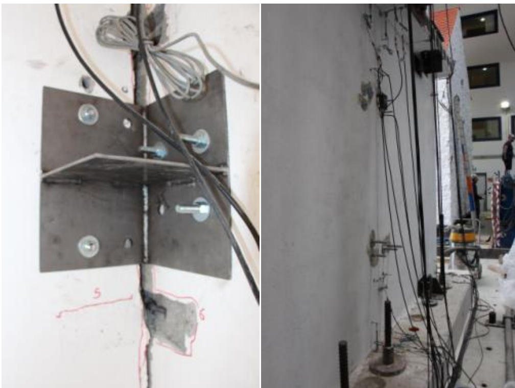
Figure 217. EUC-BUILD4 “retrofitted” specimen – Number of bolts per angle and opposite wall face.
