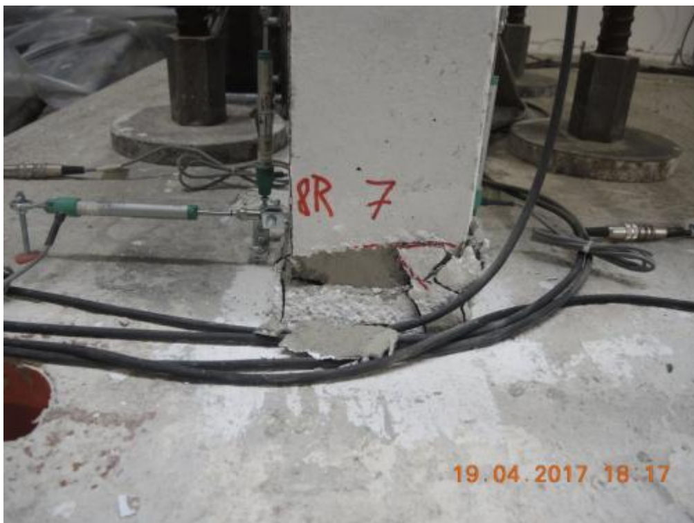
Figure 290. Concrete crushing at the base of lateral wall W1L1 – East side, lateral face.
