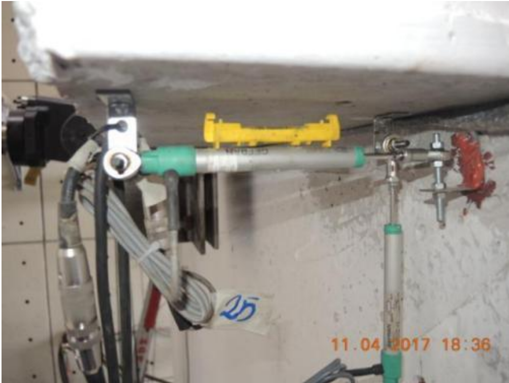
Figure 111. Instrumentation installed onto lateral walls – top of the wall, second storey.
