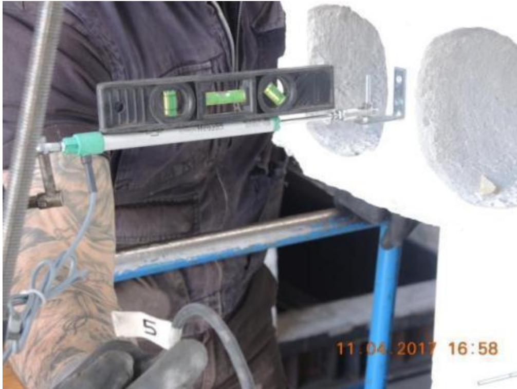
Figure 97. Detail of a potentiometer for global displacement of the first storey – Opposite lateral slab panel.
