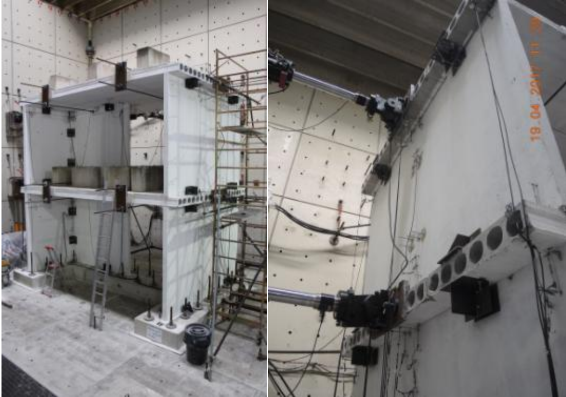
Figure 214. EUC-BUILD4 “retrofitted” specimen before test run.
