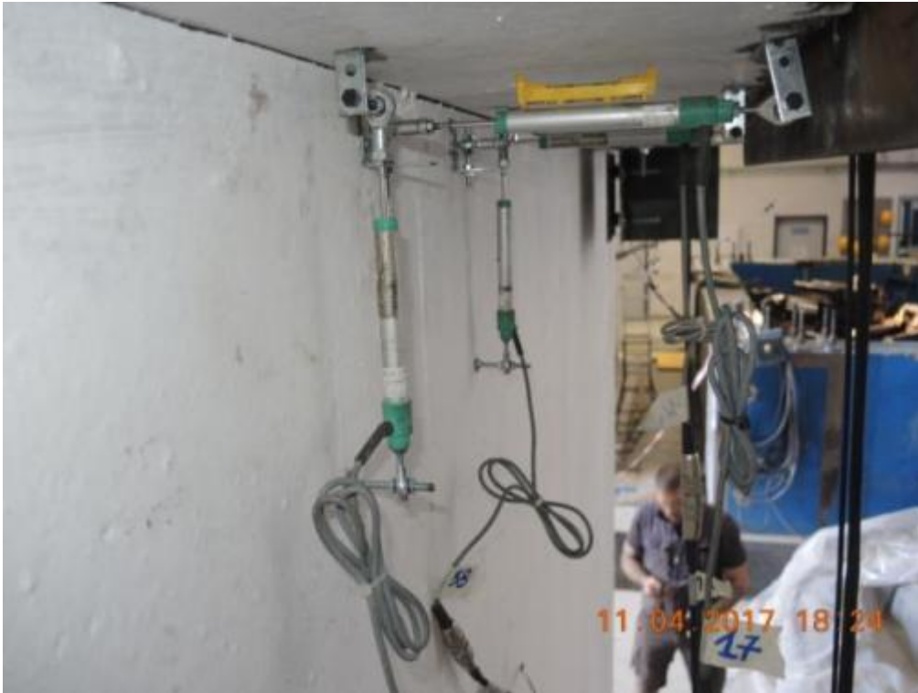
Figure 107. Instrumentation at the top of lateral walls – Central zone.
