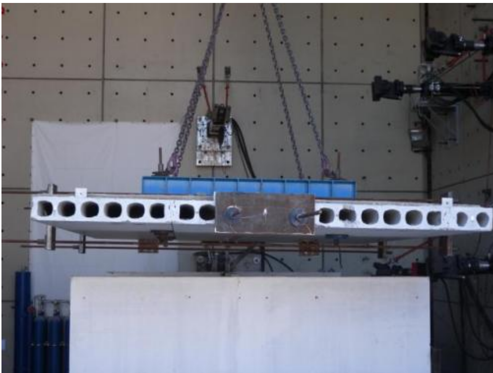
Figure 341. Uplift of first-storey flooring system without disassembling concrete screed and precast panels.
