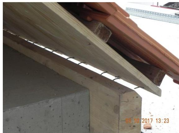
*Figure 6.8 Damage after the 350 mm pushover – West side.*
