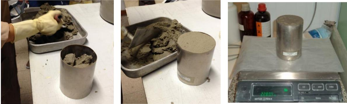
Figure 2.5 Carrying out the determination of bulk density of fresh mortar.
