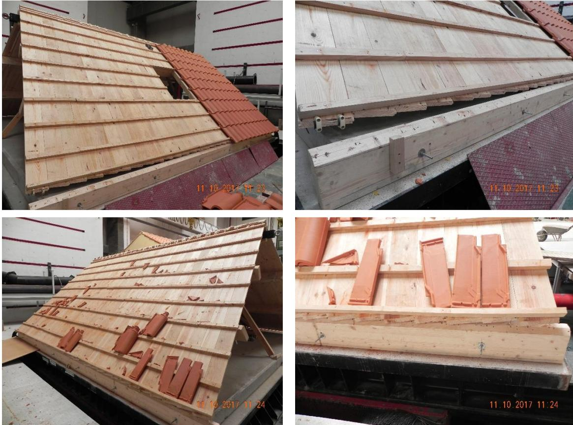
*Figure 6.13 Distortion of timber planks.*
