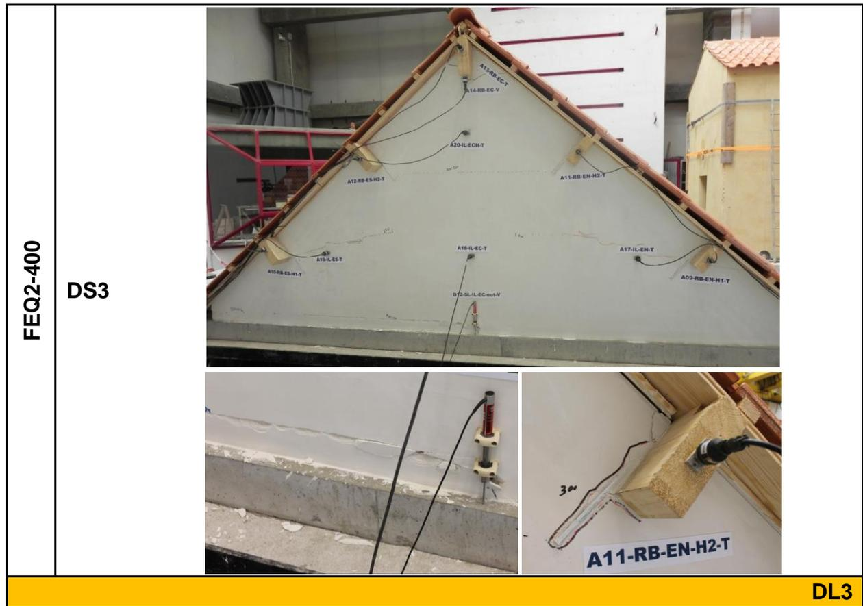
Figure 5.53 Evolution of damage in the gable walls up to DL3.
