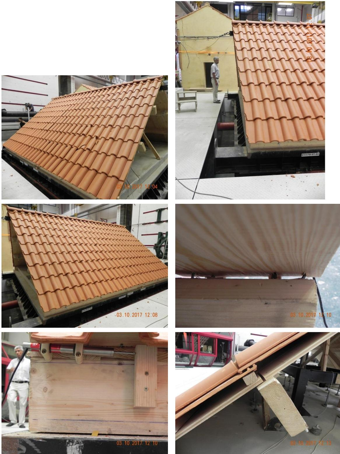
Figure 6.6 Damage after the 220 mm pushover.
