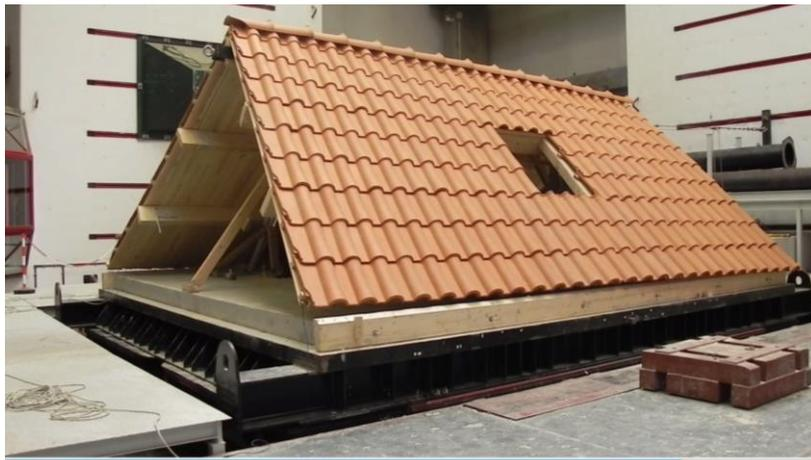
*Figure 6.7 Video images of the damage during the 350 mm pushover.*
