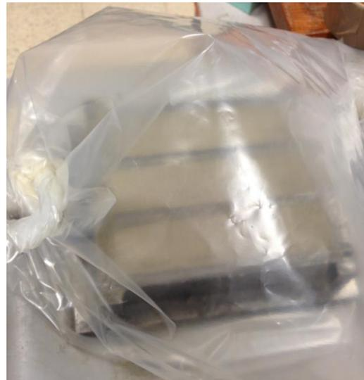
*Figure 2.8 Curing conditions of mortar specimens.*
