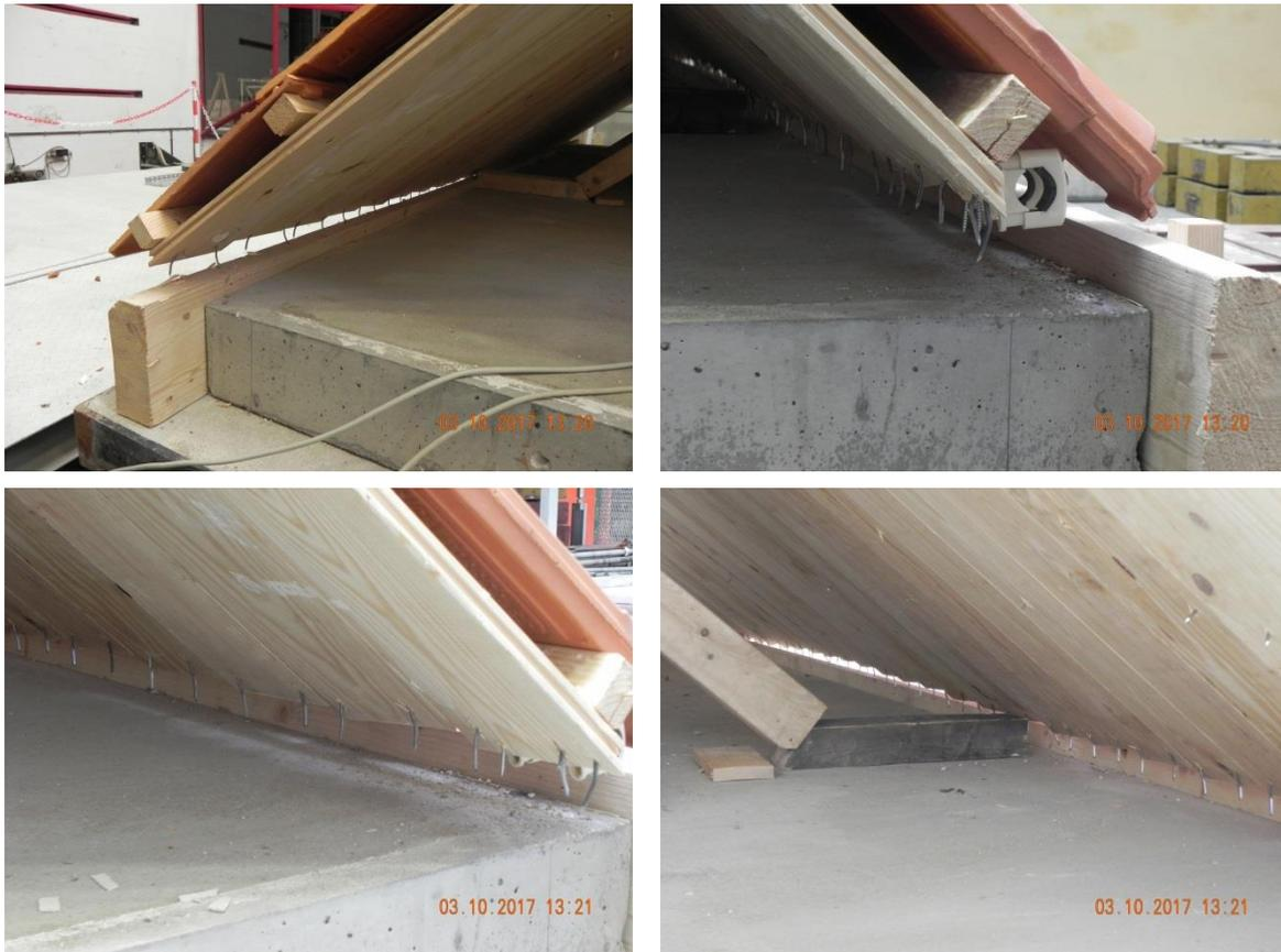
Figure 6.9 Damage after the 350 mm pushover – East side.
