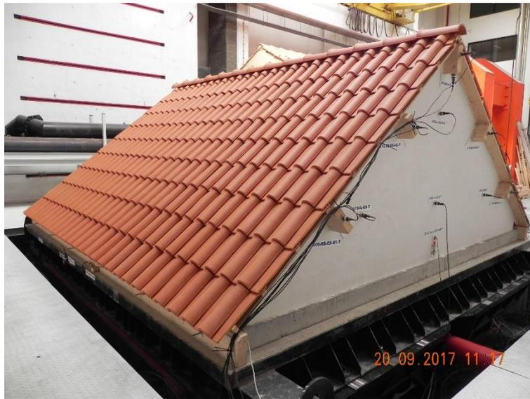
Figure 5.10 Test specimen fully instrumented on the shake table.
