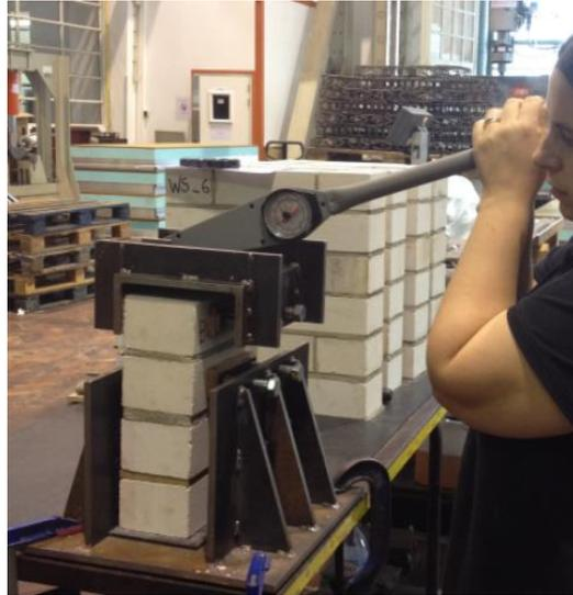
Figure 2.98 Application of vertical force until bond failure.
