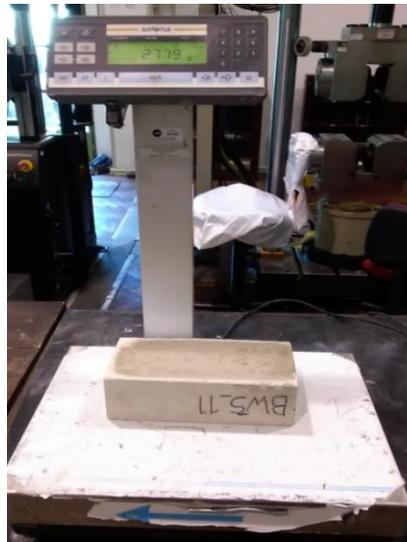
Figure 2.99 Measure of the weight of the top unit and adherent mortar.
