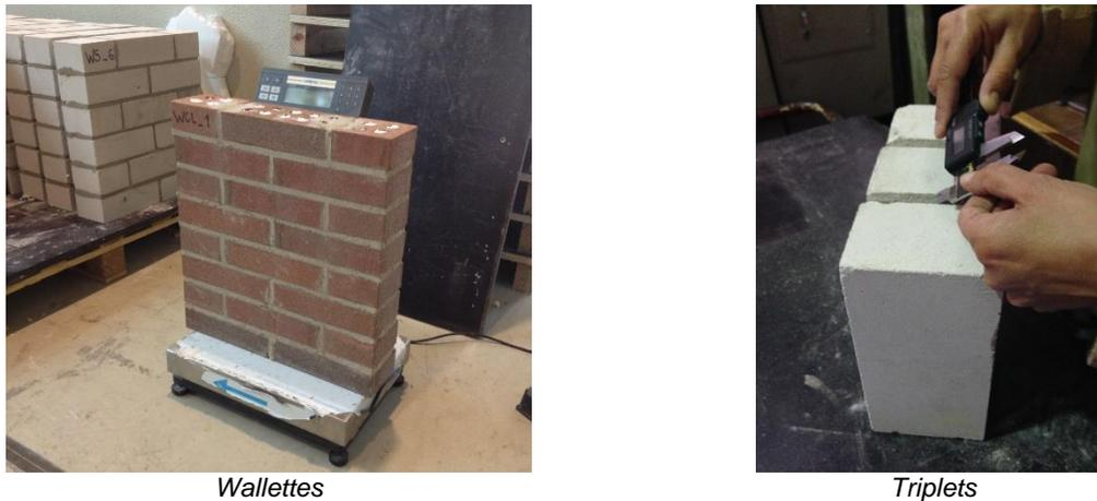
Figure 2.46 Example of characterisation (measure and weight) of all specimens.
