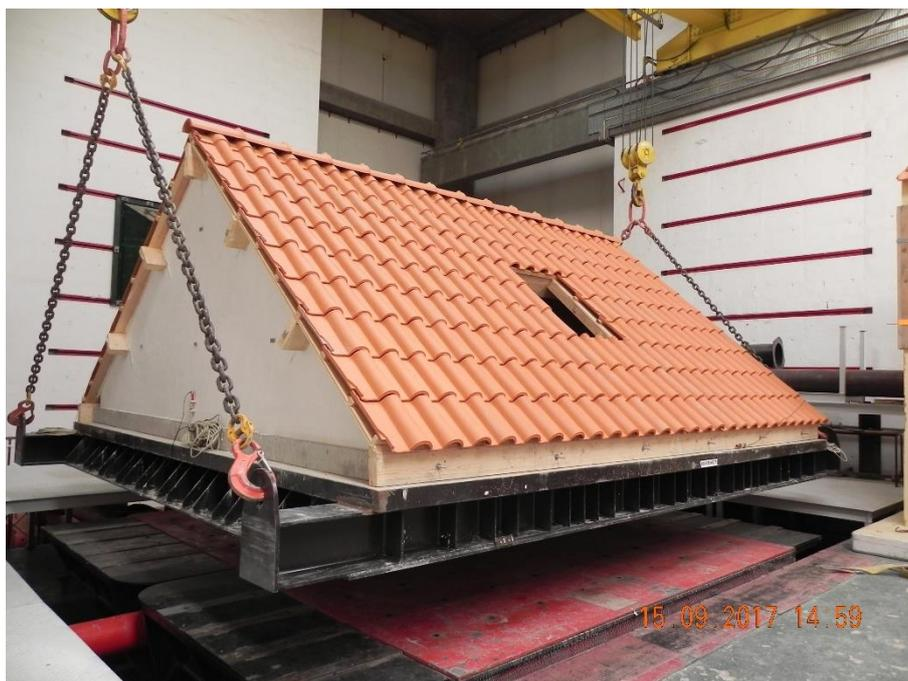
Figure 5.1 Specimen transportation to the shake table.
