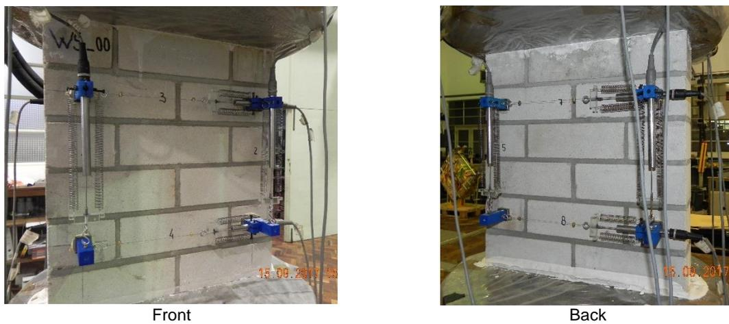
Figure 2.54 Instrumentation placed on each face of the CS wallettes.
