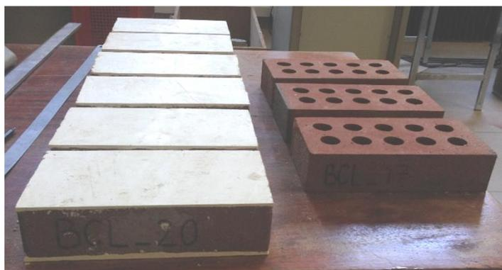
Figure 2.42 Clay bricks tested with different surface smoothing techniques.
