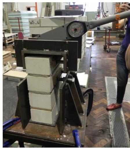
Figure 2.96 Test of the two connections in CS blocks using the same test device.
