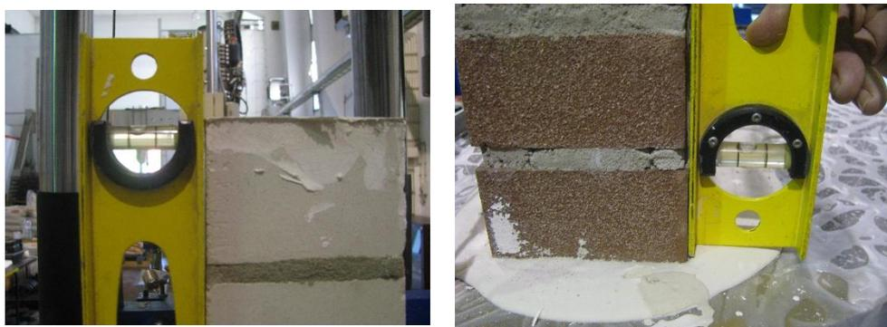
Figure 2.50 Lack of verticality in wallettes.
