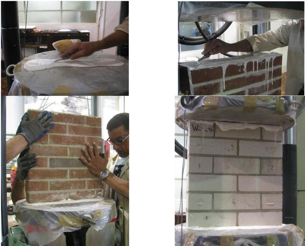
Figure 2.49 Final regularisation of the wallettes' faces on top of the testing machine.
