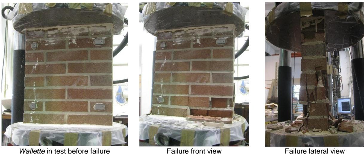
Wallette in test before failure
