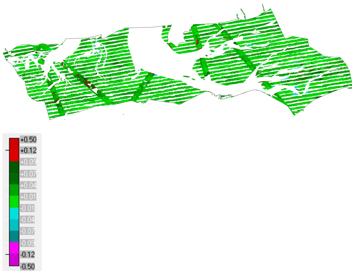
Figure 6.1 Height difference grids of the strip overlaps; color bar is in meters.
