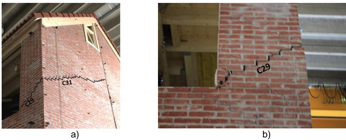
Figure 174 EQ-NPR 100% cracks: a) C29, C31 overview; b) C29 zoom in.
