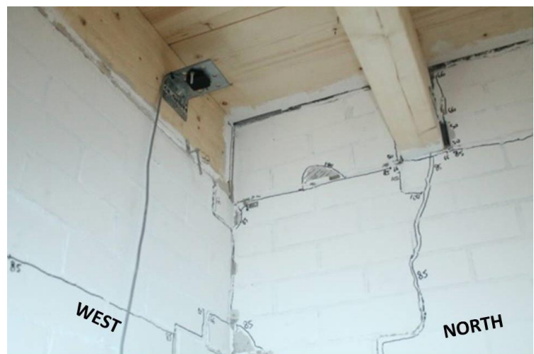
Figure 189 Crack C4 after EQ-NPR 100%: a) overview; b) zoom in.
