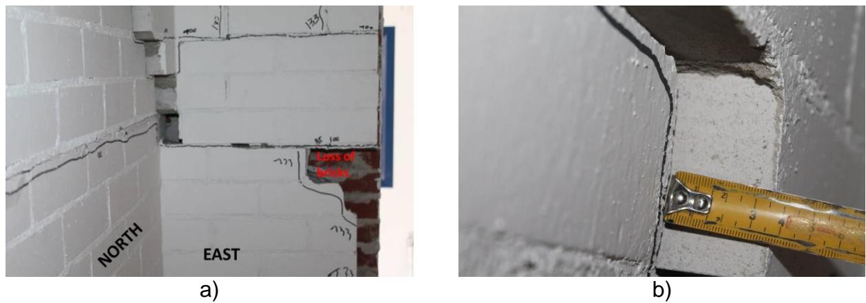
Figure 194 Cracks C13 after EQ-NPR IS 133%: a) looking East; b) Out-of-plane residual width zoom in.
