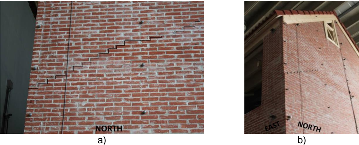
Figure 198 Crack C31: a) after EQ-NPR 85%; b) after EQ-NPR 100%.
