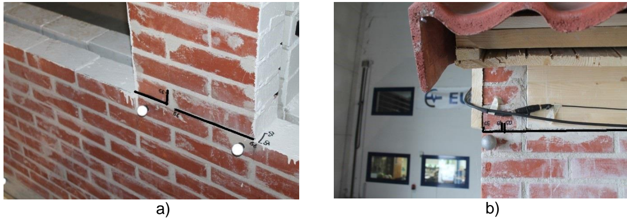
Figure 157 EQ-NPR 66% cracks: a) C23; b) C25.
