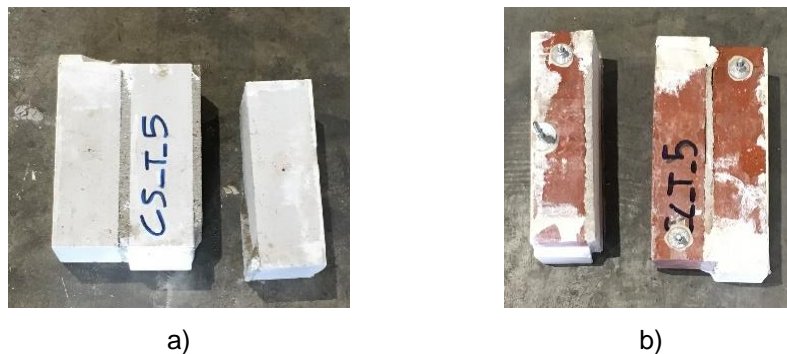
Figure 90 Shear test: a) CS specimen; b) CL specimen.
