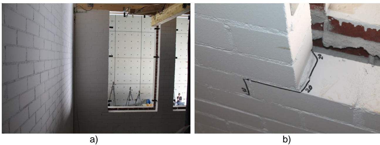
Figure 135 EQ-NPR 20% Cracks on the West facade: a) overall view; b) window corner.
