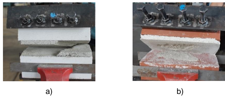
Figure 86 Examples of the tested specimens: a) CS masonry; b) CL masonry.
