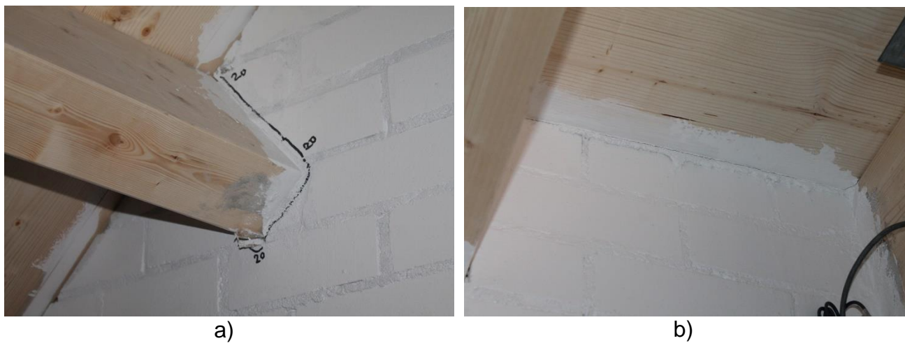
Figure 134 EQ-NPR 20% Cracks view: a) South façade roof joist-to-wall connection; b) plank-to-wall interface.
