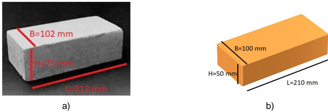
Figure 50 Brick dimensions: a) calcium silicate; b) clay.
