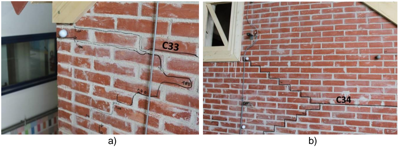
Figure 172 EQ-NPR 100% cracks: a) C33; b) C34.
