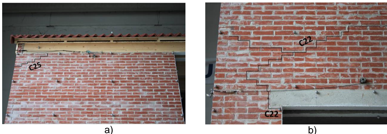
Figure 165 EQ-NPR 85% cracks: a) C25; b) C22.
