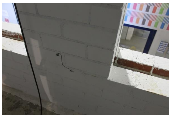
Figure 156 EQ-NPR 66% cracks: C10 overview.
