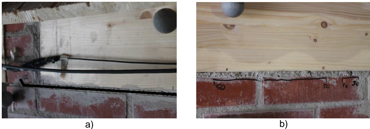
Figure 149 EQ-NPR 50% sliding cracks: between timber spreader beam and West façade outer leaf: a) North end; b) mid-span.
