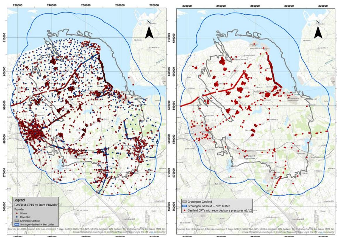
Figure 4.1 Map of CPT locations in the Rockworks® database (left), CPT's with pore pressures  $u_1/u_2$  (right).
