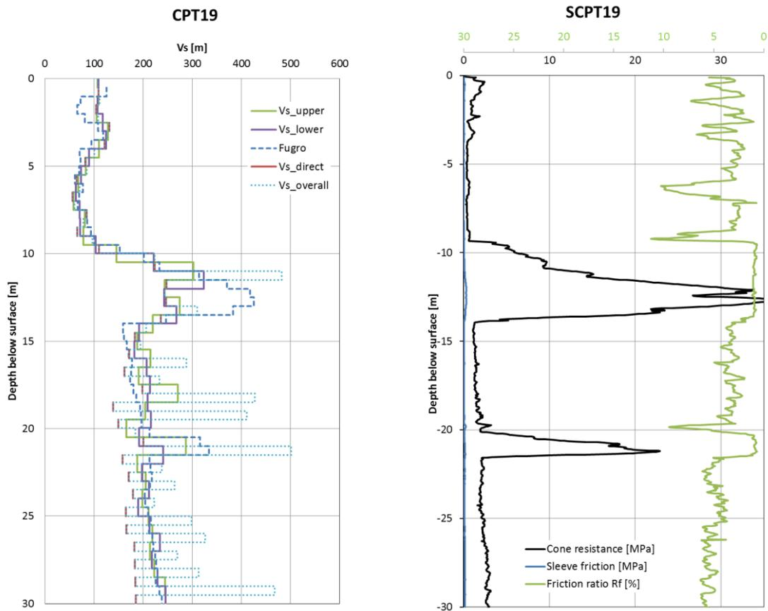
Figure 5.3 Left:  $V_s$  interpreted by Fugro and reprocessed  $V_s$  by separation of direct ( $V_{s\_direct}$ ) and pseudo interval travel times ( $V_{s\_upper}$  and  $V_{s\_lower}$ ). Right: corresponding CPT readings indicating relatively homogeneous Pleistocene clay between 14 and 30 m, separated by a sand layer between 20 and 22 m (de Lange et al., 2017).
