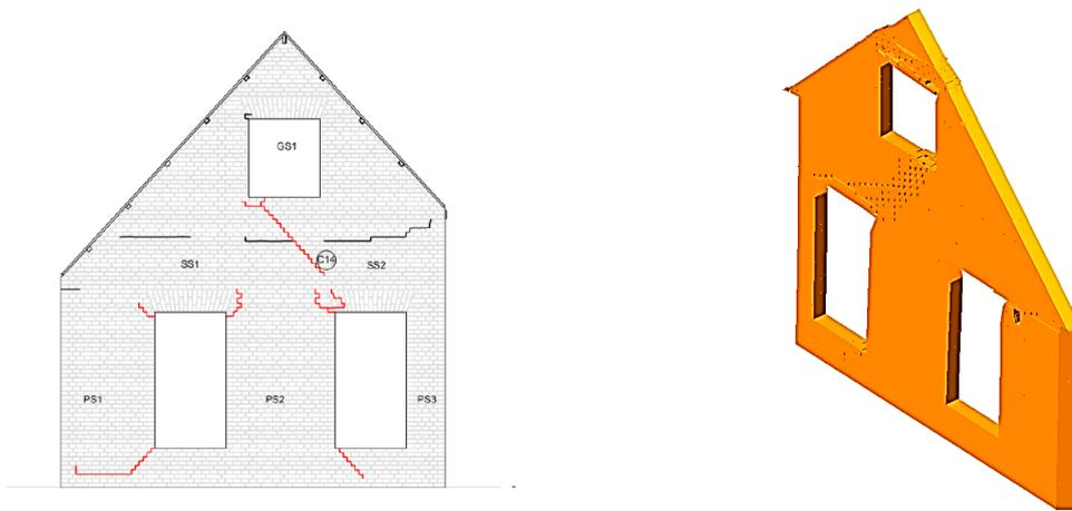
Figure 30 EQ2@300 \_ Experimental (left) and numerical (right) damage plot of South wall
