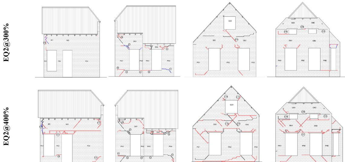
Figure 21 Significant damage detected at EQ2@300 and EQ2@400, (Graziotti et al. 2016)
