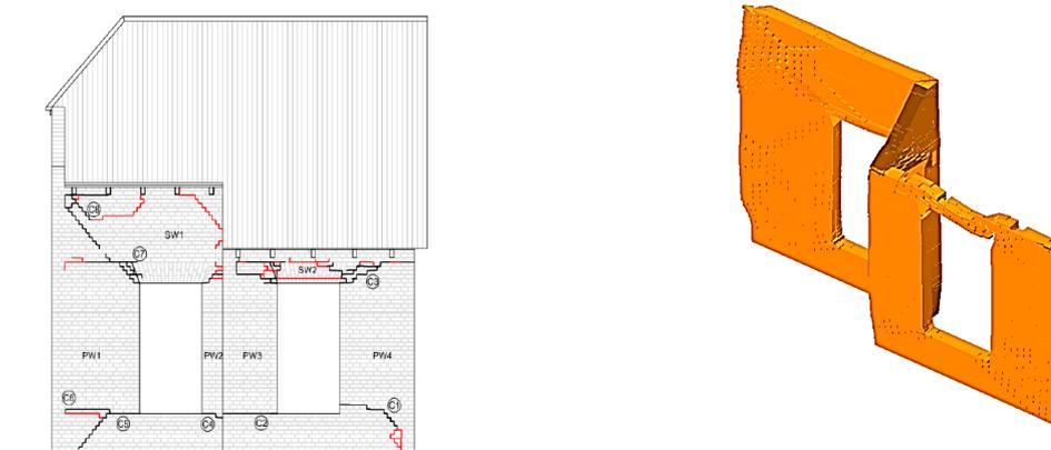
Figure 31 EQ2@400 \_ Experimental (left) and numerical (right) damage plot of West wall
