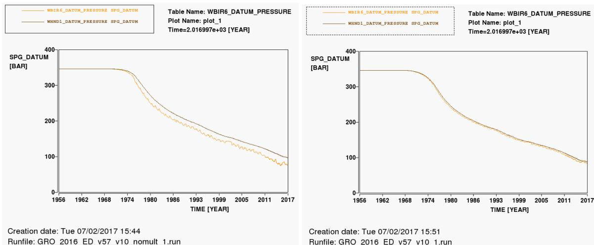
**Figure 31** Both figures show the model output for BIR-6 and HND-1, without permeability increase in the north (left) and with permeability increase in the north (right).
