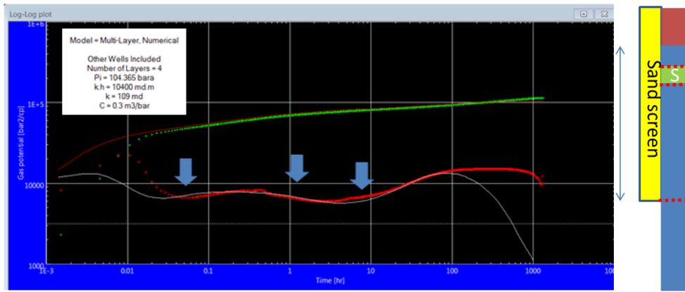
Figure 40: Numerical simulation with 1 high permeability streak in connection with the Sand Screen and a kv/kh of 0.1 and reservoir permeability of 100 mD. The fault model is depicted in Figure 41.
