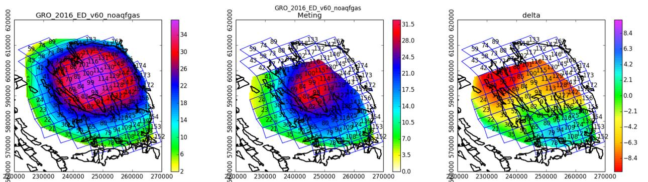
**Figure 28: Scenario 1 – Subsidence proxy calculation for a model without gas in the aquifer**
