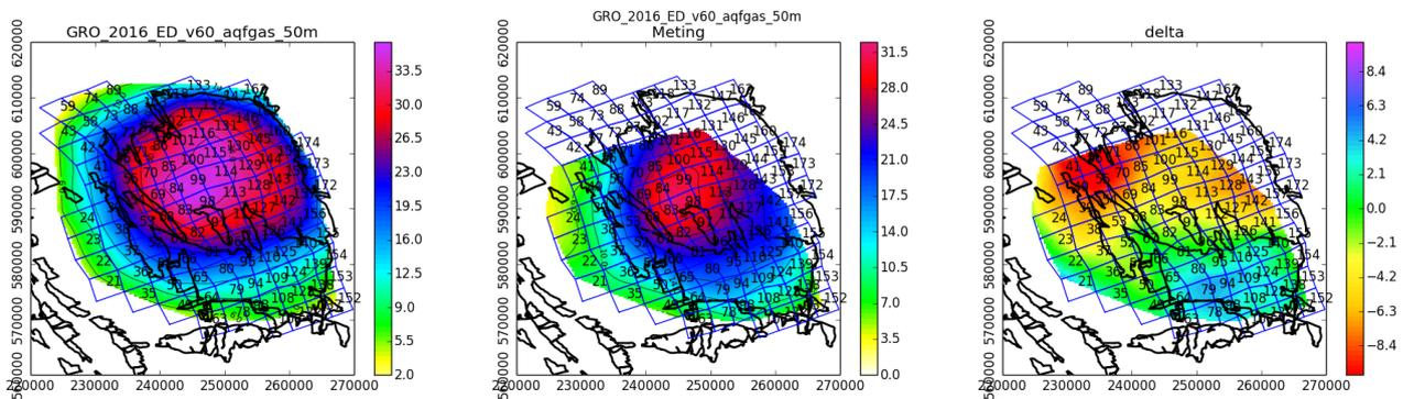
**Figure 29: Scenario 2 – Subsidence proxy calculation for a model with 10% gas in the aquifer down to a depth of 50 m below the free water level**
