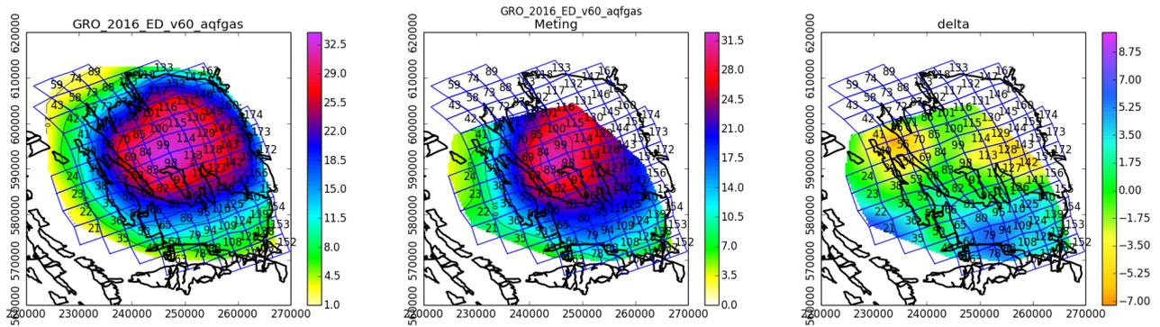
**Figure 30: Scenario 3 –Subsidence proxy calculation for a model with average gas saturations below the free water level distributed based on open-hole measurements**
