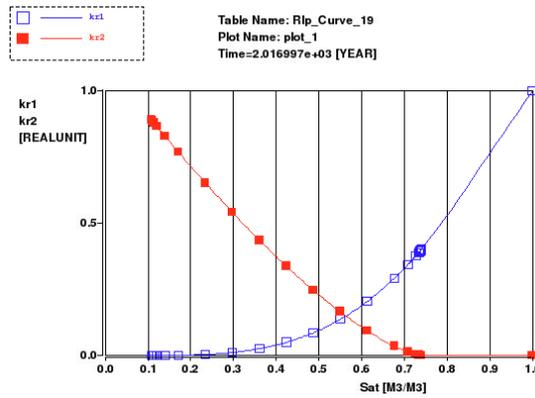
**Figure 27: Gas (kr2-red) and water (kr1-blue) relative permeability curves for 19% porosity shown as a function of water saturation**
