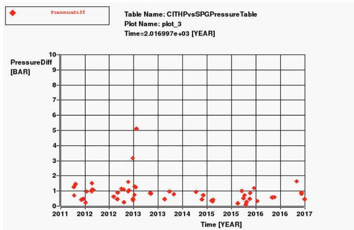
**Figure 35** difference between model output for SPG and converted closed-in tubing head pressure (a positive value means the modelled SPG pressure is higher than the modelled closed-in tubing head pressure).
