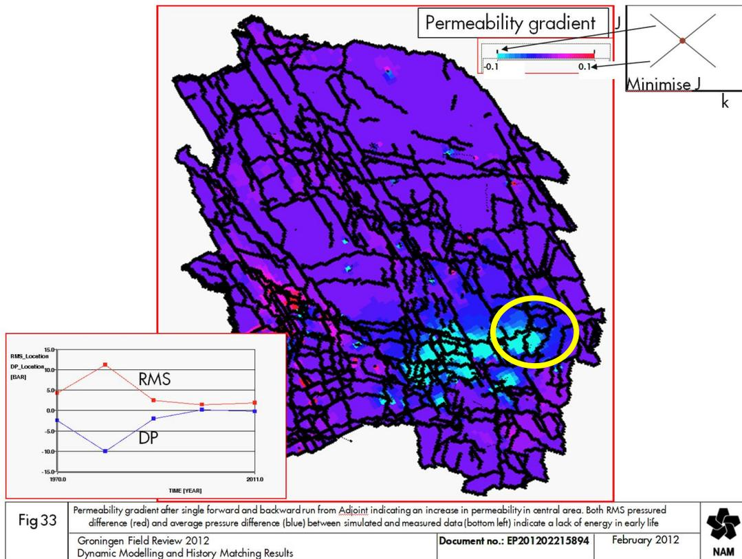
**Figure 37** Permeability gradient resulting from Adjoint run on GFR 2012 Groningen MoReS model (top). The Central area clearly stands out (high permeability multipliers in red), with the ZPD location marked by the yellow circle.
