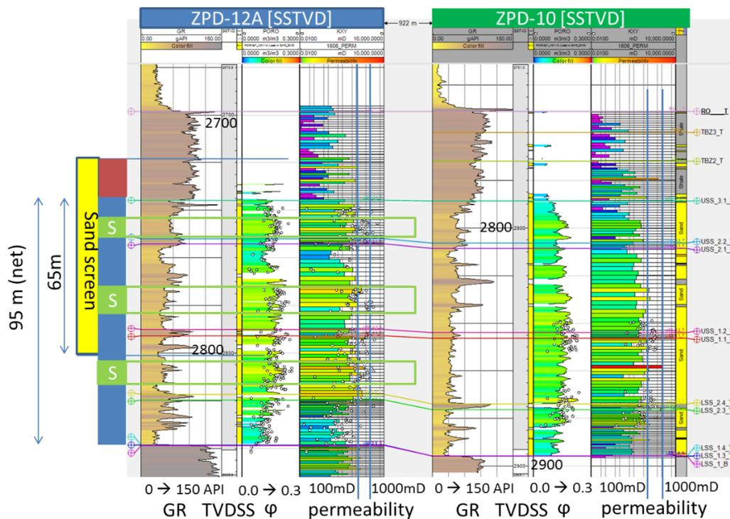
**Figure 39: Well log of ZPD-12A and ZPD-10 showing both permeabilities as in the static model (colored bars in the rightmost logs) and core measurements (white dots in the rightmost logs).**
