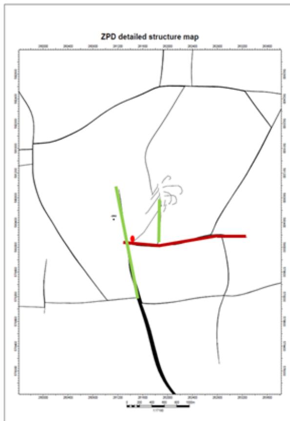
Figure 41: Fault representation around ZPD-12A in a high permeability streak model. The green line indicates a fully open fault (leak factor of 1.0), the red lines indicate a leak factor of 0.01 and the red dot marks the ZPD-12A well.
