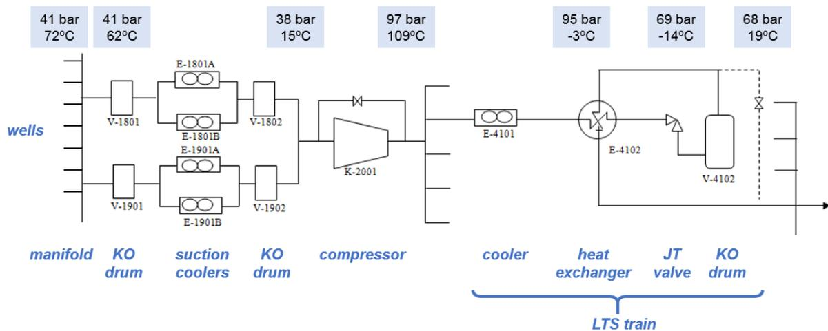
Figure 3-5 Simplified process diagram for a Groningen production cluster
