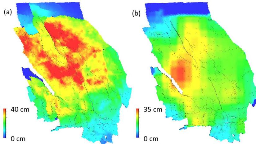
Figure 4-2 Preliminary comparison of estimated compaction at 31st Dec 2016 when using compressibility data from core data (a) versus subsidence inversion (b). The compressibility values used are assuming a linear model in pressure.
