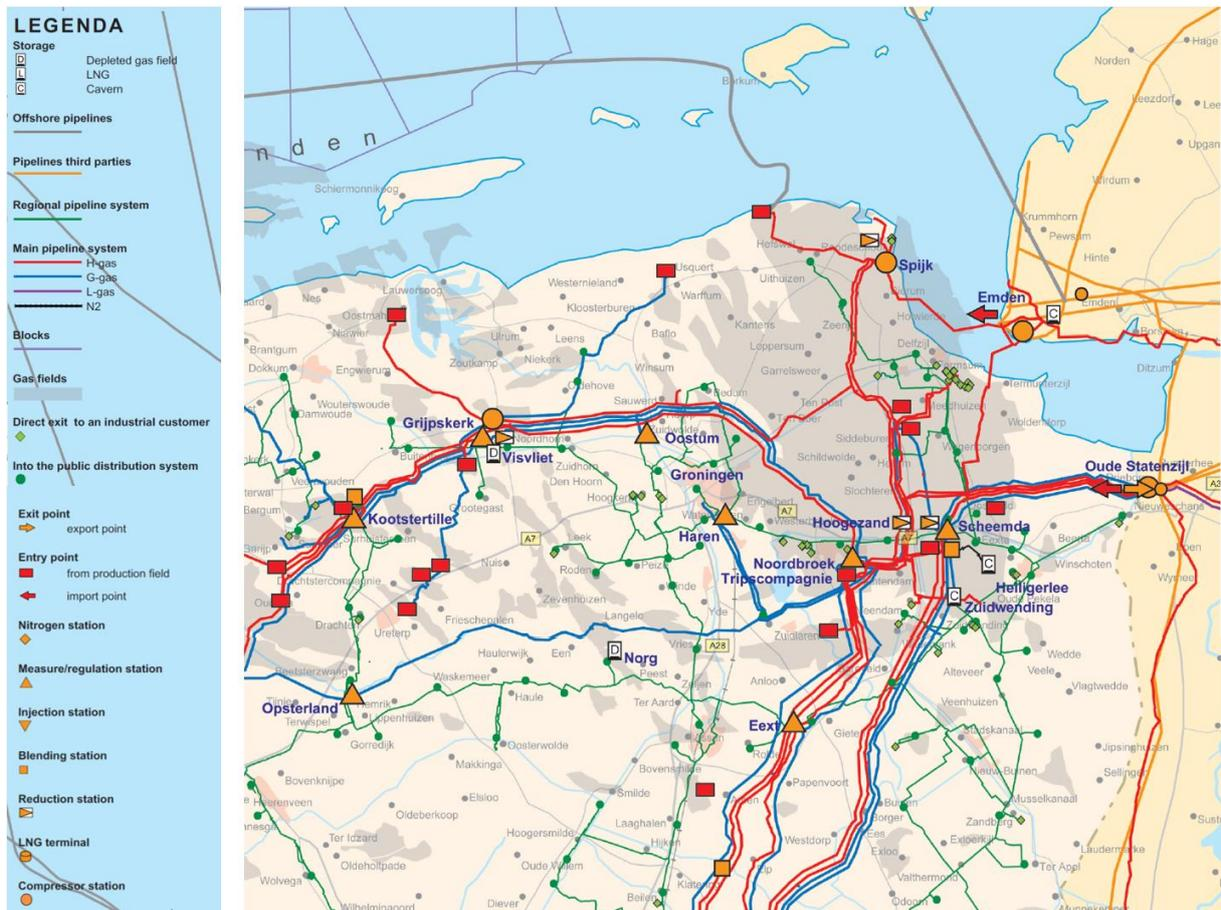
Figure 3-3 A closer look at the Gasunie Transport Solutions pipeline grid around Groningen (source: GTS).
