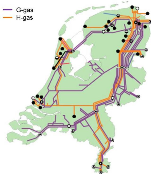
Figure 3-2 Gasunie Transport Solutions pipeline grid in the Netherlands. All L-gas pipelines originate from the Groningen field.
