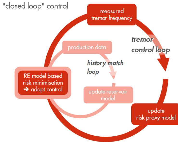
Figure 5-1 Schematic representation of the model based optimization loop
