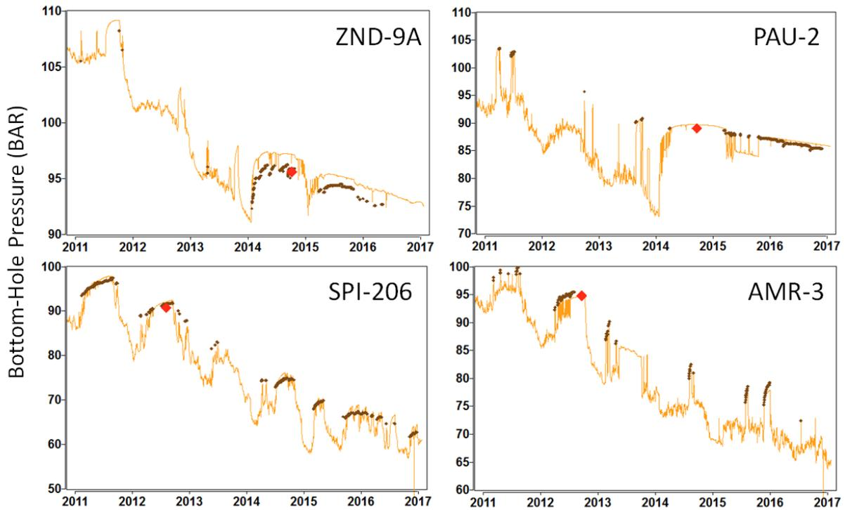
Figure 4-1 Preliminary comparison of modelled bottom-hole pressure (lines) to SPTG data (red points) and CITHP-CIBHP data (brown points) for selected wells.
