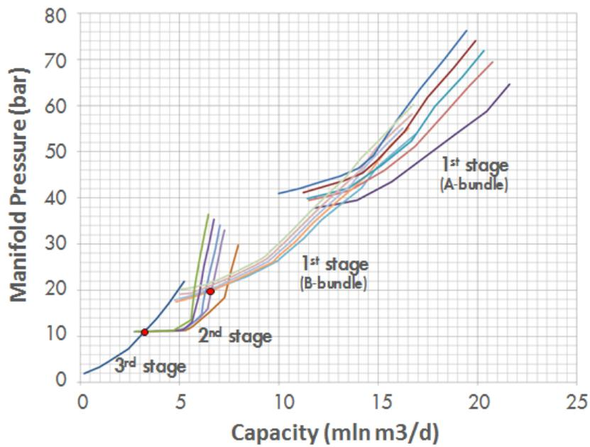
Figure 5-8 Typical compressor performance curves for various compressor stages and ambient temperatures.
