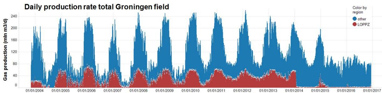
Figure 4-7 Daily production rates for the Groningen field, highlighting the production from the LOPPZ clusters.
