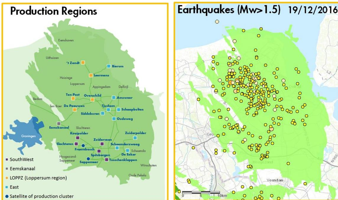
Figure 2-6 Production regions and earthquakes to date (Mw>1.5)
