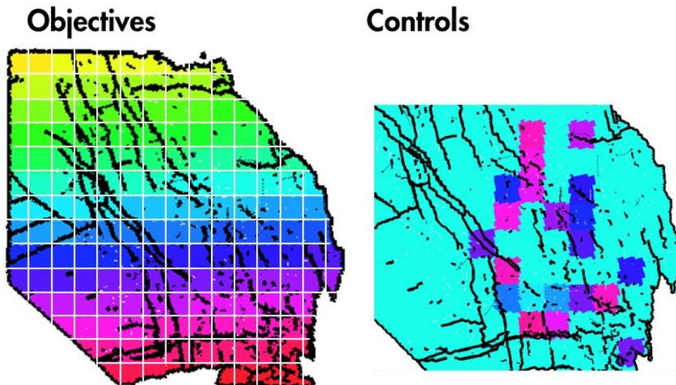
Figure 5-3 Dividing the field in 192 regions, of which 21 are controllable.
