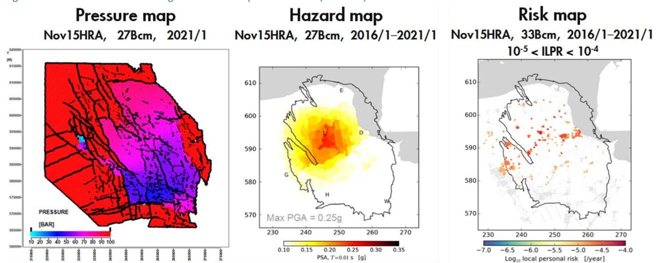
Figure 2-7 Combined visualization showing 1) the expected reservoir pressure distribution across the field in 2021 as per the Nov2015HRA forecast at 27Bcm/y ; 2) the associated Hazard map ; 3) the Risk map at 33Bcm annual offtake
