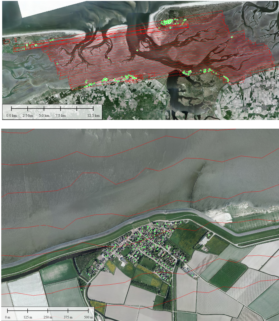
Figure 10: Control points distribution over the project area
