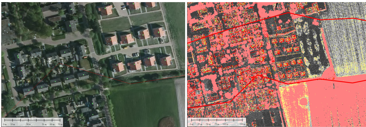
Figure 11: Left control points on the roof ridges and right the vertical separation analysis
