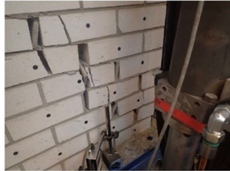
Figure 47: TUD-COMP-4: DIANA post-test refined prediction - Damage plot at end of analysis (top) compared to observed damage in laboratory
