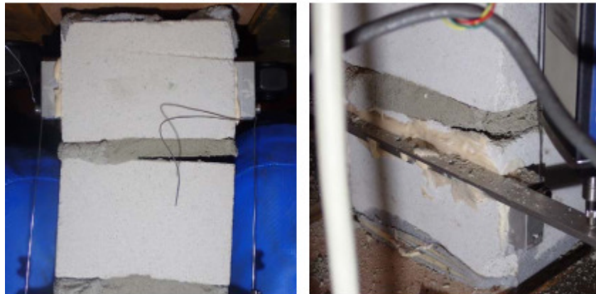
Figure 98: TUD-COMP-7: Final deflected shape of the (top) and cracks at top and bottom supports (bottom).
