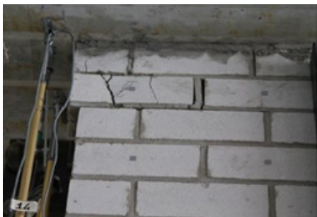
Figure 76: EUC-COMP-1: LS-DYNA blind prediction – Damage plot at end of analysis (top) compared to observed damage in laboratory
