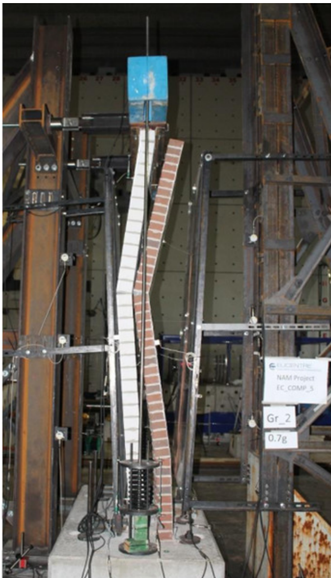
Figure 143: EUC-COMP-5: Collapse of specimen
