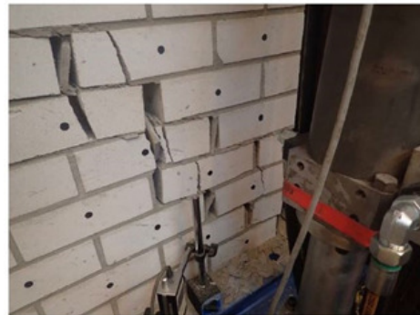
Figure 43: TUD-COMP-4: LS-DYNA post-test refined prediction - Damage plot at end of analysis (top right) compared to observed damage in laboratory
