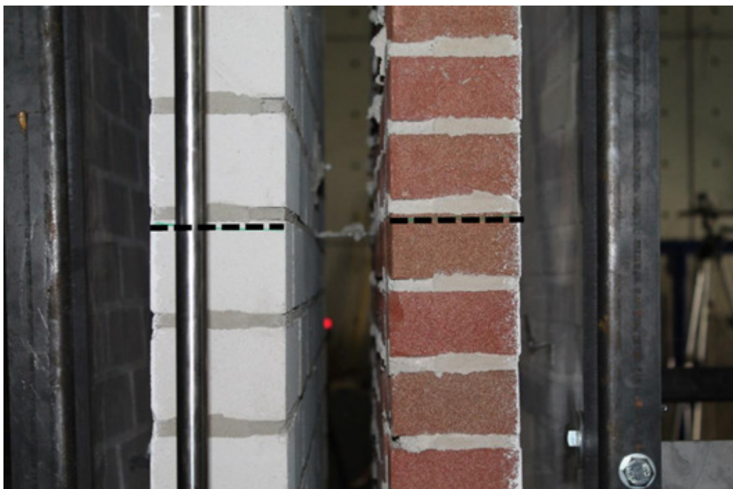
Figure 137: EUC-COMP-5: Formation of mid-height cracks at the tie location
