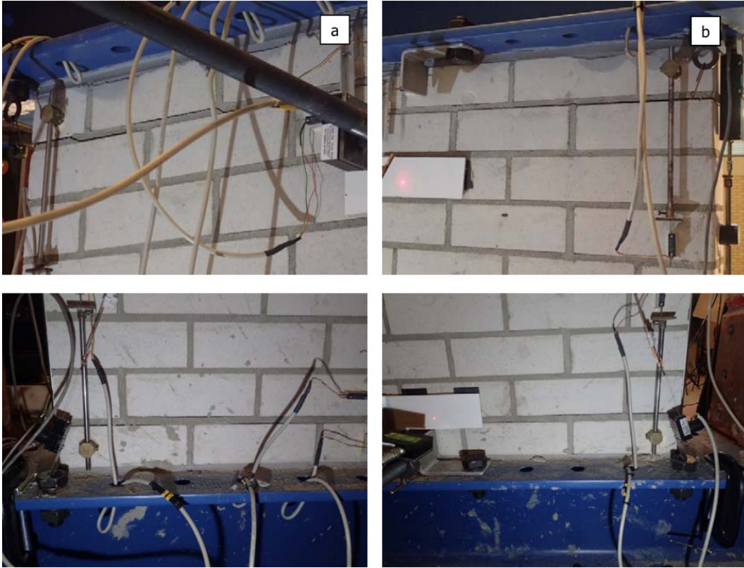
Figure 30: TUD-COMP-3: Rocking cracks at the top & bottom left corners (a) and top & bottom right corners (b)
