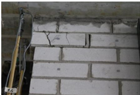
Figure 78: EUC-COMP-1: DIANA post-test refined prediction - Damage plot at end of analysis (top) compared to observed damage in laboratory
