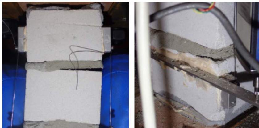
Figure 101: TUD-COMP-7: Final deflected shape of the (top) and cracks at top and bottom supports (bottom).
