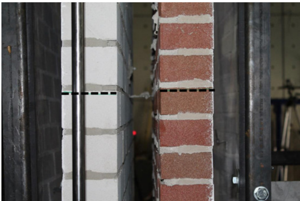
Figure 141: EUC-COMP-5: Formation of mid-height cracks at the tie location
