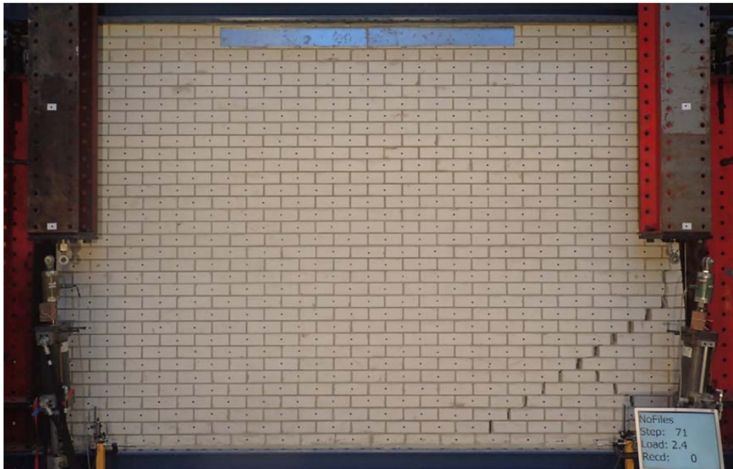
Figure 53: TUD-COMP-5: Crack pattern at the end of the test
