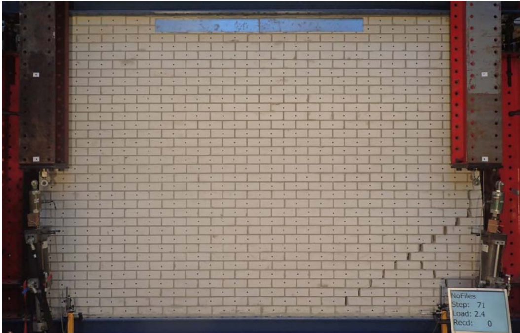
Figure 49: TUD-COMP-5: Crack pattern at the end of the test
