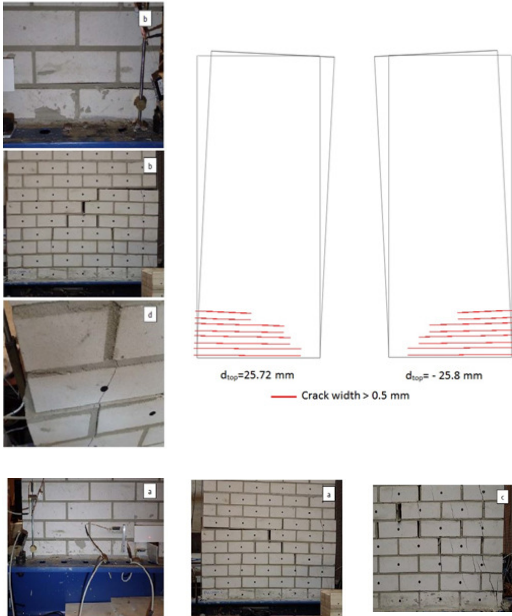
Figure 26: TUD-COMP-2: DIANA post-test refined prediction - Damage plot at end of analysis (top right) compared to observed damage in laboratory
