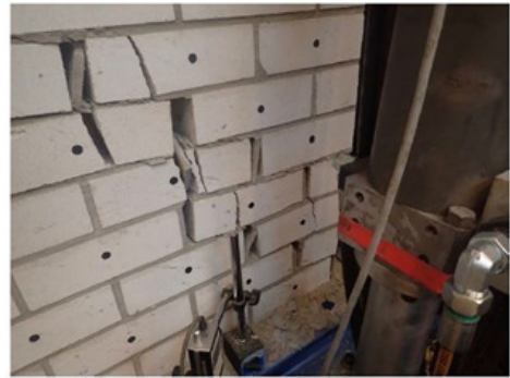
Figure 51: TUD-COMP-4: DIANA blind prediction - Damage plot at end of analysis (top right) compared to observed damage in laboratory
