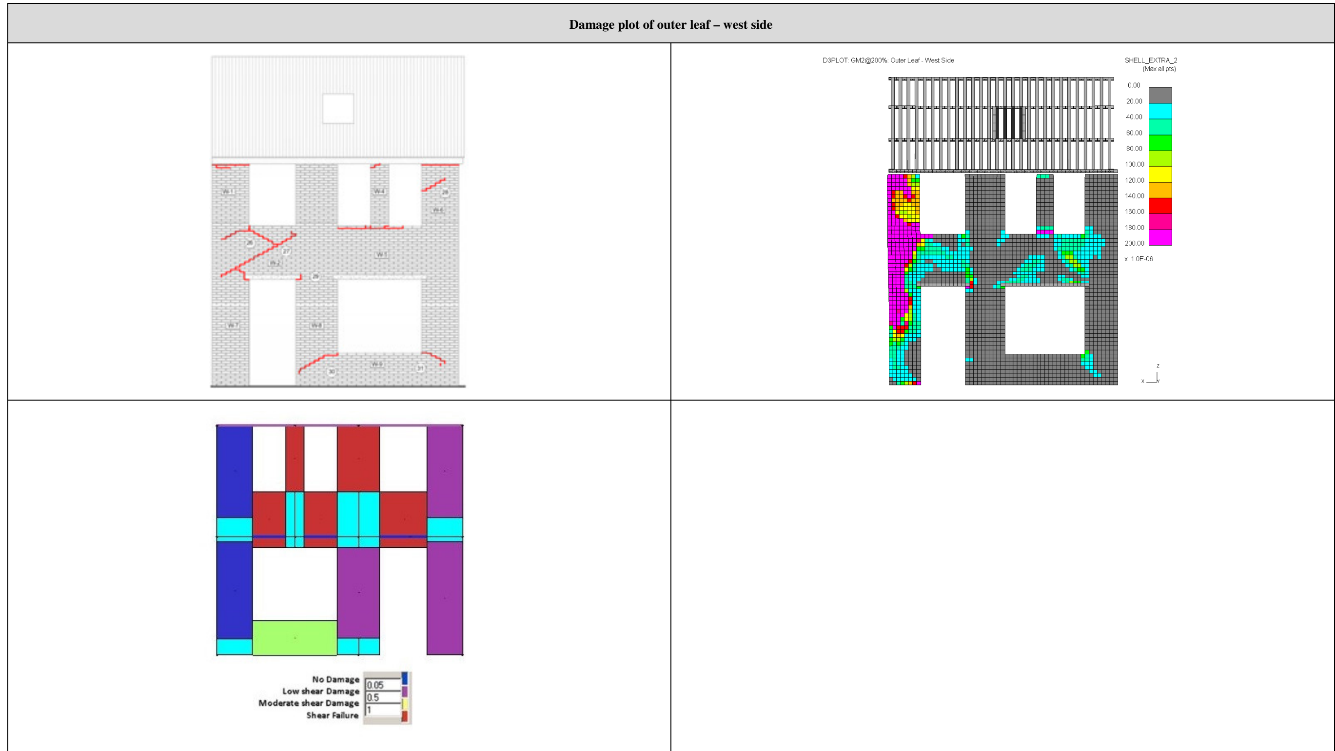
Figure 16: Damage plot of outer leaf - west side of test result (top left), Arup LS-DYNA (top right), and EUCENTRE (bottom left)
