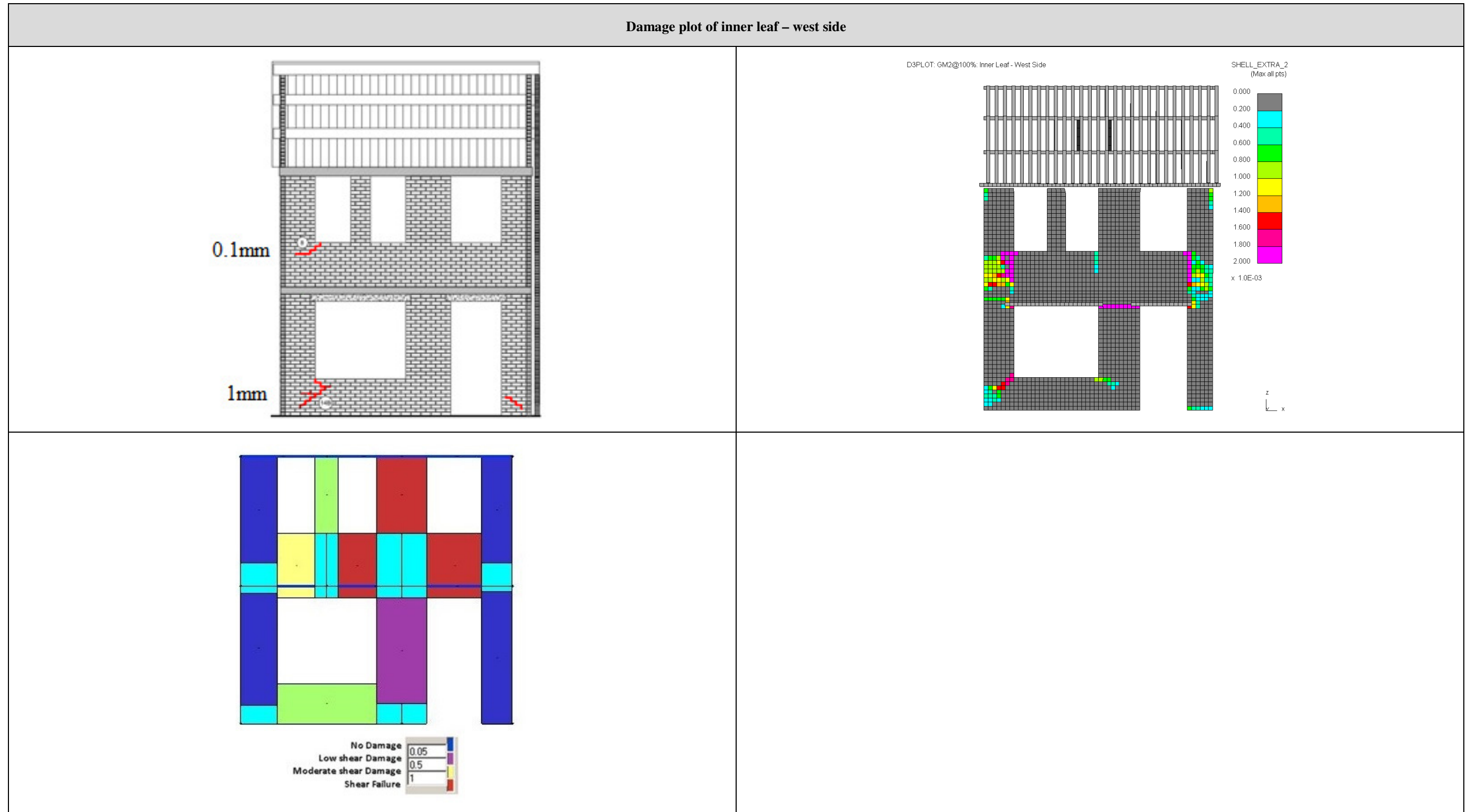
Figure 8: Damage plot of inner leaf - west side of test result (top left), Arup LS-DYNA (top right), and EUCENTRE (bottom left)
