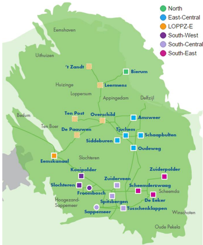
Production cluster by location, as used to display the areal distribution of production. Note that the Loppersum clusters (LOPPZ) are lumped with the Eemskanaal cluster for display purposes (LOPPZ-E). However, in none of the forecast scenarios there is any production from the LOPPZ clusters (only for the imposed production distribution there is production from Eemskanaal), hence the LOPPZ clusters are shaded here.
