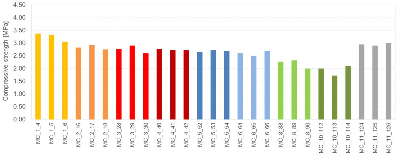
Figure 8.52 Compressive strength and modulus of elasticity test results for the mortars collected directly from the building prototype after 20 days of age.
