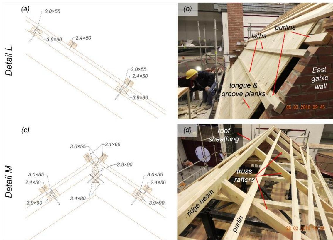
Figure 2.22 Construction details of the roof: (a, b) connections among purlins, planks, and laths; (c, d) realisation of the nail connections at the ridge.
