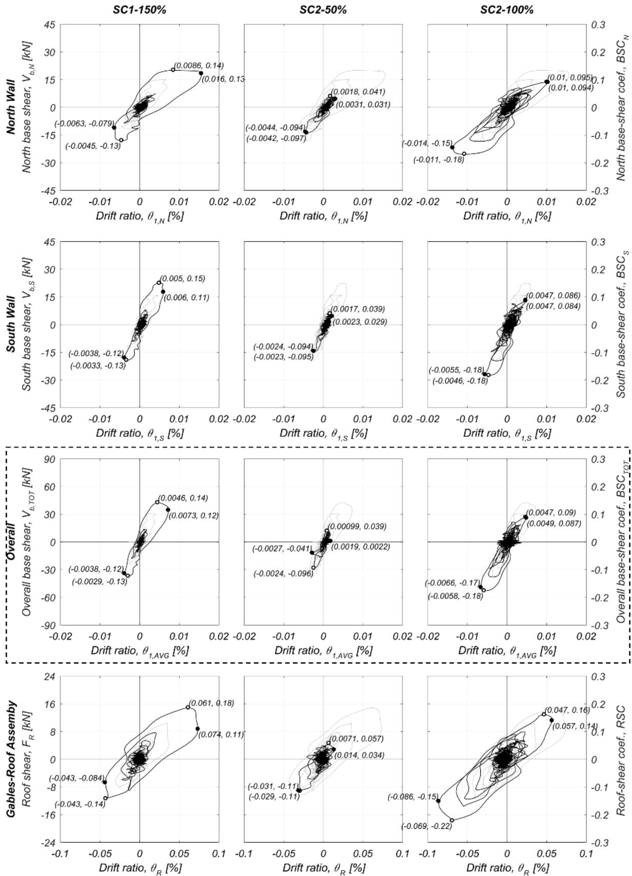
Figure 6.39 Specimen hysteretic responses: test runs SC1-150%, SC2-50% and SC2-100%.
