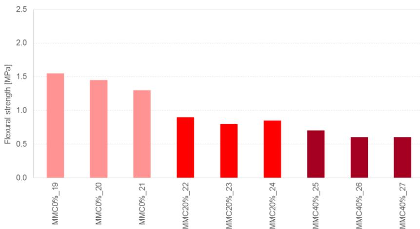
Figure 8.20 Flexural strength test results mortar for maturation curve (MMC\_0%, MMC\_20% and MMC\_40%) after 28 days of age.
