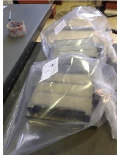
Figure 8.9 Curing conditions of study mortar specimens.
