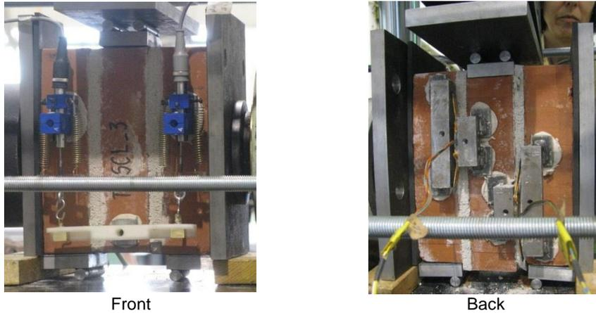
Figure 8.120 Instrumentation placed on the triplets.
