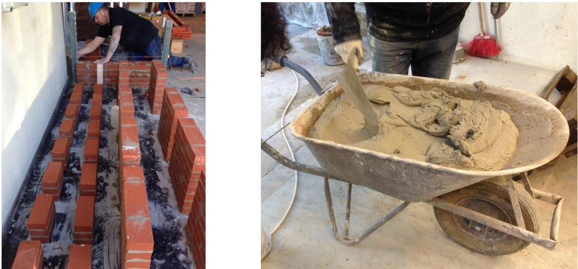
Figure 8.28 Construction of characterisation specimens at the time of mortar sampling.
