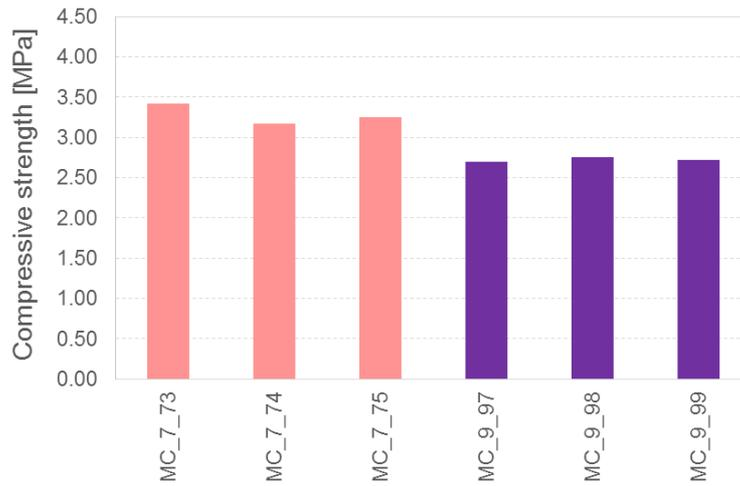
Figure 8.55 Compressive strength and modulus of elasticity test results for the mortars collected directly from the characterisation specimens after 10 days of age.
