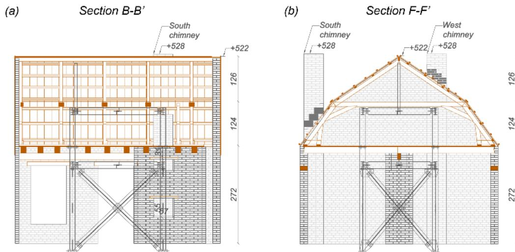
Figure 2.4 Sections in elevation of the building specimen: (a) section B-B'; (b) section F-F'. Units of cm.
