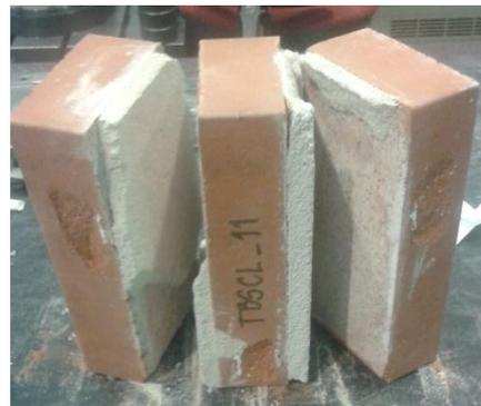
Figure 8.131 Example of one of the failure mechanisms obtained for each triplet in the shear strength test.
