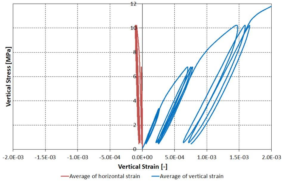
Figure 8.83 Vertical stress vs. vertical and horizontal strains for single wallette CTBSCL\_1S.
