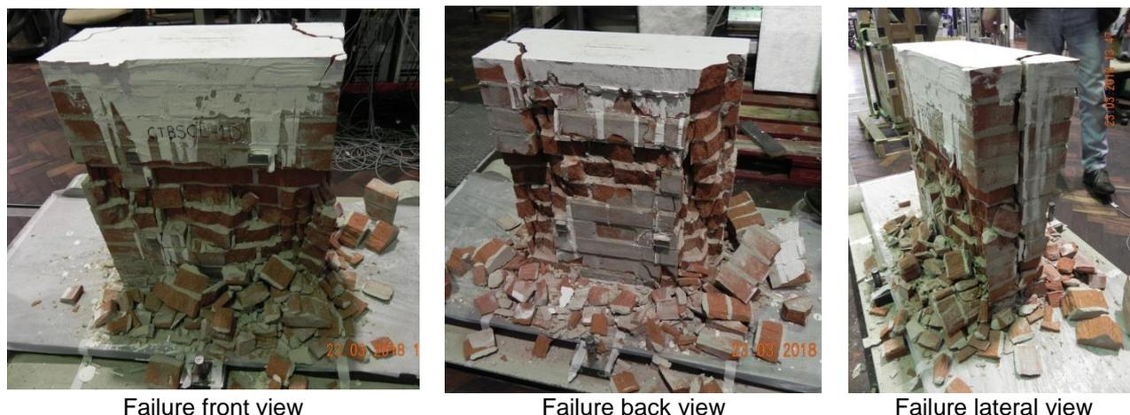
Figure 8.82 Double wallette during the test and after failure.
