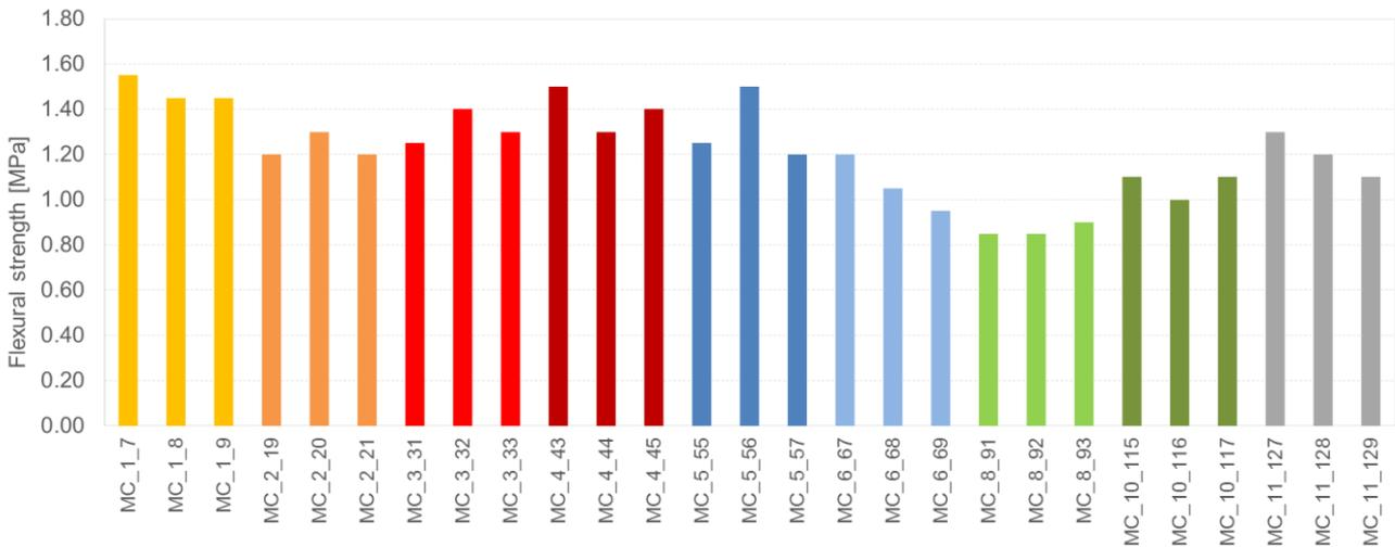
Figure 8.45 Flexural strength test results for the mortars collected directly from the building prototype after 28 days of age.
