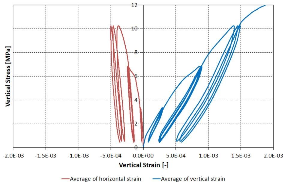
Figure 8.86 Vertical stress vs. vertical and horizontal strains for single wallette CTBSCL\_4S.
