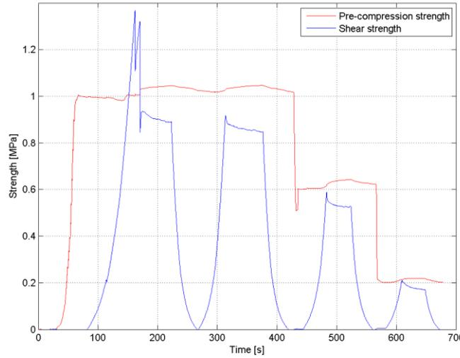
Figure 8.126 Application of pre-compression and shear stresses throughout the test started at the highest pre-compression level (TBSCCL\_8).
