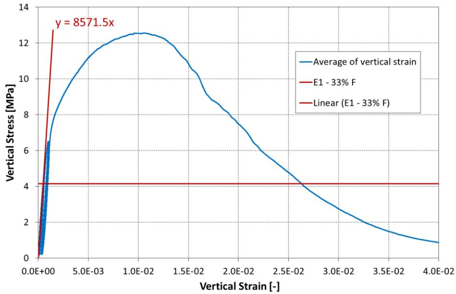
Figure 8.103 Vertical stress vs. vertical strain and determination of the modulus of elasticity for double wallette CTBSCL\_2D.
