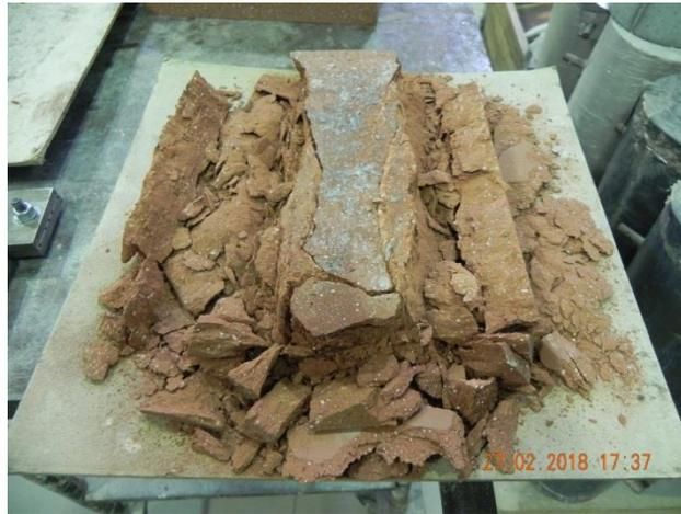
Figure 8.66 Brick for the compressive strength test after failure.
