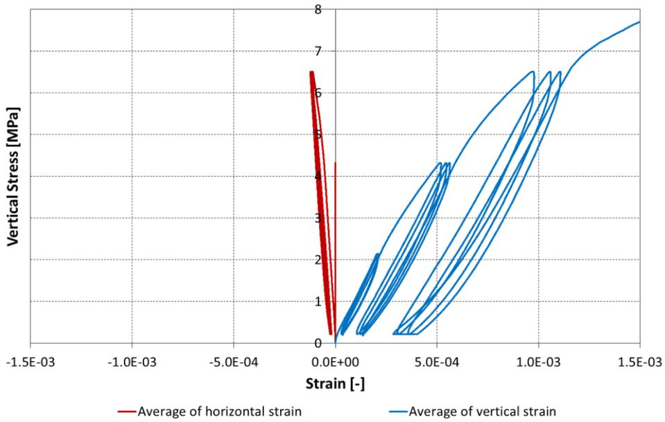
Figure 8.97 Vertical stress vs. vertical and horizontal strains for double wallette CTBSCL\_2D.
