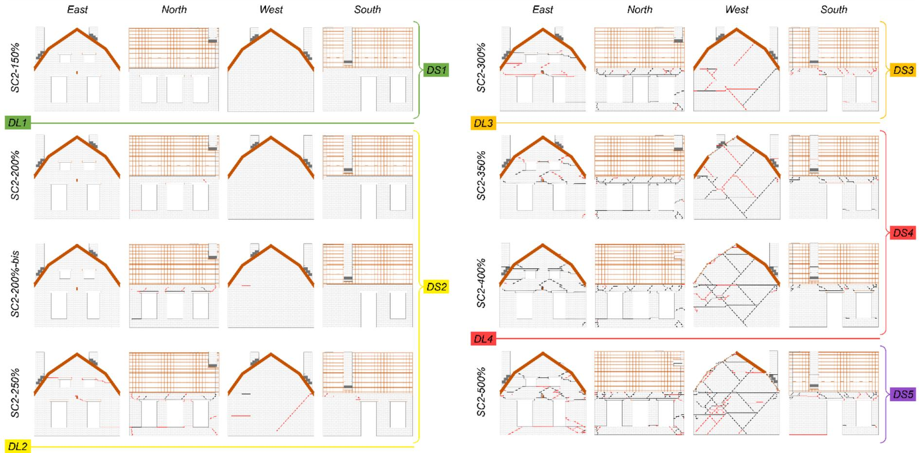
Figure 7.2 Evolution of specimen crack pattern and identification of global damage states and damage limits.
