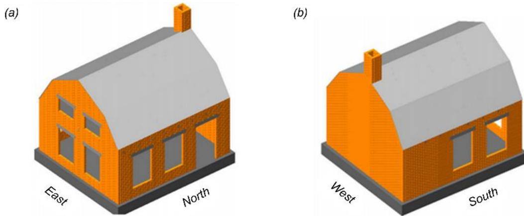
Figure 1.2 Numerical model of a building resembling the LNEC-BUILD-3 prototype developed on Extreme Loading for Structures software: (a) East-North view; (b) West-South view (Pinho et al., 2017).
