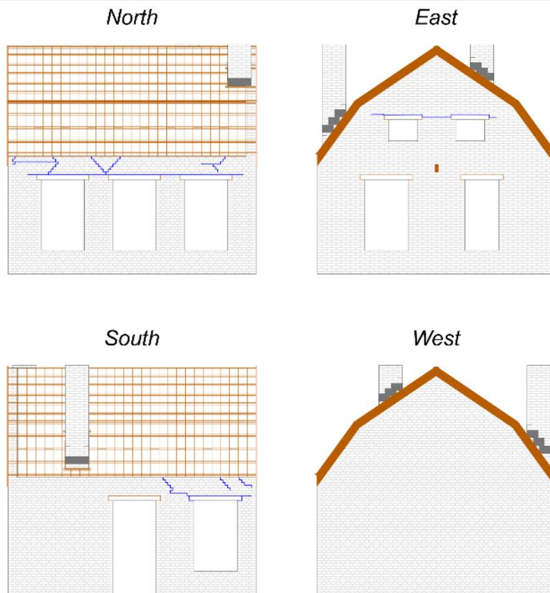
Figure 2.29 Observed crack pattern on the perimeter walls of the prototype building after the end of the construction (exterior view).
