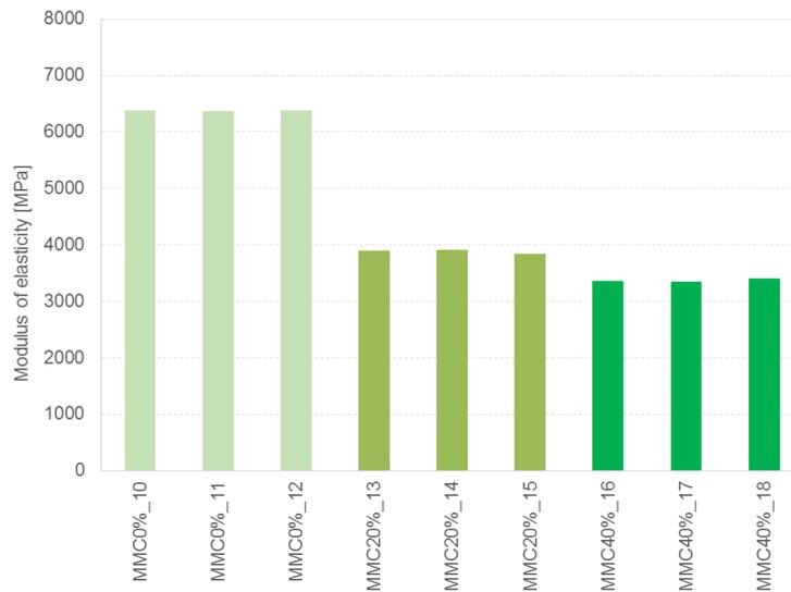
Figure 8.12 Test results for the determination of the dynamic modulus of elasticity of mortar for maturation curve (MMC\_0%, MMC\_20% and MMC\_40%) after 20 days of age.
