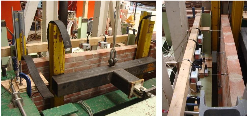
Figure 8.133 Test setup for four-point out-of-plane bending tests.
