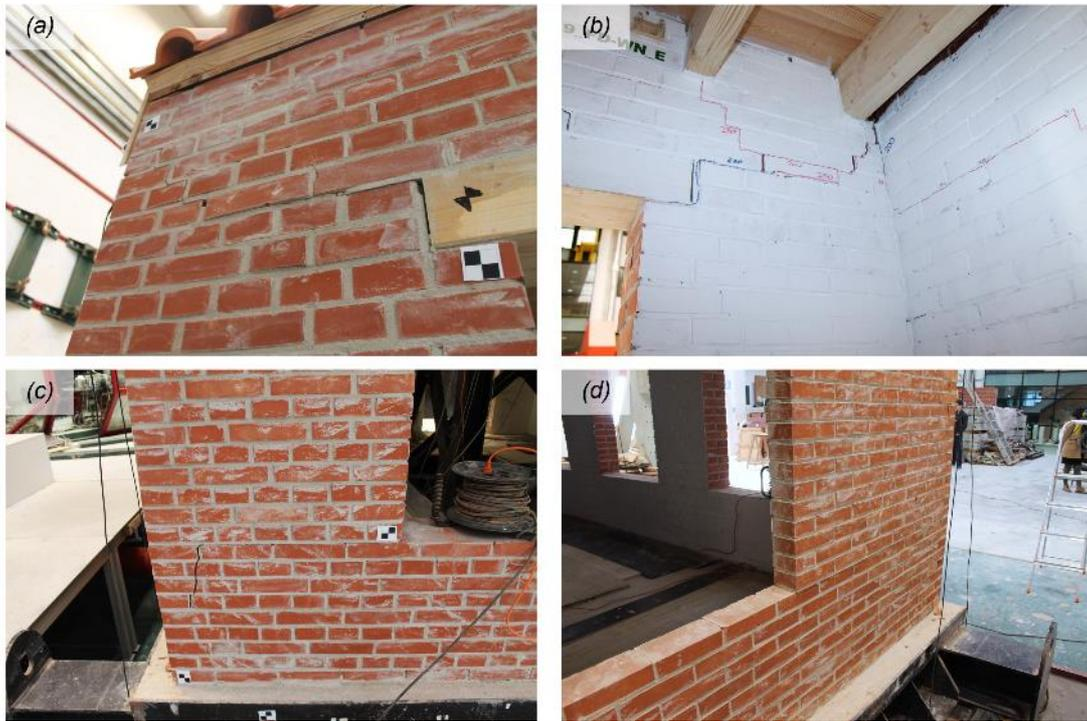
Figure 6.24 Damage on the intersecting piers of North and East façades at the end of test SC2-300%.
