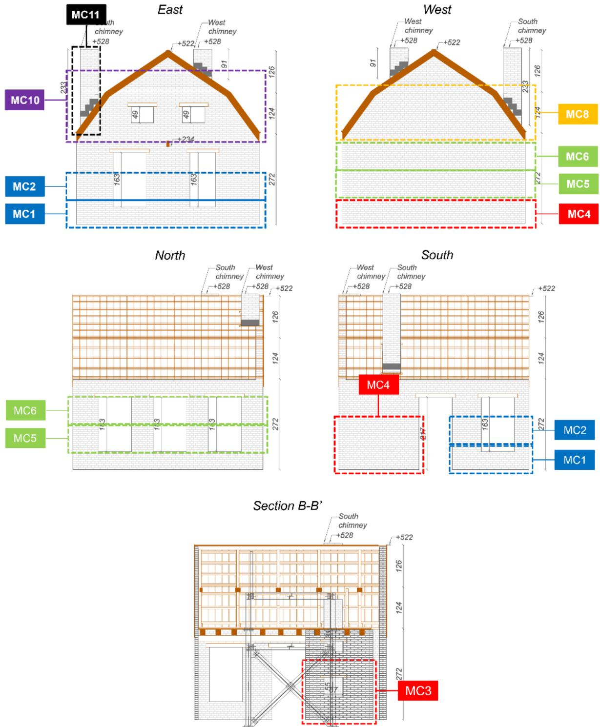
Figure 8.29 Mortar sampling from the construction of the building prototype
