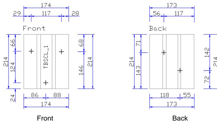
Figure 8.121 Location of the instrumentation placed on the triplets (dimensions in mm).
