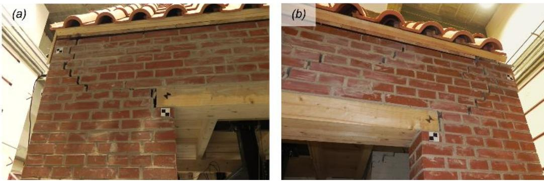
Figure 6.31 Damage on the North façade after test SC2-400%: wide permanent openings at the top of the corner piers.
