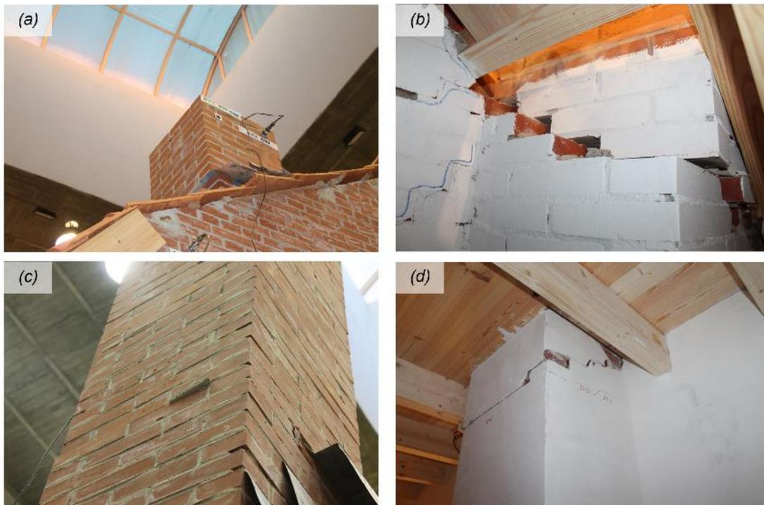
Figure 6.26 Damage to the chimneys during test SC2-350%: (a) failure in the West chimney at the location of flashing; (b) permanent sliding of the West at the level of the roofline; (c) fracture at mid-height of the South chimney stack; (d) residual displacement at the base of the South chimney stack.
