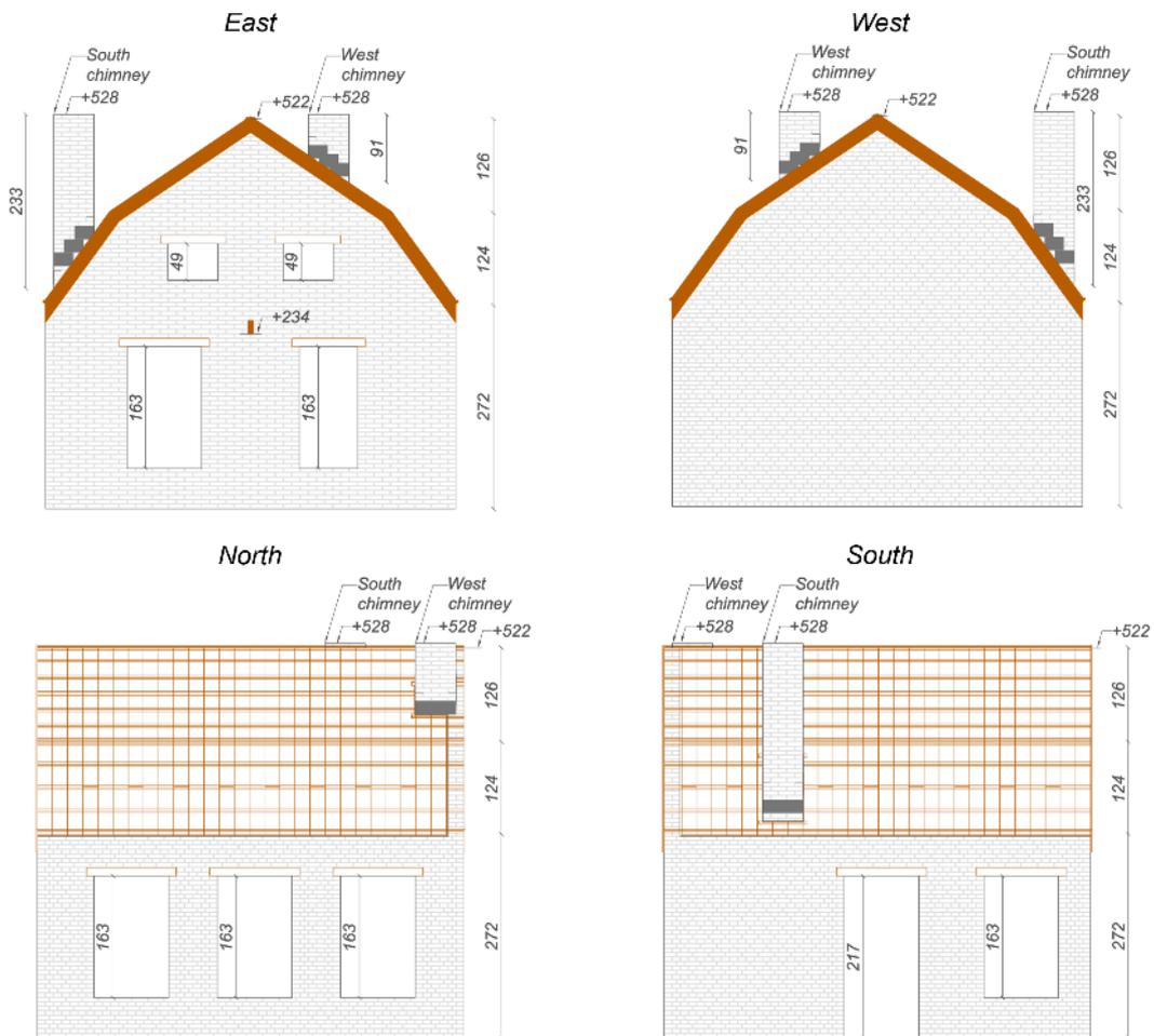
Figure 2.3 Elevation views of the building specimen. Units of cm.
