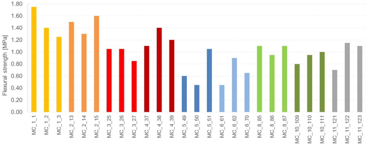
Figure 8.43 Flexural strength test results for the mortars collected directly from the building prototype after 10 days of age.
