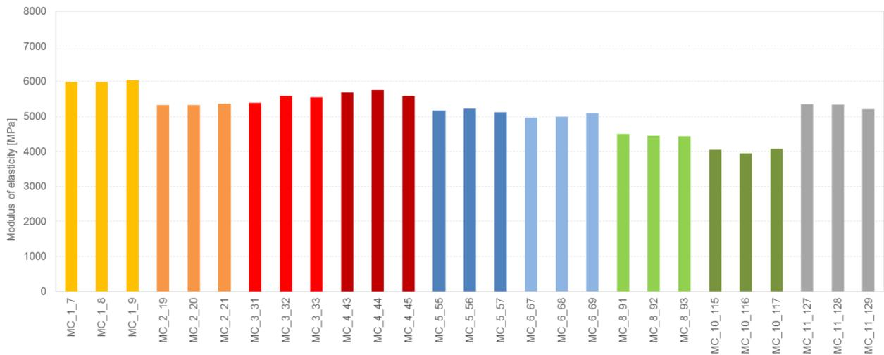
Figure 8.35 Test results for the determination of the dynamic modulus of elasticity for the mortars collected directly from the building prototype after 28 days of age.
