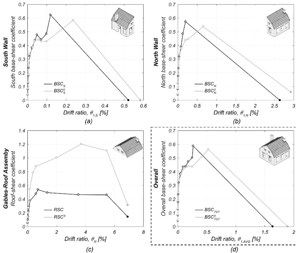
Figure 6.44 Specimen backbone curves: (a) South subsystem; (b) North subsystem; (c) gables-roof subsystem; (d) Overall structure.
