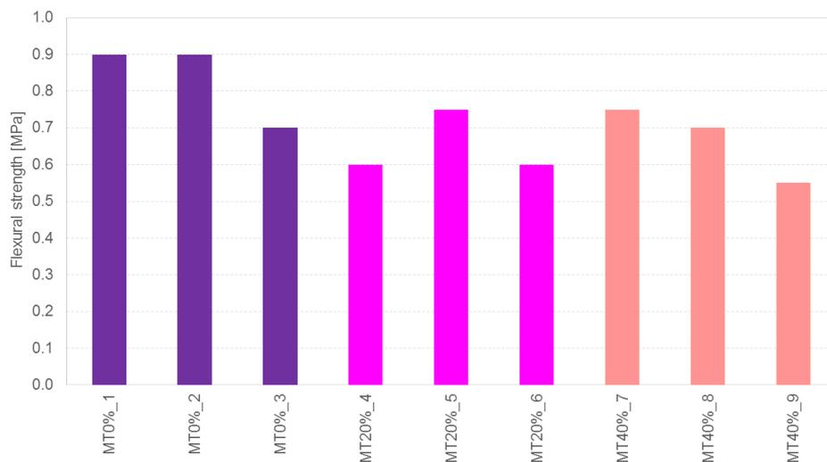
Figure 8.17 Flexural strength test results for mortar test (MT\_0%, MT\_20% and MT\_40%) after 6 days of age.
