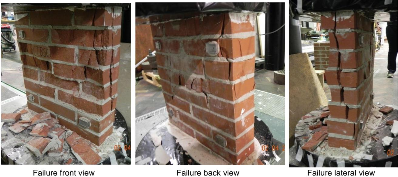
Figure 8.81 Single *wallette* during the test and after failure.
