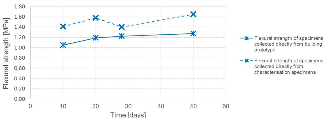
Figure 8.61 Relation between flexural strength and maturation time for the bedding mortars removed from the building prototype and the characterisation test specimens.
