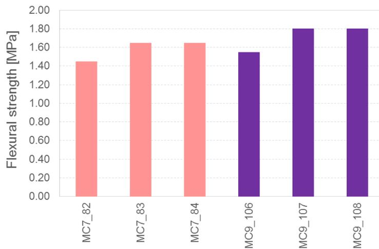
Figure 8.50 Flexural strength test results for the mortars collected directly from the characterisation specimens during the seismic test.
