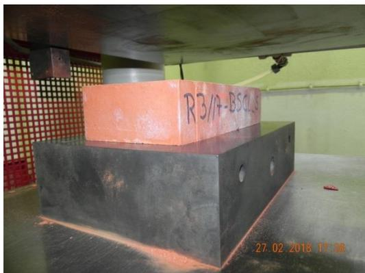
Bricks on the test machine plate
