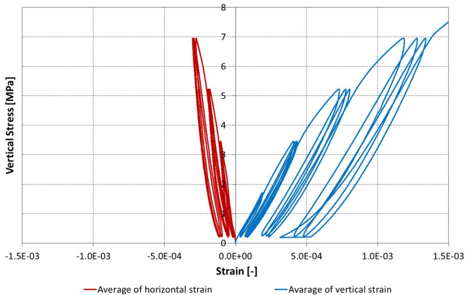
Figure 8.96 Vertical stress vs. vertical and horizontal strains for double wallette CTBSCL\_1D.
