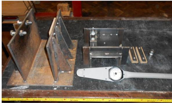
Figure 8.111 Test device used for bond-wrench test.
