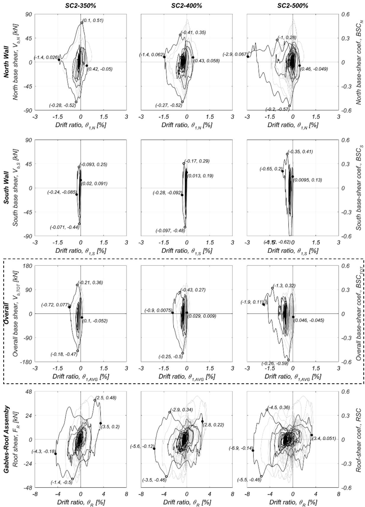
Figure 6.42 Specimen hysteretic responses: test runs SC2-350%, SC2-400% and SC2-500%.
