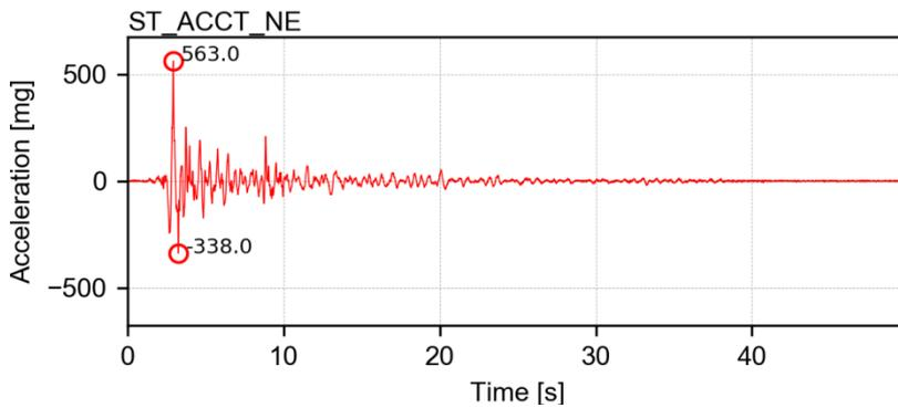
Channel ST\_ACCT\_NE – Transverse acceleration of the North-East LNEC 3D shake table platform
