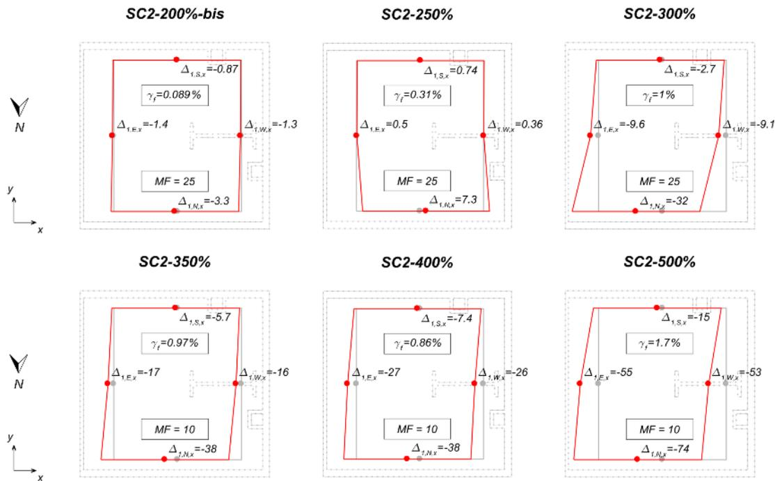
Figure 6.35 Deformed shapes of the floor at the instants of maximum diaphragm shear deformations: test runs SC2-200%-bis to SC2-500%. MF is the displacement magnification factor on the figure. Units of mm unless otherwise specified.
