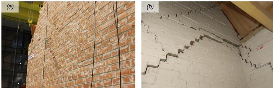
Figure 6.29 Damage on the West façade after test SC2-400%: mortar-joint sliding due to rigid-body out-of-plane mechanism.
