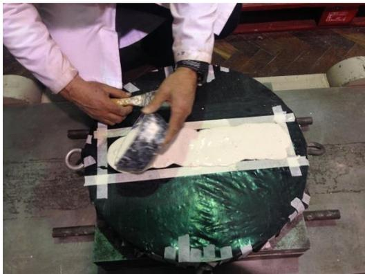
Layer of gypsum levelled by the plates of the press machine
