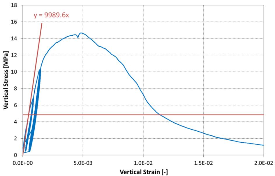
Figure 8.92 Vertical stress vs. vertical strain and determination of the modulus of elasticity for single wallette CTBSCL\_4S.
