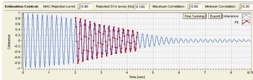
Figure 6.4 Frequency estimate (zero-crossings) and damping (logarithm decrement) of the impulse response estimate.
