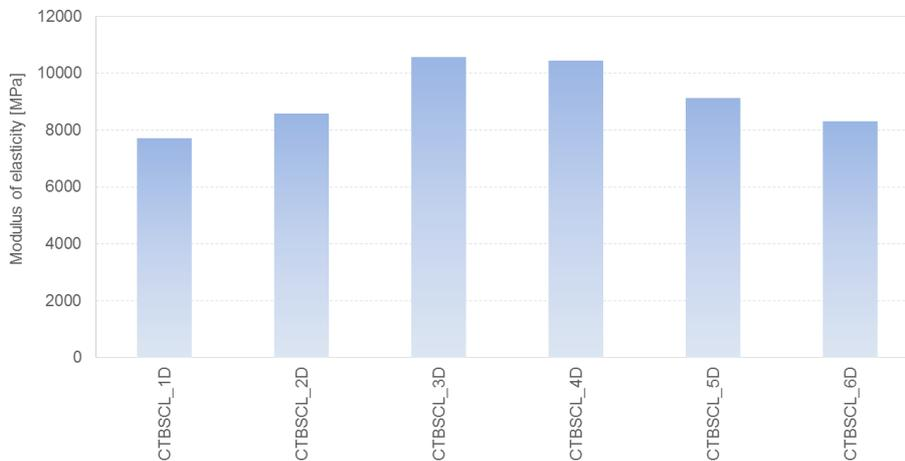
Figure 8.108 Distribution of moduli of elasticity obtained for double wallettes.
