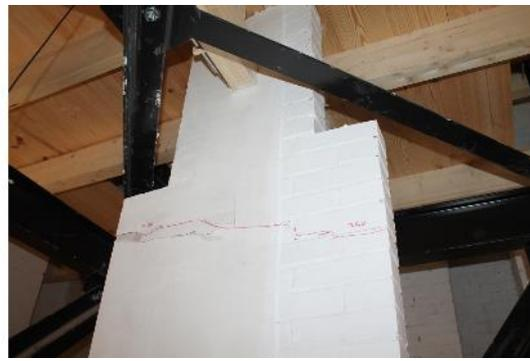
Figure 6.21 Damage on the interior wall after test SC2-250%.
