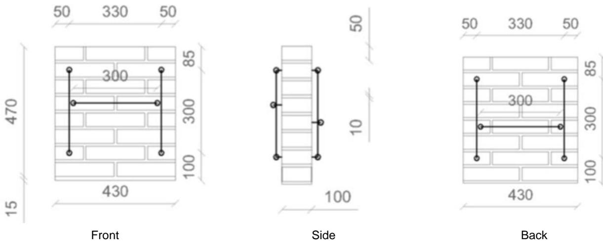
Figure 8.75 Scheme and numbering of the transducers placed on each face of the single wallettes.
