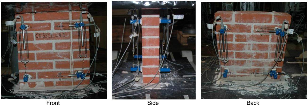
Figure 8.77 Instrumentation placed on each face of the single wallettes.
