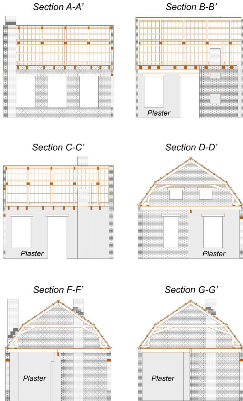
Figure 2.26 Sections in elevation of the building specimen: wall rendering with plaster.
