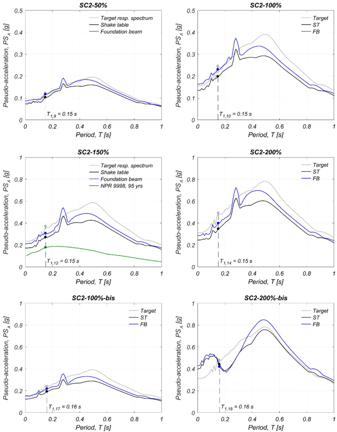
Figure 6.10 Comparison between elastic 5%-damped pseudo-acceleration response spectra of the actual input signals and target spectra for SC2 motion scaled up to 200%-bis. Comparison against the NPR 9998 (2017) elastic spectrum for events with return period of 95 years for the area of Loppersum, Groningen (lat. 53.330115, long. 6.747205).
