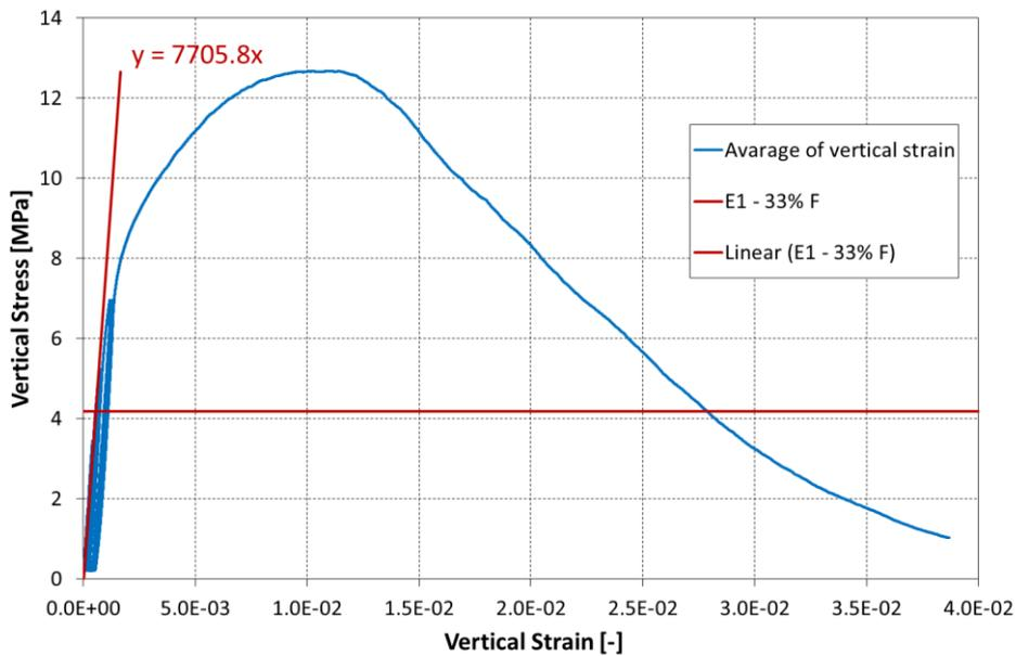
Figure 8.102 Vertical stress vs. vertical strain and determination of the modulus of elasticity for double wallette CTBSCL\_1D.
