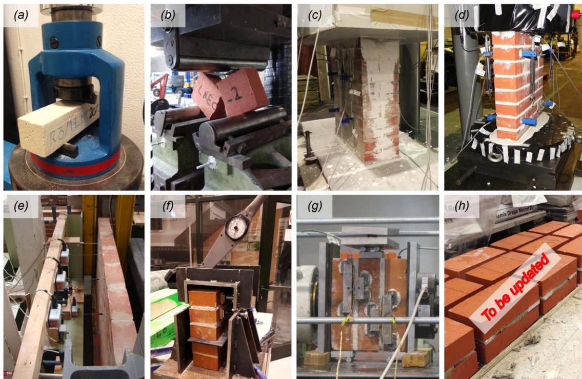
Figure 8.1 Mechanical characterization tests: (a) three-point bending test on a mortar specimen; (b) three-point bending test on a solid-clay brick; (c) compression test on a double-wythe masonry wallette; (d) compression test on a single-wythe masonry wallette; (e) four-point out-of-plane bending test; (f) bond wrench test; (g) direct shear test on a triplet; (h) shear test in torsion on a doublet.
