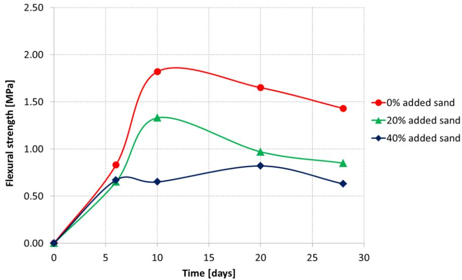
Figure 8.25 Maturation curve over time for the flexural strengths of MMC and MT mortars.
