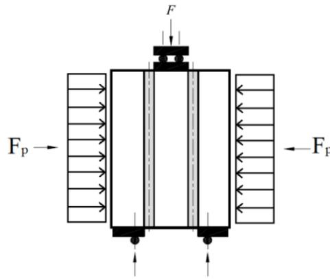
Figure 8.122 Test scheme for the determination of shear strength.
