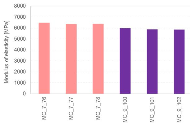
Figure 8.38 Test results for the determination of the dynamic modulus of elasticity for the mortars collected directly from the characterisation specimens after 20 days of age.
