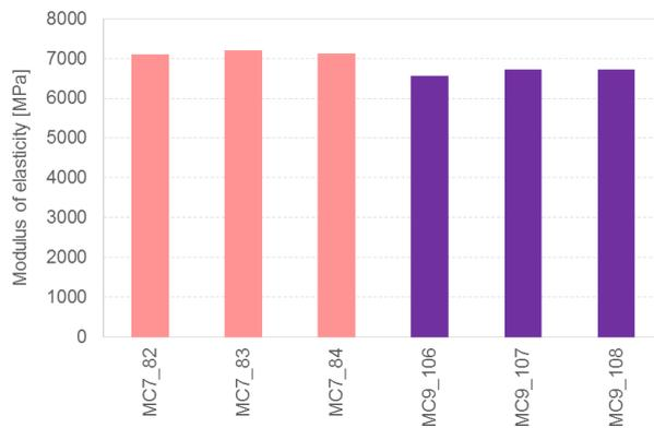
Figure 8.40 Test results for the determination of the dynamic modulus of elasticity for the mortars collected directly from the characterisation specimens during the seismic test.
