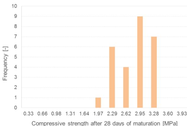
Specimens collected directly from building prototype
