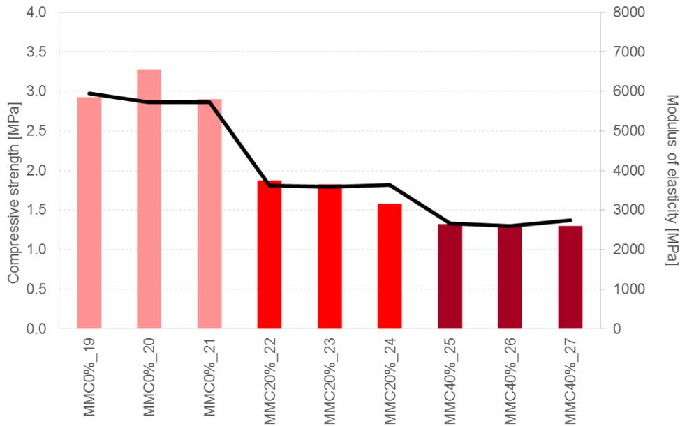
Figure 8.24 Compressive strength and modulus of elasticity test results for maturation curve (MMC\_0%, MMC\_20% and MMC\_40%) after 28 days of age.
