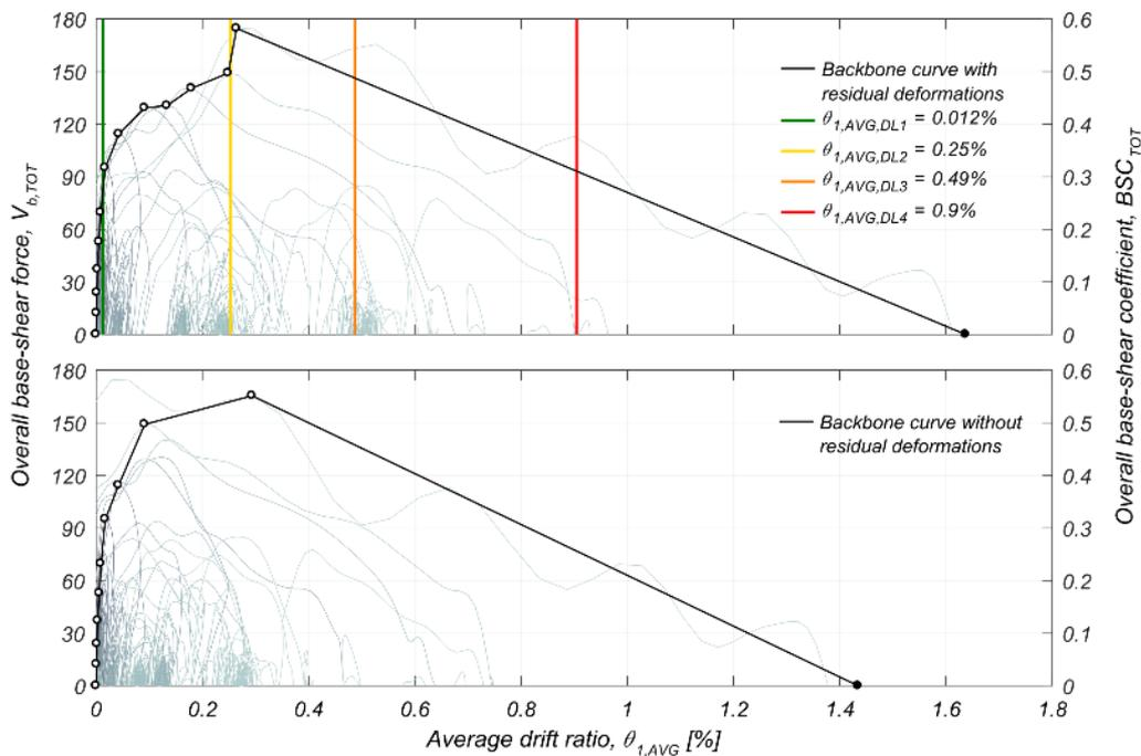
Figure 7.3 Backbone curves and damage limit states for the overall building response. Top: with the inclusion of residual deformations; bottom: without residuals from previous tests.
