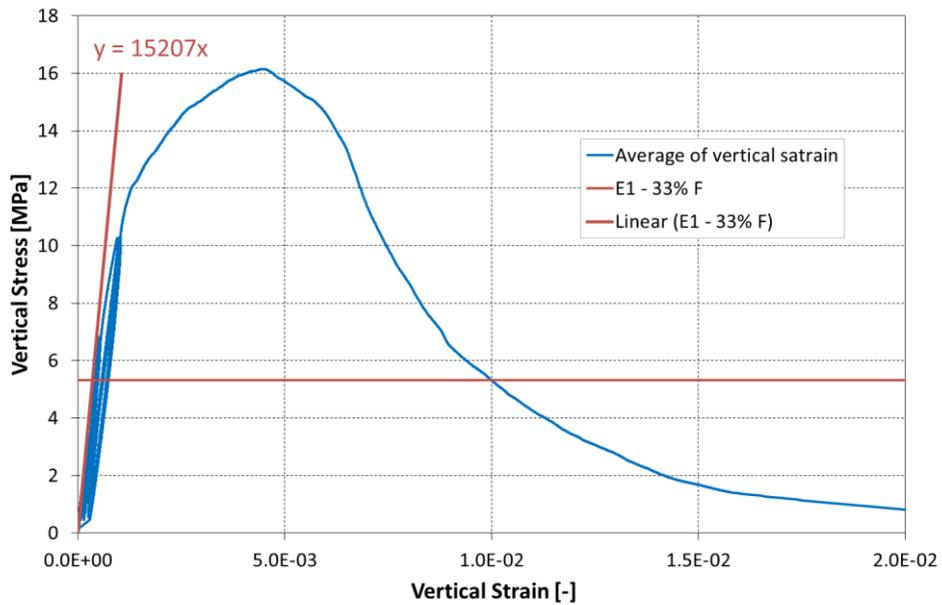
Figure 8.94 Vertical stress vs. vertical strain and determination of the modulus of elasticity for single wallette CTBSCL\_6S.
