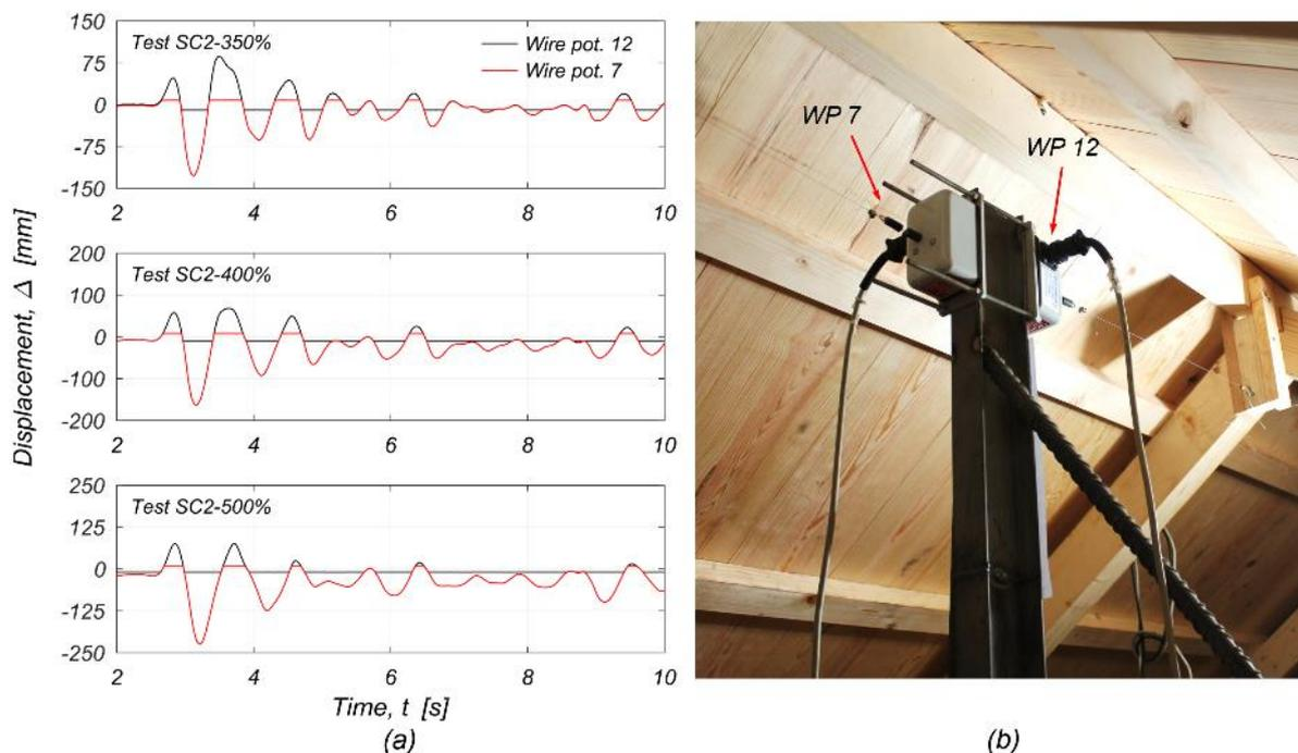
Figure 5.1 Measuring the displacement of the roof ridge during tests SC2-350%, SC2-400% and SC2-500%: (a) displacement recordings by WP 12 and WP 7 in the time window 2-10 s; (b) location of wire potentiometers WP 12 and WP 7.
