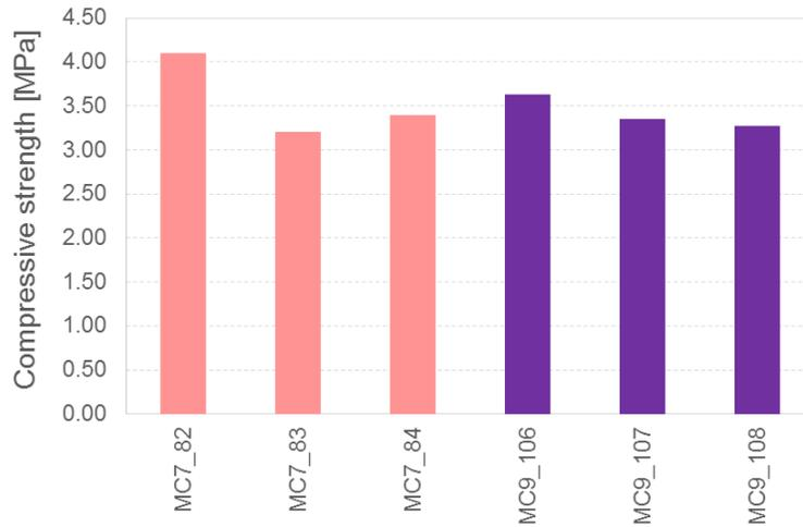
Figure 8.58 Compressive strength and modulus of elasticity test results for the mortars collected directly from the characterisation specimens during the seismic test.
