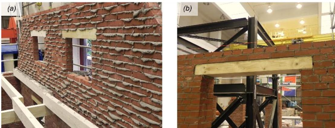
Figure 2.8 Construction details of the building specimen: (a) timber lintels above the openings of the East gable wall; (b) lintel placed above the window of the South façade.
