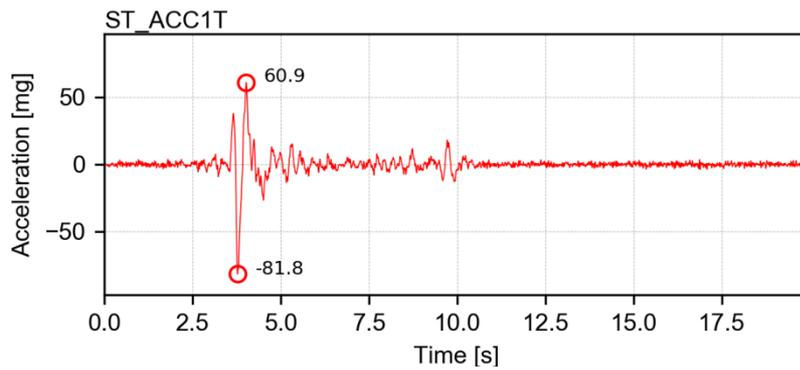
Channel ST\_ACC\_T – Transverse acceleration of the LNEC 3D shake table motion control
