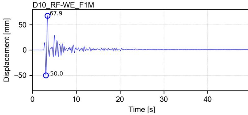
Channel D10\_RF-WE\_F1M – displacement
