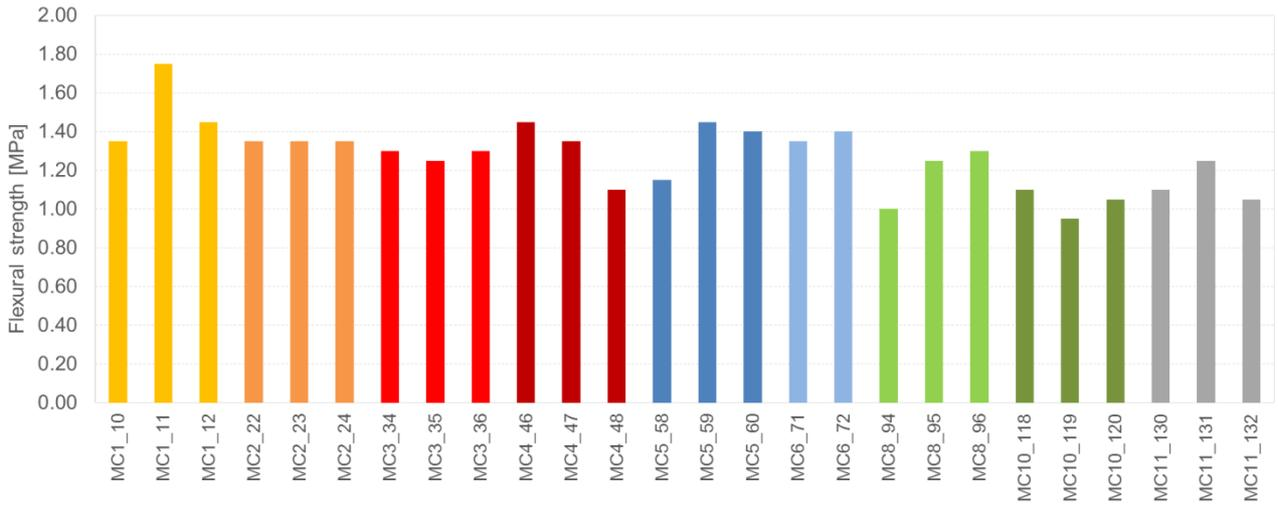
Figure 8.46 Flexural strength test results for the mortars collected directly from the building prototype during the seismic test.
