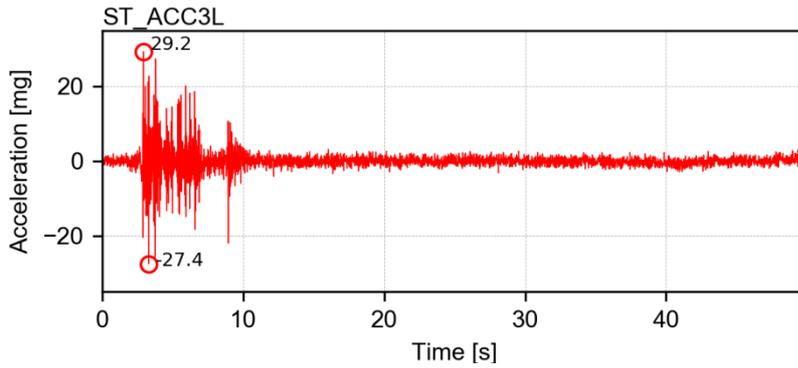
Channel ST\_ACC\_V – Longitudinal acceleration of the LNEC 3D shake table motion control
