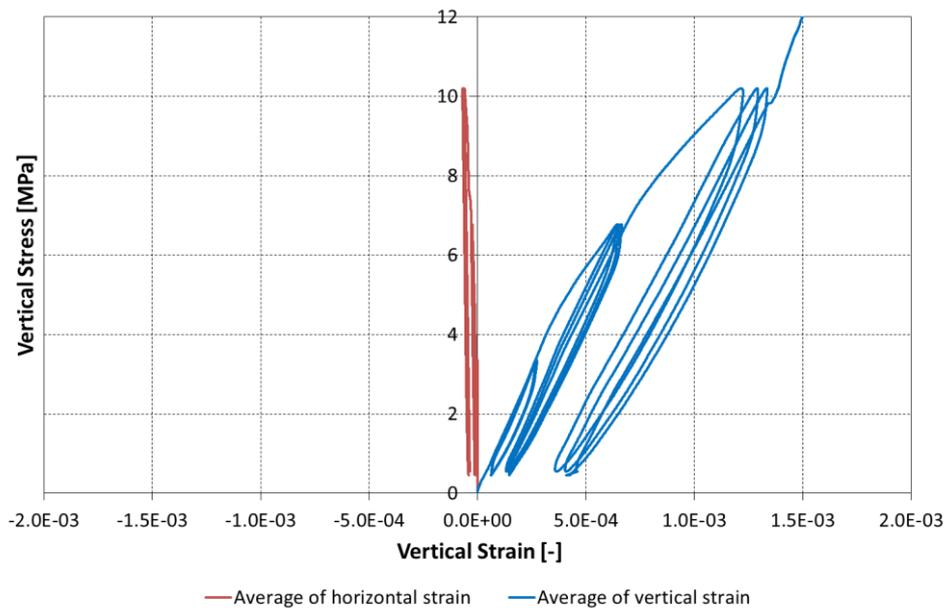
Figure 8.84 Vertical stress vs. vertical and horizontal strains for single wallette CTBSCL\_2S.
