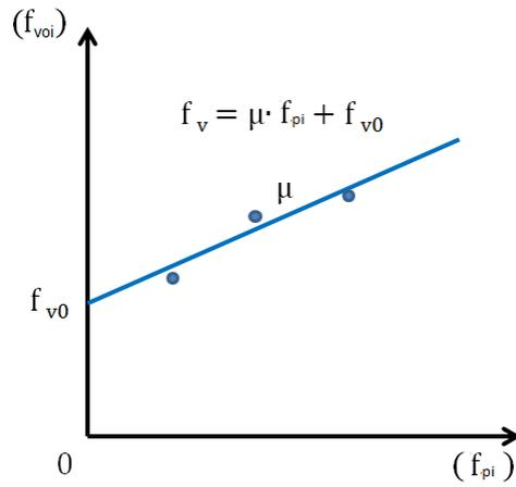
Figure 8.127 Theoretical determination of cohesion and angle of friction in the shear strength test.
