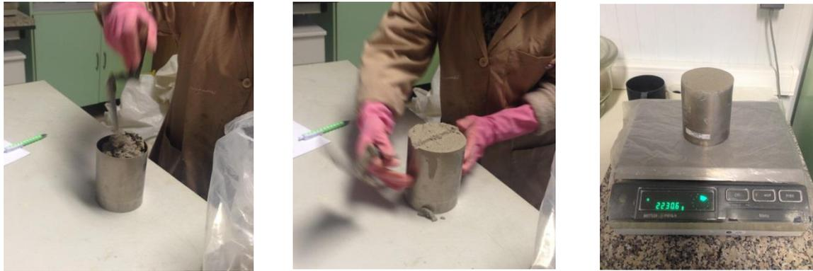
Figure 8.6 Carrying out the determination of bulk density of fresh study mortars.
