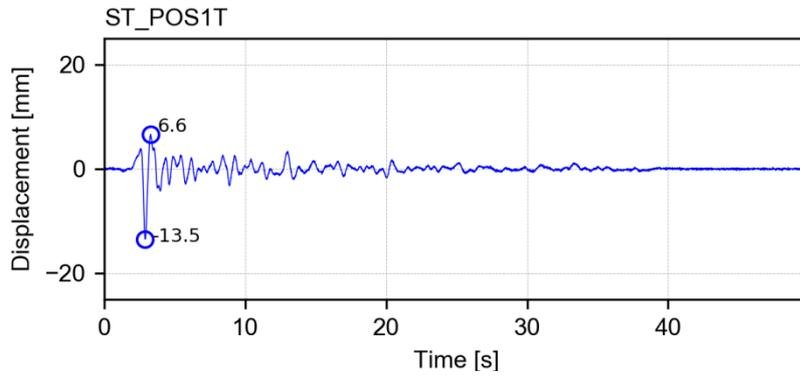
Channel *ST\_POS\_T* – Transverse displacement of the LNEC 3D shake table motion control
