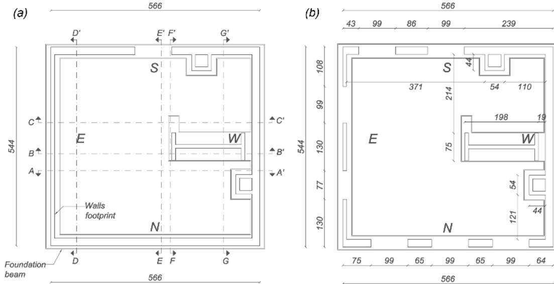
Figure 2.2 Plan of the building specimen: (a) walls footprint; (b) section at 1 m from the base. Units of cm.
