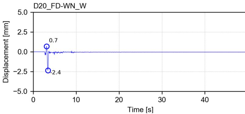
Channel D20\_FD-WN\_W – displacement
