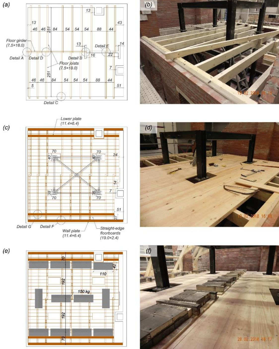
Figure 2.9 Floor framing: (a) floor framing plan; (b) floor joists during construction; (c) floorboards layout; (d) floor sheathing during construction; (e, f) additional masses on top of the floor. Units of cm.
