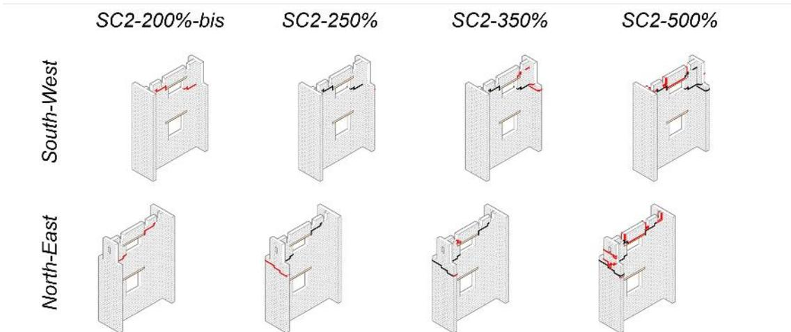
Figure 6.14 Evolution of the crack pattern of the interior wall. Cracks marked in red were observed at the end of the annotated test run. Cracks marked in black were already detected in previous test runs.
