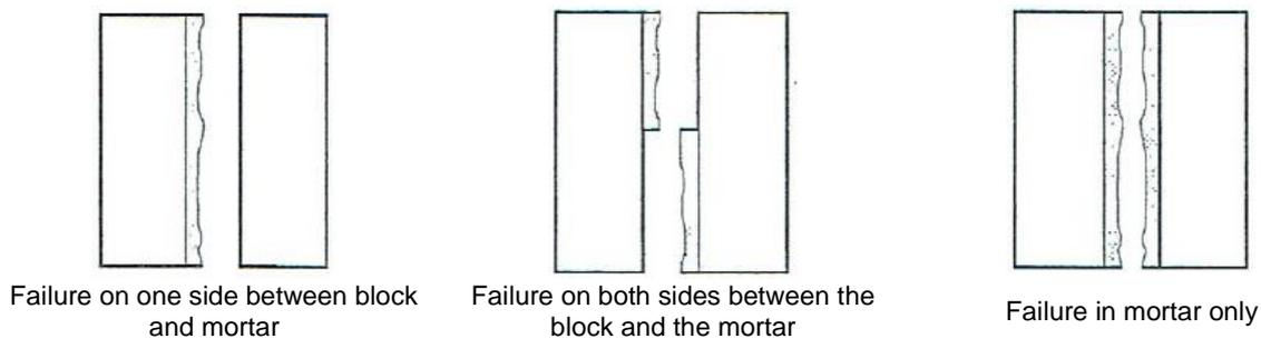
Figure 8.129 Acceptable collapse mechanisms for the shear strength test.
