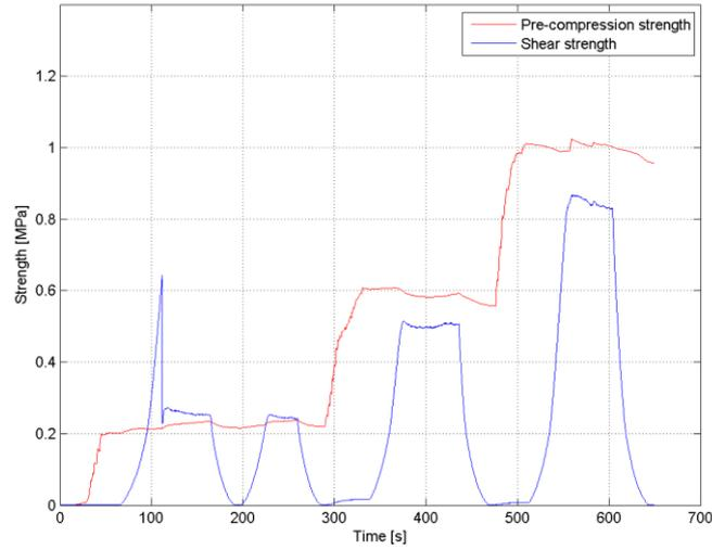
Figure 8.124 Application of the pre-compression and shear stresses throughout the test starting with the lowest pre-compression level (TBSCL\_2).
