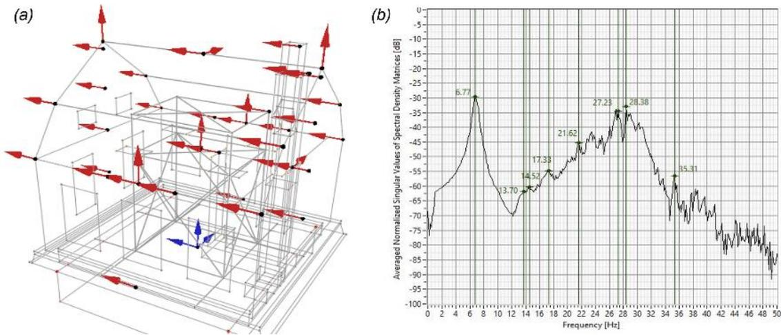
Figure 6.5 Dynamic identification test CHAR#0: (a) accelerometers location; (b) FDD analysis results.
