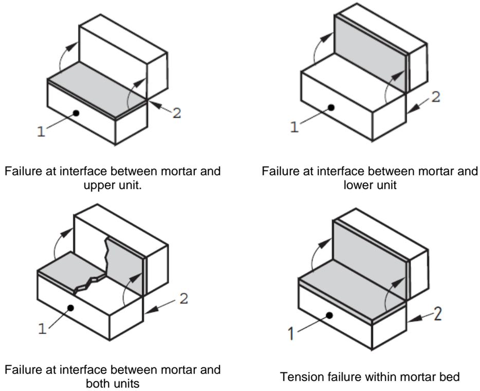
Figure 8.117 Admissible failure mechanisms for the bond wrench test.
