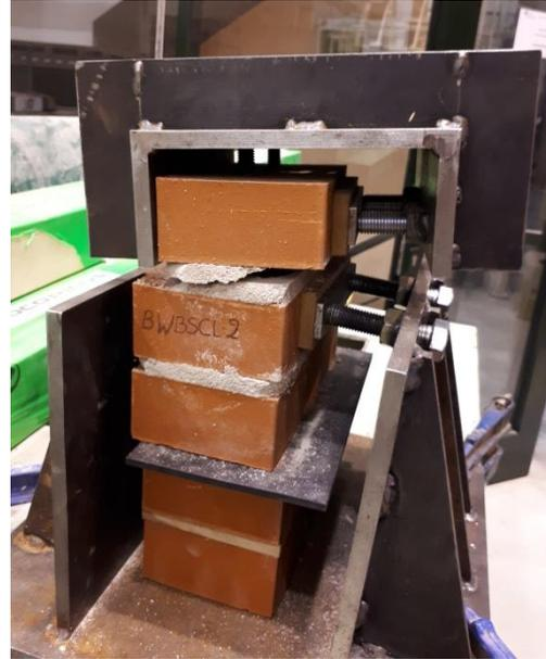
Failure of second joint
