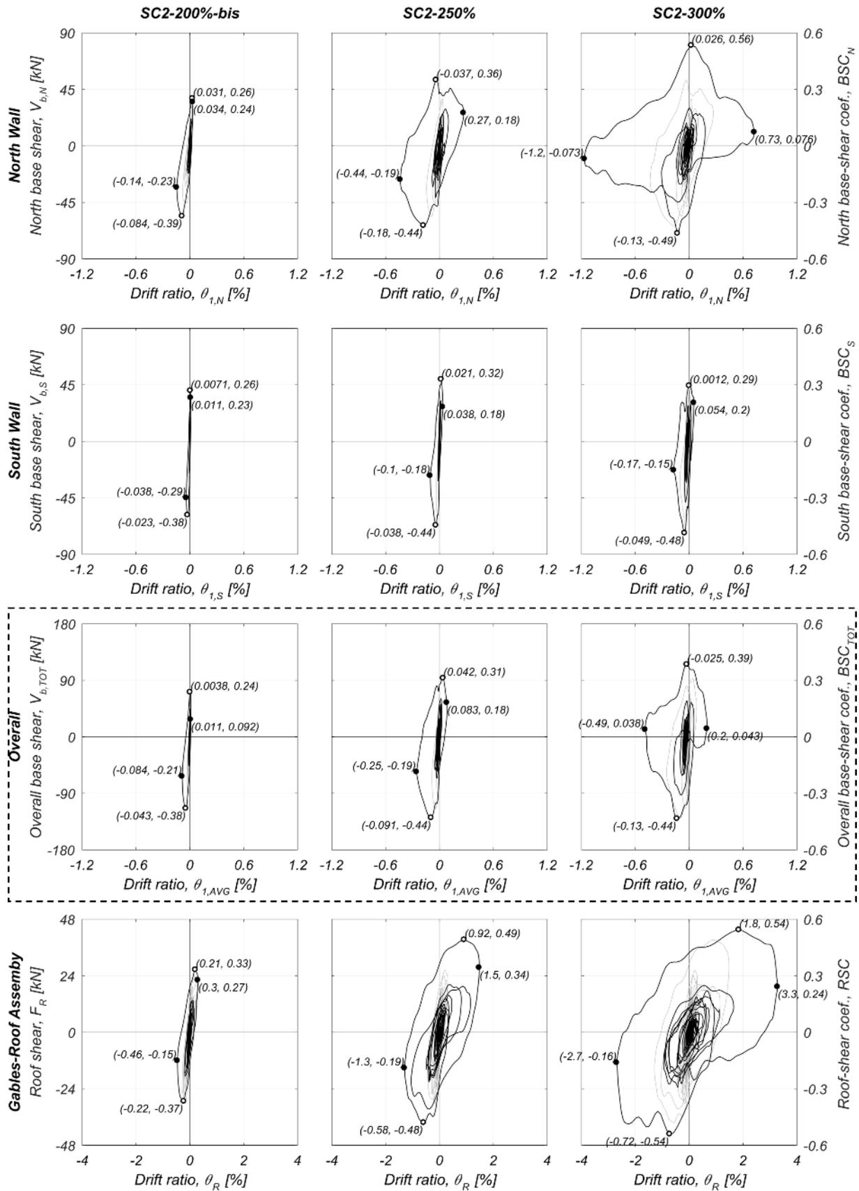
Figure 6.41 Specimen hysteretic responses: test runs SC2-200%-bis, SC2-250% and SC2-300%.
