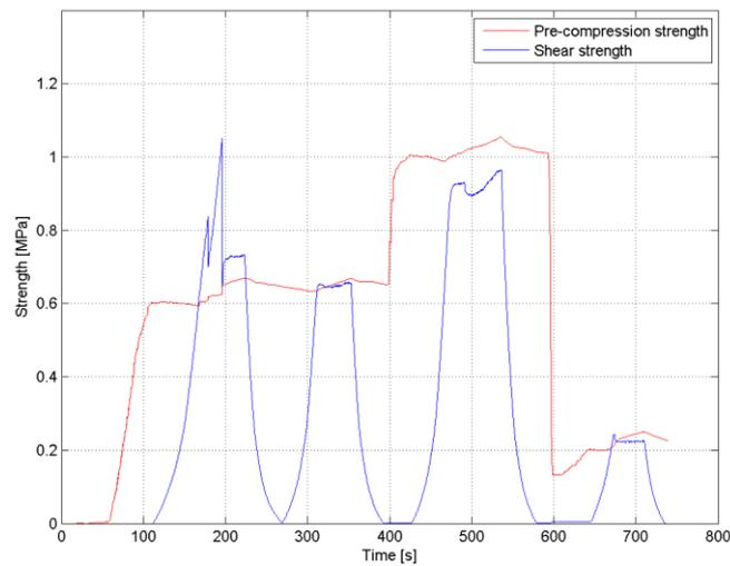
Figure 8.125 Application of the pre-compression and shear stresses throughout the test initiated with the intermediate pre-compression level (TBSCL\_5).
