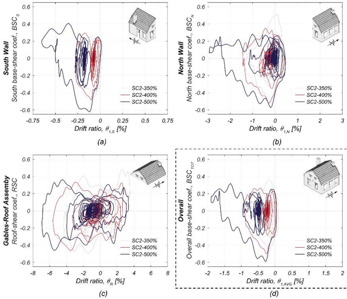
Figure 6.43 Specimen hysteretic responses during the last three earthquake simulations: (a) South subsystem; (b) North subsystem; (c) gables-roof subsystem; (d) Overall structure.
