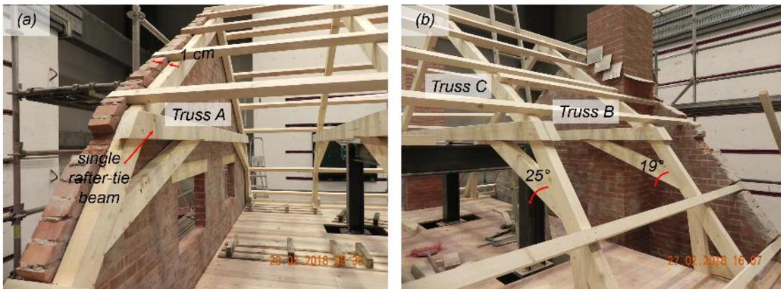
Figure 2.19 Construction details of the roof trusses: (a) Truss A and East gable; (b) Truss B and Truss C.
