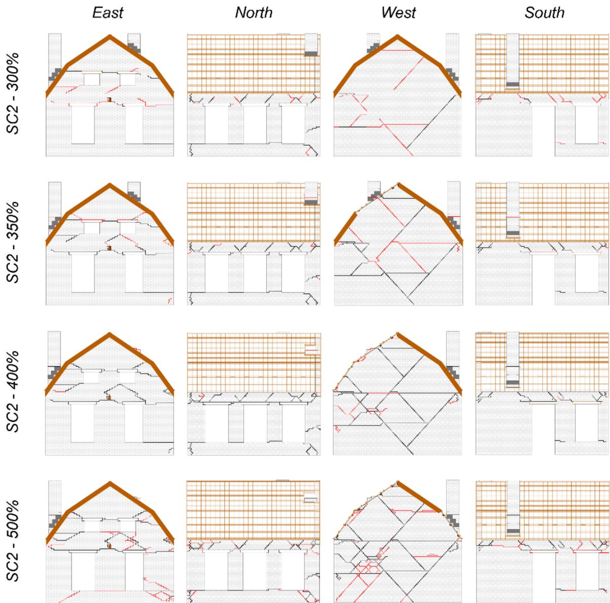
Figure 6.13 Evolution of the specimen crack pattern: tests SC2-300% to SC2-500%. Cracks marked in red were observed at the end of the annotated test run. Cracks marked in black were already detected in previous test runs.
