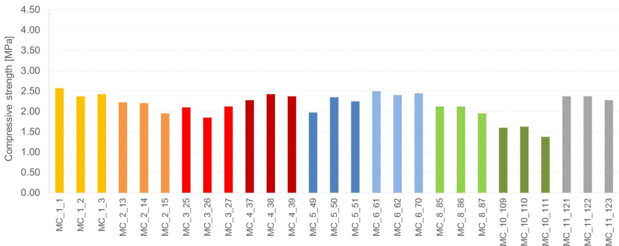
Figure 8.51 Compressive strength and modulus of elasticity test results for the mortars collected directly from the building prototype after 10 days of age.
