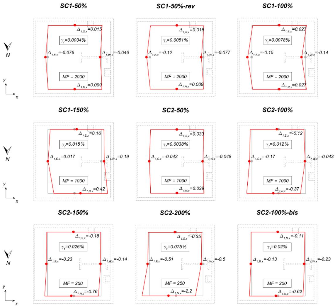
Figure 6.34 Deformed shapes of the floor at the instants of maximum diaphragm shear deformations: test runs SC1-50% to SC2-100%-bis. MF is the displacement magnification factor on the figure. Units of mm unless otherwise specified.
