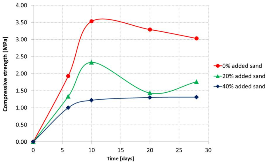
Figure 8.26 Maturation curve over time for the compressive strengths of MMC and MT mortars.
