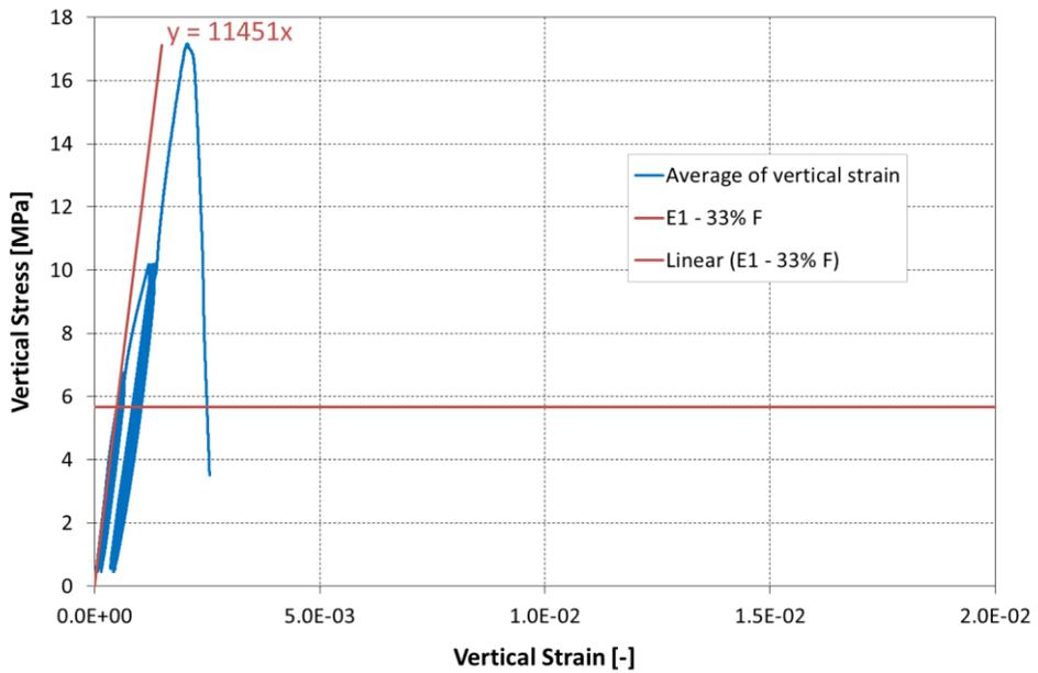
Figure 8.90 Vertical stress vs. vertical strain and determination of the modulus of elasticity for single wallette CTBSCL\_2S.
