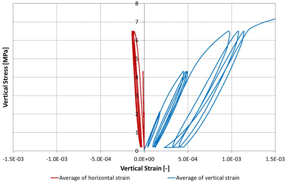
Figure 8.99 Vertical stress vs. vertical and horizontal strains for double wallette CTBSCL\_4D.
