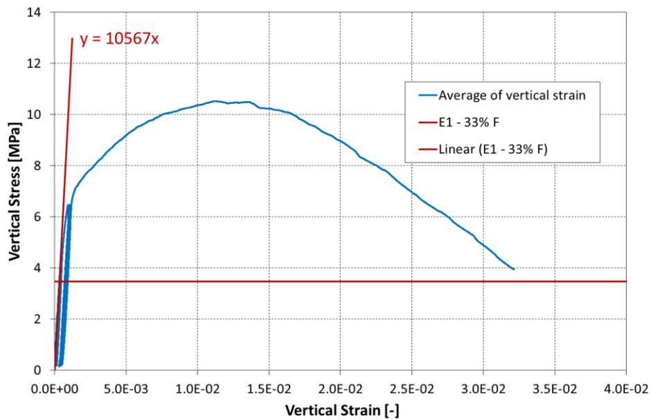
Figure 8.104 Vertical stress vs. vertical strain and determination of the modulus of elasticity for double wallette CTBSCL\_3D.
