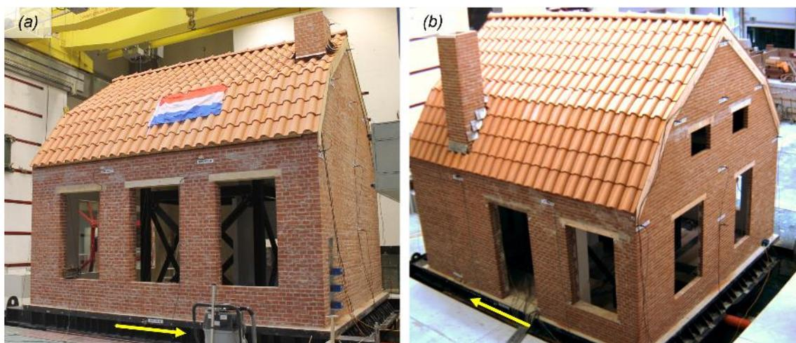
Figure 2.1 Full-scale building specimen: (a) North-West view; (b) South-East view. Arrows indicate the direction of shaking.
