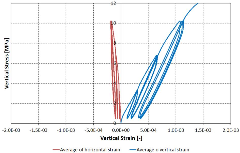
Figure 8.87 Vertical stress vs. vertical and horizontal strains for single wallette CTBSCL\_5S.
