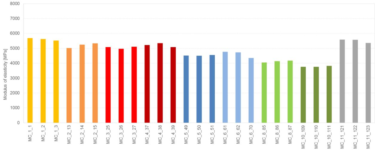
Figure 8.33 Test results for the determination of the dynamic modulus of elasticity for the mortars collected directly from the building prototype after 10 days of age.
