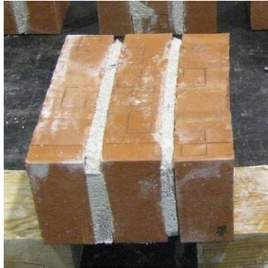
Figure 8.109 Type of specimens subjected to bond strength test.
