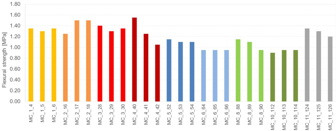
Figure 8.44 Flexural strength test results for the mortars collected directly from the building prototype after 20 days of age.
