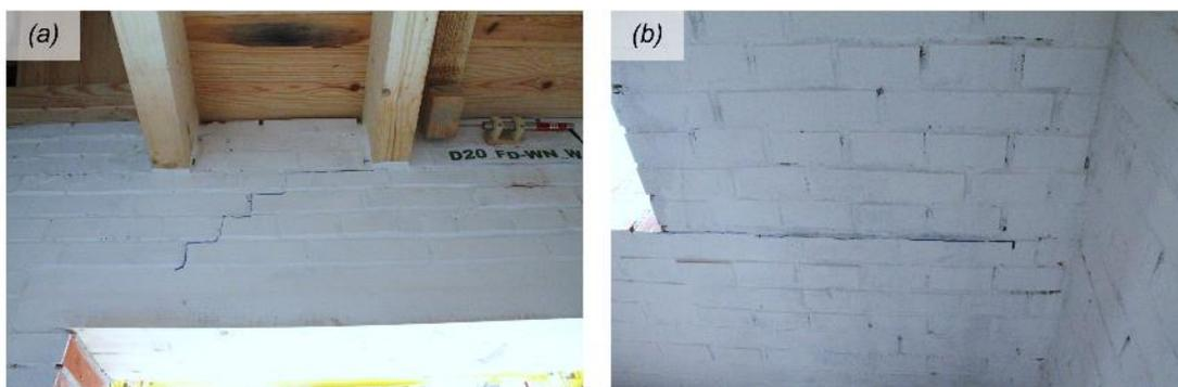
Figure 6.15 Damage on the North wall after test SC2-200%: (a) diagonal crack above the opening; (b) flexural crack at the base of the pier.
