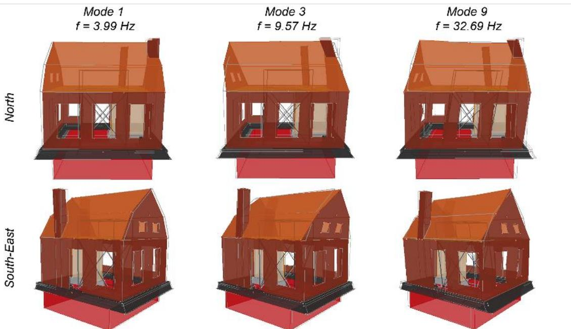
Figure 6.8 Dynamic identification test CHAR#9: vibration-mode shapes.
