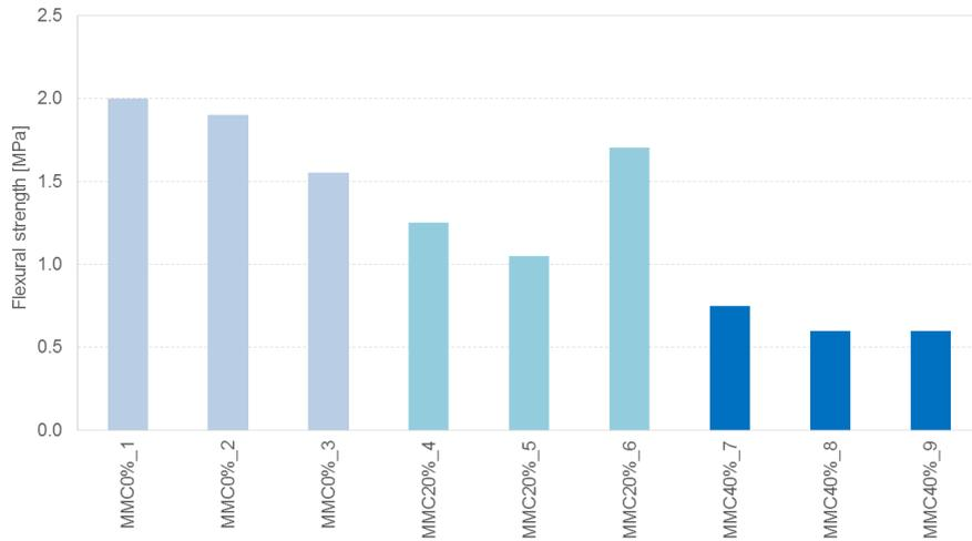
Figure 8.18 Flexural strength test results mortar for maturation curve (MMC\_0%, MMC\_20% and MMC\_40%) after 10 days of age.
