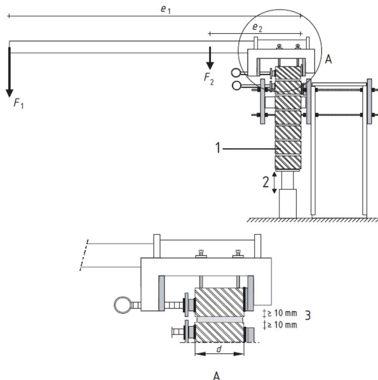
Figure 8.110 Example of a possible device for the test in accordance with EN 1052-5 (2005).
