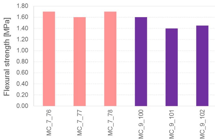
Figure 8.48 Flexural strength test results for the mortars collected directly from the characterisation specimens after 20 days of age.
