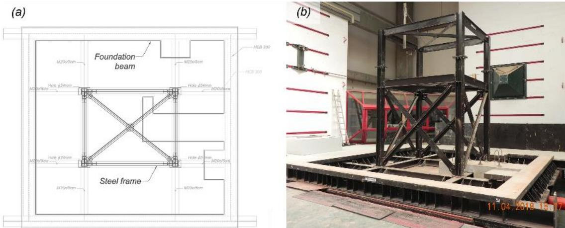
Figure 2.5 Building foundation and safety frame: (a) foundation plan; (b) North-West view of the steel frame.
