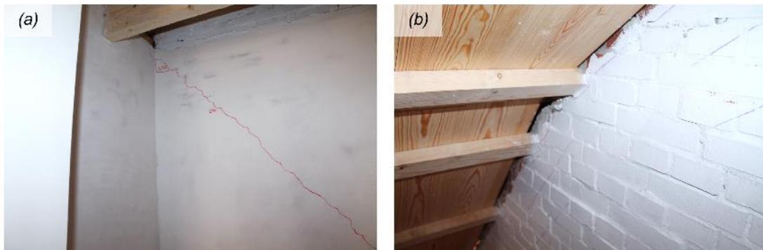
Figure 6.19 Damage on the West façade after test SC2-250%: (a) stair-stepped crack visible from the interior side; (b) damage to the connections between the roof purlins and the gable.
