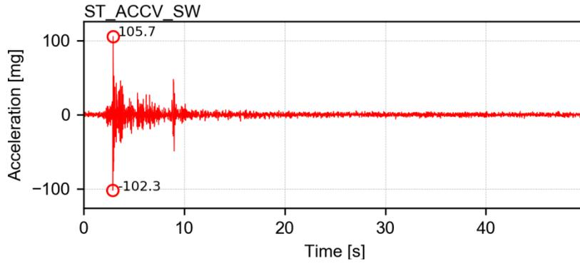
Channel ST\_ACCV\_SW – Vertical acceleration of the South-West LNEC 3D shake table platform
