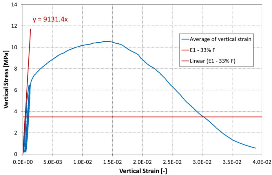
Figure 8.106 Vertical stress vs. vertical strain and determination of the modulus of elasticity for double wallette CTBSCL\_5D.
