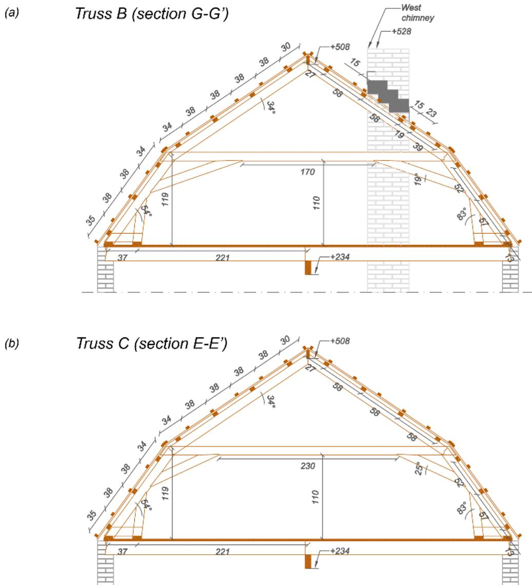
Figure 2.20 Elevation views of the roof trusses: (a) Truss B (section G-G'); (b) Truss C (section E-E'). Units of cm.
