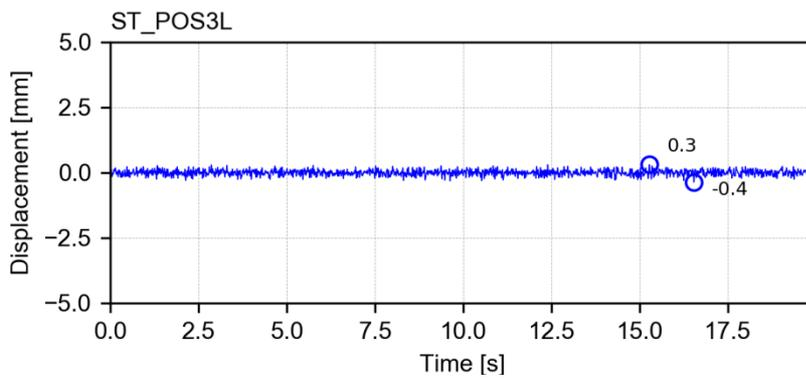
Channel ST\_POS\_L – Vertical displacement of the LNEC 3D shake table motion control
