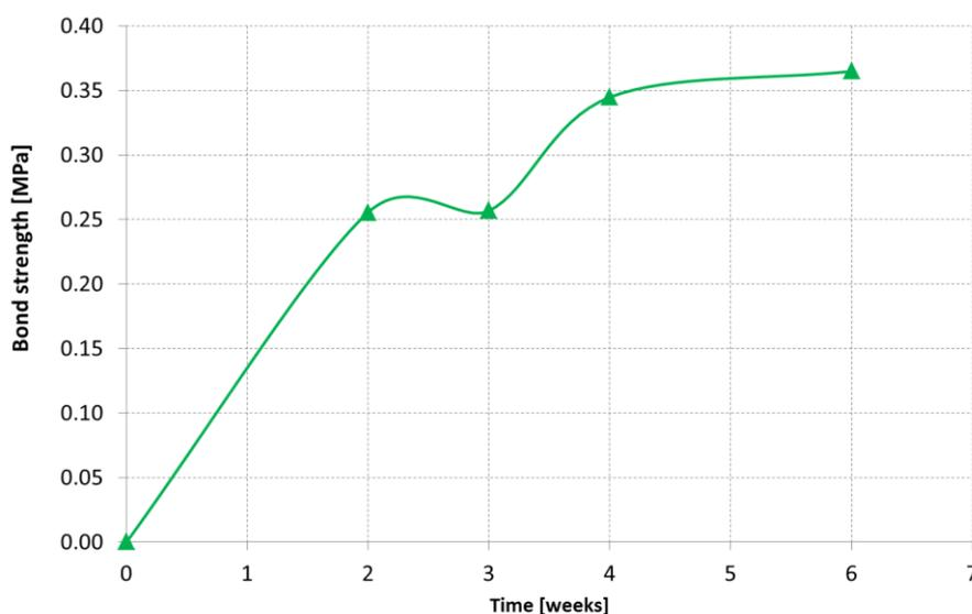
Figure 8.119 Maturation curve over time for the flexural bond strengths of triplets.
