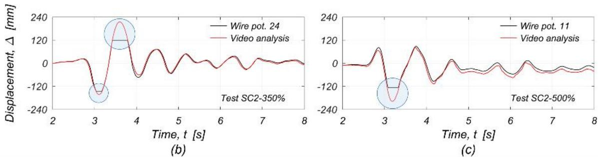
Figure 5.3 Retrieval of the missing data using software Tracker: (a) example of video analysis for the West chimney in test SC2-300%; (b) displacement histories for the West chimney in test SC2-350%; (c) displacement histories for the West gable wall, at mid-height, in test SC2-500%.
