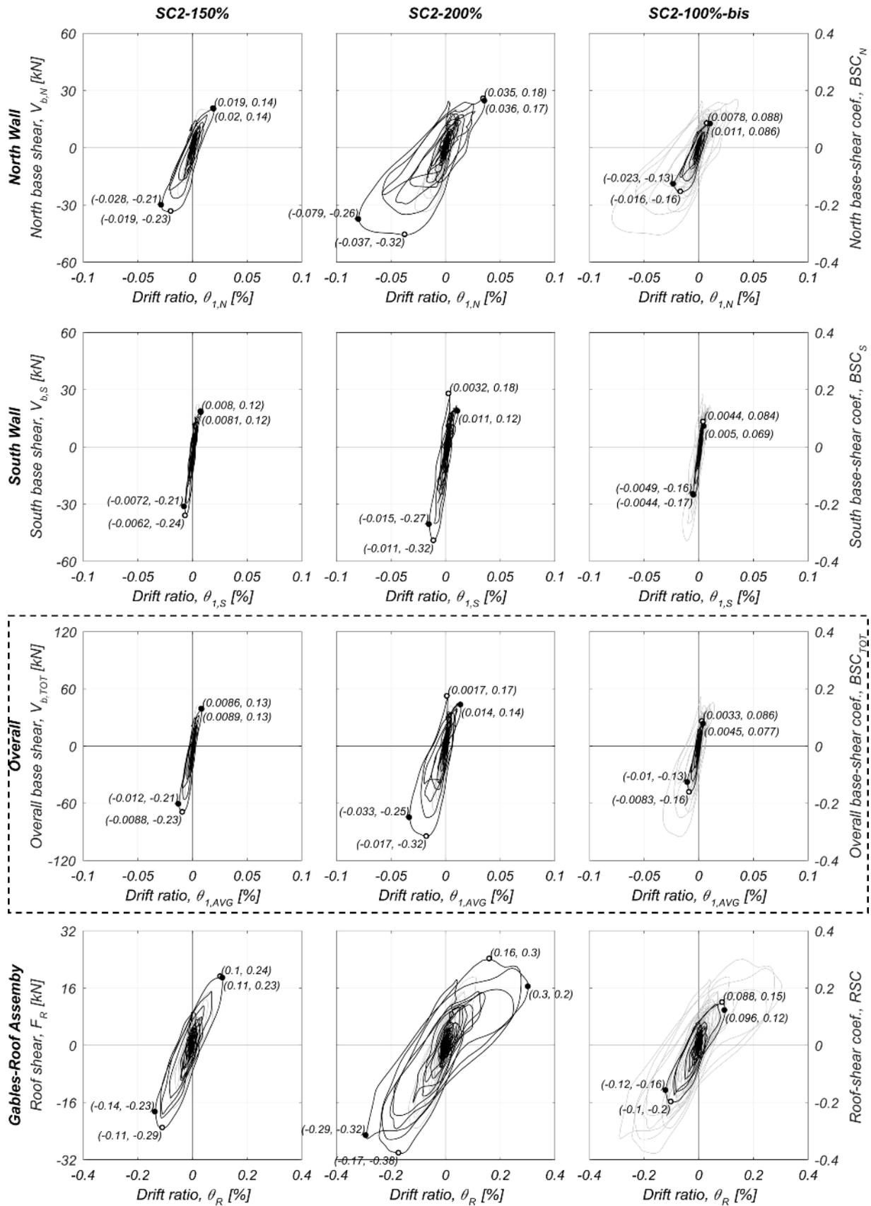
Figure 6.40 Specimen hysteretic responses: test runs SC2-150%, SC2-200% and SC2-100%-bis.
