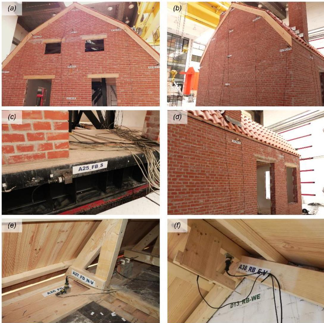
Figure 3.3 Accelerometers mounted on (a) the East façade; (b) the West façade; (c) the foundation beam; (d) the South façade; (e) the floor diaphragm; (f) the roof ridge beam.
