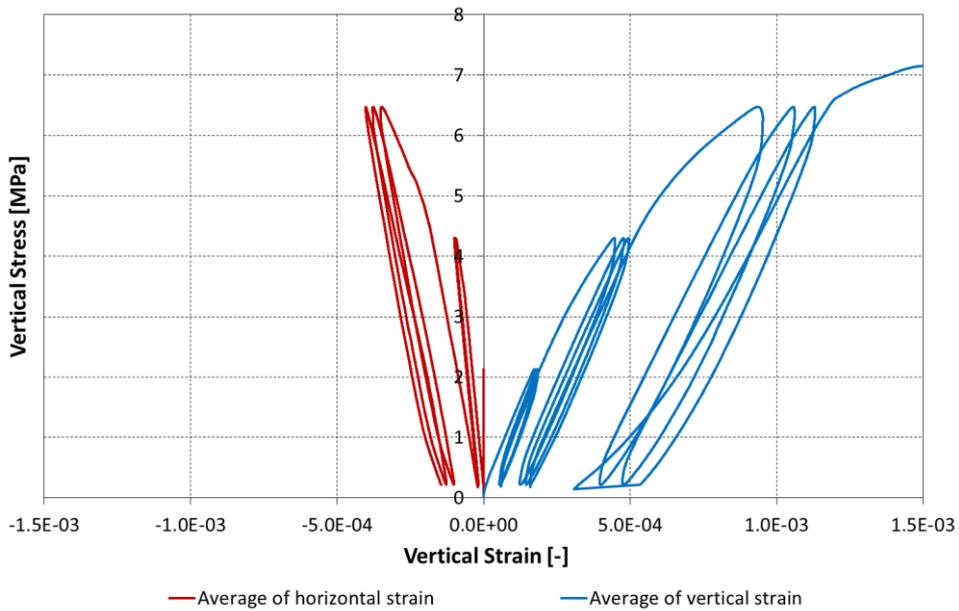
Figure 8.98 Vertical stress vs. vertical and horizontal strains for double wallette CTBSCL\_3D.
