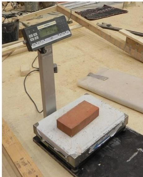
Figure 8.115 Measure of the weight of the top unit and adherent mortar.
