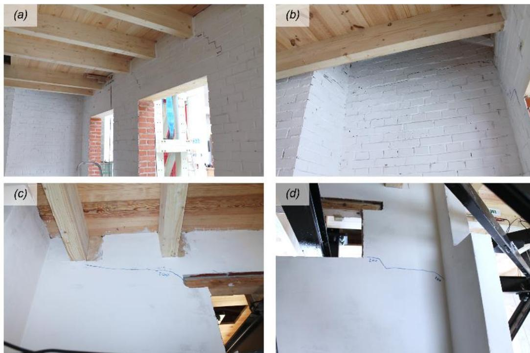
Figure 6.16 Damage after test SC2-200%-bis: (a) diagonal cracks above the openings of the North wall; (b) horizontal crack on the West façade; (c, d) cracks on the plaster of the interior wall.
