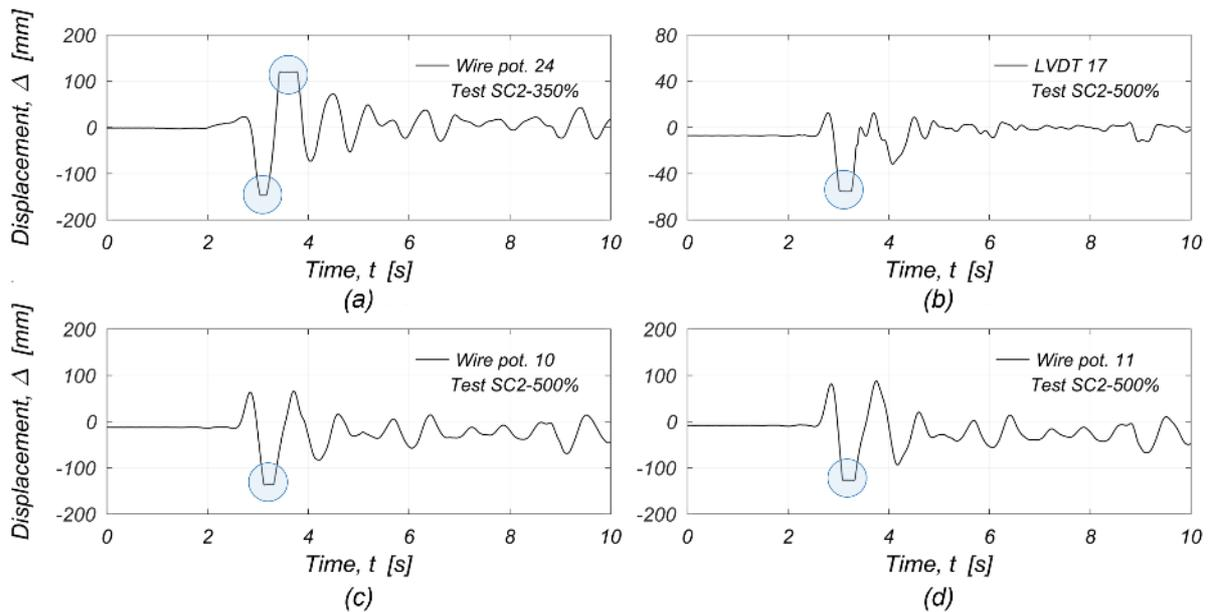
Figure 5.2 Saturated displacement transducers: (a) wire potentiometer at the top of the West chimney; (b) LVDT on the North side of the floor; (c) wire potentiometer at mid-height of the East gable; (d) wire potentiometer at mid-height of the West gable.
