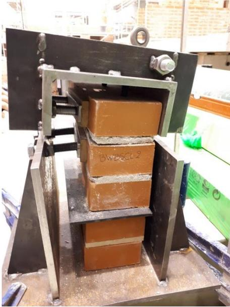
Failure of second joint
