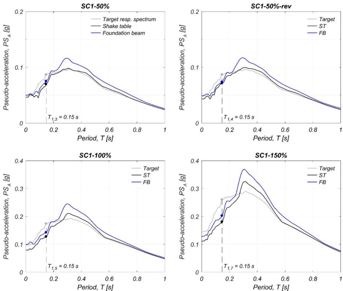
Figure 6.9 Comparison between elastic 5%-damped pseudo-acceleration response spectra of the actual input signals and target spectra for SC1 motions.
