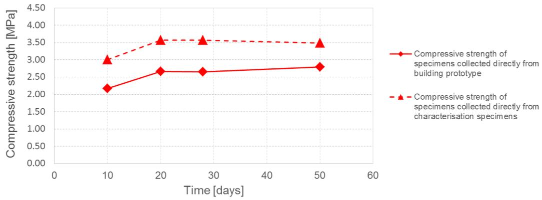
Figure 8.62 Relation between compressive strength and maturation time for the bedding mortars removed from the building prototype and the characterisation test specimens.
