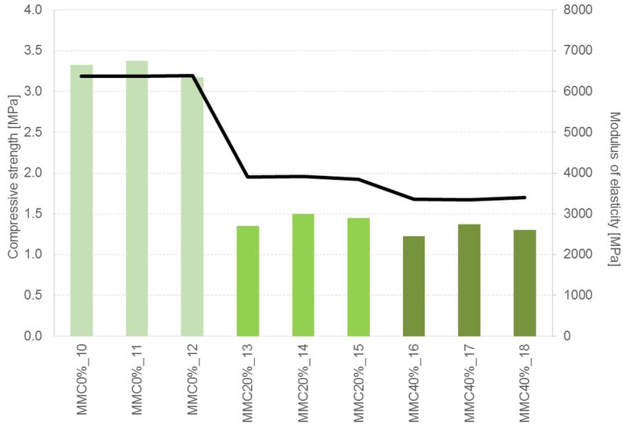
Figure 8.23 Compressive strength and modulus of elasticity test results for maturation curve (MMC\_0%, MMC\_20% and MMC\_40%) after 20 days of age.
