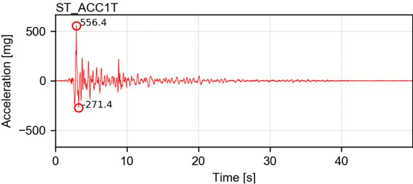
Channel ST\_ACC\_T – Transverse acceleration of the LNEC 3D shake table motion control
