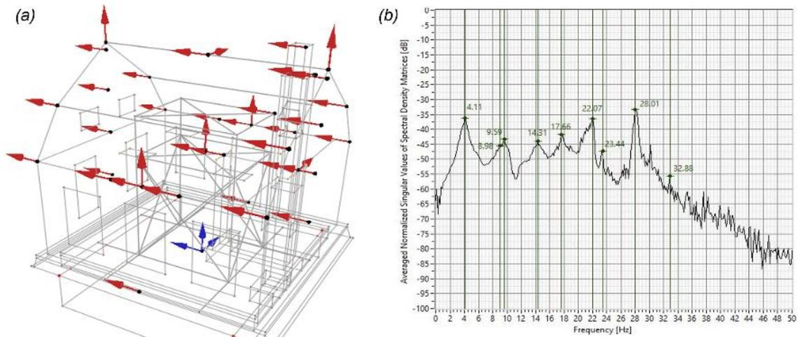
Figure 6.7 Dynamic identification test CHAR#9: (a) accelerometers location; (b) FDD analysis results.
