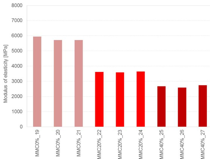
Figure 8.13 Test results for the determination of the dynamic modulus of elasticity of mortar for maturation curve (MMC\_0%, MMC\_20% and MMC\_40%) after 28 days of age.
