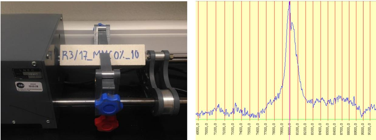
Figure 8.10 Performing the test to determine the dynamic modulus of elasticity and plot obtained.
