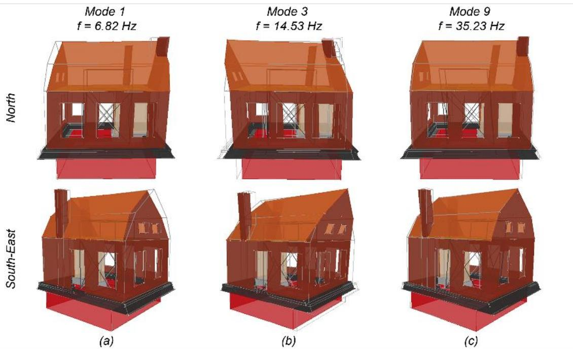
Figure 6.6 Dynamic identification test CHAR#0: vibration-mode shapes.
