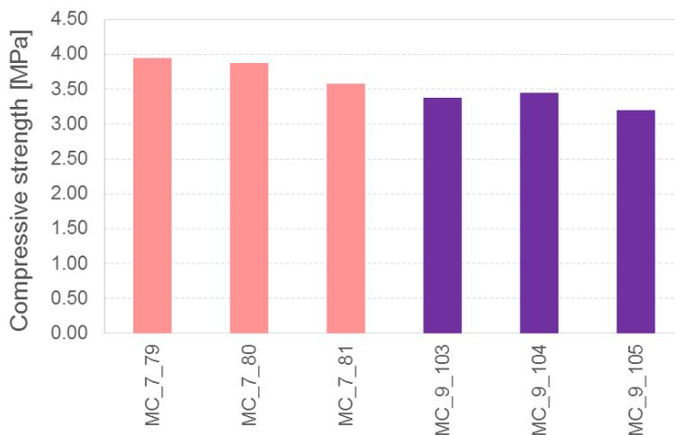
Figure 8.57 Compressive strength and modulus of elasticity test results for the mortars collected directly from the characterisation specimens after 28 days of age.
