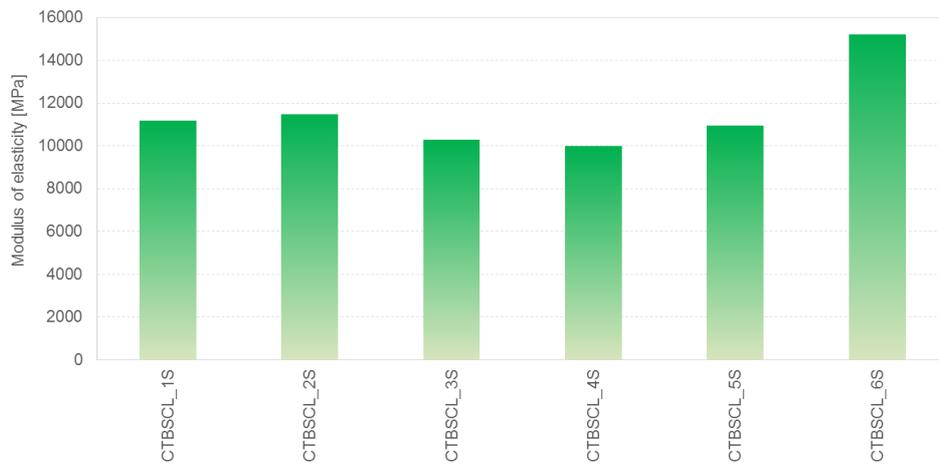
Figure 8.95 Distribution of moduli of elasticity obtained for single wallettes.
