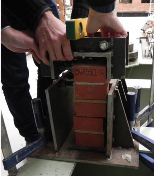
Figure 8.113 Application of vertical force until bond failure.
