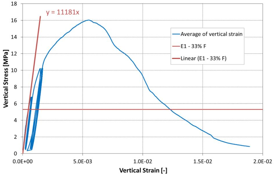
Figure 8.89 Vertical stress vs. vertical strain and determination of the modulus of elasticity for single wallette CTBSCL\_1S.
