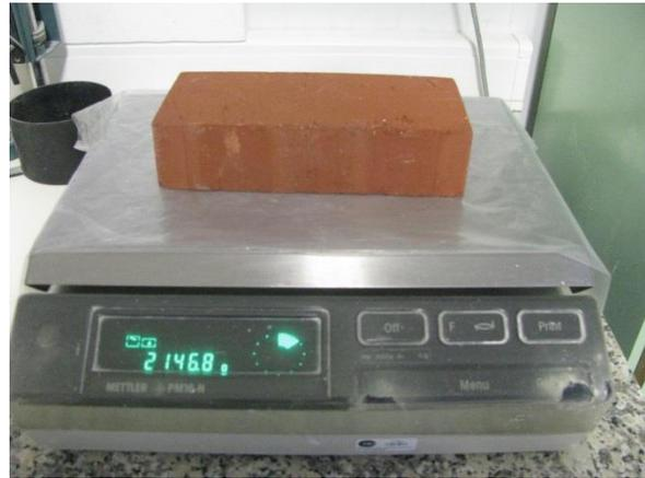
Figure 8.69 Weighing of blocks.
