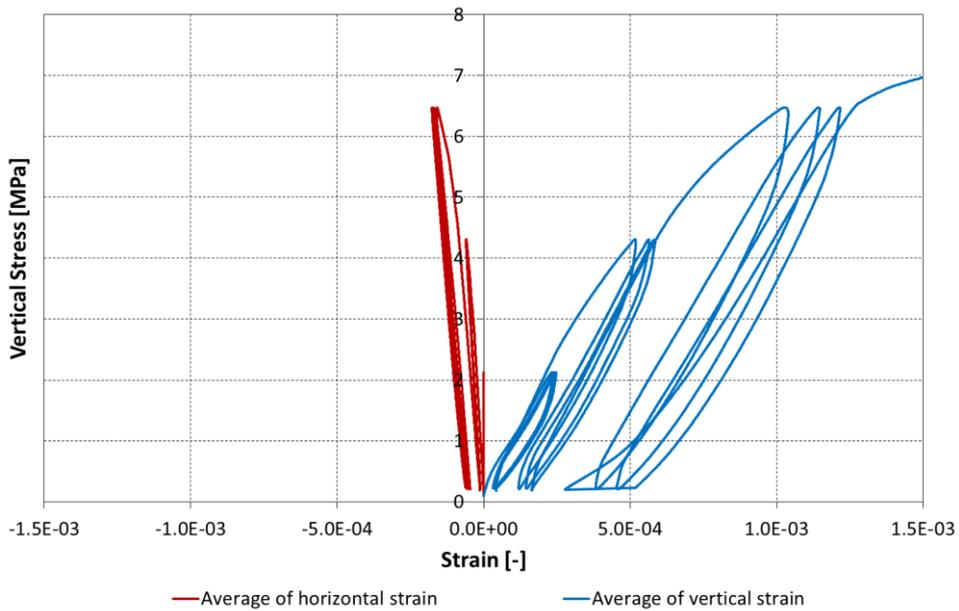
Figure 8.100 Vertical stress vs. vertical and horizontal strains for double wallette CTBSCL\_5D.
