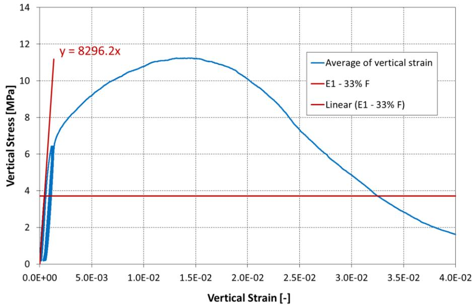
Figure 8.107 Vertical stress vs. vertical strain and determination of the modulus of elasticity for double wallette CTBSCL\_6D.
