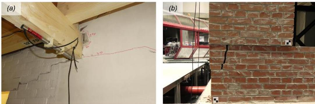
Figure 6.30 Damage on the East façade after test SC2-400%: (a) cracking around the support of the floor girder; (b) permanent sliding at the North-East corner.
