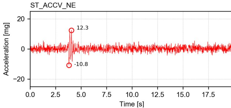
Channel ST\_ACCV\_NE – Vertical acceleration of the North-East LNEC 3D shake table platform
