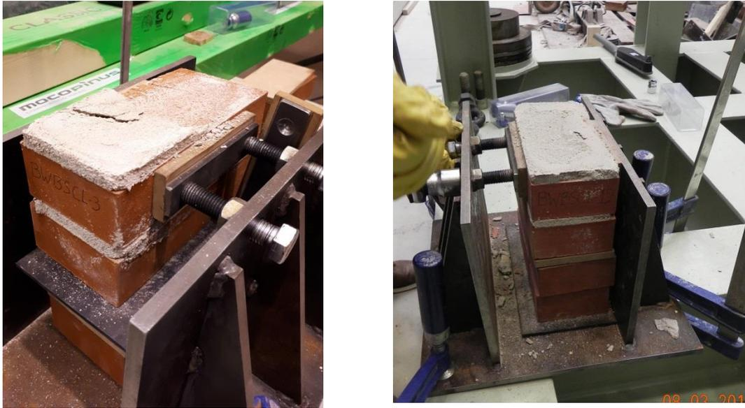
Figure 8.118 Example of failure mechanisms obtained for triplets in the bond wrench test.
