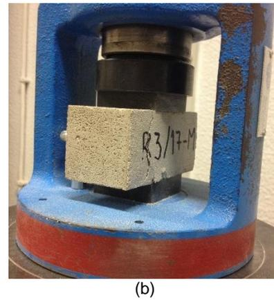
Figure 8.16 Test for compressive strength: (a) test scheme and (b) specimen being tested.
