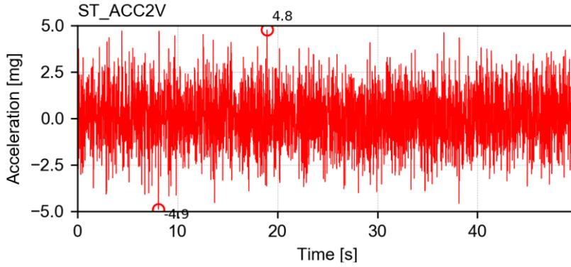
Channel ST\_ACC\_L – Vertical acceleration of the LNEC 3D shake table motion control
