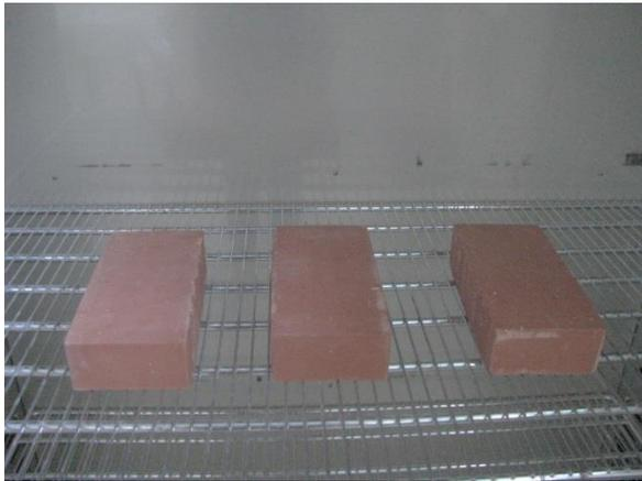
Figure 8.68 Drying the blocks in a ventilated oven.
