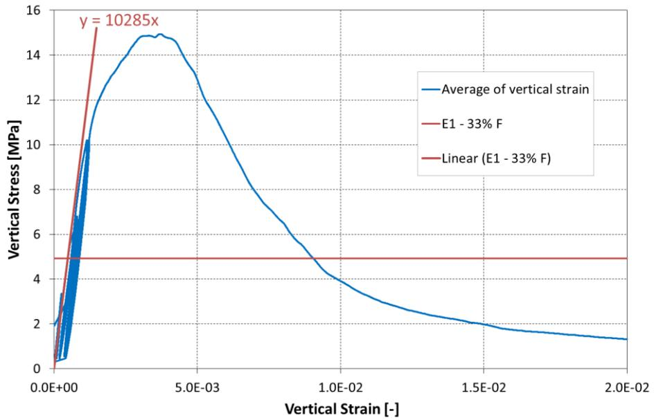
Figure 8.91 Vertical stress vs. vertical strain and determination of the modulus of elasticity for single wallette CTBSCL\_3S.
