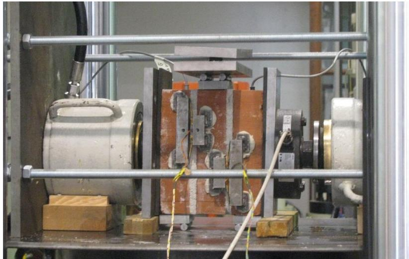
Figure 8.123 Device used in shear test.
