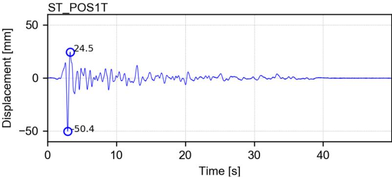
Channel ST\_POS\_T – Transverse displacement of the LNEC 3D shake table motion control
