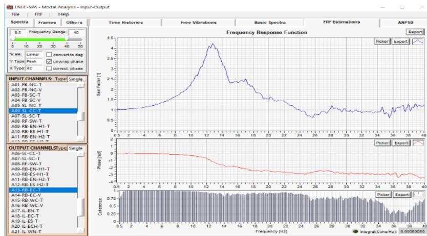
Figure 6.2 Specimen dynamic identification: frequency response function from the accelerations recorded in the longitudinal direction of the specimen.
