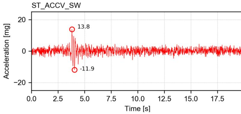
Channel ST\_ACCV\_SW – Vertical acceleration of the South-West LNEC 3D shake table platform
