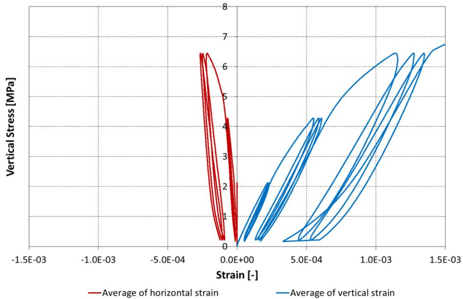
Figure 8.101 Vertical stress vs. vertical and horizontal strains for double wallette CTBSCL\_6D.
