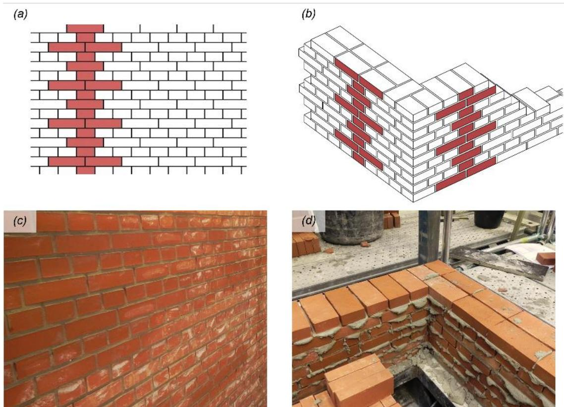
Figure 2.6 Construction details of the building specimen: (a, b) Dutch cross bond scheme; (c) brickwork bond of the West building façade; (d) interlocking of walls at the South-West corner.
