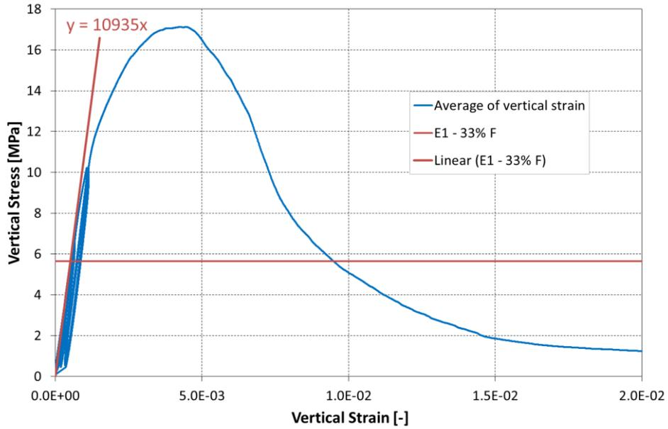
Figure 8.93 Vertical stress vs. vertical strain and determination of the modulus of elasticity for single wallette CTBSCL\_5S.
