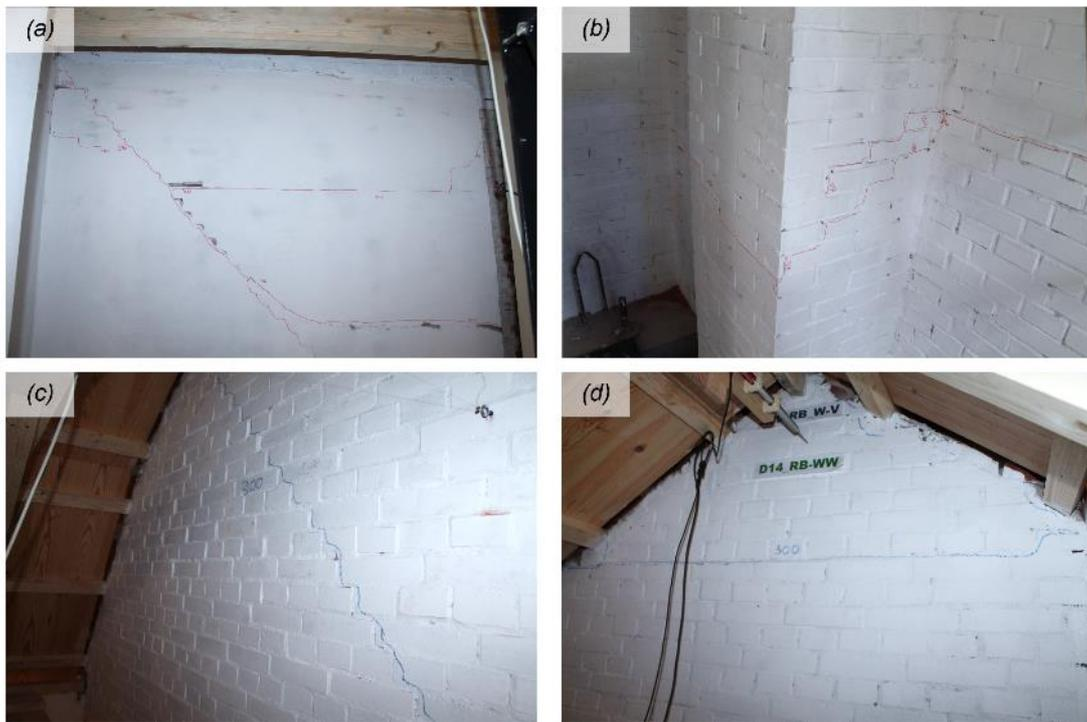
Figure 6.22 Damage on the West façade after test SC2-300%: (a, b) cracks at mid-height of the first storey; (c, b) cracks on the gable wall.
