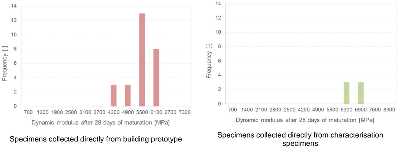
Figure 8.41 Distribution of the dynamic modulus of elasticity of collected mortars after 28 days of age.
