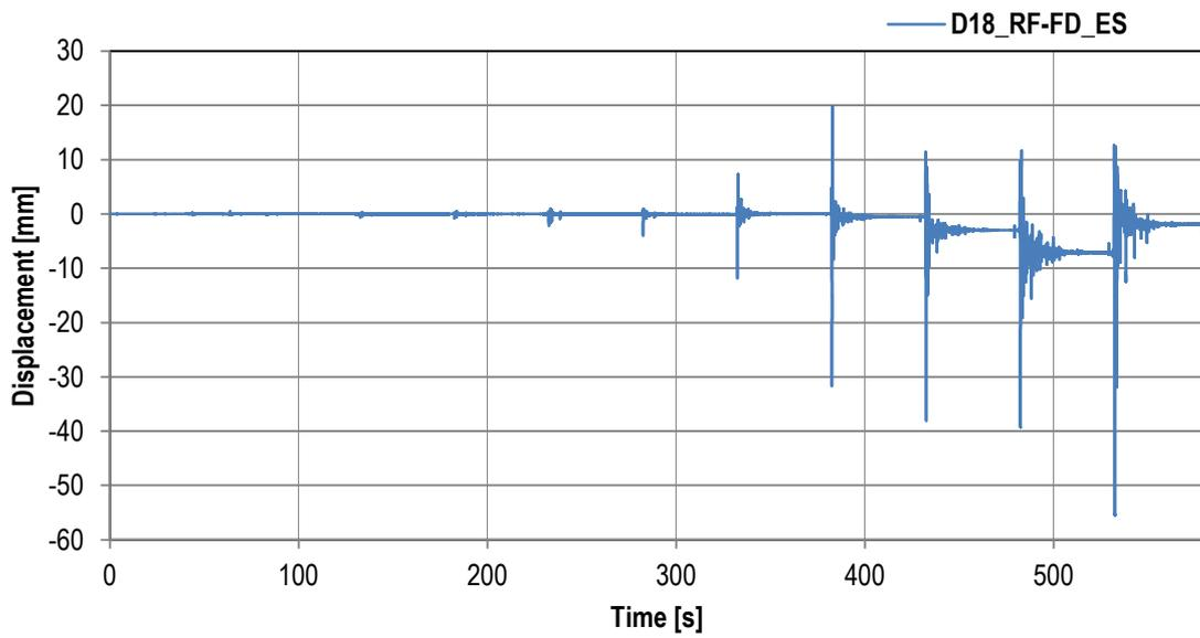
Channel D18\_RF-FD\_ES – Relative displacement
