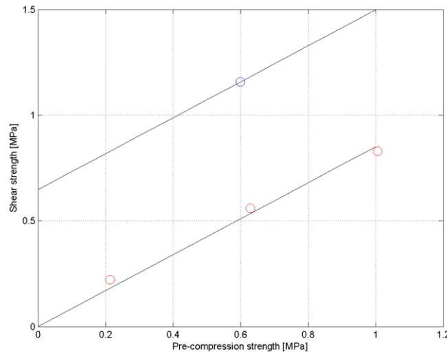
Figure 8.128 Determination of cohesion and friction angle for specimen TS\_3.
