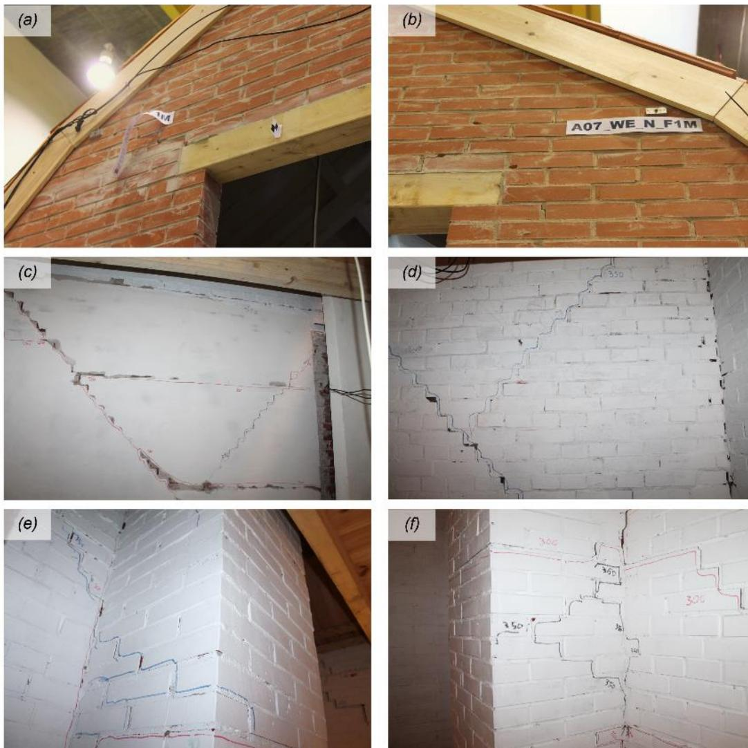
Figure 6.27 Damage on the transverse walls after test SC2-350%: (a, b) diagonal cracks propagating from the lintels to the supports of the purlins on the East gable wall; (c, d) new horizontal and diagonal cracks in both stories of the West wall; (e, f) damage at the connection of the chimney to the West building façade.
