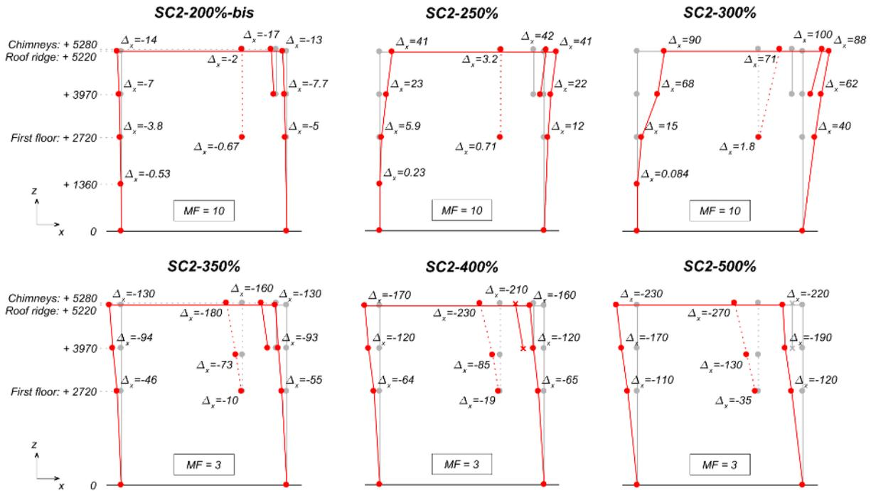
Figure 6.37 Displacement profiles at midspan of the transverse walls, at the instants of maximum roof ridge displacements: test runs SC2-200%-bis to SC2-500%. MF is the displacement magnification factor on the figure. Units of mm.
