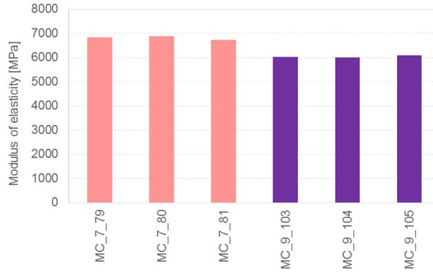
Figure 8.39 Test results for the determination of the dynamic modulus of elasticity for the mortars collected directly from the characterisation specimens after 28 days of age.
