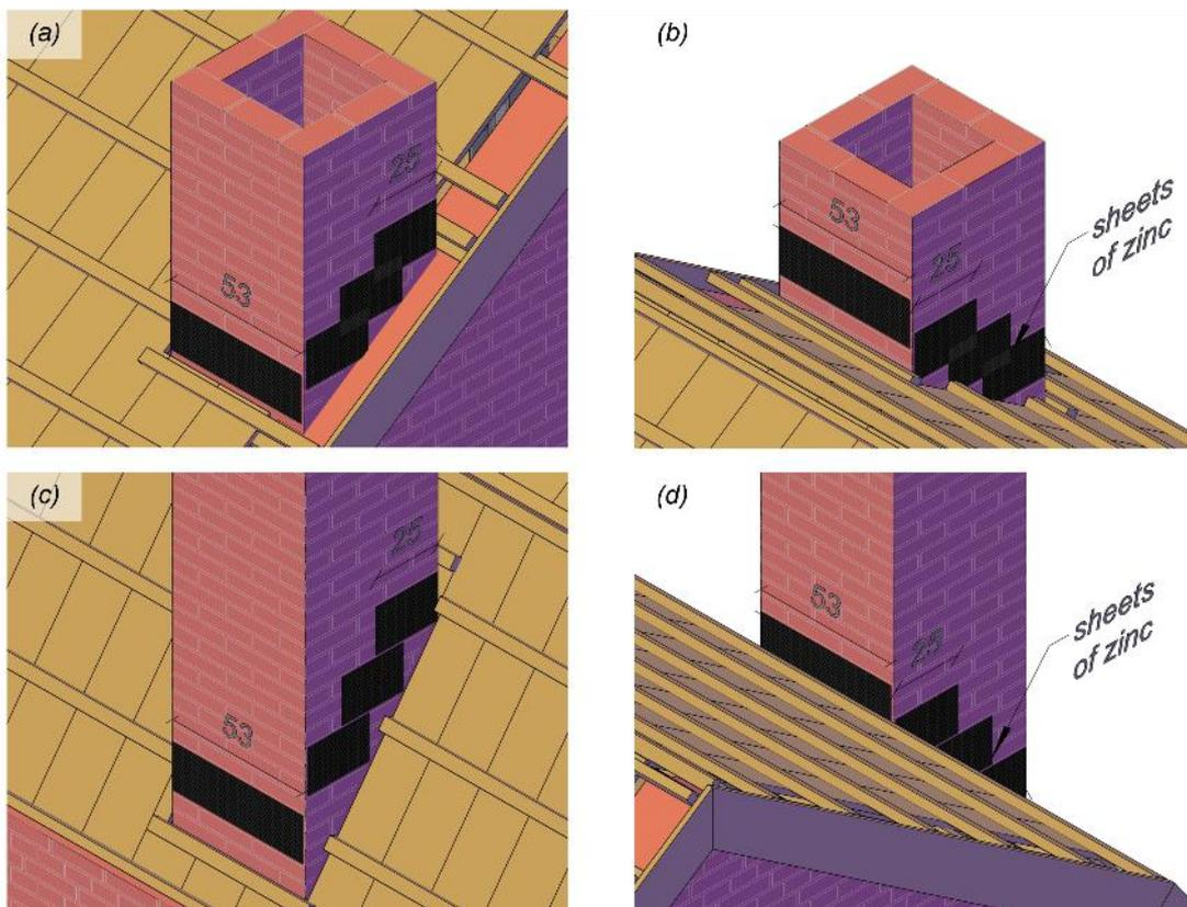
Figure 2.24 Chimney flashing: (a) North-West view of West chimney; (b) South-East view of West chimney; (c) South-East view of South chimney; (d) North-West view of South chimney.
