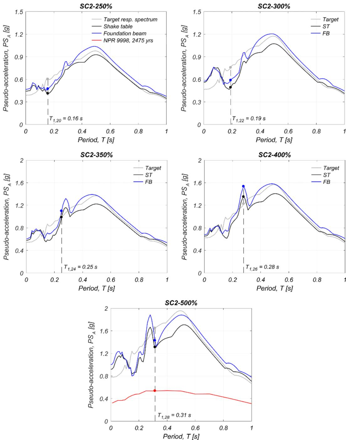
Figure 6.11 Comparison between elastic 5%-damped pseudo-acceleration response spectra of the actual input signals and target spectra for SC2 motion scaled from 250% to 500%. Comparison against the NPR 9998 (2017) elastic spectrum for events with return period 2475 years for the area of Loppersum, Groningen (lat. 53.33, long. 6.75)
