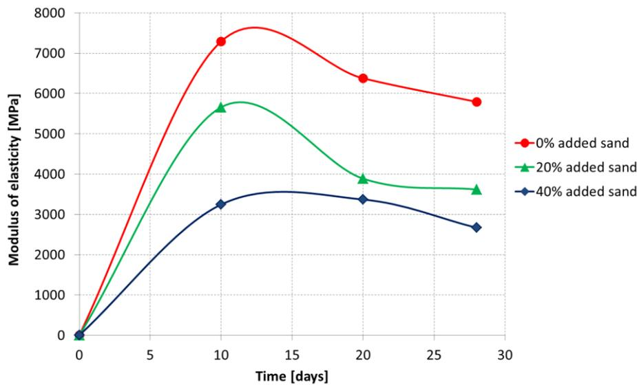
Figure 8.14 Maturation curve over time for the dynamic modulus of elasticity of MMC mortars.
