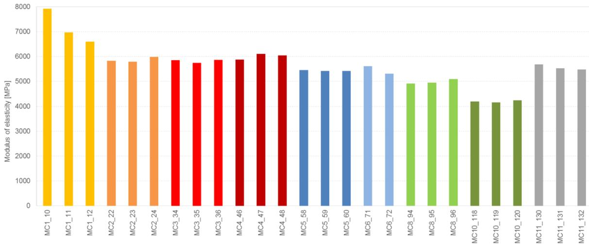
Figure 8.36 Test results for the determination of the dynamic modulus of elasticity for the mortars collected directly from the building prototype during the seismic test.
