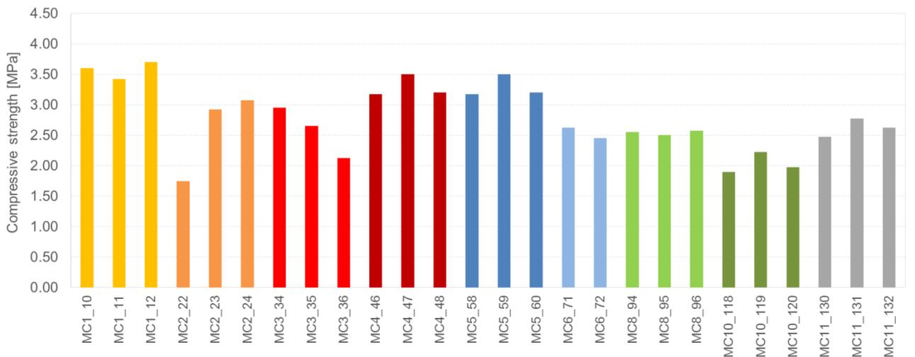
Figure 8.54 Compressive strength and modulus of elasticity test results for the mortars collected directly from the building prototype during the seismic test.
