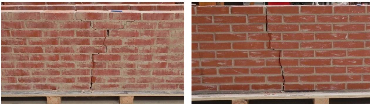
Figure 8.134 Failure mechanisms in out-of-plane bending tests.
