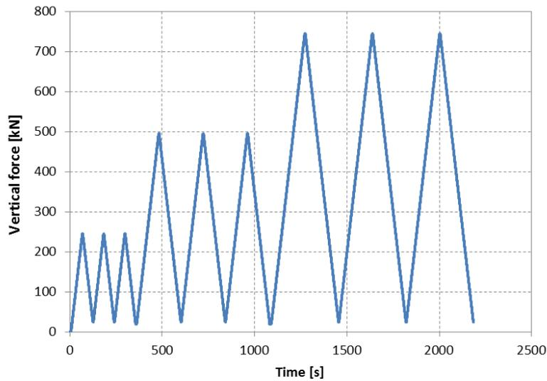
Figure 8.80 Application of force as a function of time for the double wallettes.
