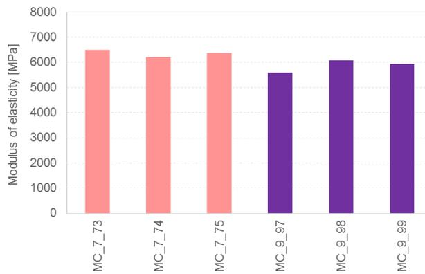
Figure 8.37 Test results for the determination of the dynamic modulus of elasticity for the mortars collected directly from the characterisation specimens after 10 days of age.
