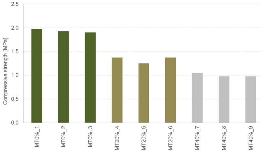
Figure 8.21 Compressive strength and modulus of elasticity test results for mortar test (MT\_0%, MT\_20% and MT\_40%) after 6 days of age.
