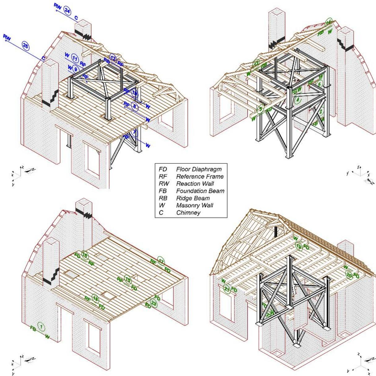
Figure 3.2 Instrumentation plan: wire potentiometers (blue) and LVDTs (green). Letters indicate the component on which each instrument is mounted.
