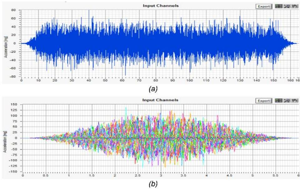
Figure 6.1 Specimen dynamic identification: (a) input acceleration history; (b) windowed average input.
