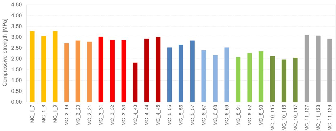
Figure 8.53 Compressive strength and modulus of elasticity test results for the mortars collected directly from the building prototype after 28 days of age.
