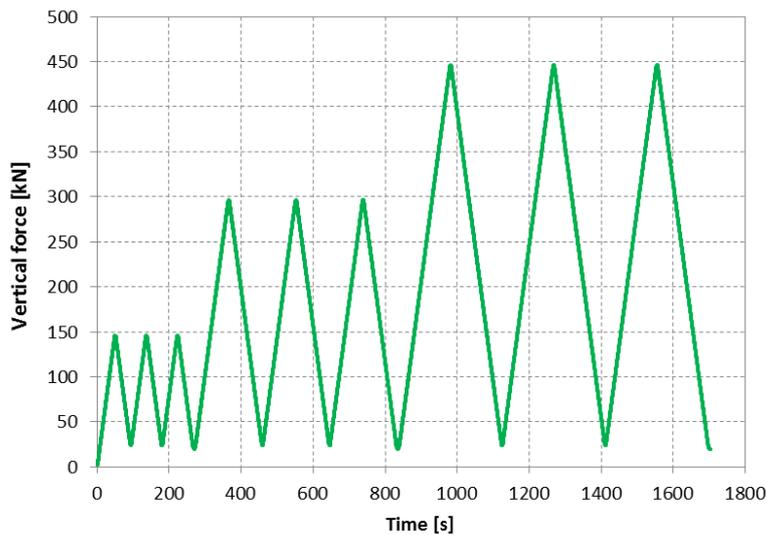
Figure 8.79 Application of force as a function of time for the single *wallettes*.
