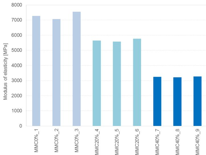
Figure 8.11 Test results for the determination of the dynamic modulus of elasticity of mortar for maturation curve (MMC\_0%, MMC\_20% and MMC\_40%) after 10 days of age.
