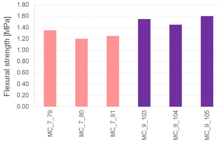
Figure 8.49 Flexural strength test results for the mortars collected directly from the characterisation specimens after 28 days of age.
