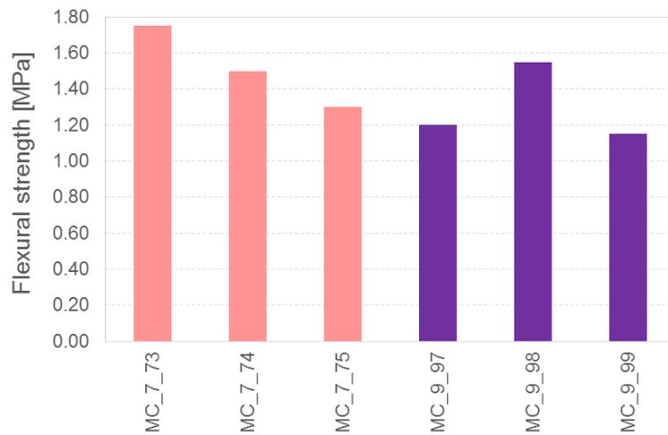
Figure 8.47 Flexural strength test results for the mortars collected directly from the characterisation specimens after 10 days of age.
