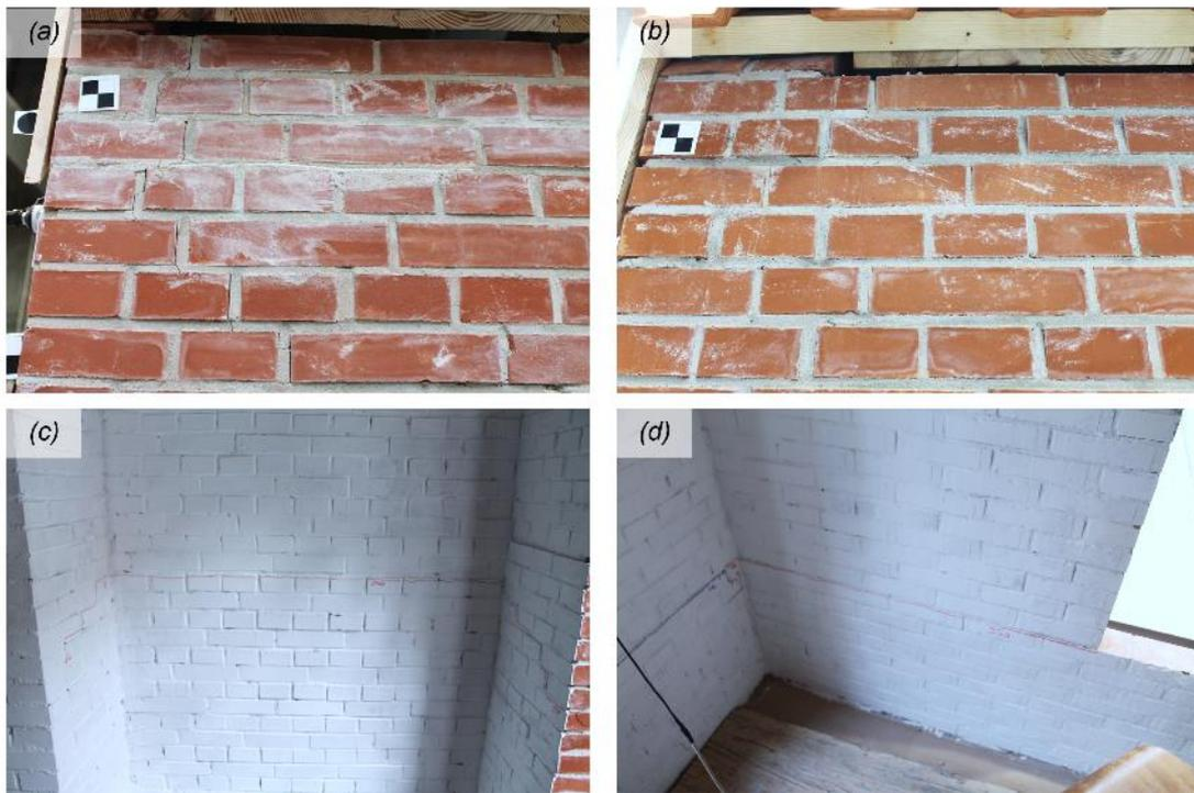
Figure 6.18 Damage due to interaction between in-plane and out-of-plane wall responses after test SC2-250%: (a, b) vertical cracks at the top of the longitudinal corner piers; (c) horizontal crack at mid-height of the West façade; (d) horizontal crack along the base of a pier of the East façade.
