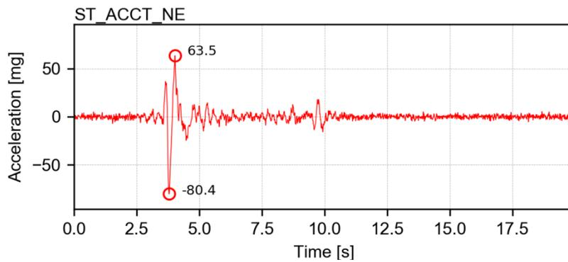
Channel ST\_ACCT\_NE – Transverse acceleration of the North-East LNEC 3D shake table platform
