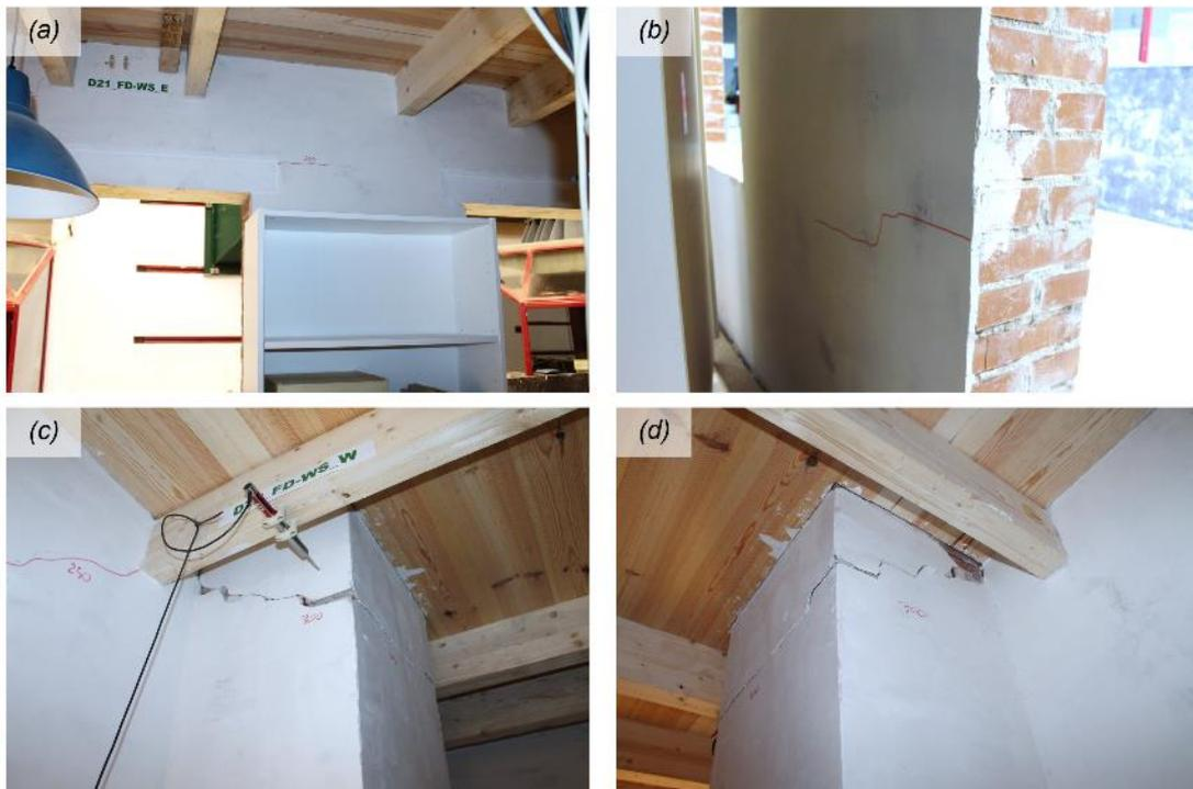
Figure 6.25 Damage on the South building façade after test SC2-300%: (a, b) cracks at the top and bottom ends of the central pier; (c, d) flexural crack at the base of the chimney stack.
