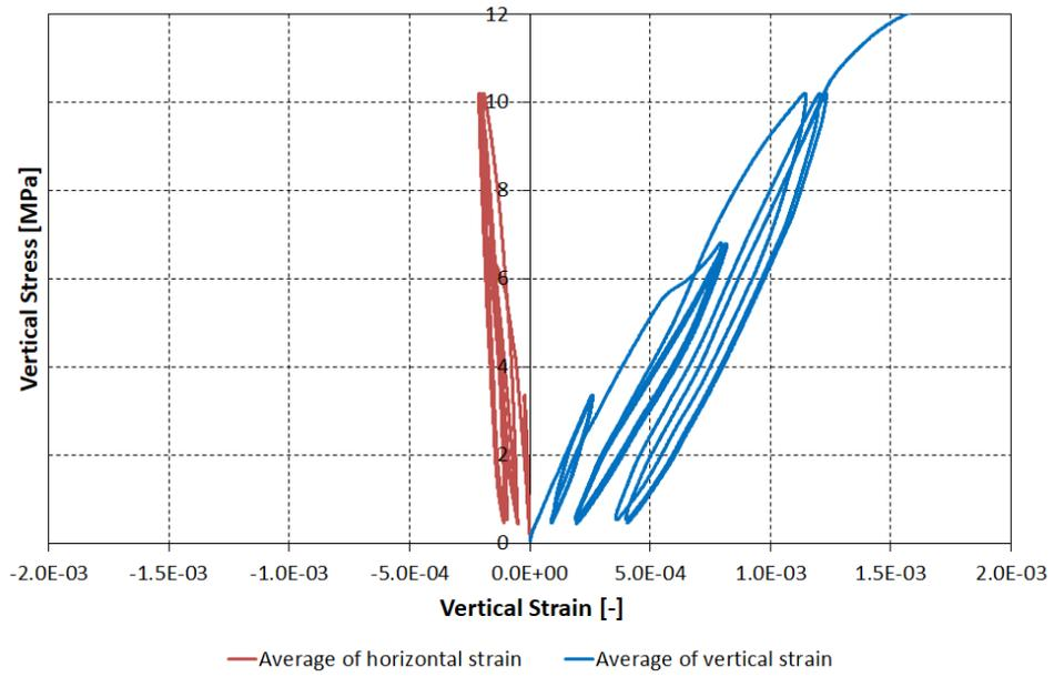
Figure 8.85 Vertical stress vs. vertical and horizontal strains for single wallette CTBSCL\_3S.
