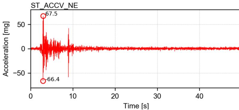
Channel ST\_ACCV\_NE – Vertical acceleration of the North-East LNEC 3D shake table platform
