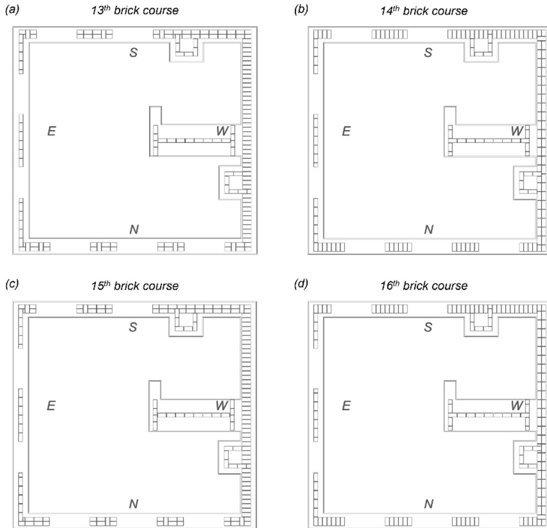
Figure 2.7 Successive courses of bricks in the Dutch cross bond: (a) 13<sup>th</sup>; (b) 14<sup>th</sup>; (c) 15<sup>th</sup>; (d) 16<sup>th</sup> brick layers (above the level of the windows apron).
