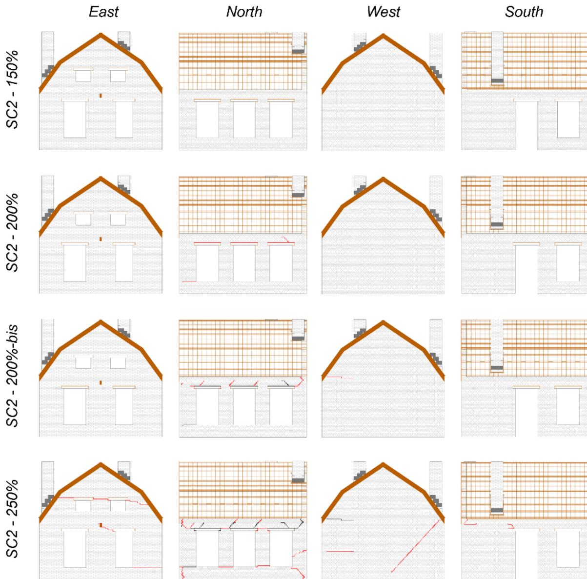
Figure 6.12 Evolution of the specimen crack pattern: tests SC2-150% to SC2-250%. Cracks marked in red were observed at the end of the annotated test run. Cracks marked in black were already detected in previous test runs.
