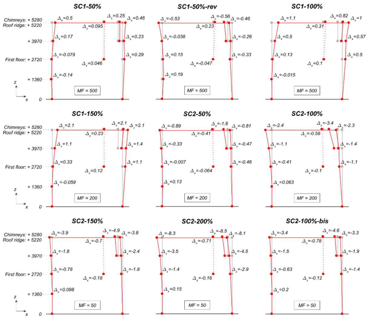
Figure 6.36 Displacement profiles at midspan of the transverse walls, at the instants of maximum roof ridge displacements: test runs SC1-50% to SC2-100%-bis. MF is the displacement magnification factor on the figure. Units of mm.
