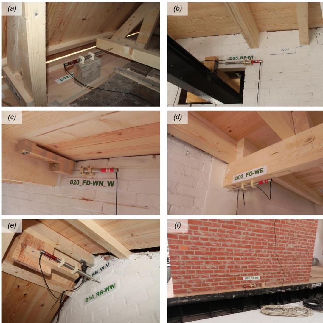
Figure 3.4 LVDTs monitoring differential displacements between (a) reference frame-floor diaphragm; (b) reference frame-interior wall; (c) longitudinal walls-floor diaphragm (i.e. lower plates); (d) floor girder-East wall; (e) gable wall-ridge beam; (f) foundation beam-South squat pier.
