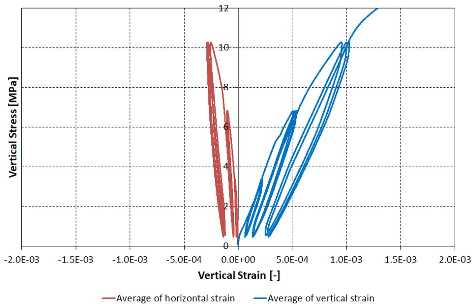
Figure 8.88 Vertical stress vs. vertical and horizontal strains for single wallette CTBSCL\_6S.
