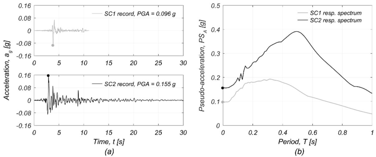
Figure 4.1 SC1 and SC2 signals: (a) acceleration histories; (b) elastic pseudo-acceleration response spectra for 5% viscous damping ratio.
