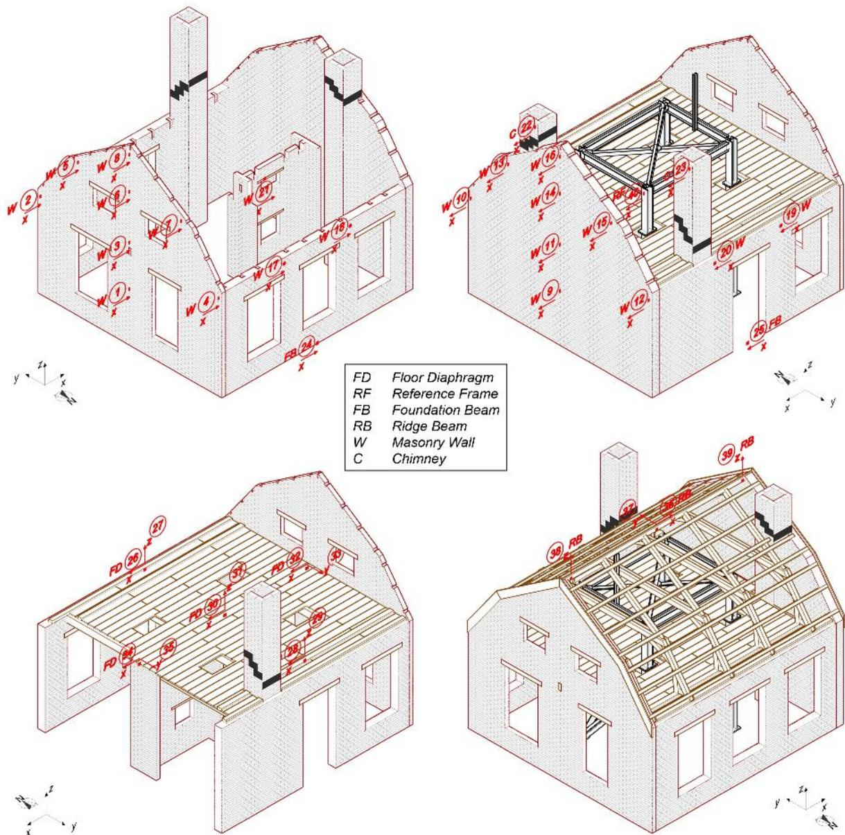
Figure 3.1 Instrumentation plan: 1D accelerometers. Letters indicate the component on which each instrument is mounted.
