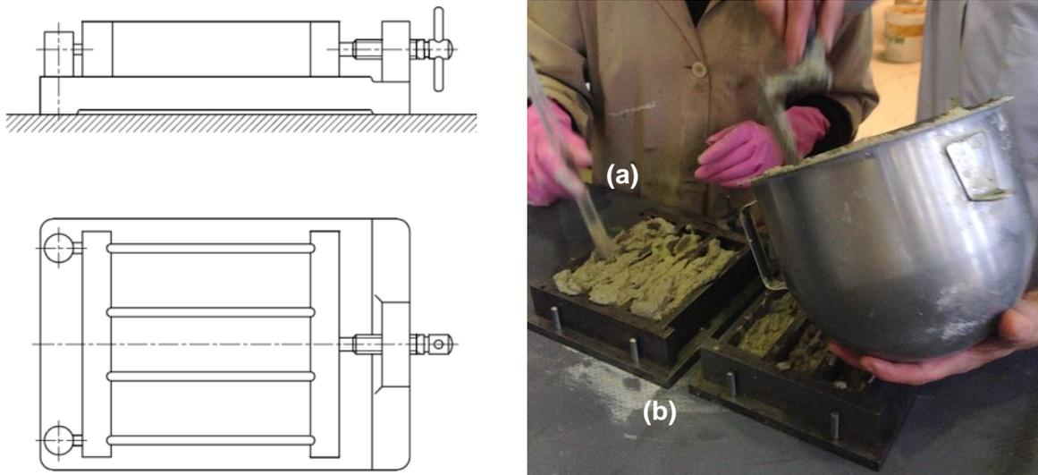
Figure 8.5 Moulding of mortar specimens: (a) pestle and (b) mould.
