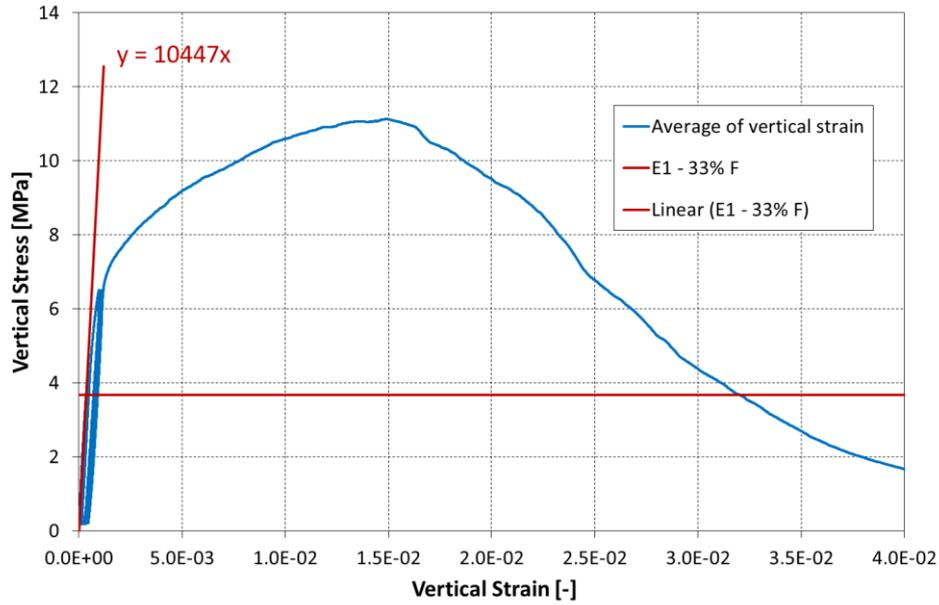
Figure 8.105 Vertical stress vs. vertical strain and determination of the modulus of elasticity for double wallette CTBSCL\_4D.
