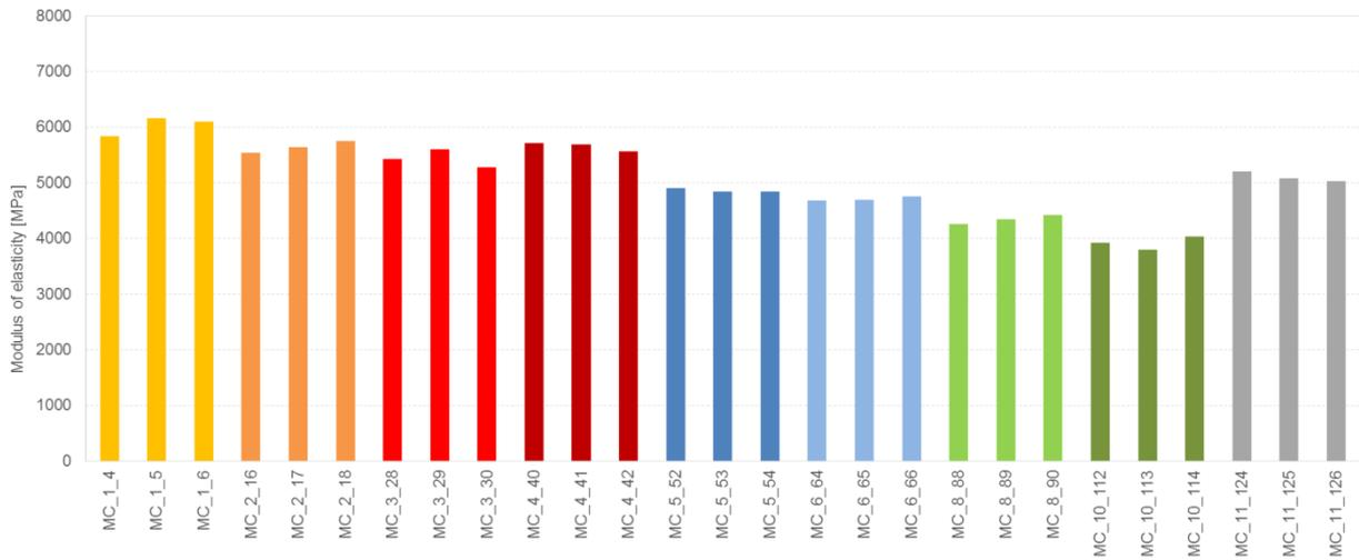
Figure 8.34 Test results for the determination of the dynamic modulus of elasticity for the mortars collected directly from the building prototype after 20 days of age.
