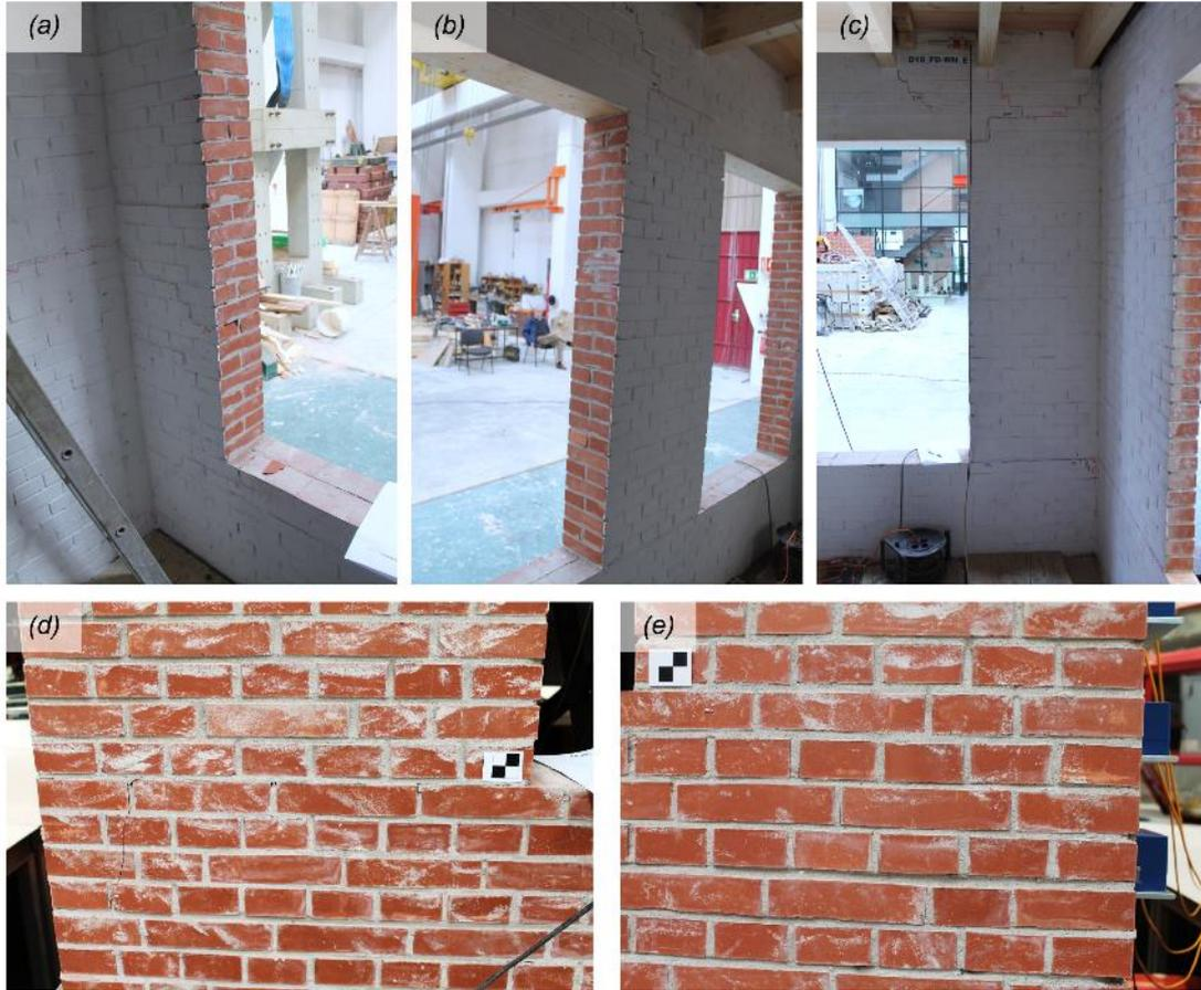
Figure 6.17 Damage on the North façade after test SC2-250%: (a, b, c) hairline flexural cracks at the top and bottom ends of all piers; (d, e) cracks at the base of the corner piers.
