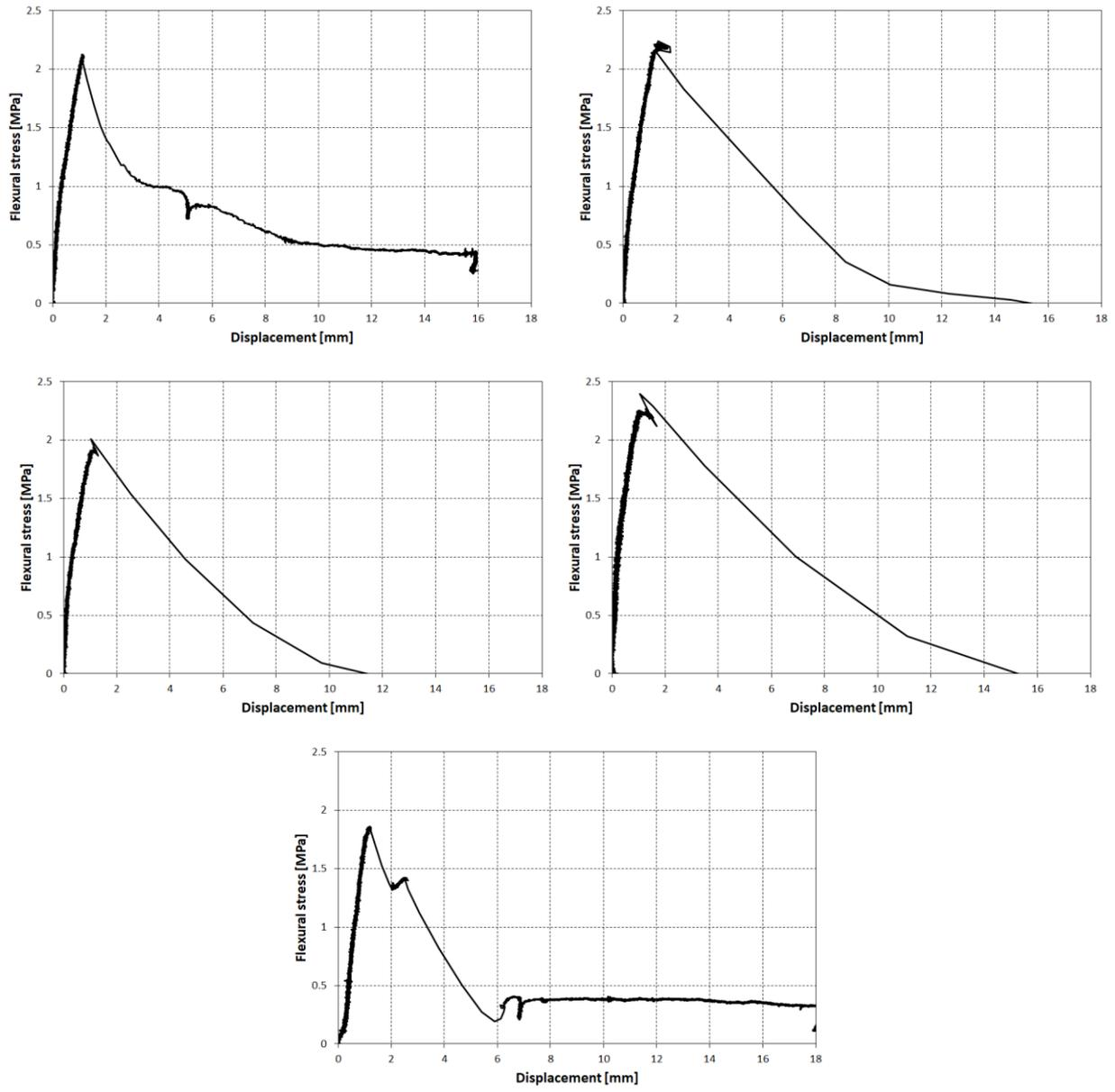
Figure 8.135 Four-point out-of-plane bending test response curves.
