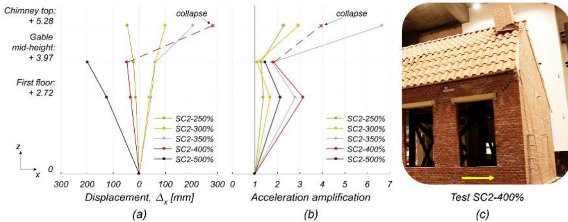
Figure 6.45 Dynamic response of the West chimney: (a) deflected shape at the instant of peak displacement at the top; (b) acceleration amplification profile; (c) snapshot at the instant of collapse for shaking at SC2-400%.
