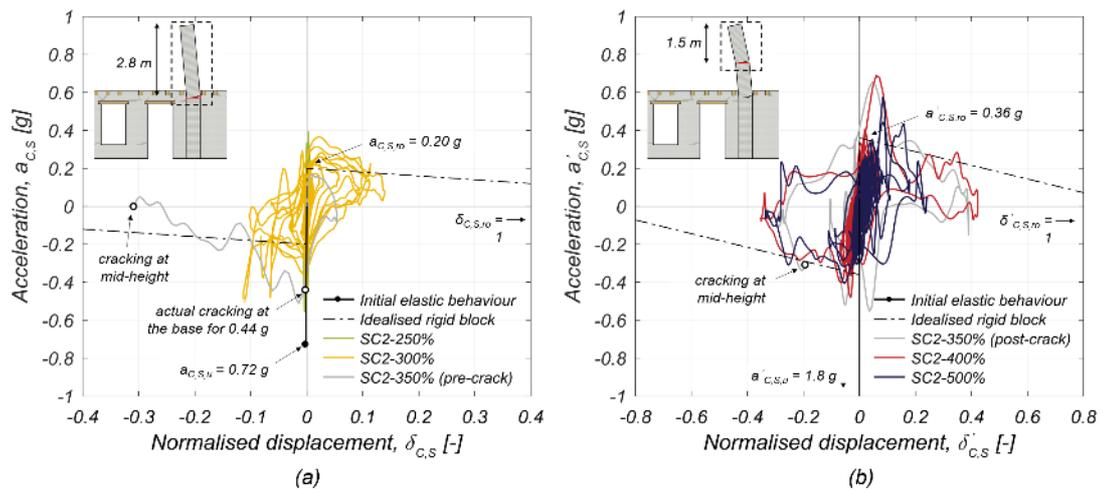
Figure 6.47 Hysteretic response of the South building chimney: (a) rocking over the entire height of the chimney stack; (b) rocking of the upper portion of the chimney after the fracture above the roofline.
