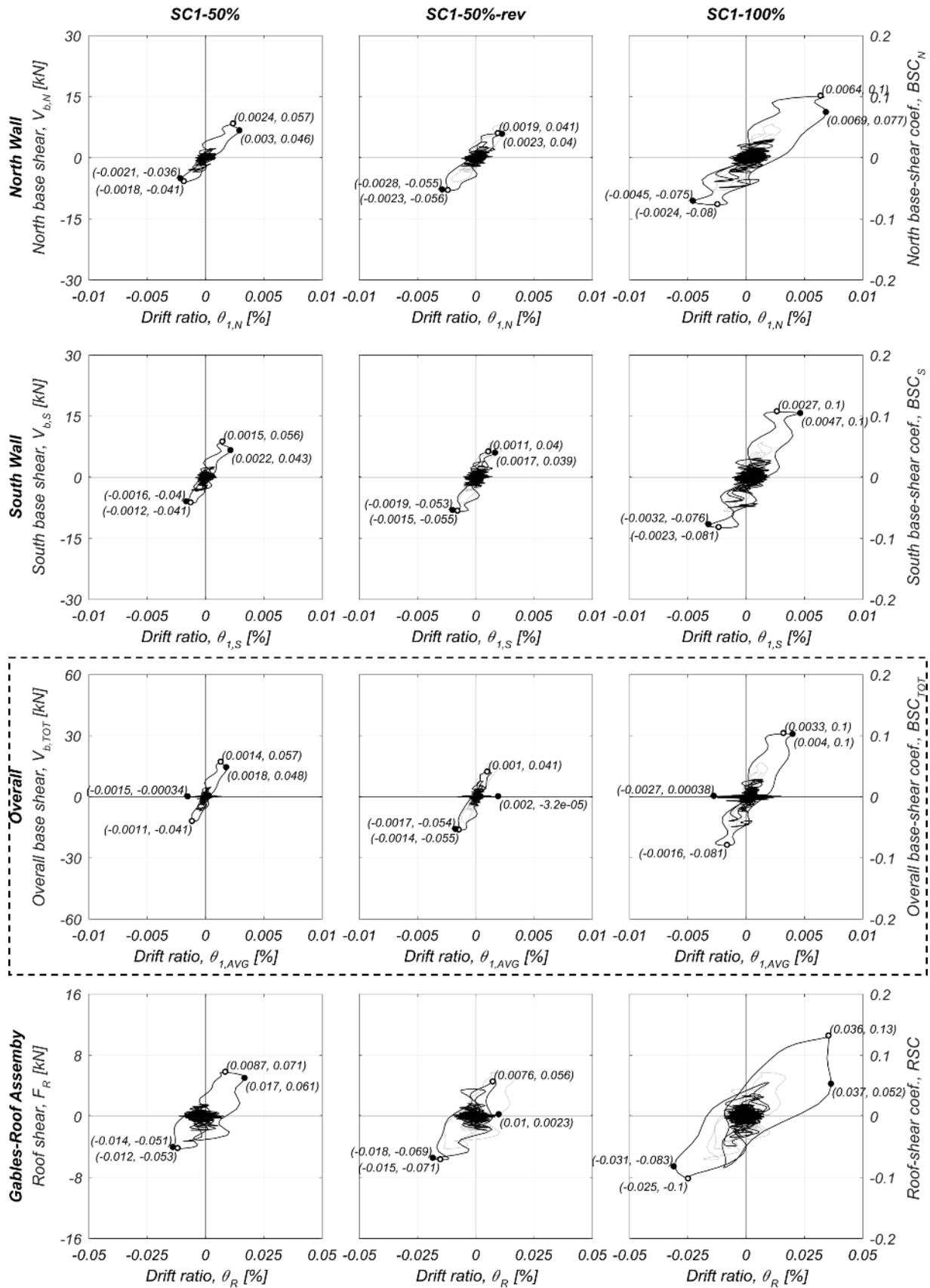
Figure 6.38 Specimen hysteretic responses: test runs SC1-50%, SC1-50%-rev and SC1-100%.
