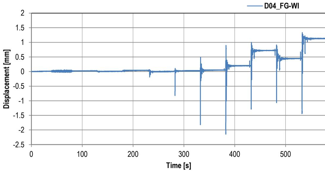
Channel D04\_FG-WI – Relative displacement
