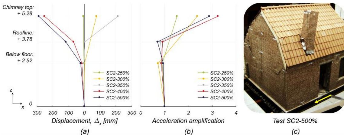
Figure 6.46 Dynamic response of the South chimney: (a) deflected shape at the instant of peak displacement at the top; (b) acceleration amplification profile; (c) snapshot at the instant of peak top displacement during test SC2-500%.
