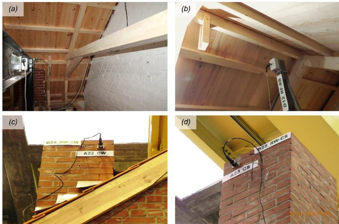
Figure 3.5 Wire potentiometers recording displacements at (a) the mid-height of the West gable wall (w.r.t. the reference frame); (b) the roof ridge beam (w.r.t. the reference frame); (c) the top of the West chimney (w.r.t. the reaction wall); (d) the top of the South chimney (w.r.t. the reaction wall).
