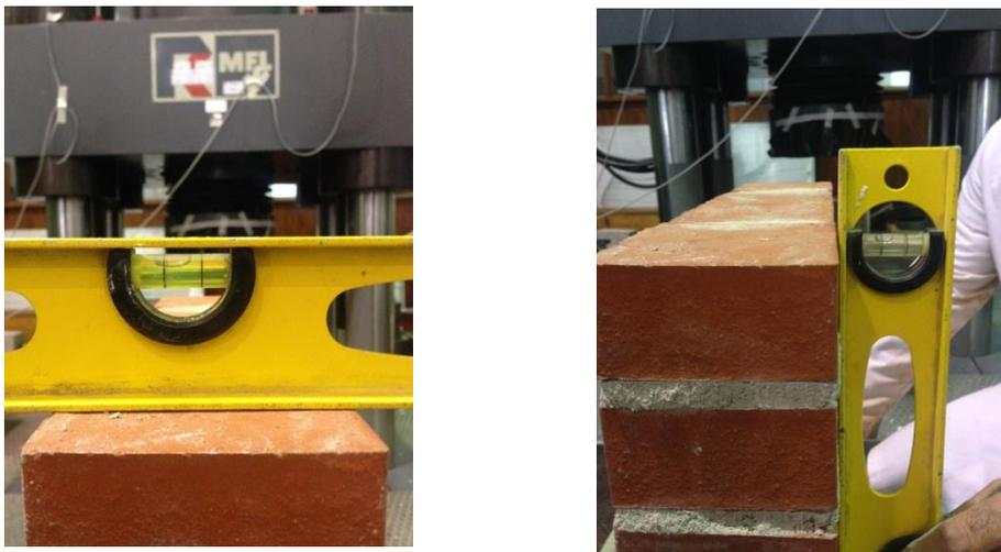
Figure 8.73 *Wallettes* with lack of orthogonality between them.
