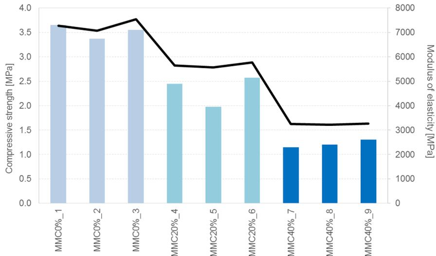
Figure 8.22 Compressive strength and modulus of elasticity test results for maturation curve (MMC\_0%, MMC\_20% and MMC\_40%) after 10 days of age.
