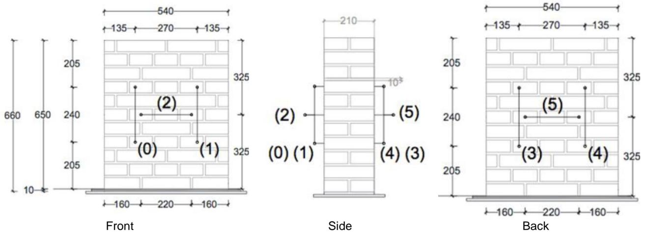
Figure 8.76 Scheme and numbering of the transducers placed on each face of the double wallettes.
