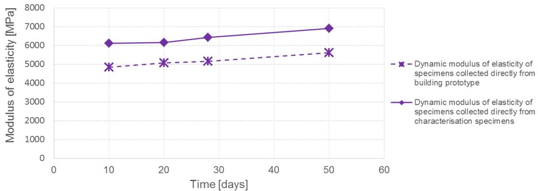
Figure 8.42 Relation between dynamic modulus of elasticity and maturation time for the bedding mortars removed from the building prototype and the characterisation test specimens.
