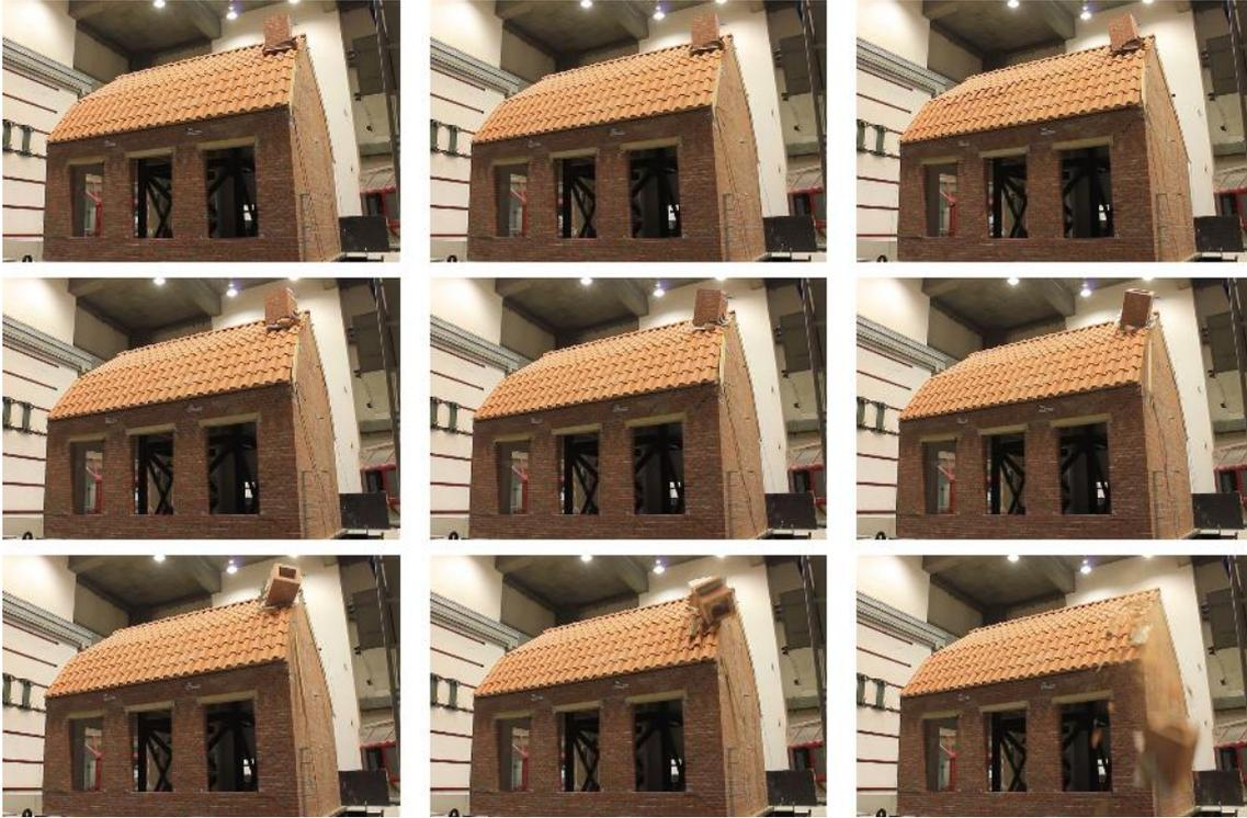
Figure 6.28 Collapse of the West chimney during testing under SC2-400%.
