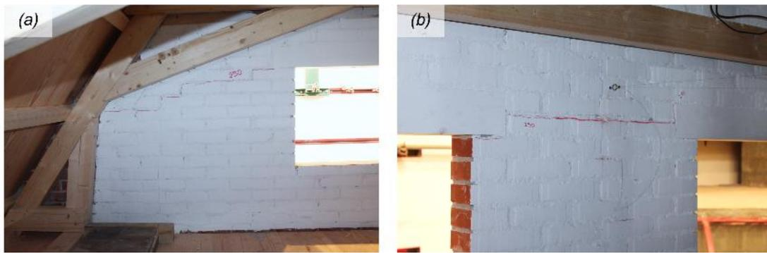
Figure 6.20 Damage on the East gable wall after test SC2-250%: (a) stair-stepped crack starting from the lintel; (b) horizontal crack between the lintels.
