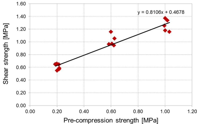
Figure 8.132 Shear strength, cohesion and internal friction angle for the solid clay triplets tested.
