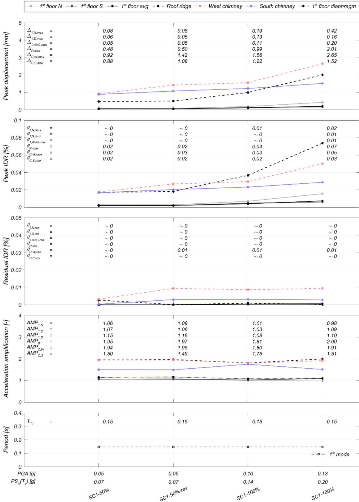
Figure 7.4 Summary of the performance of the building specimen under SC1 motions.
