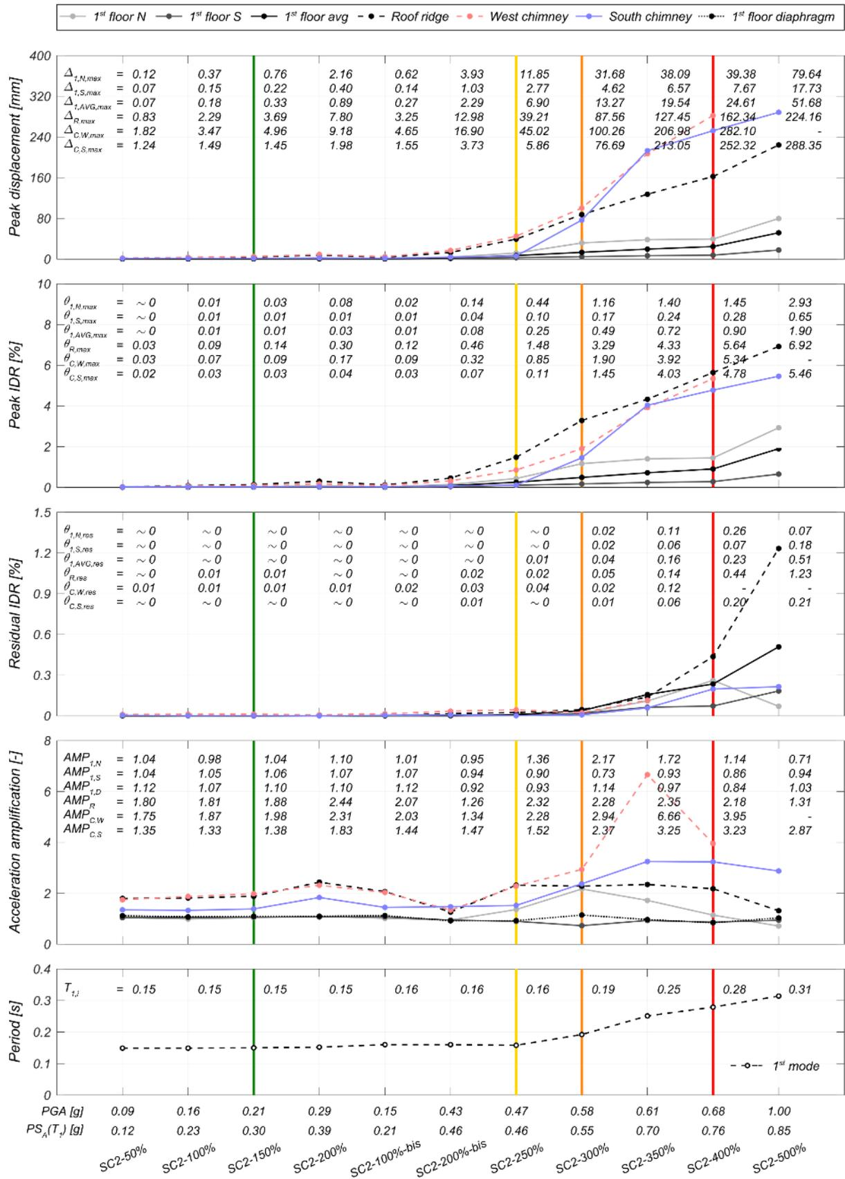
Figure 7.5 Summary of the performance of the building specimen under SC2 motions.
