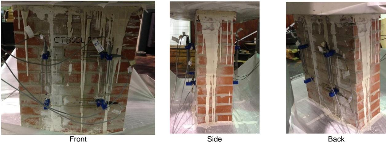
Figure 8.78 Instrumentation placed on each face of the double wallettes.
