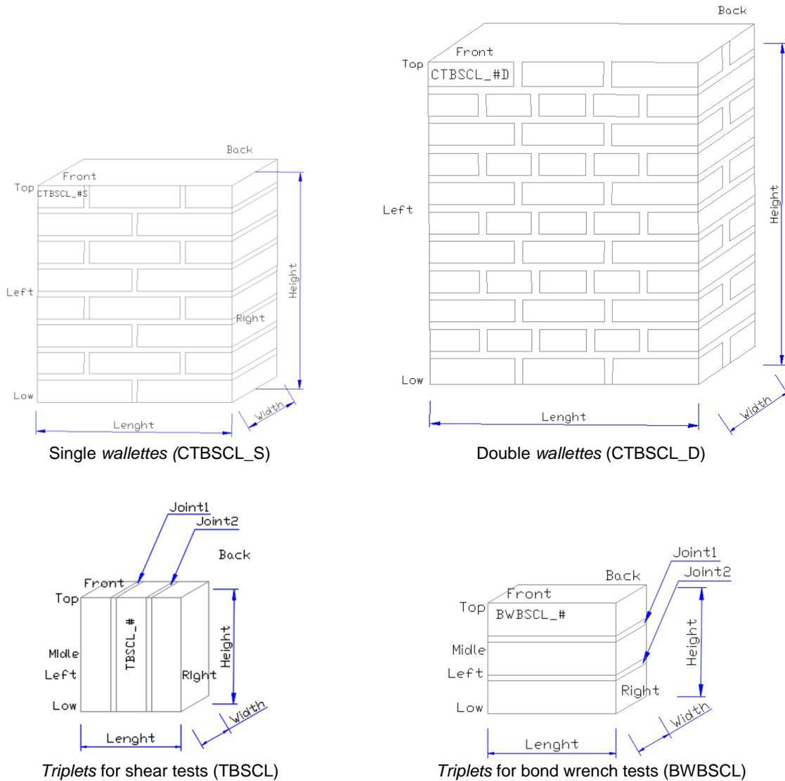
Figure 8.72 Schematic with the identification of the parameters measured in the various specimens.
