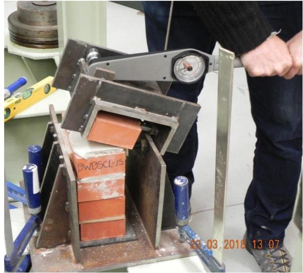
Figure 8.114 Application of vertical force until bond failure.
