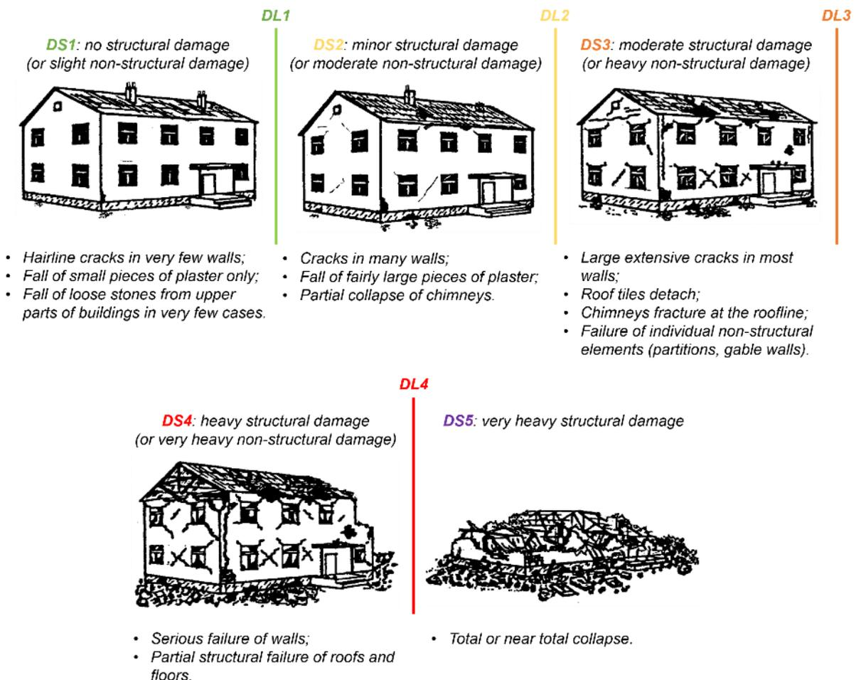
Figure 7.1 Classification of damage to masonry buildings (adapted from Grünthal, 1998).
