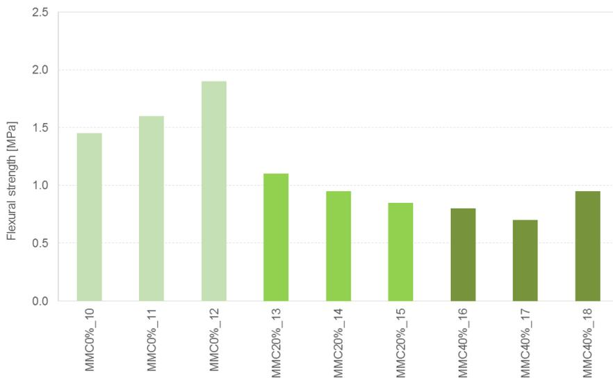
Figure 8.19 Flexural strength test results mortar for maturation curve (MMC\_0%, MMC\_20% and MMC\_40%) after 20 days of age.
