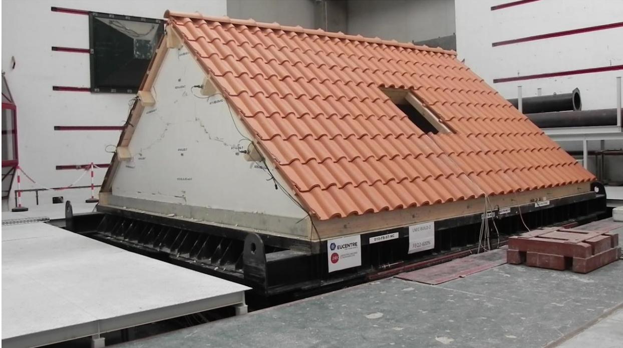
Figure 7.20 Roof structure of a terraced house building on the shaking table (Ref. 12)
