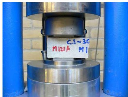
Figure 1 - Flexural test set-up.
