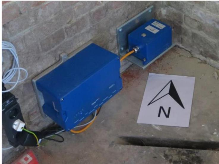
Figure 4.7 Vibration monitoring system – recorder (left) and sensor (right)
