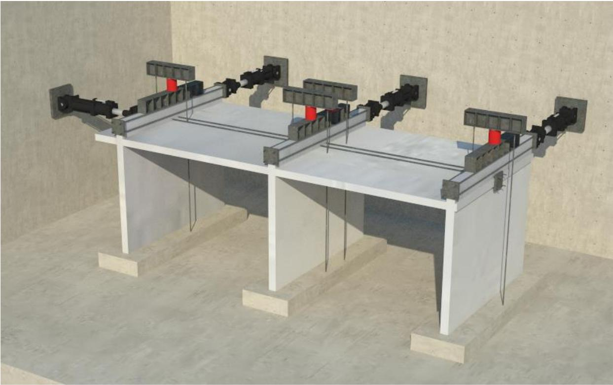
Figure 7.30 The cast-in-place concrete structure with the actuators for the dynamic push-over tests clearly visible (Ref. 15).
