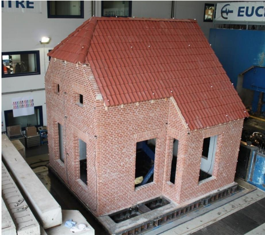
Figure 7.22 Detached house on the shake-table in the Eucentre laboratory (Ref. 7).
