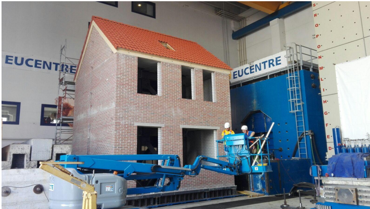
Figure 5.14 Full-scale terraced house building on the shaking table
