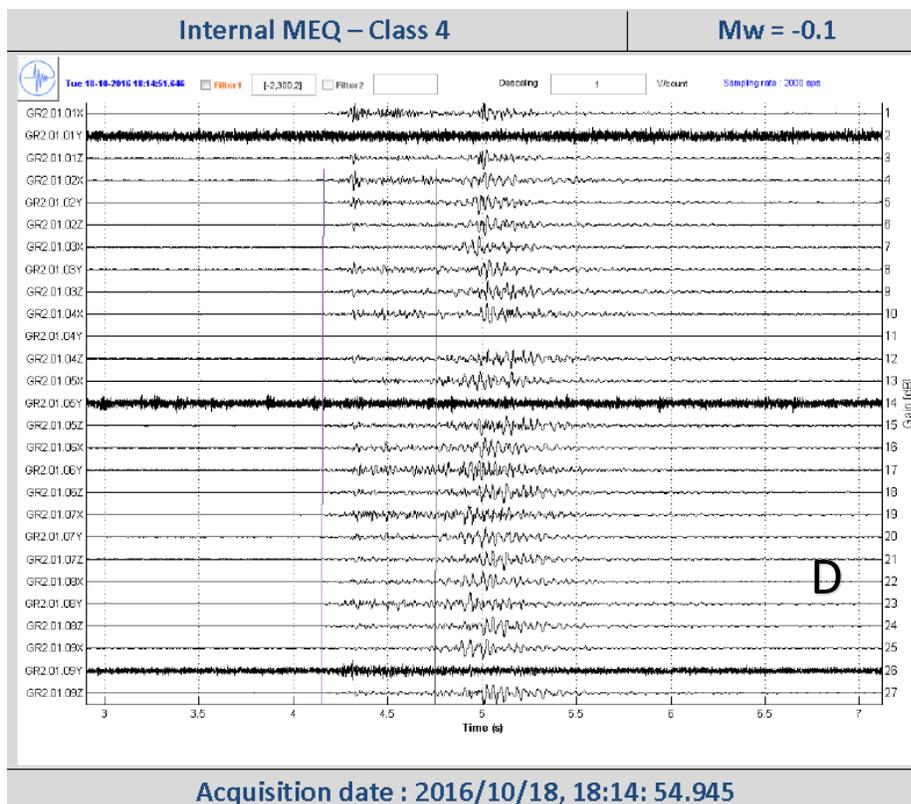
**Figure 17 (A-D).** Examples of Class 1 through 4 events shown in figures A to D, also correlated with KNMI database. Figure A shows an event that has also been detected by the KNMI surface array. Note that KNMI determines the magnitude of this event at 1.1. See discussion in section Events Correlated with KNMI Catalogue for more detail.
