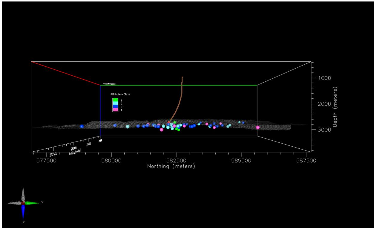
**Figure 14.** Depth view of the entire data catalog. HRS2A well shown as brown-ish line. The grey draped surface indicates the top of the Rotliegendes reservoir.
