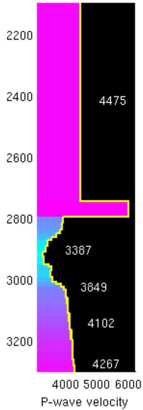
**Figure 15.** Velocity model used in the location of events. Provided by NAM on 20/23/2014.
