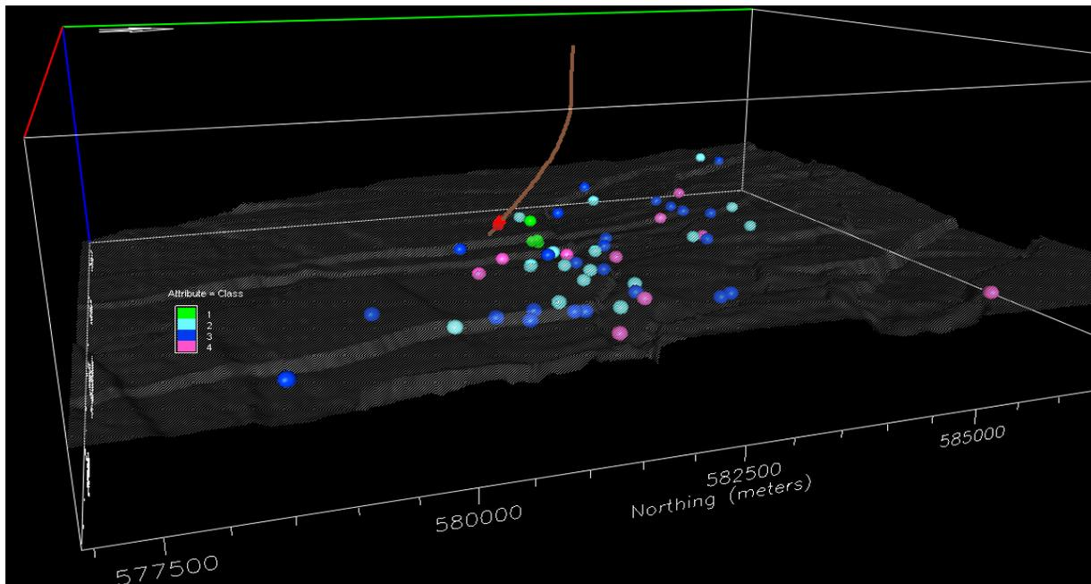
**Figure 3.** Oblique view of all the located seismicity recorded by HRS2A, displayed with respect to the top of the Rotliegend reservoir. Red symbols along the wellbore are the geophones.
