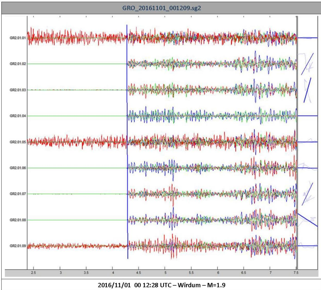
Figure 9. A screenshot showing waveforms of the M1.9 Wirdum event, one the events used in tool calibration.
