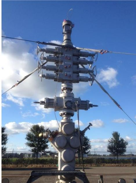
*Figure 5. HRS 2a well head (“xmas tree”)*
