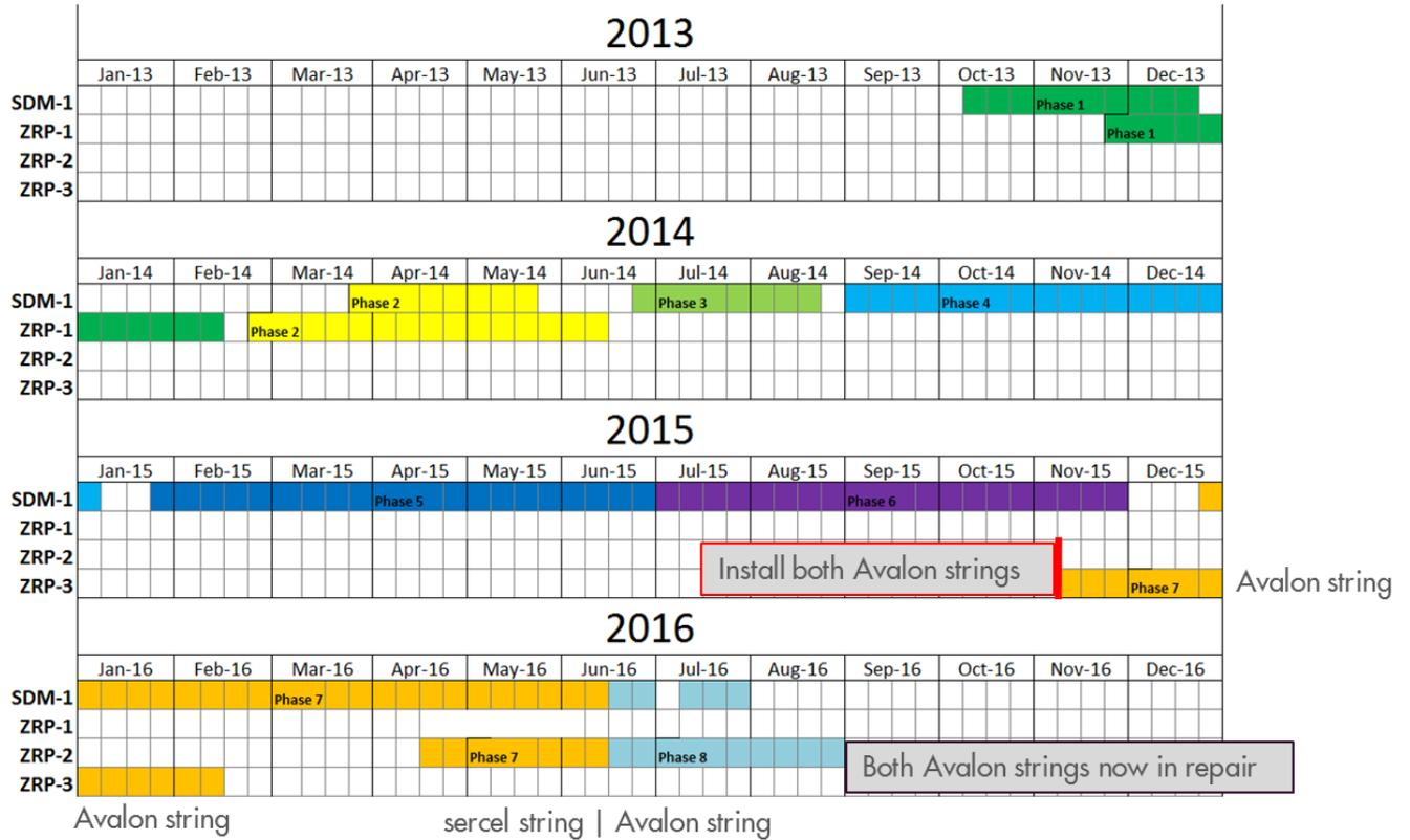
**Figure B1.** Time span of microseismic monitoring campaigns for 3 dedicated wells.
