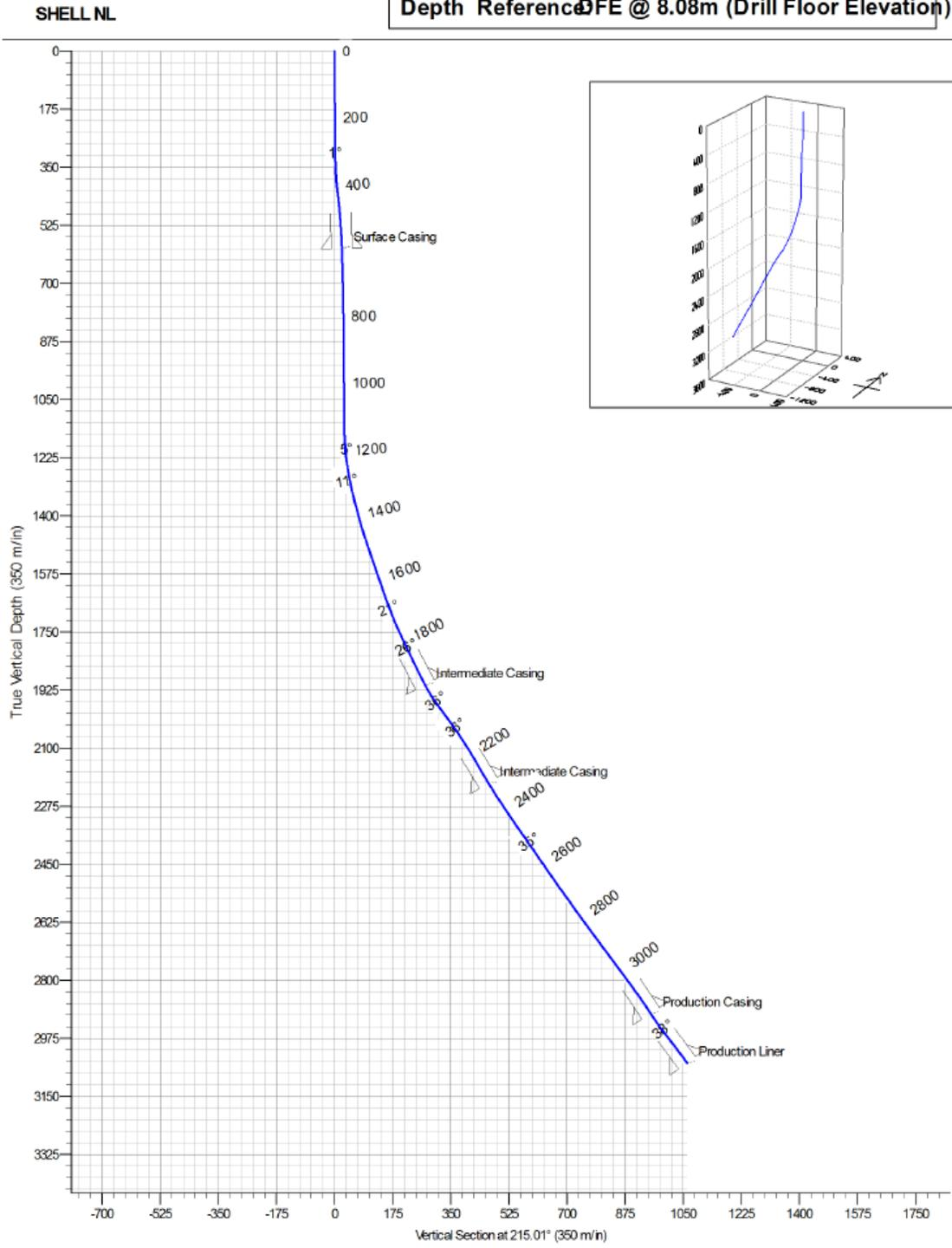
Figure 7. Schematic of the deviated well trajectory. Depth reference is DFE (Drill Floor Elevation).
