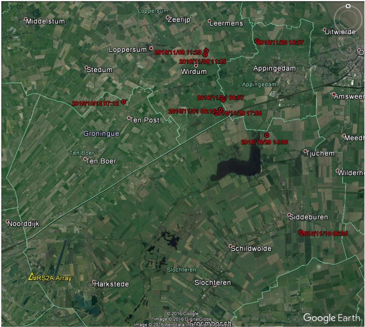
**Figure 8.** Locations of all 9 events used in the data orientation are shown in map view (red lettering) as computed by KNMI. The HRS-2A well is in the lower left hand corner shown as a yellow triangle.
