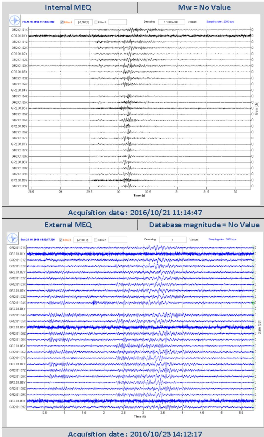
**Figure 18.** Examples of an internal and external event waveforms. Upper figure shows a recording of a typical earthquake waveform for a near-by event (deemed “internal”) where S-P time difference is less than 1 second. The lower graph shows an earthquake that occurred further away or “externally” with S-P time over 1 second.
