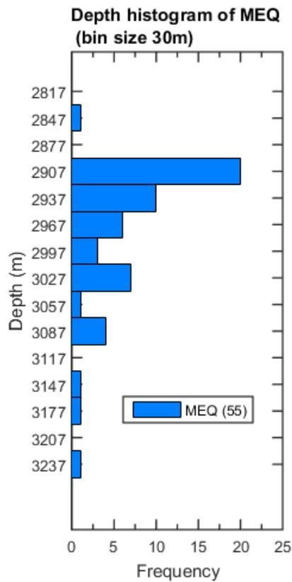
**Figure 13.** Histogram of event frequency versus depth since the beginning of recording on October 06. 2016 shows pseudo-clustering around 2907 m.
