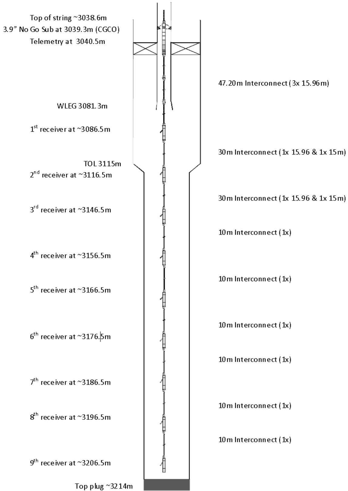
**Figure 6.** A well schematic Depths shown are measured using DFE (Drill Floor Elevation).
