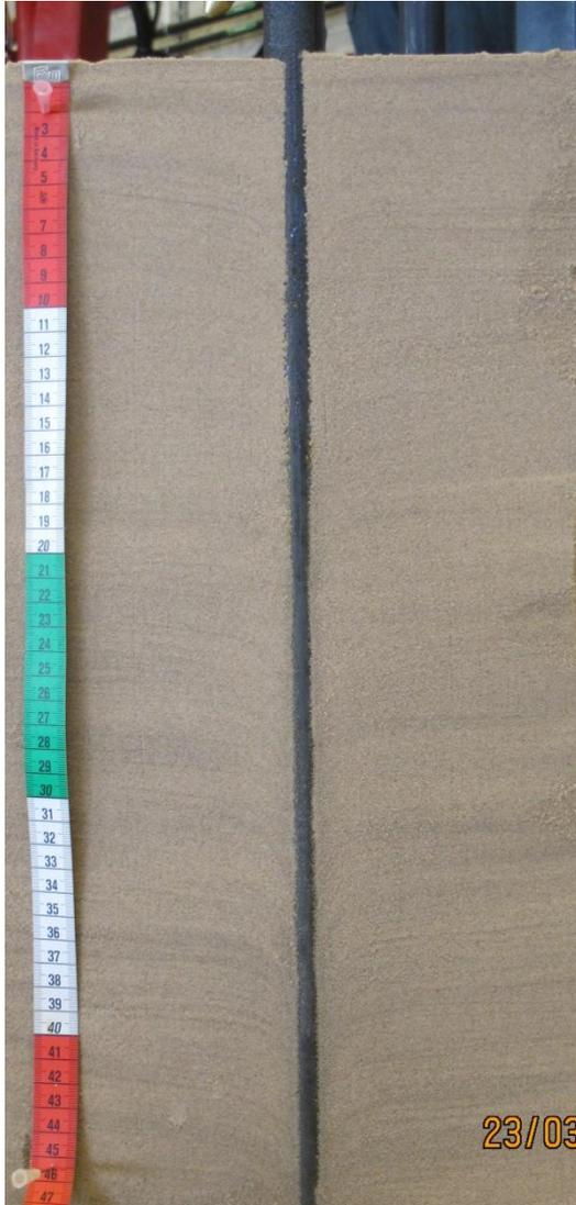
Figure C.10 Photographed cross section of soil sample 2 after testing with the cone penetrated with a surcharge load of 50 kPa
