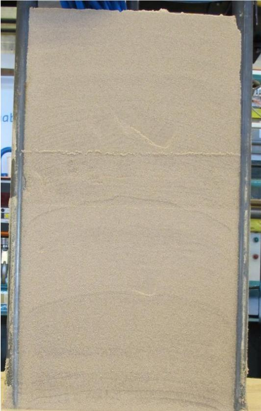
Figure C.14 Photographed cross section of soil sample 3 after CPT testing
