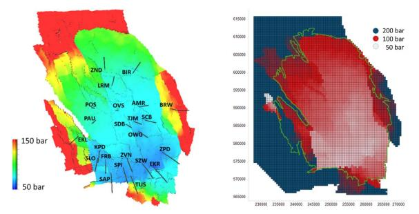
Figure 3-3:Reservoir pressure at 1/1/2018. Both figures show the same data. On the left is the output from the reservoir<br/>simulator constrained to the Groningen field, while on the right is pressure used as input to the hazard and risk<br/>assessment.
