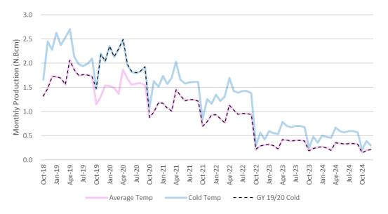
*Figure 3-20:* Groningen field production profiles for average and cold temperatures along with the profile used where a single year follows the cold temperature profile, in this case gas-year 2019-20.
