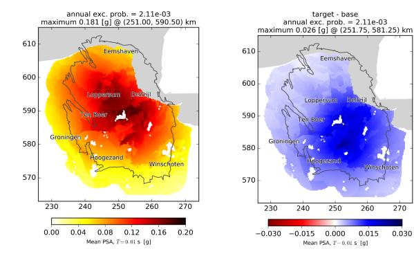
Figure 4-8a Cold-temperature scenario -- annual hazard plots (left) and difference w.r.t. corresponding average-temperature scenario hazard (right)
