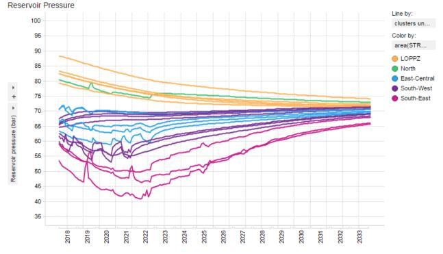
case. Again, there is only limited impact on the Loppersum region for the five-year period shown in Figure 3.14. For this production case there is a slight reduction in pressure in the Borgsweer area due to less water injected.
