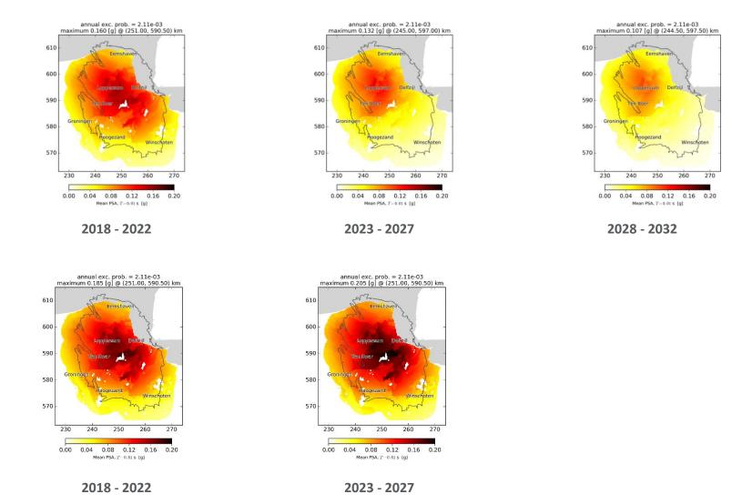
Figure 4.5 The three 5-year hazard maps for the average weather "Basispad Kabinet" scenario (top) and the two 5-year hazard maps for the average weather 24 Bcm/year scenario (bottom).
