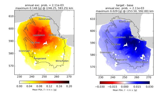
Figure 4-8b Cold-temperature scenario -- annual hazard plots (left) and difference w.r.t. corresponding average-temperature scenario hazard (right)
