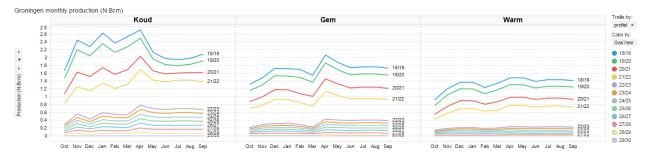
*Figure 2-3 Monthly production fluctuation by gas-year for cold (left), average (middle) and warm (right) temperatures.*
