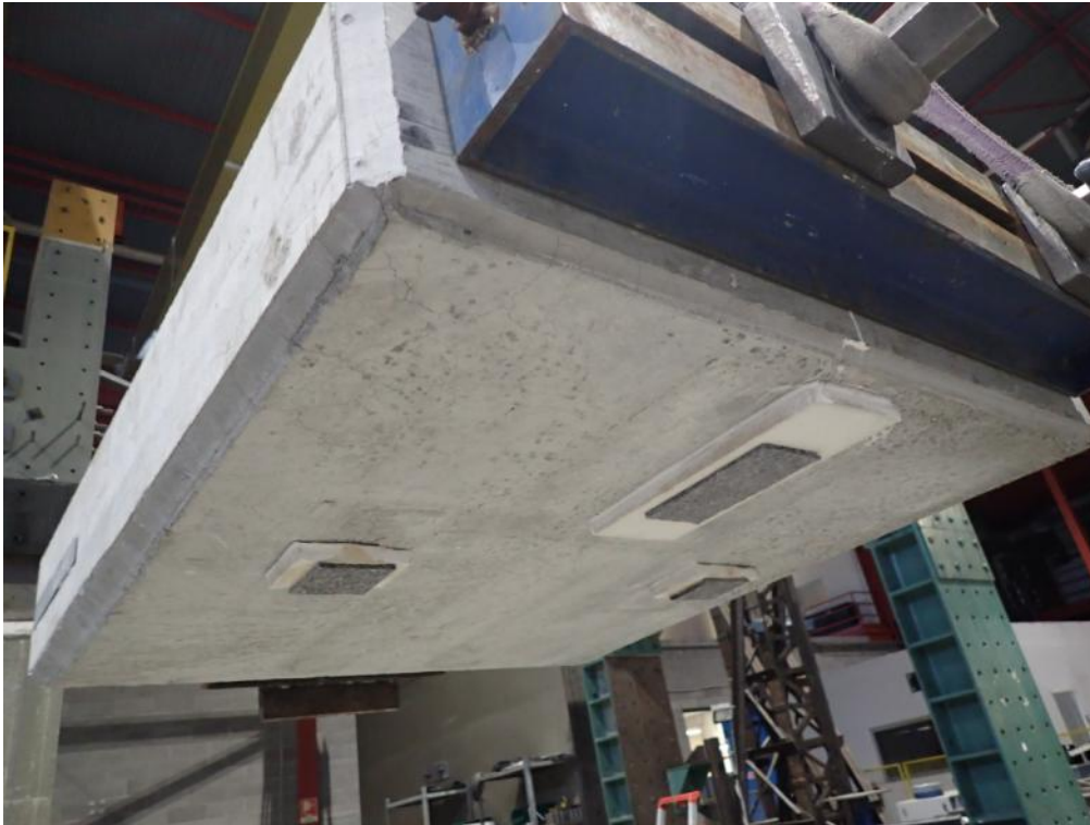
Figure C1. First cyclic friction testing attempts – Asymmetric configuration, one felt layer plus gypsum.
