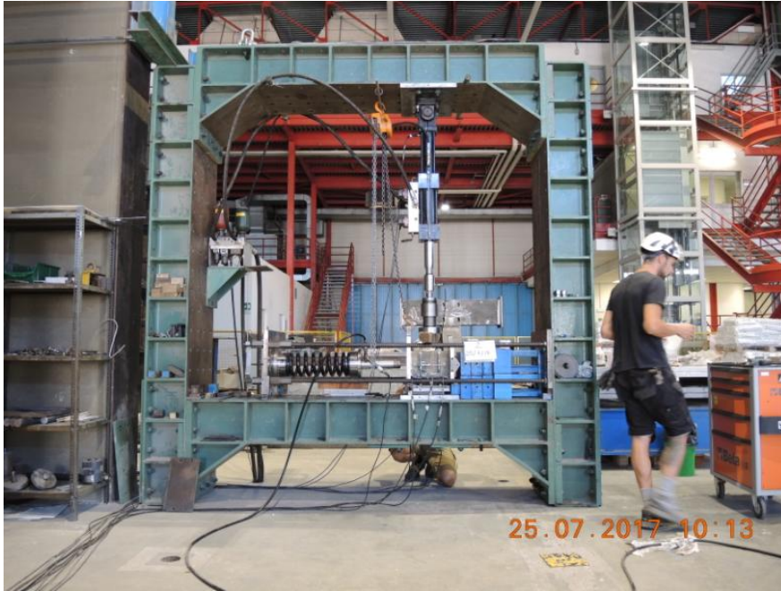
Figure 8. Experimental setup for friction testing of felt material.
