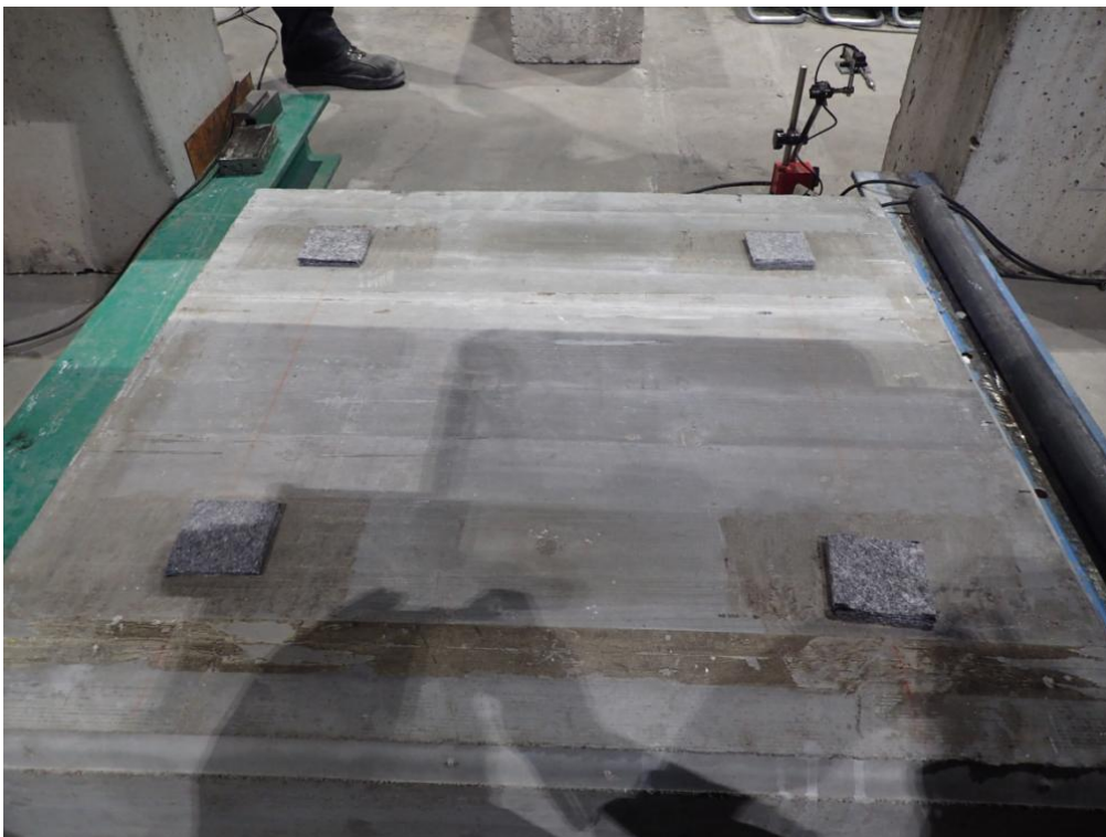
Figure 35. Position and size of the portions of felt in-between the two concrete blocks.
