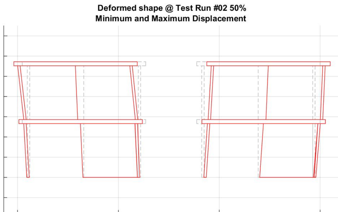
Figure 244. Deformed shape of EUC-BUILD5 specimen (max and min) – Test run #2.
