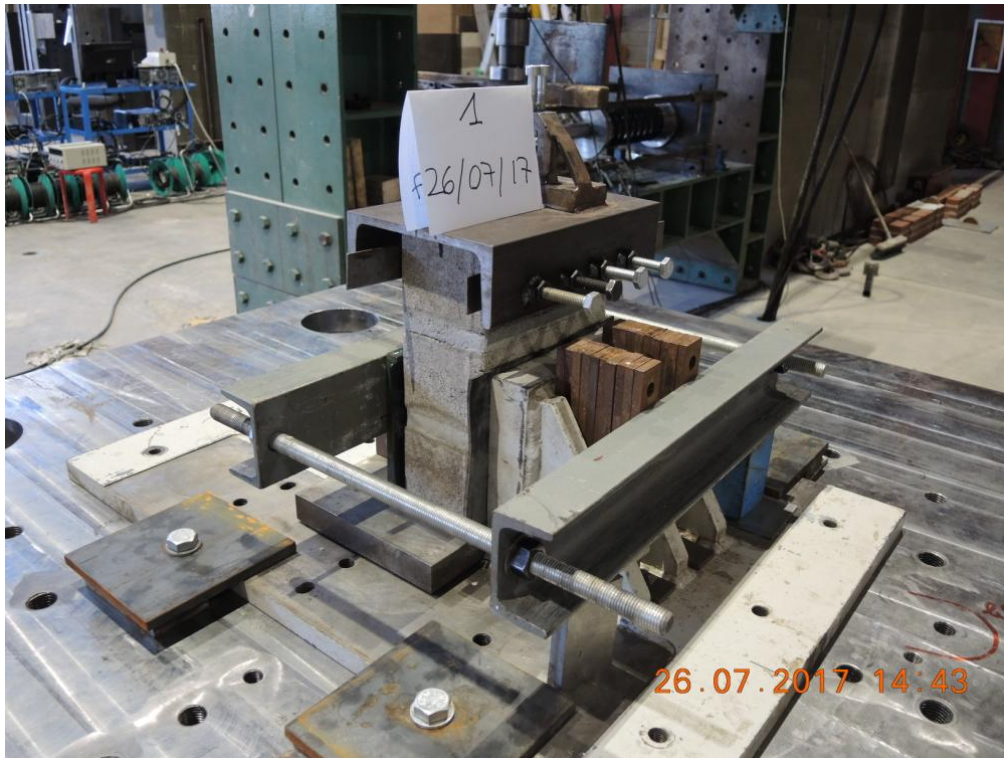
Figure 20. Bond wrench testing: Geometry and apparatus for base-campling.
