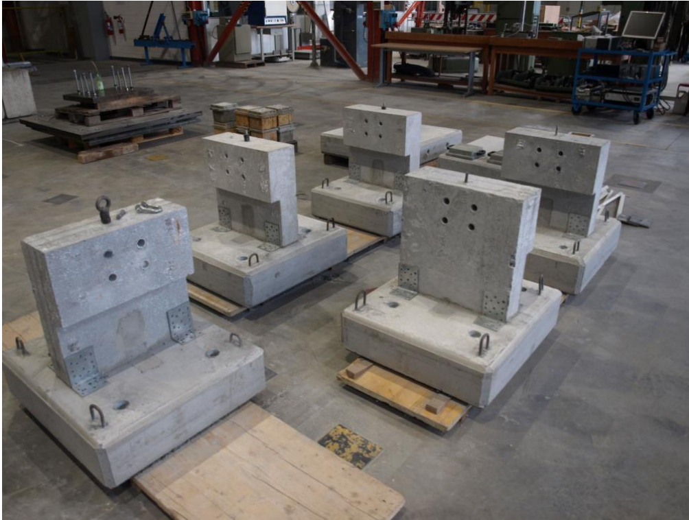
Figure 69. View of the five specimens after assembling and mortar grout.
