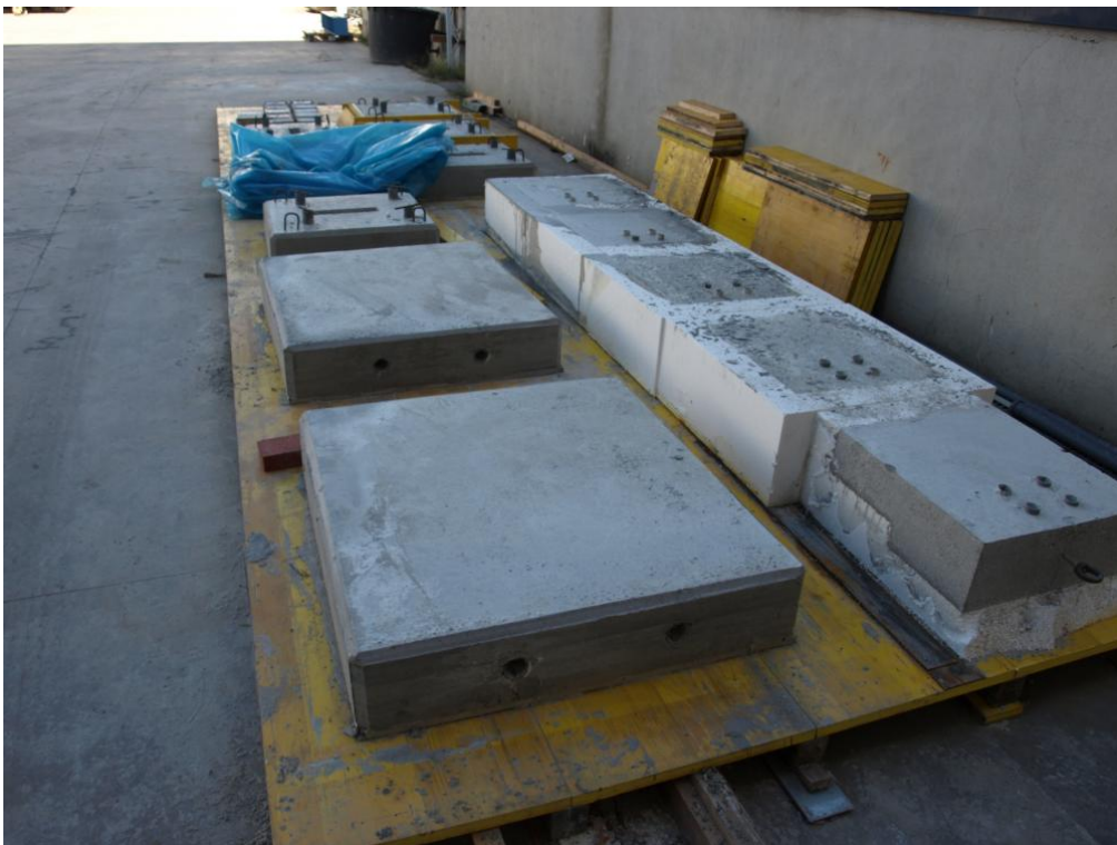
Figure 32. Concrete blocks for friction testing of felt material after removal of the formwork.
