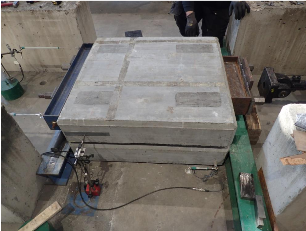
Figure 34. Experimental setup and instrumentation for cyclic testing of felt material.
