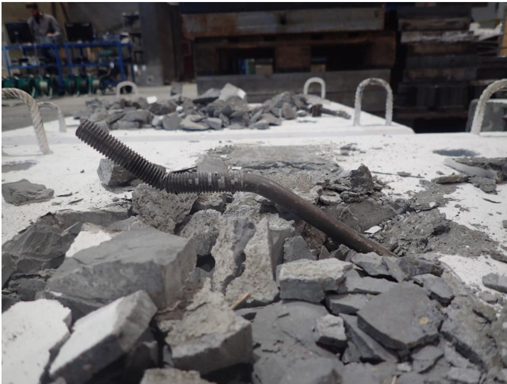
Figure 78. Flexural failure mode of the steel connector – Specimen #2.
