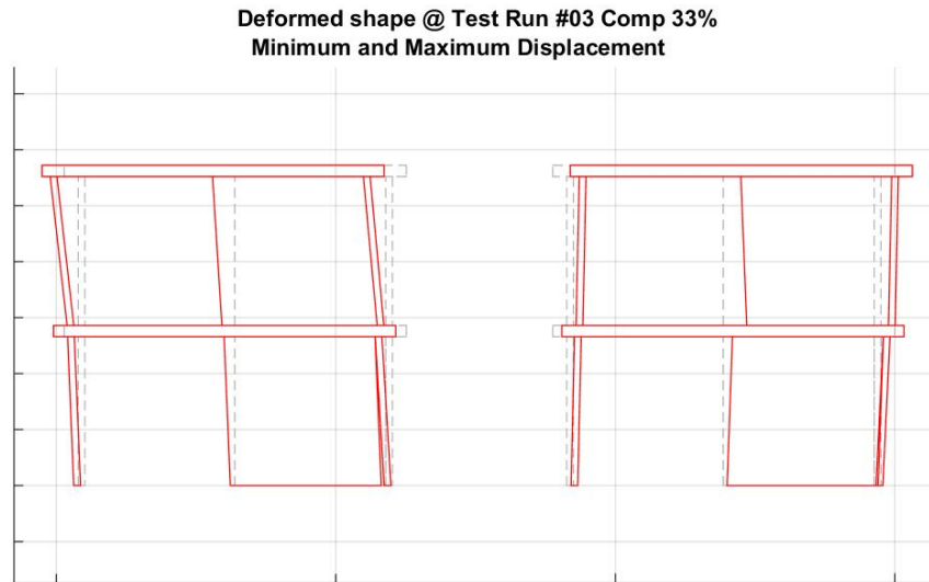
Figure A4. Deformed shape of EUC-BUILD5 specimen (max and min) – Test run #3.
