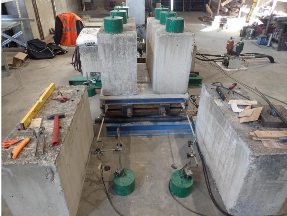
Figure 38. Vertical loading configurations – Configuration #3, high vertical pressure (0.6 MPa).
