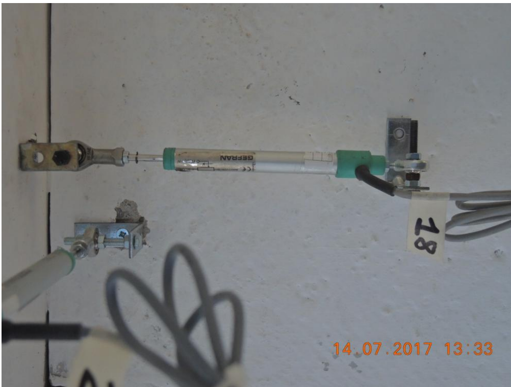
Figure 214. Potentiometers installed onto the top of the lateral walls – First storey, opposite side.
