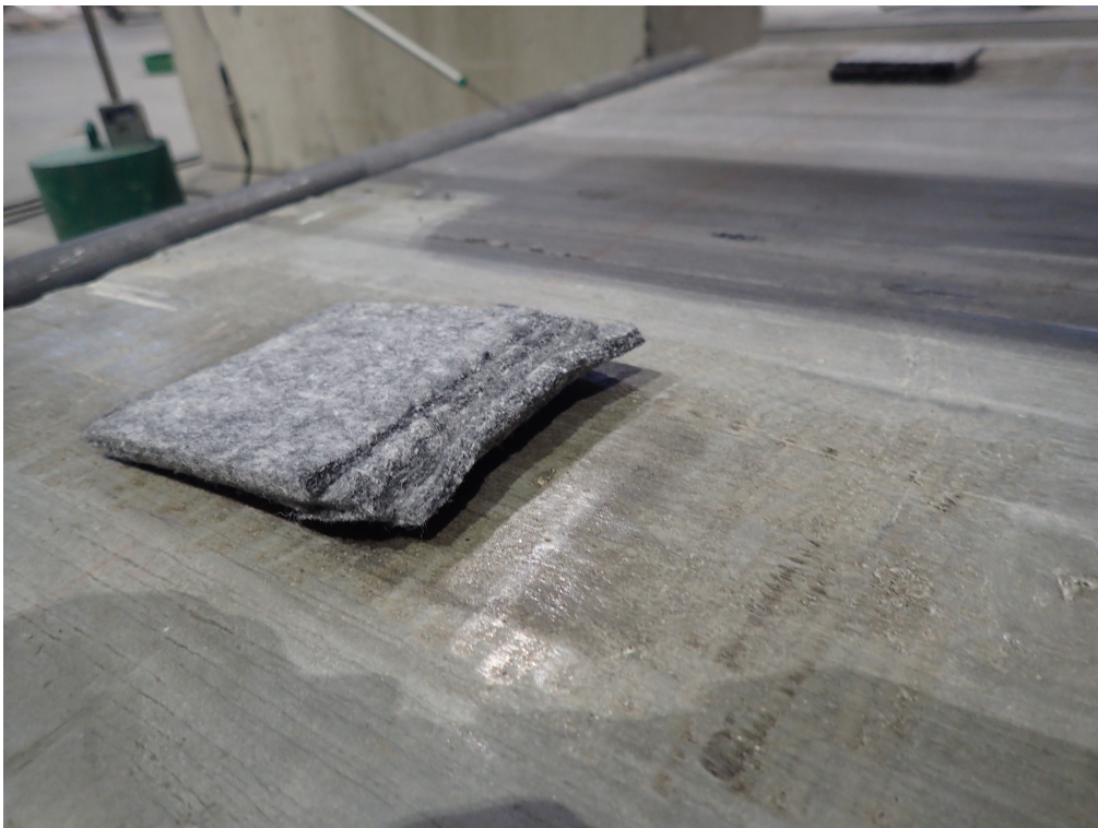
Figure C4. First cyclic friction testing attempts – Disintegrated felt stack after testing.
