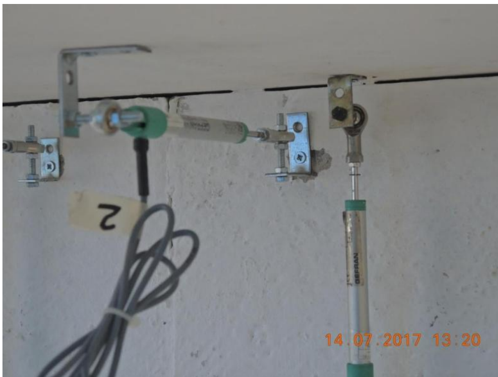
Figure 204. Potentiometer at the top of the South-East-sided lateral wall – South wall face, West corner.
