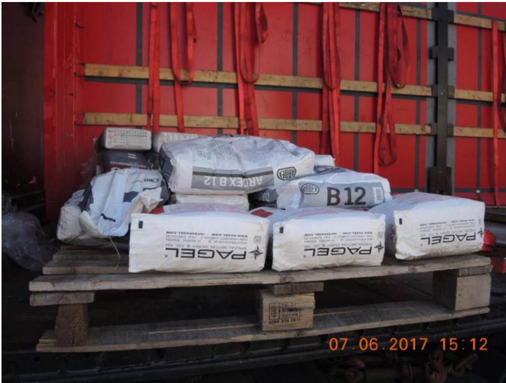
Figure 112. Delivered construction material – Mortar for finishings and structural interfaces.
