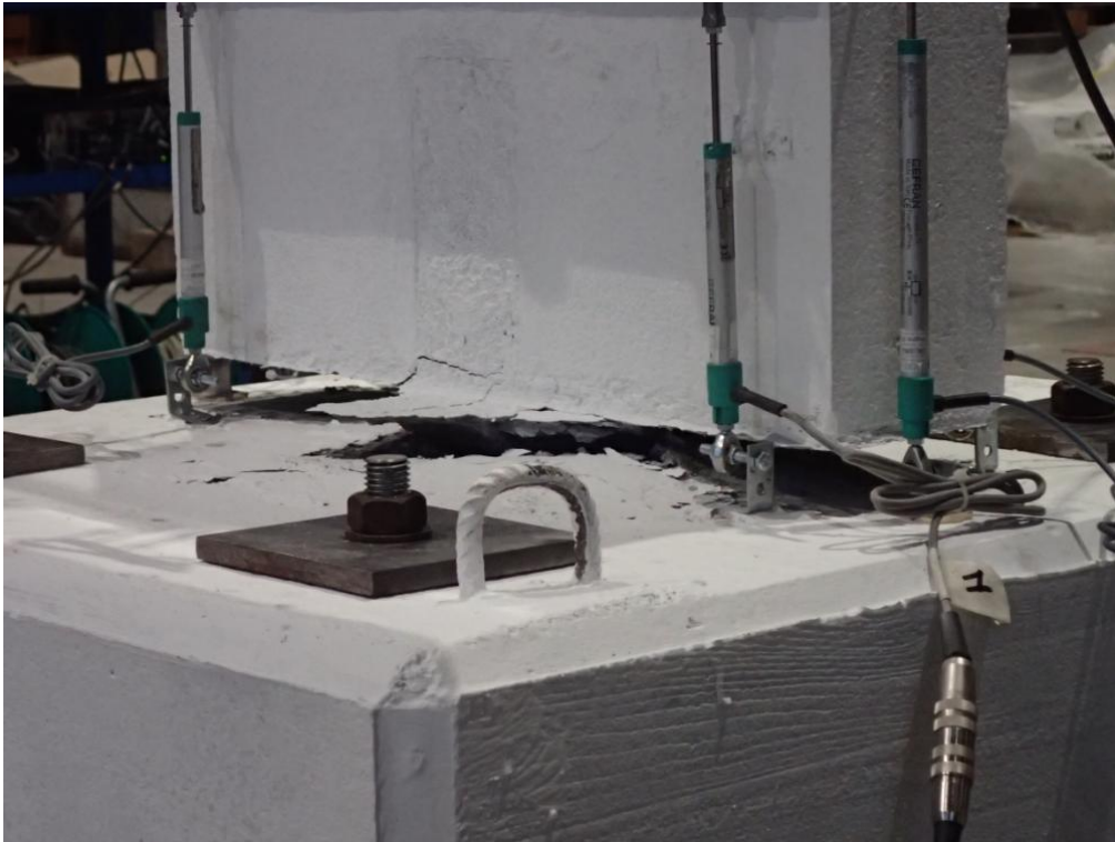
Figure 75. Damage and detachment of the two portions of the specimen.
