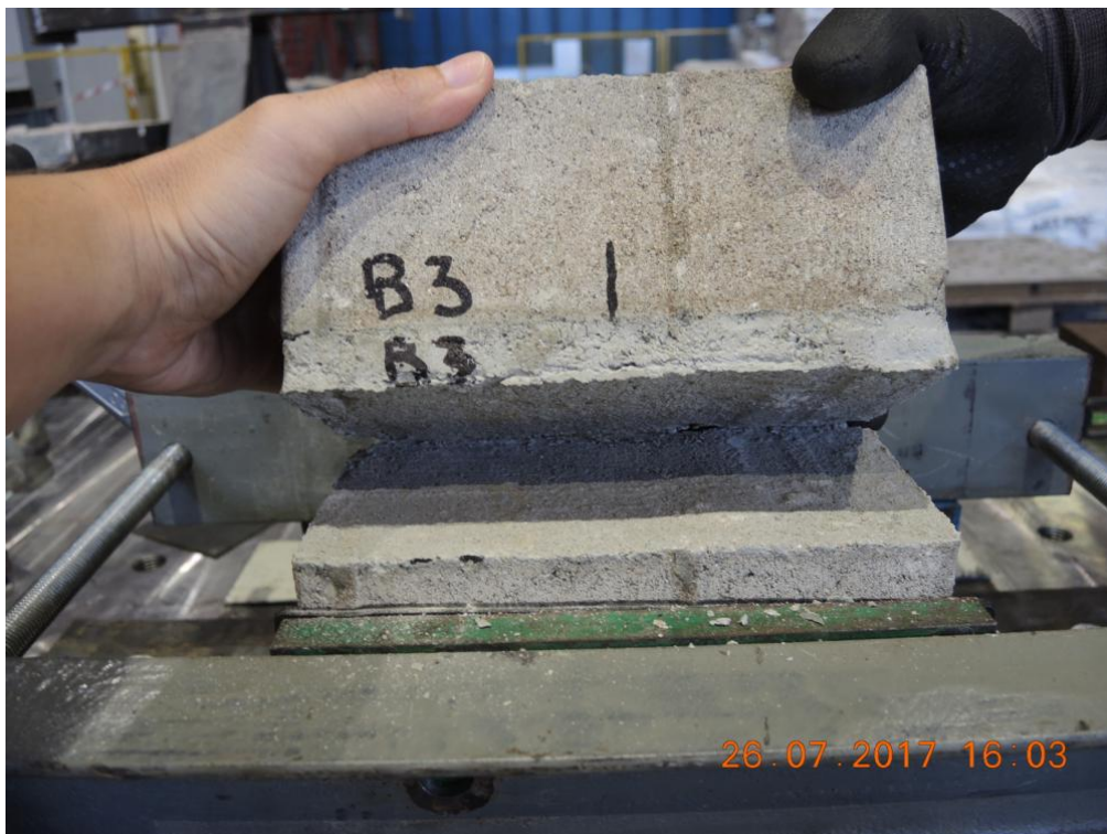
Figure 23. Bond wrench testing: third test, bed-joint #03 – Detailed view of the observed failure mode.
