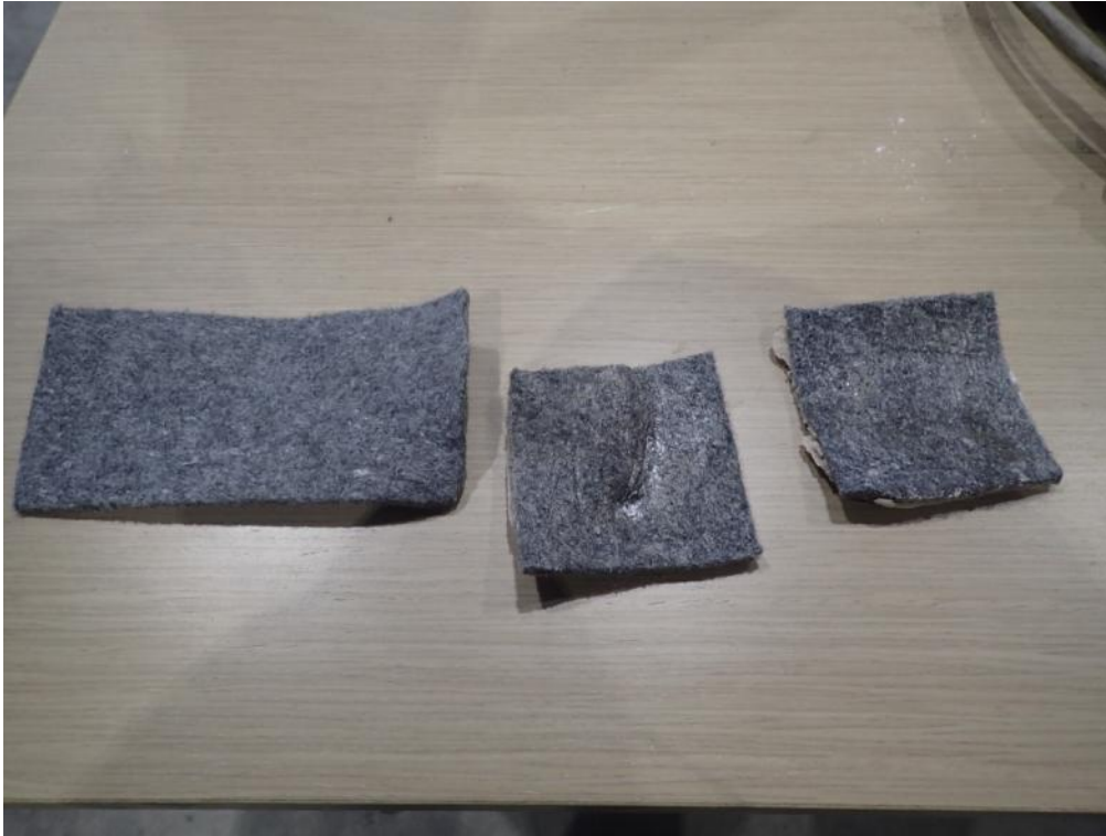
Figure C2. First cyclic friction testing attempts – Felt layers after testing.
