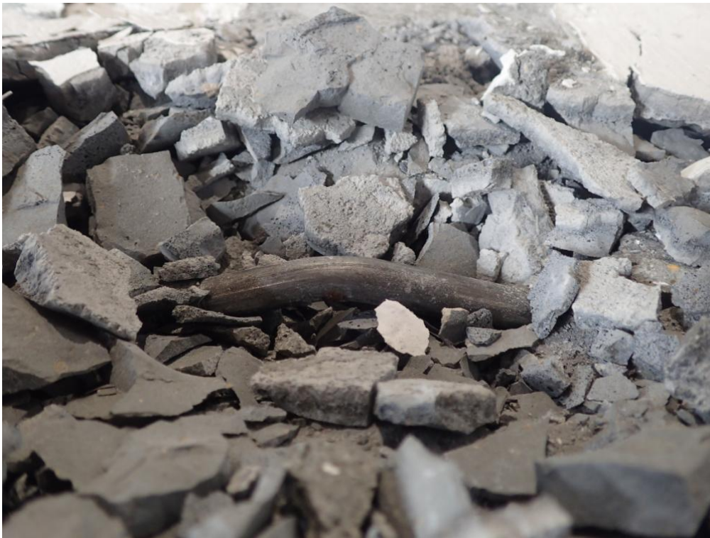
Figure 82. Bending of the steel connector embedded in the bottom connector's socket – Specimen #4.
