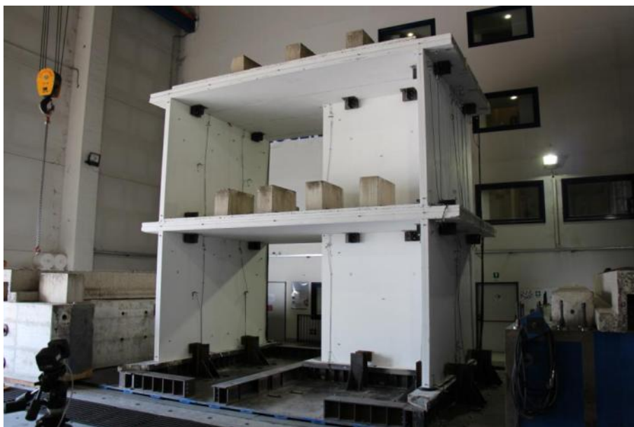
Figure 92. Photograph of EUC-BUILD5 specimen before dynamic testing.
