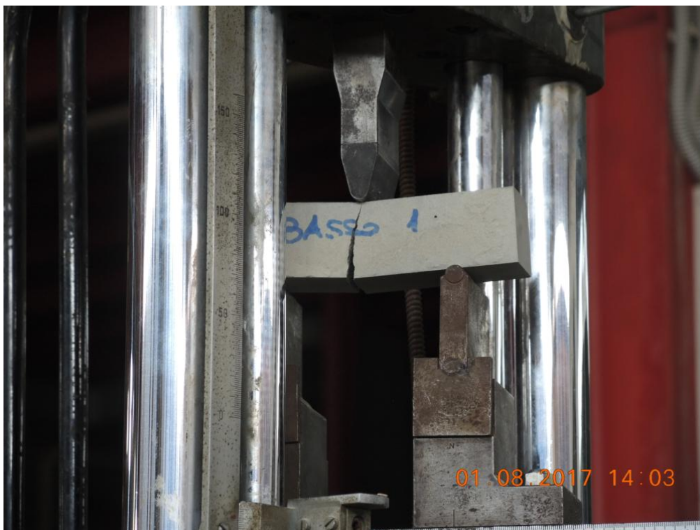
Figure 4. Three-points flexural testing for characterisation of gap-filling mortar – Failure mode of a specimen.
