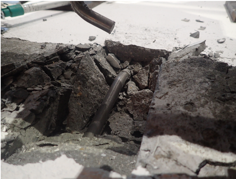
Figure 80. Deformed shape of the two steel connectors at the end of the test – Specimen #3.
