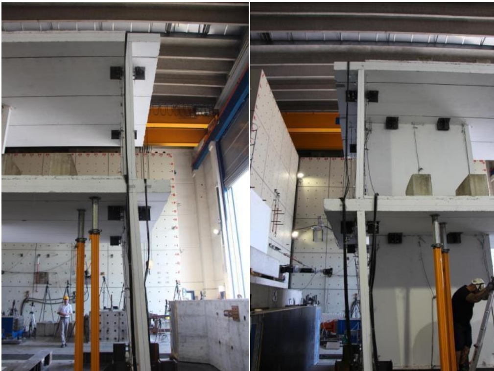
Figure 331. Propping-up at the end of the last test run – North and South sides.
