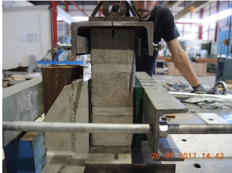
Figure 16. Example of concrete-mortar specimen for bond wrench testing – Geometrical characteristics.
