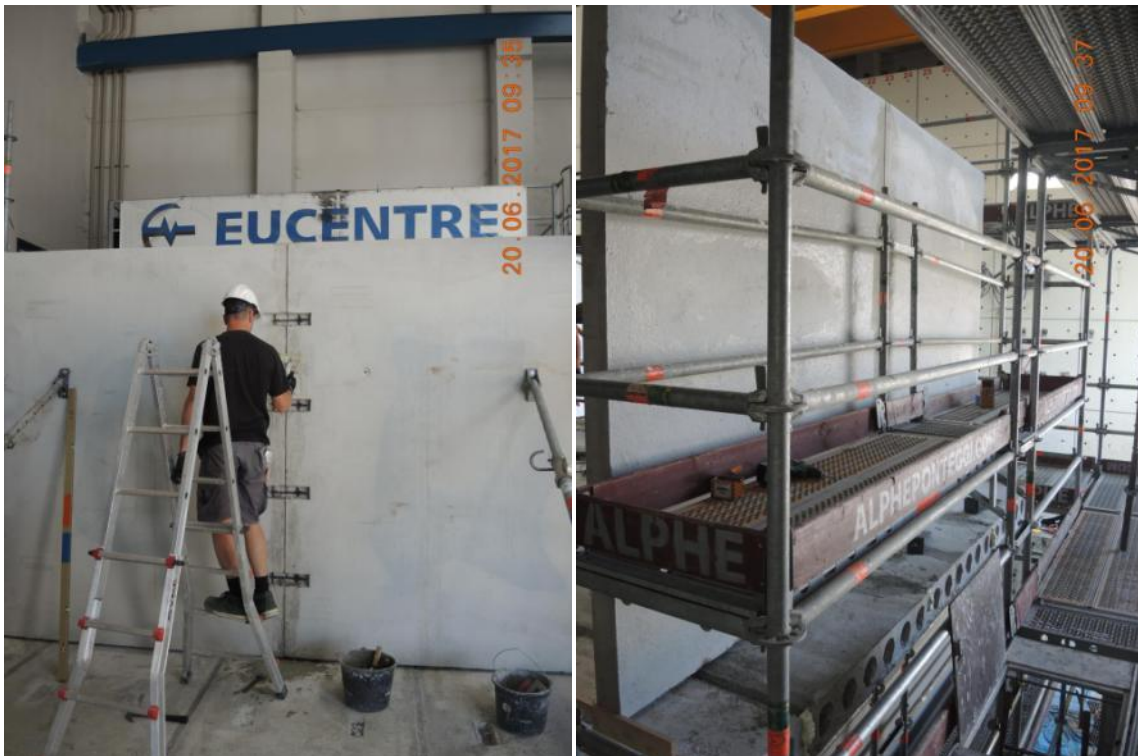
Figure 135. Erection of second-storey transversal walls – Opposite sides of EUC-BUILD5 specimen.
