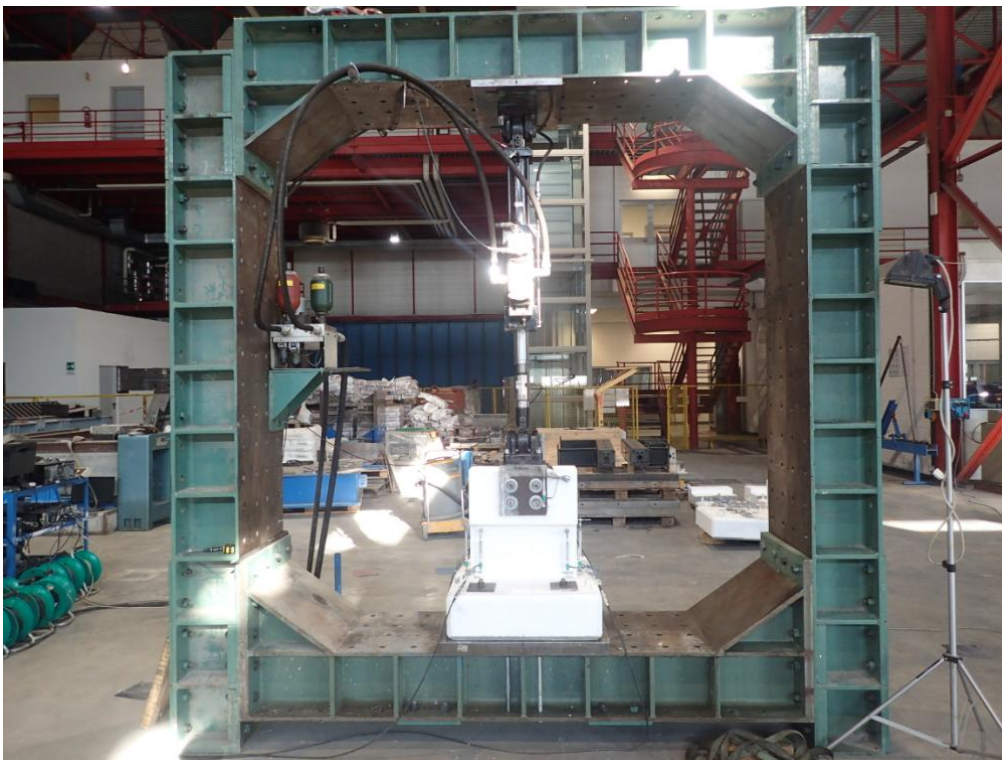
Figure 71. Global view of the experimental setup for cyclic testing of three-way panel connections.
