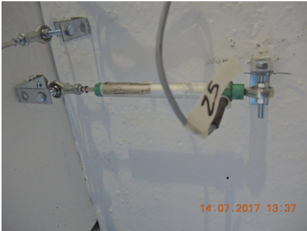
Figure 217. Detail of a potentiometer installed at the top of lateral walls.
