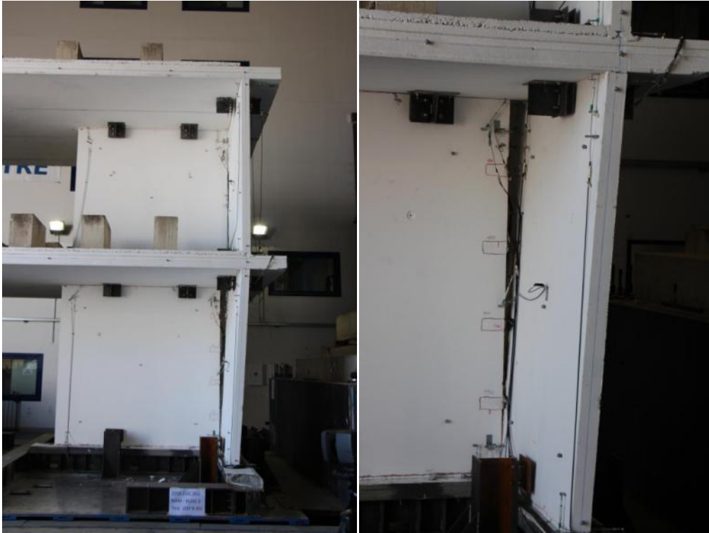
Figure 318. Loss of verticality and accumulation of residuals due to failure of bent three-way panel joints.
