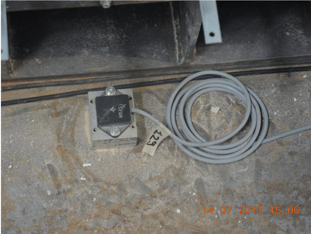
Figure 229. Detail of the 1D accelerometer installed on the shake-table.
