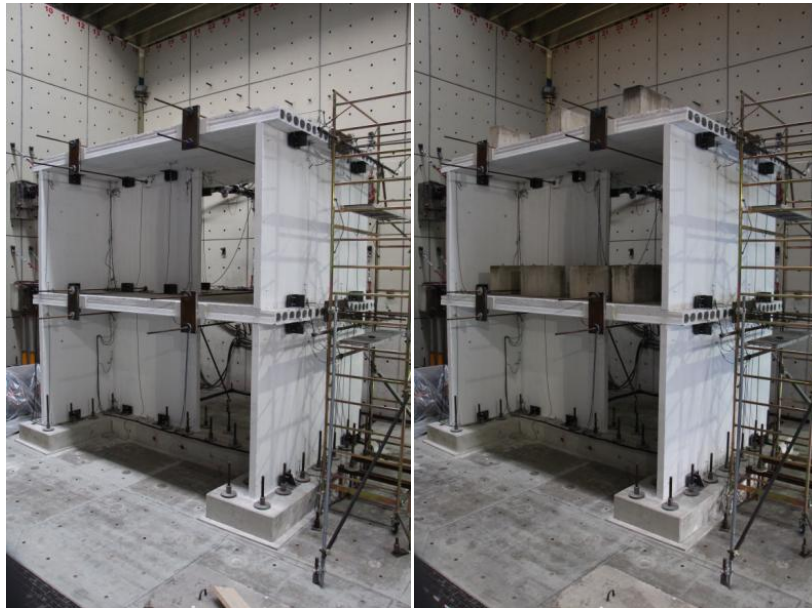
Figure 91. Photographs of EUC-BUILD4 specimen before cyclic testing.
