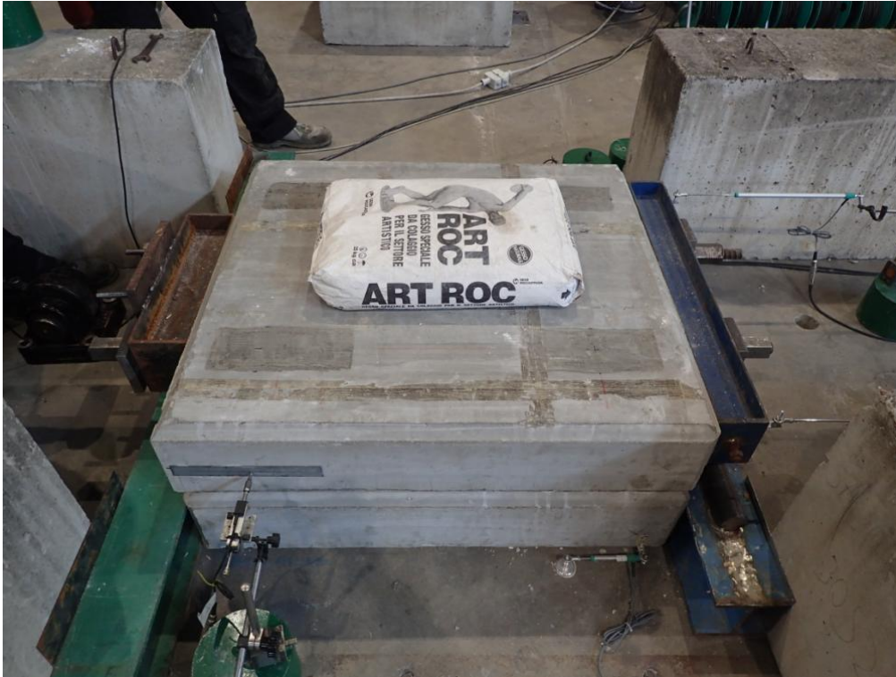
Figure 36. Vertical loading configurations – Configuration #1, low vertical pressure (0.2 MPa).
