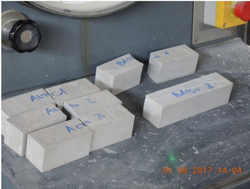
Figure 5. Failure mode of specimens at the end of three-points flexural testing of gap-filling mortar samples.
