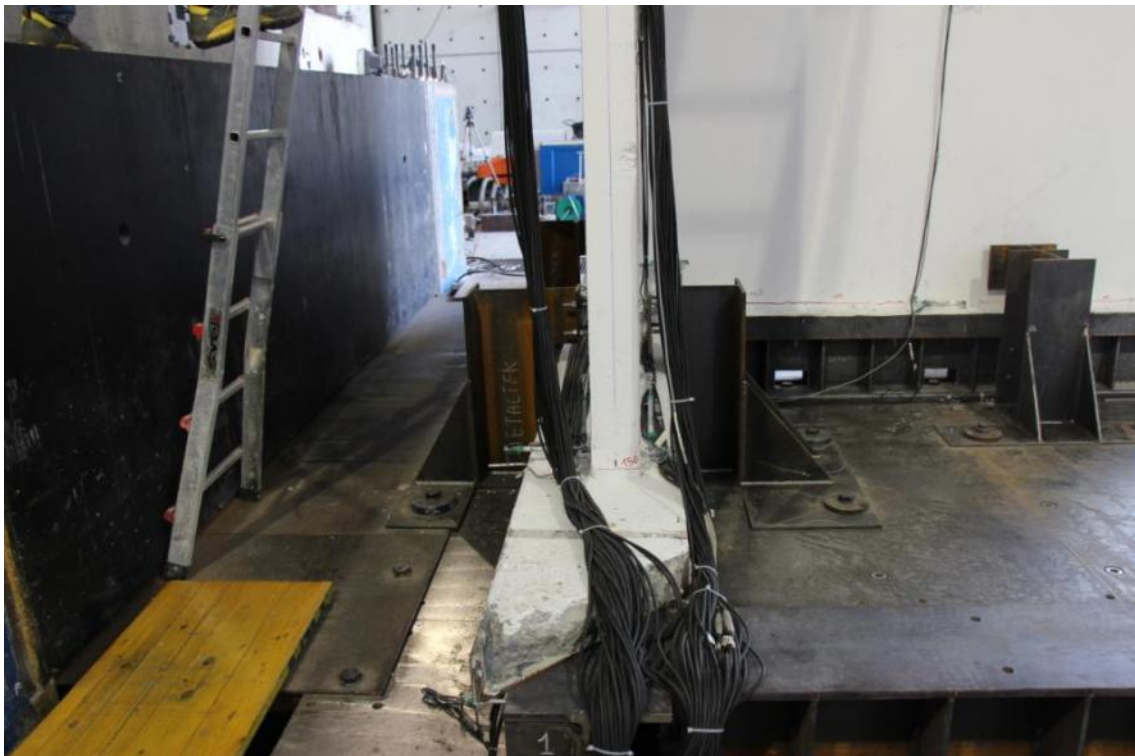
Figure 283. Formation of a new crack at the base of transversal walls – Panel 1L1, South-East side.
