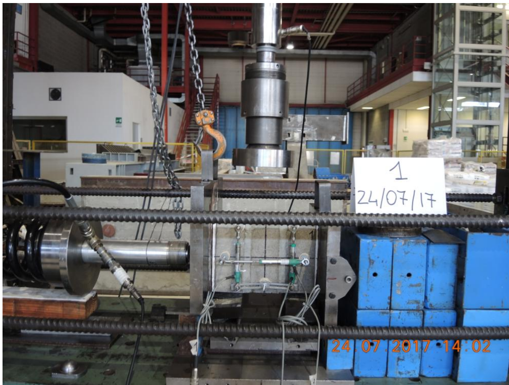
Figure 6. Testing apparatus for triplet specimens – Characterisation of cohesion and friction of mortar.
