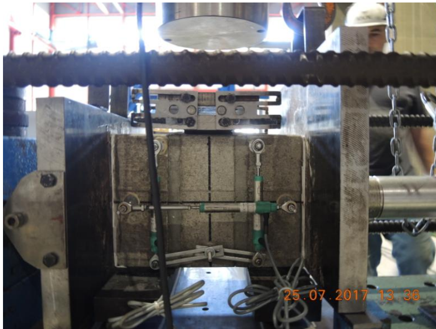
Figure 9. Testing apparatus and installed/assembled triplet specimen.
