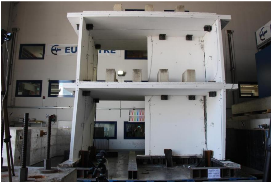
Figure 317. Deformed shape of EUC-BUILD5 specimen at the end of dynamic testing.
