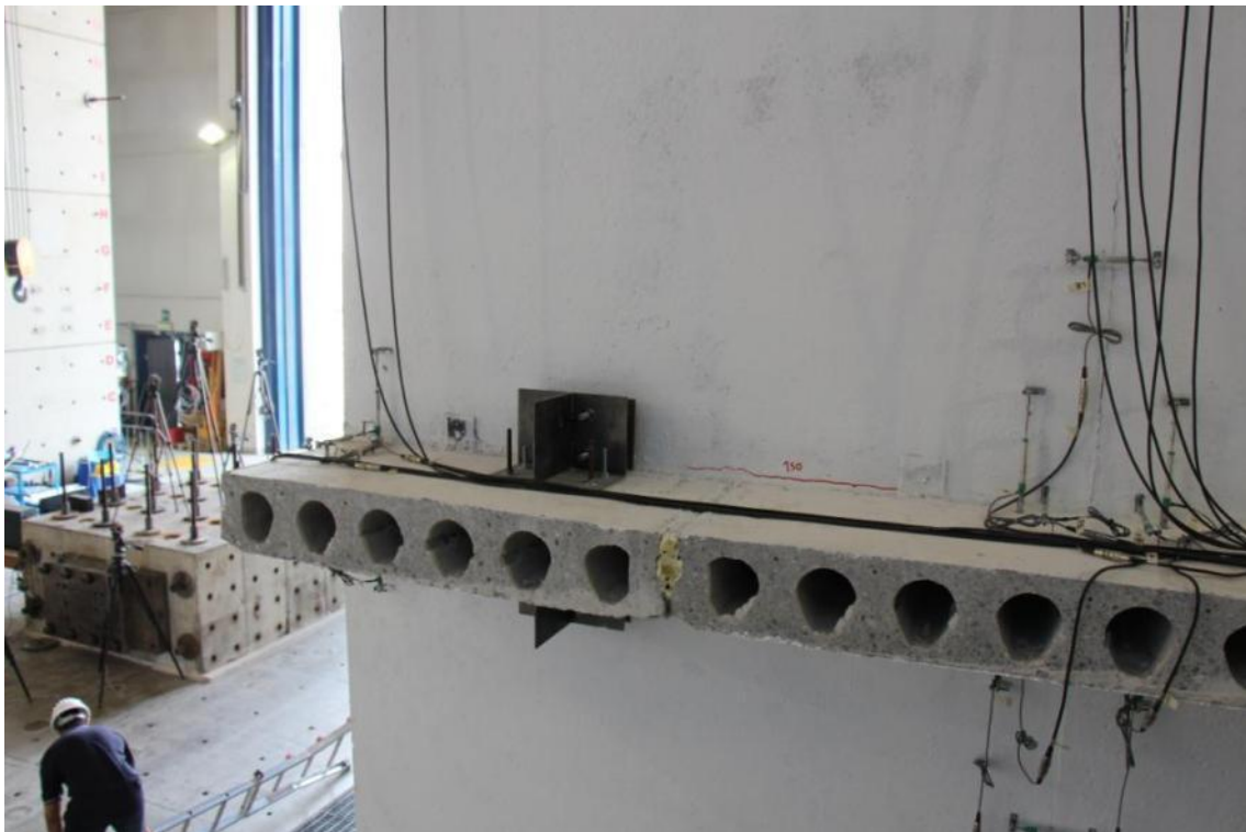
Figure 287. Development of horizontal flexural cracks at the base of panel 2L2 – Second-storey lateral wall.
