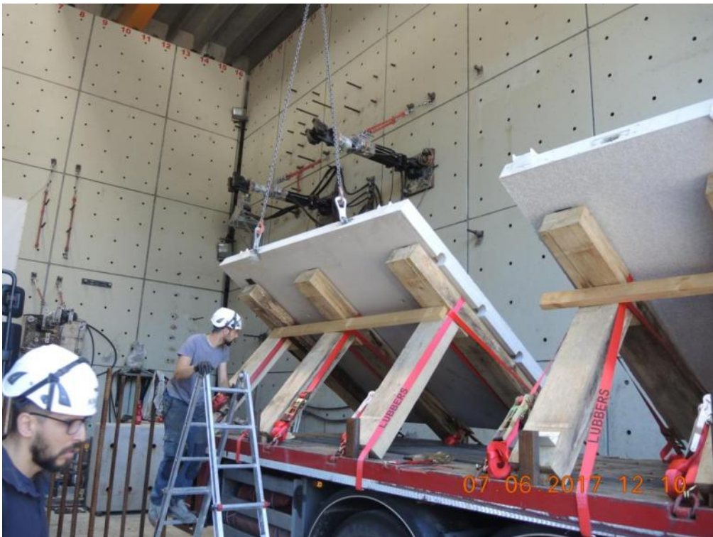
Figure 101. Crane-induced uplift of precast wall panels – Detail of the adopted two-points lifting scheme.
