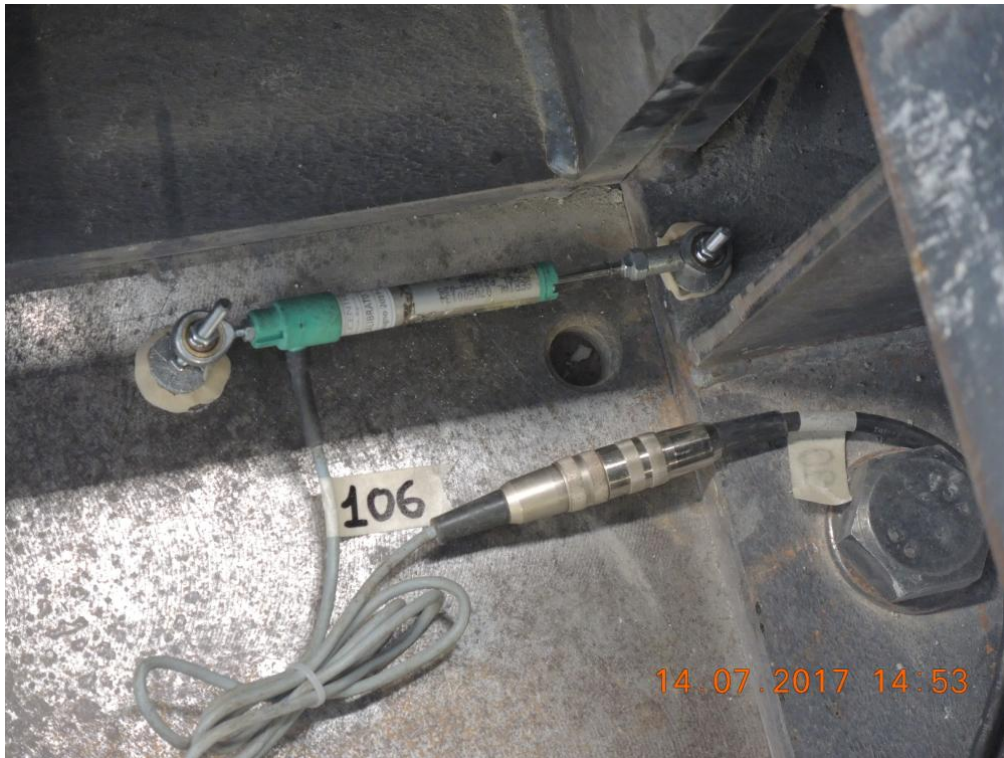
Figure 225. Potentiometer for sliding of steel foundation on the shake-table.
