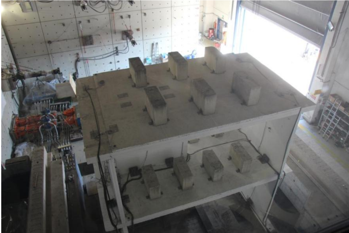
Figure 181. Isometric top view of EUC-BUILD5 specimen – Detail of restrainers and concrete masses.
