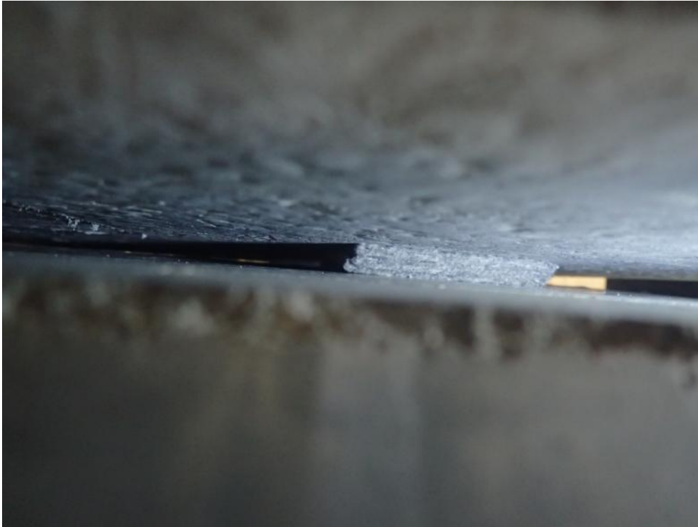
Figure C3. First cyclic friction testing attempts – Symmetric configuration, four layers of exhausted felt.
