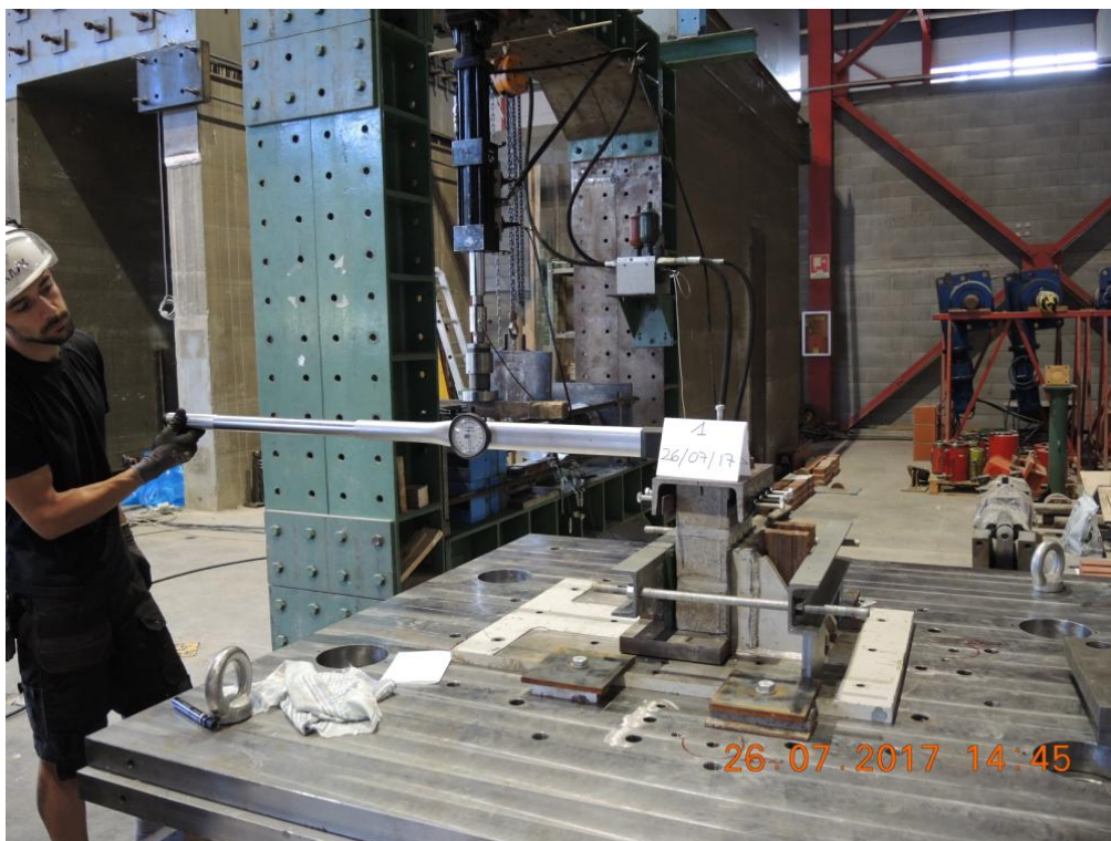
Figure 19. Testing apparatus for bond wrench tests – Boundary conditions and application of loads.
