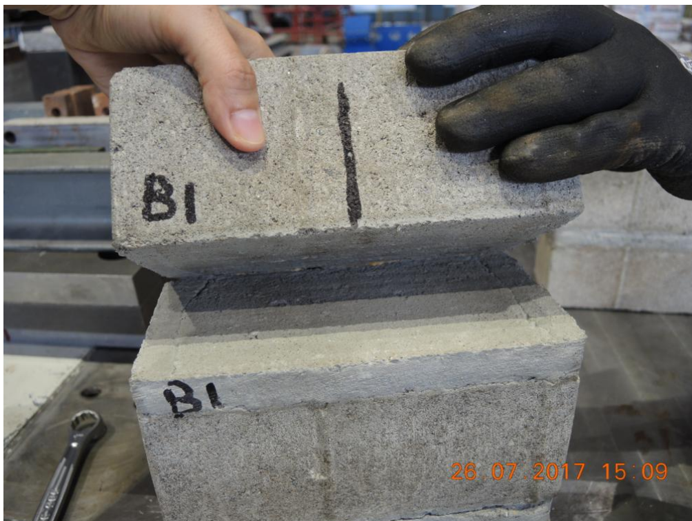
Figure 21. Bond wrench testing: first test, bed-joint #01 – Observed failure mode (A1).
