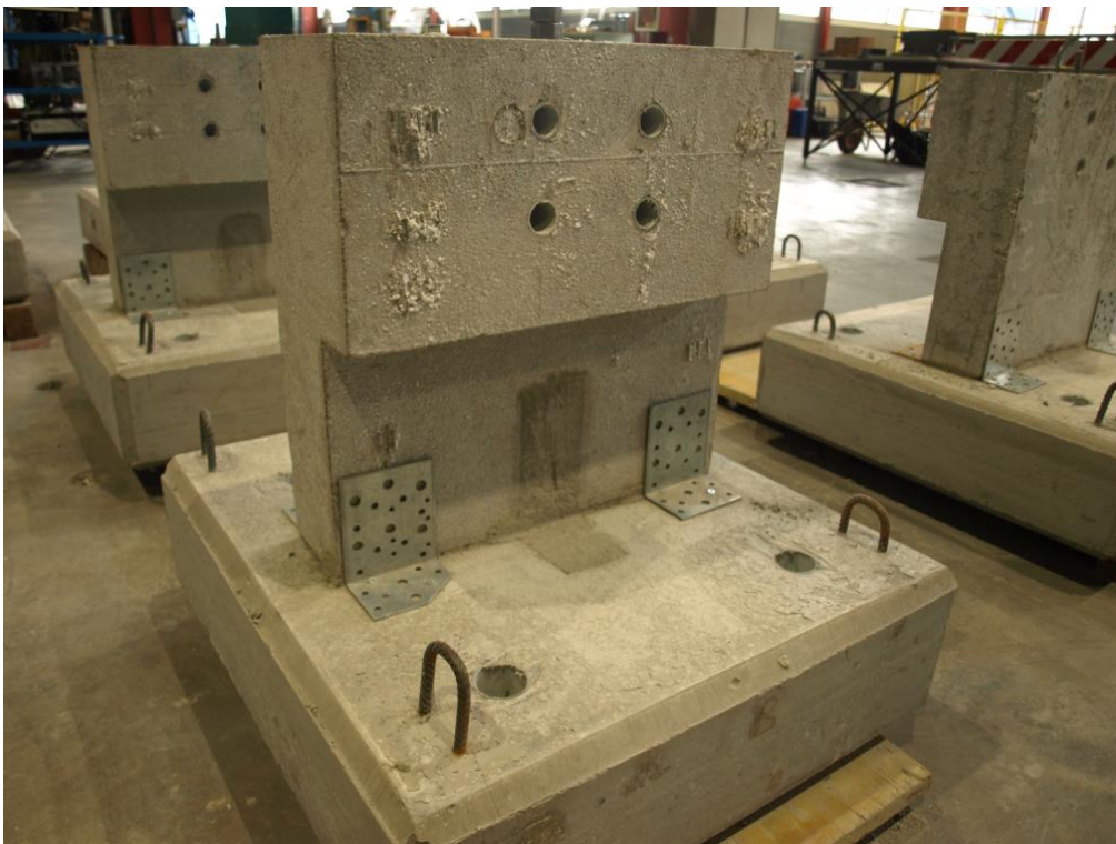
Figure 70. Detail of a specimen after mortar grout and curing.
