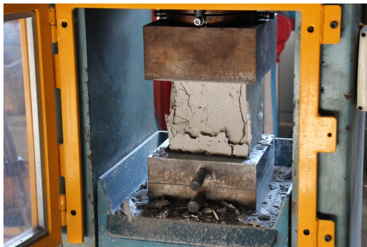
Figure 1. Testing apparatus for characterisation of compressive strength of concrete cubes.
