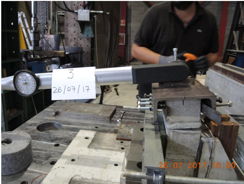
Figure 22. Bond wrench testing: third test, bed-joint #03 – Observed failure mode (A2).
