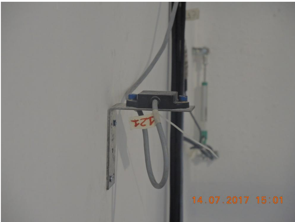
Figure 228. Detail of a 1D accelerometer mounted on a stability wall panel.
