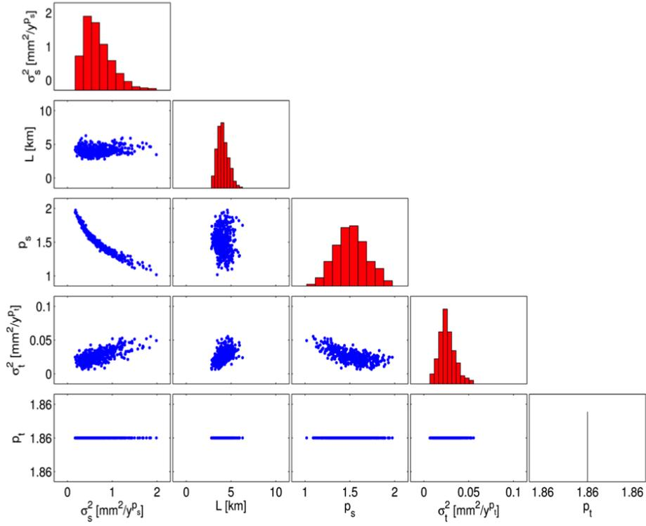
Figure 3: Results of the the Monte-Carlo approach to estimate only four model parameters. The parameter  $p_t$  has been constrained to be equal to 1.86. The plot shows the histograms and mutual scatter plot of the estimates. From 500 in total, 465 times the algorithm converged to a solution.
