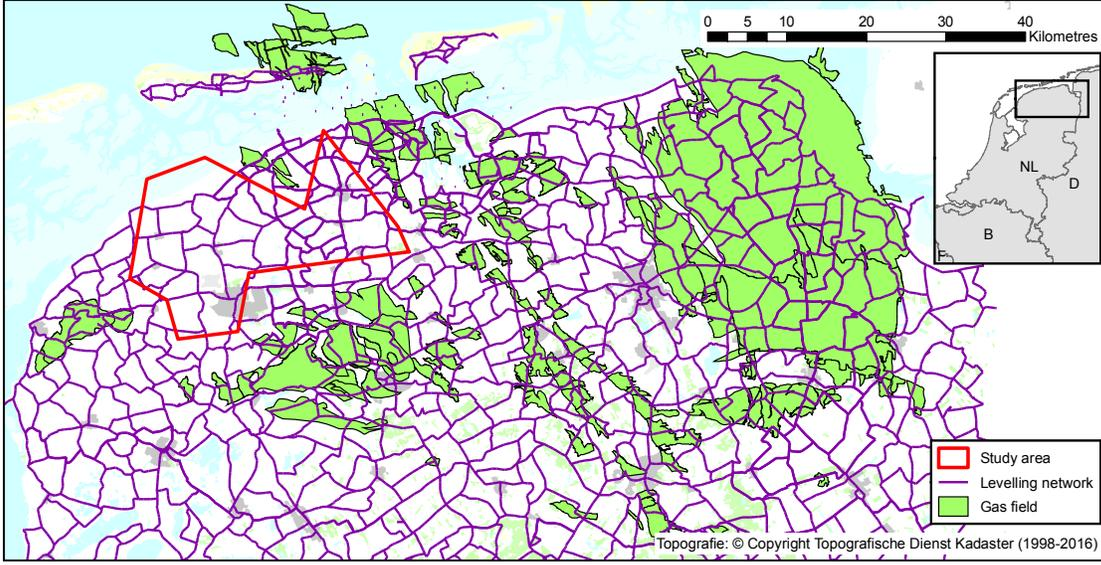
Figure 1: Selected area for levelling data analysis. For estimation of the idealisation noise parameters, the levelling surveys outside the influence area of gas production have been selected.
