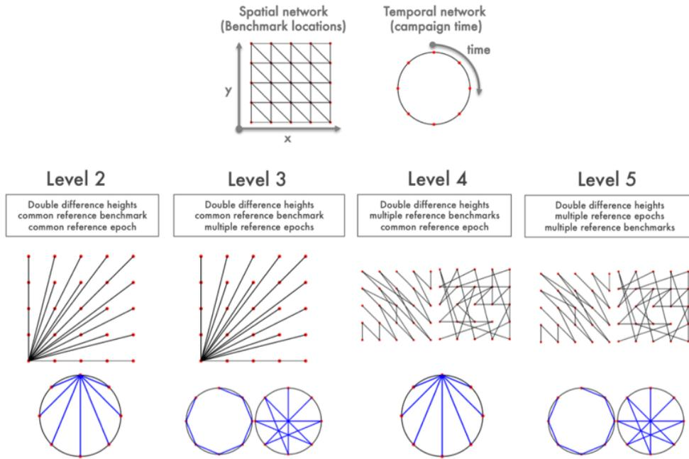
Figure 6: Schematic visualisation of output levels for levelling (as proposed in LTS1); The concept is adaptable for other techniques.
