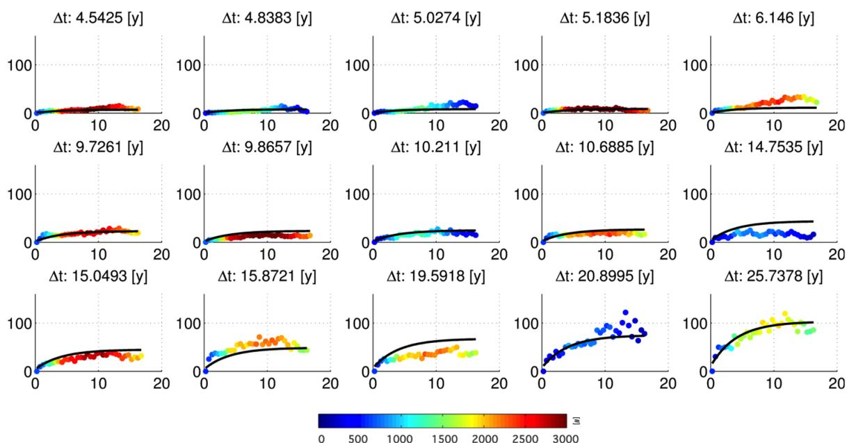
Figure 4: Spatial variogram profiles of levelling data over the signal-free area for different temporal lags (from 4.5 to 25.7 years). The X-axes are labelled by the spatial lag in [km], and the Y-axes display the variograms [mm<sup>2</sup>].
