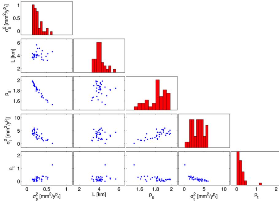
Figure 2: Results of the the Monte-Carlo approach to estimate the five model parameters. Histogram and mutual scatter plot of the estimates. Only 35 from 500 cases converged to a solution.
