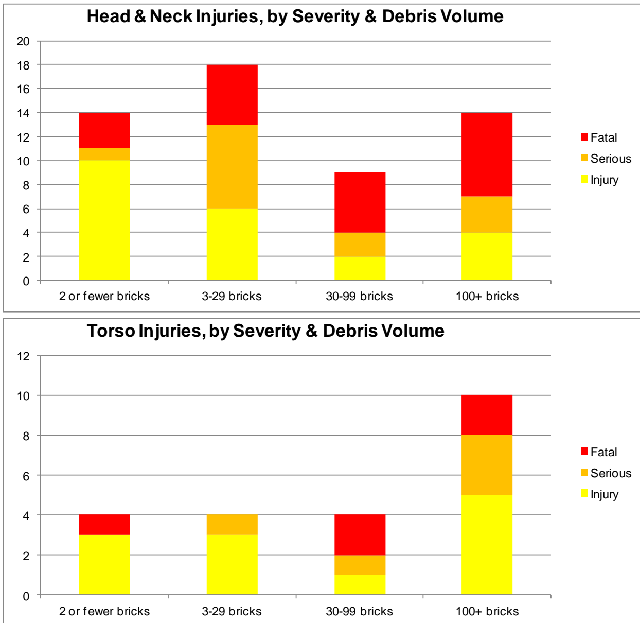
Figure A6.13: Relative Severity of Head &amp; Torso Injuries vs Debris Volume
