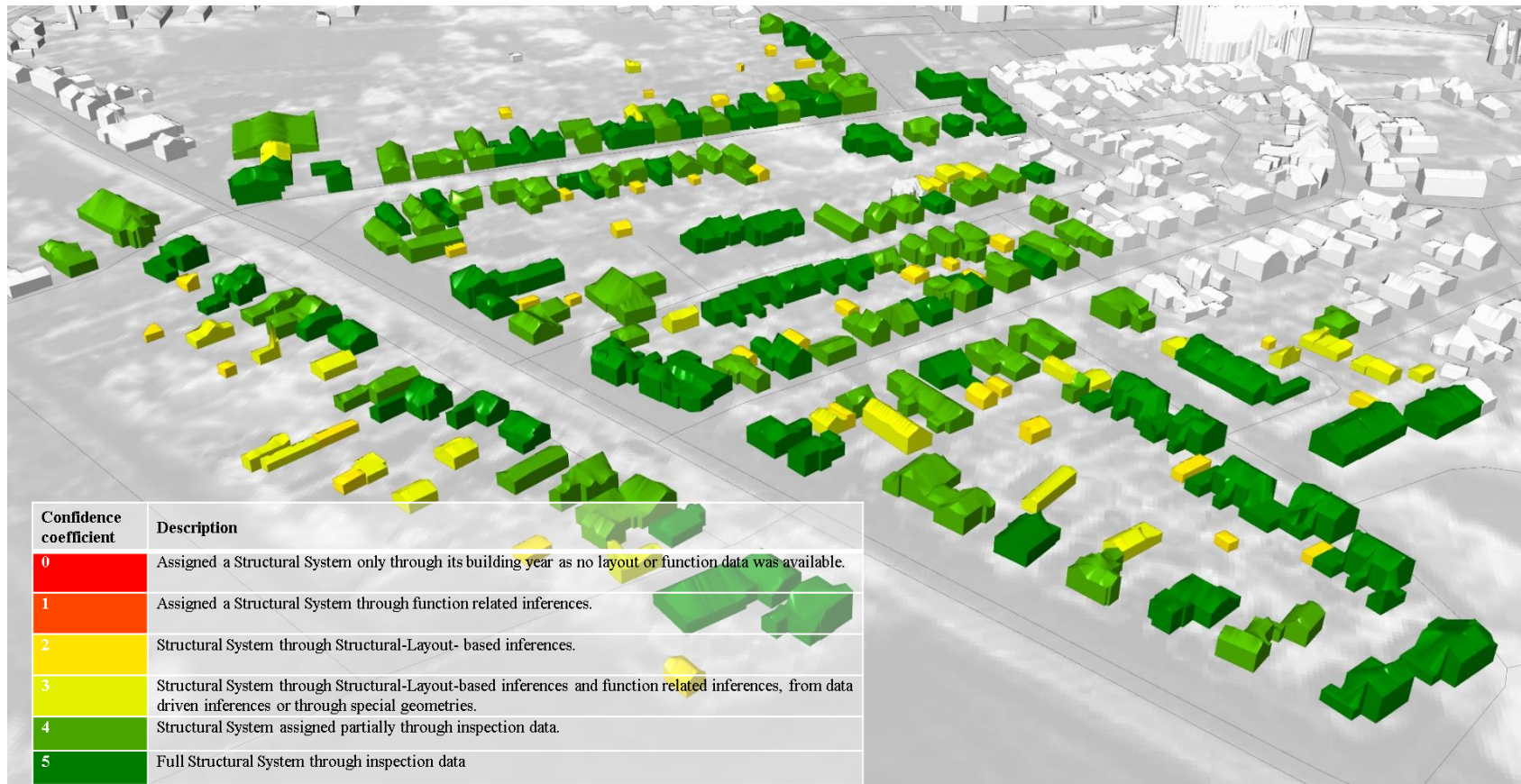
Figure 32 Set of buildings in the region color-coded based on the confidence coefficient (same buildings as the ones shown in Figure 4)
