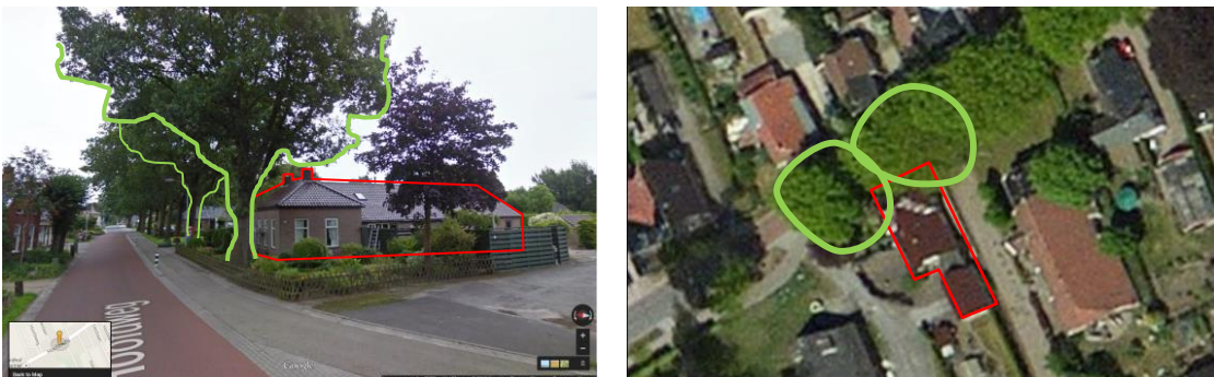
Figure 6 Example of overhanging trees creating noise in the height data.
