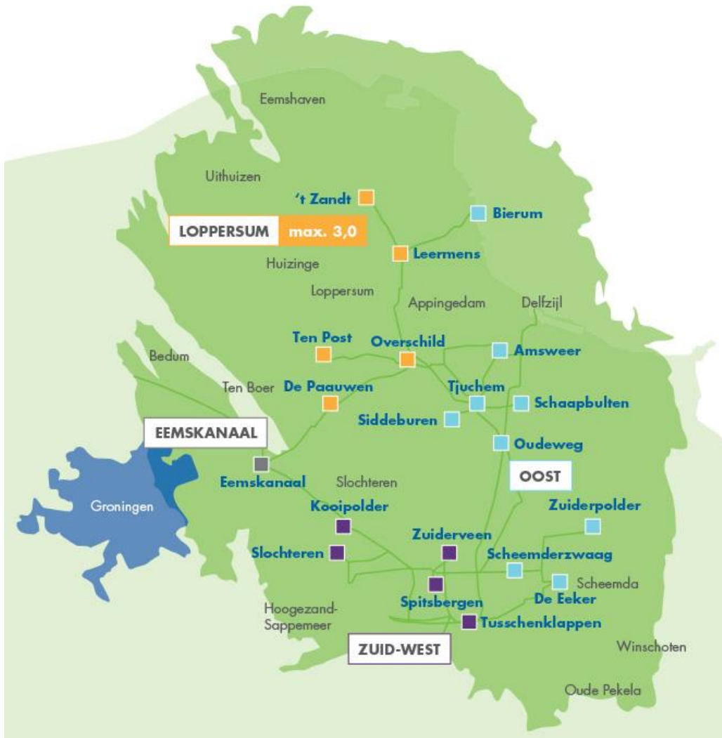
Figure A1.3: Field map showing the outline of the Groningen field with locations of production clusters, major pipelines, and locations of major towns and villages. Production from the Loppersum clusters has been constrained to 3 bcm/a.
