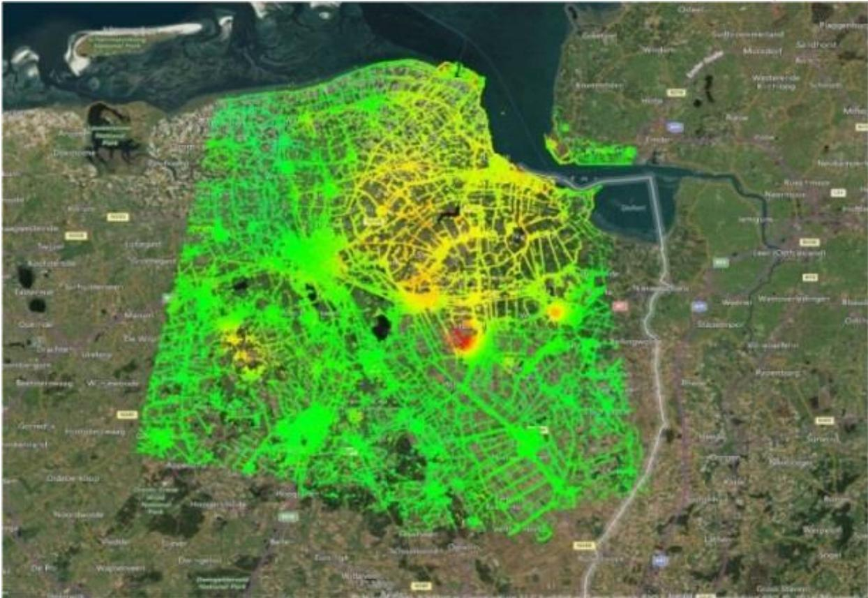
Fig. 4.3 InSAR (TSX 3 m resolution) measurements over Groningen.
