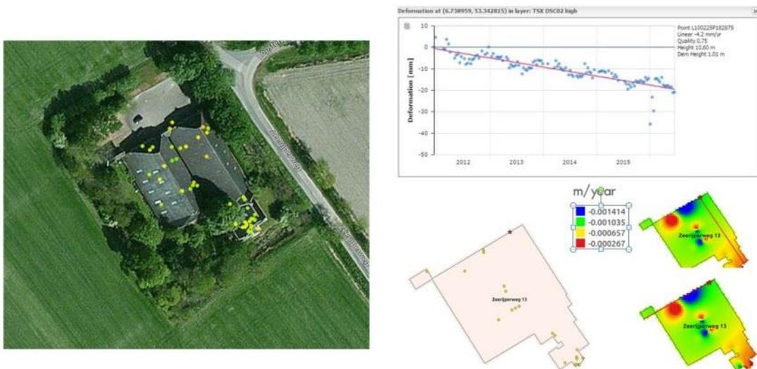
Fig. 4.5 InSAR measurements over a building (left) and deformation time series derived from one of the InSAR measurements (top right). Differential subsidence of the building can also be derived (low right).
