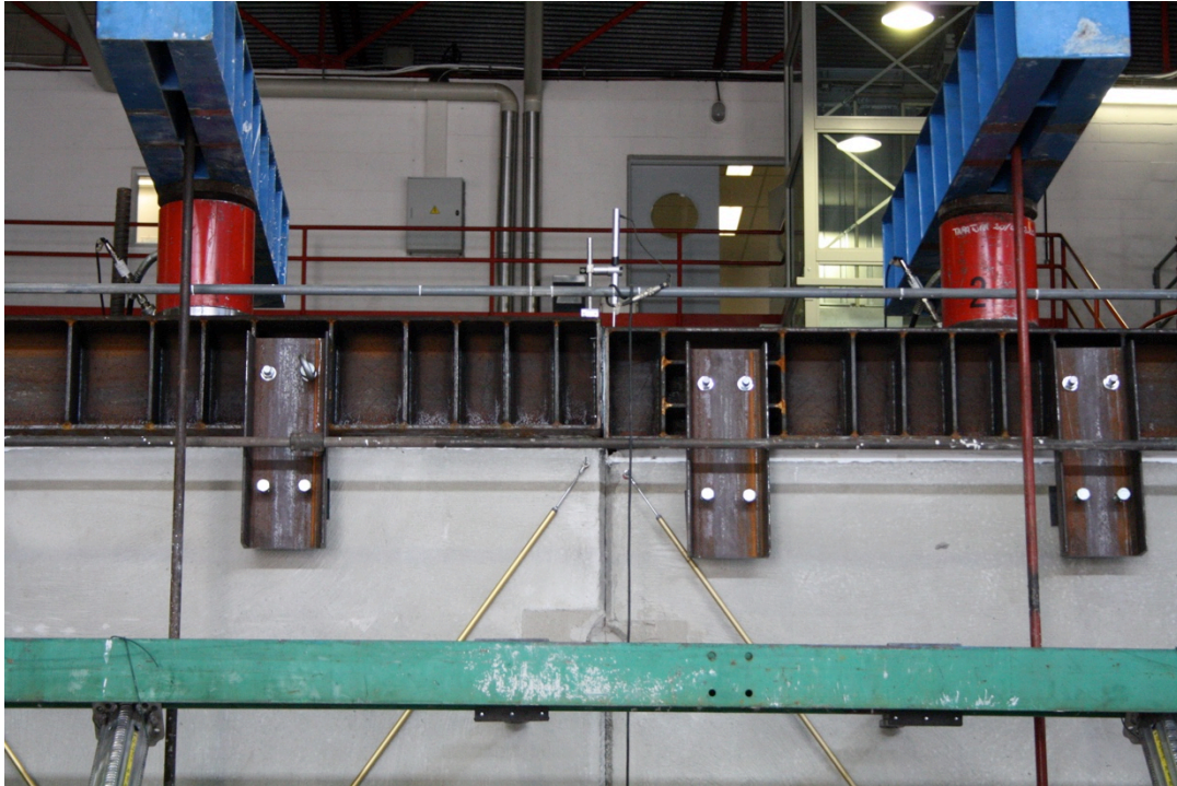
Figure 176: Vertical displacement due to rocking mechanism of Specimen 04 – detail at the top of the assembly
