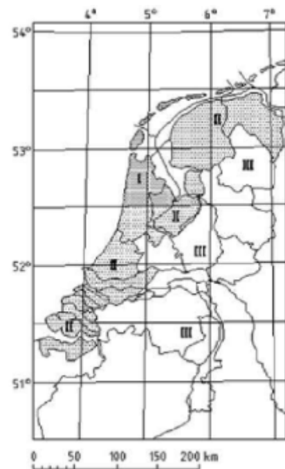
Figure 134: Classification of wind load and values assumed for design
