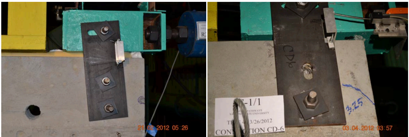
Fig. 39: Horizontal slot top slotted connection: (a) translation of the coil rod; (b) Rotation of the slotted connection plate connections with the fracture of coil rod at slotted connection
