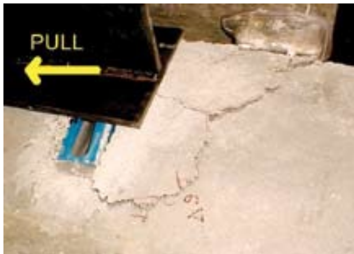
Fig. 50: Slotted connector shear test
