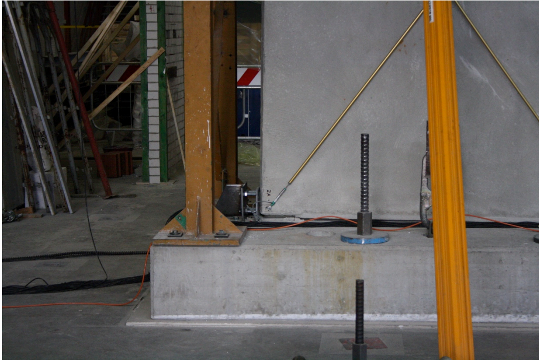
Figure 178: Rocking behaviour and base uplift at the corner of the panel – Specimen 04
