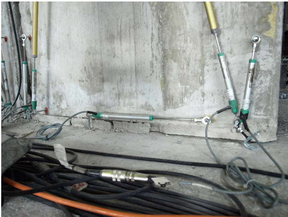
Figure 211: Base uplift along the entire pier of Specimen 08 – opposite side
