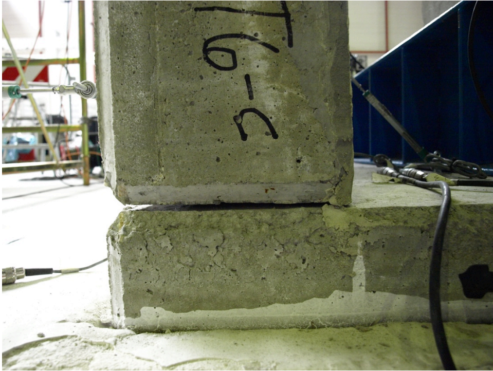
Figure 249: Detail of gap opening at the end of the test – Specimen 12
