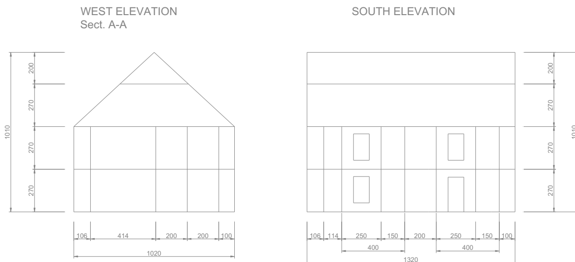
Fig.92: Building case study: west and south elevation
