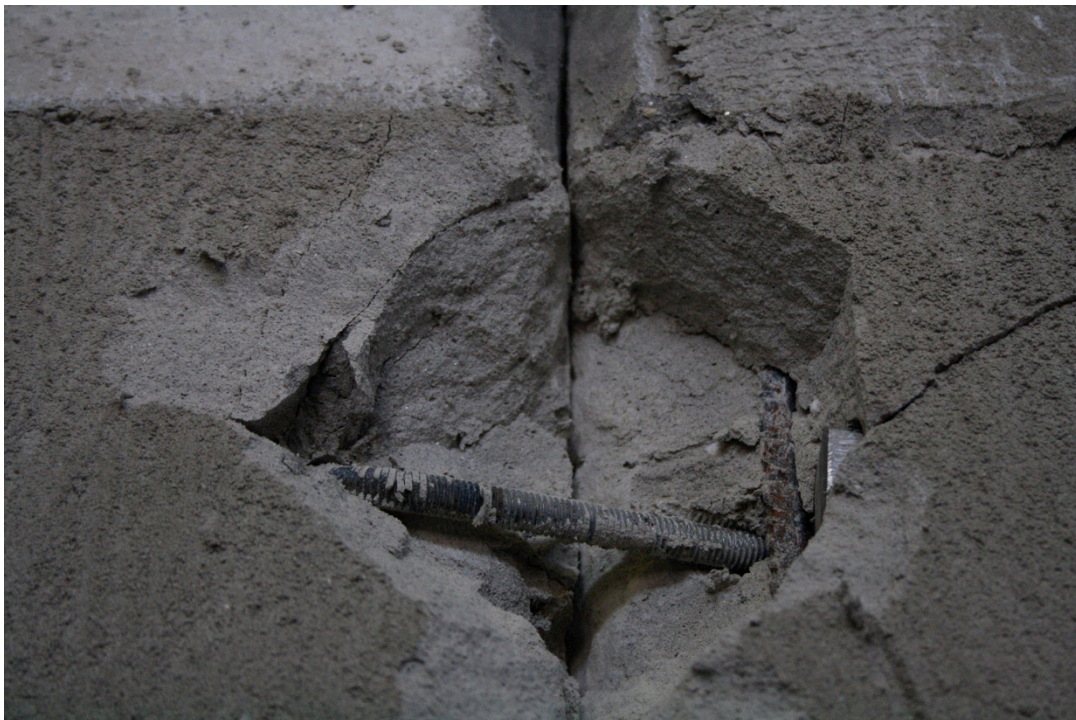
Figure 181: Failure of the anchors – Specimen 04
