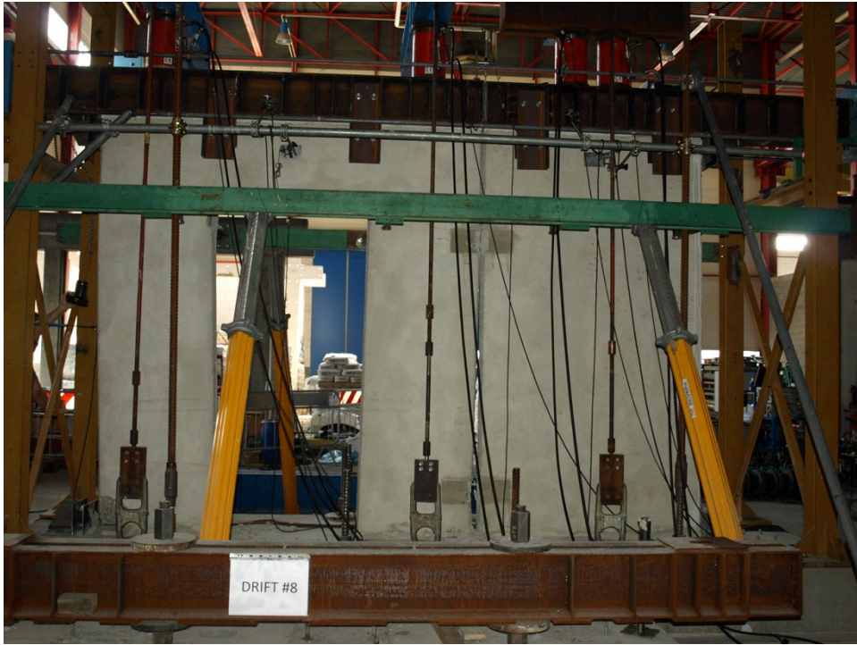
Figure 199: Deformed shape at the end of the test – Specimen 07
