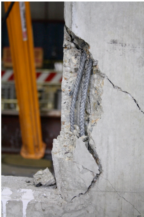
Figure 193: Cracking at the corners of the window in Specimen 06 – detail of the bottom left and right sides
