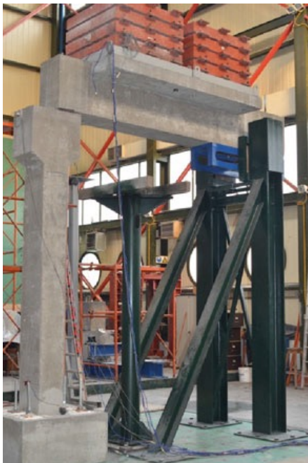
Fig. 22: (a) Prototype single-bay frame (left) and corresponding half-frame specimen (right) in deformed position (displacements and rotations are exaggerated); (b) experimental setup showing the half-frame specimen and the additional mass; (c) special device for achieving sliding pinned support at the free end of the beam
