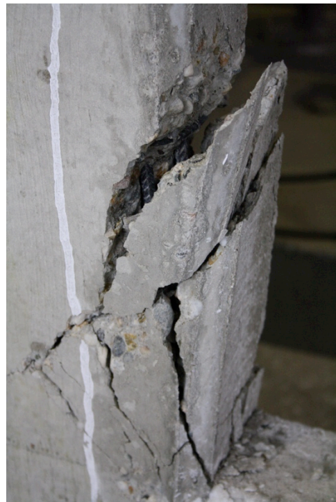
Figure 193: Cracking at the corners of the window in Specimen 06 – detail of the bottom left and right sides
