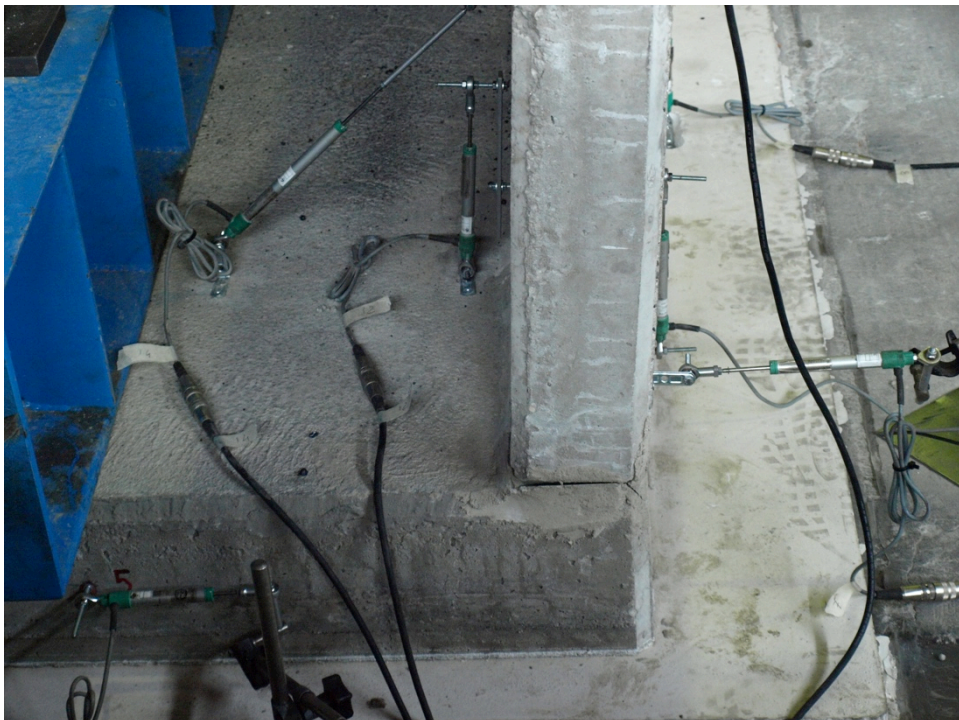
Figure 230: Rotation at the panels connection – side view of Specimen 09
