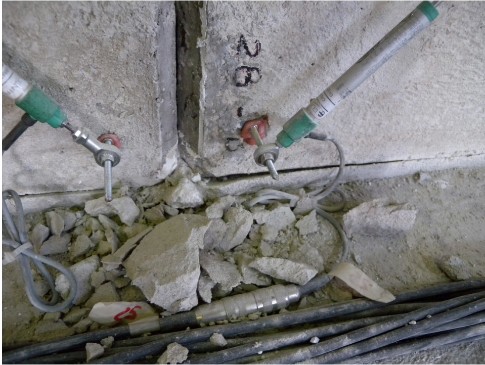
Figure 172: Rocking and base uplift at mid-panel assembly – Specimen 03
