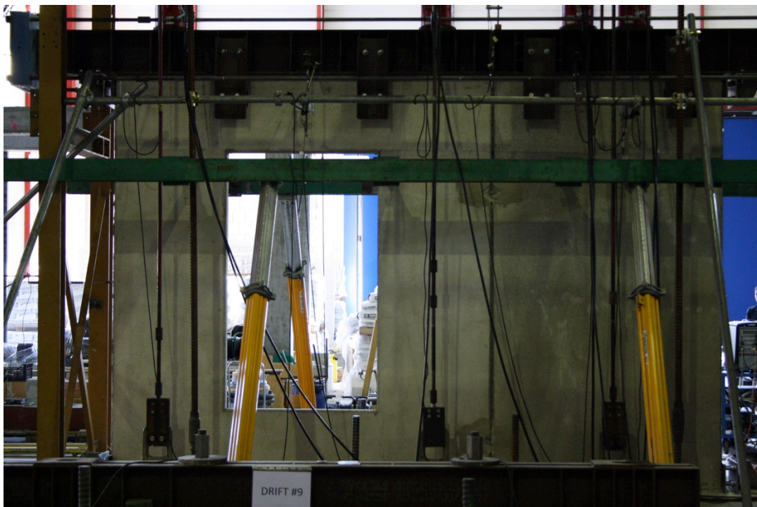
Figure 183: Deformed shape at the end of the test – Specimen 05
