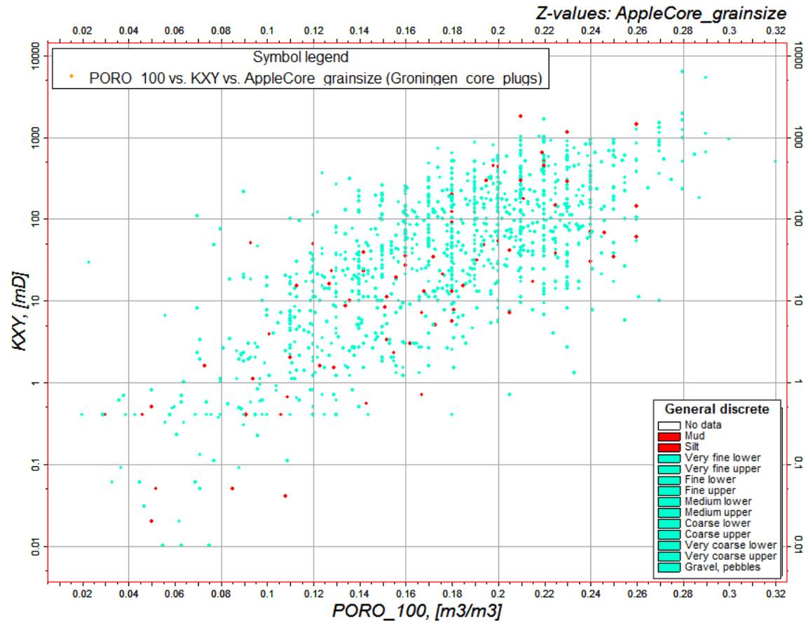
Fig. 19: Porosity-permeability cross-plot from core plug data, mud and silt plugs coloured red
