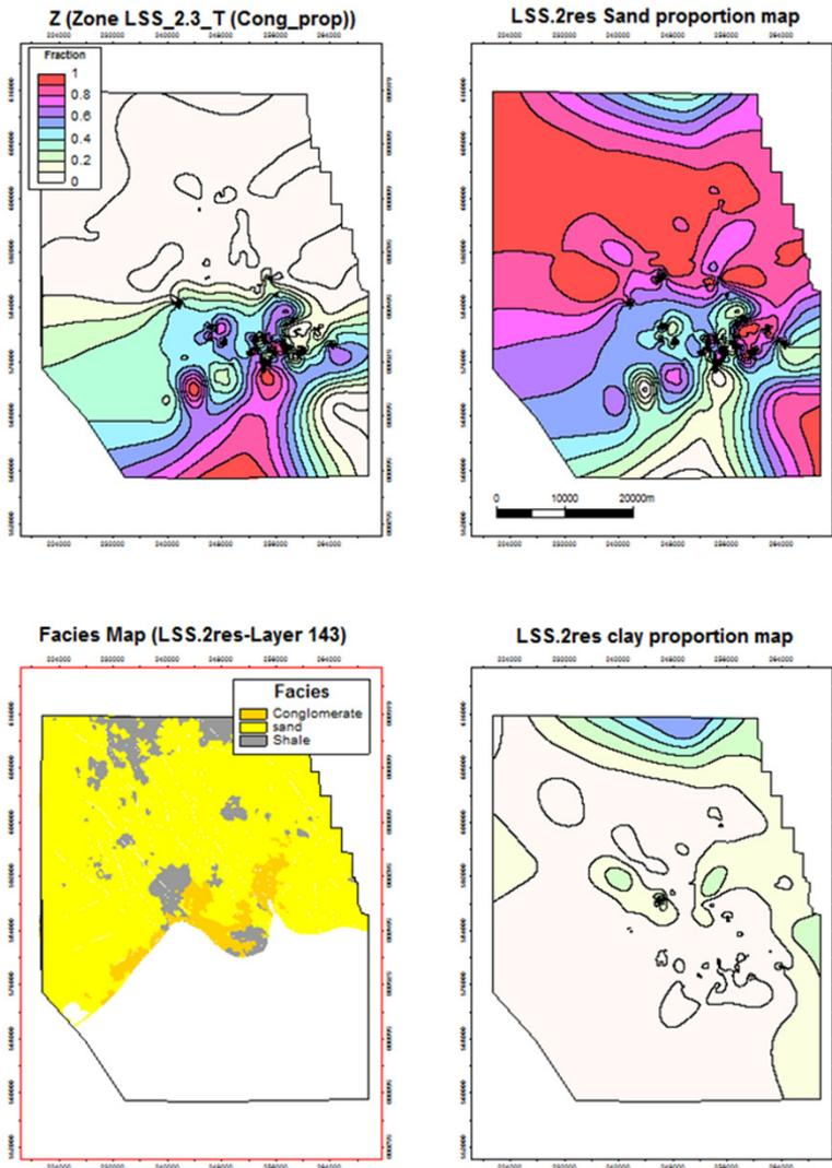
Fig. 26: Vertical proportion maps per electrofacies and one representative model layer for reservoir unit LSS.2res
