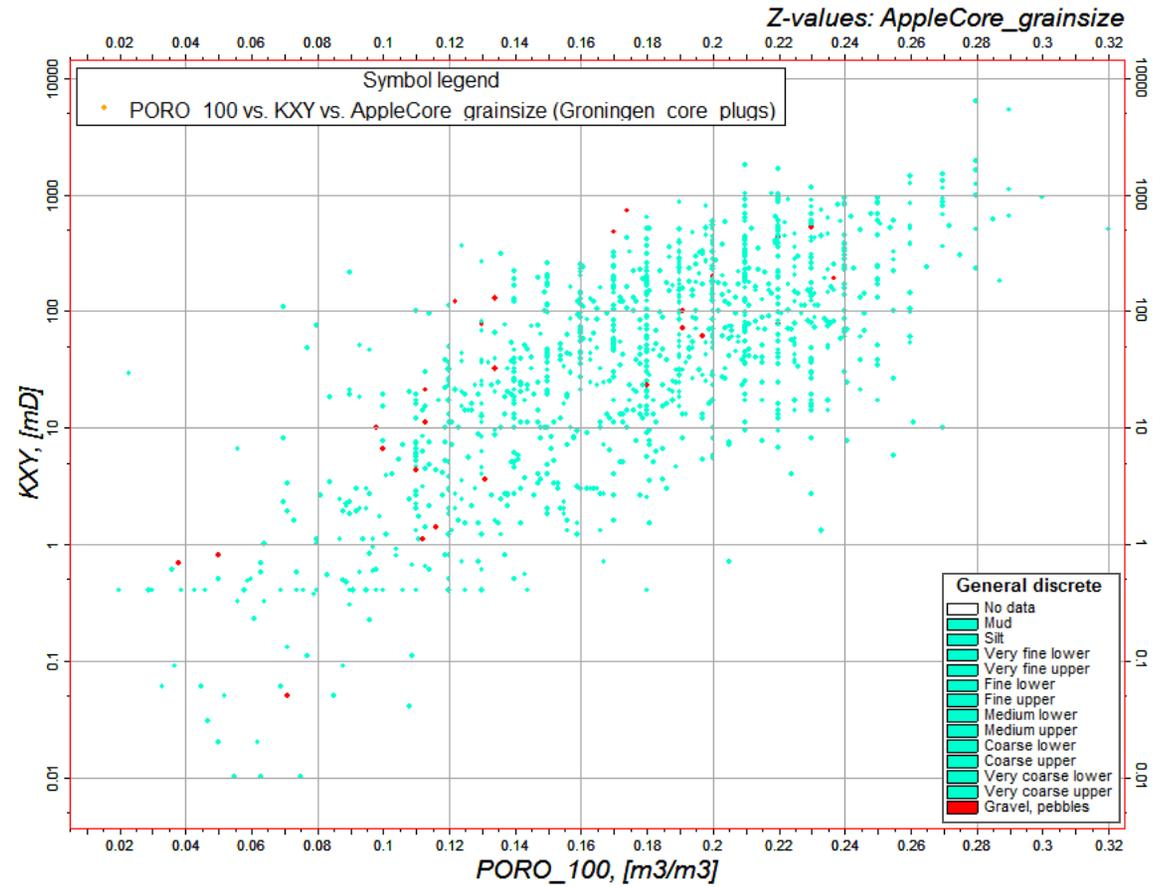
Fig. 24: Porosity-permeability cross-plot from core plug data, pebbly sandstone and conglomerate plugs coloured red
