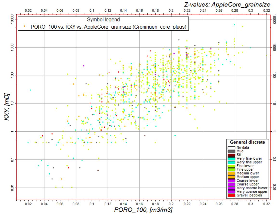
Fig. 18: Porosity-permeability cross-plot from core plug data, grouped by grain size class
