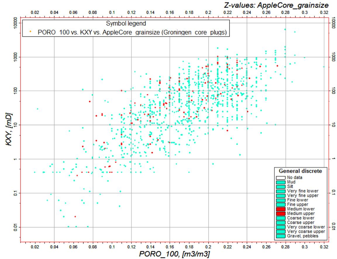
Fig. 22: Porosity-permeability cross-plot from core plug data, medium sandstone plugs coloured red
