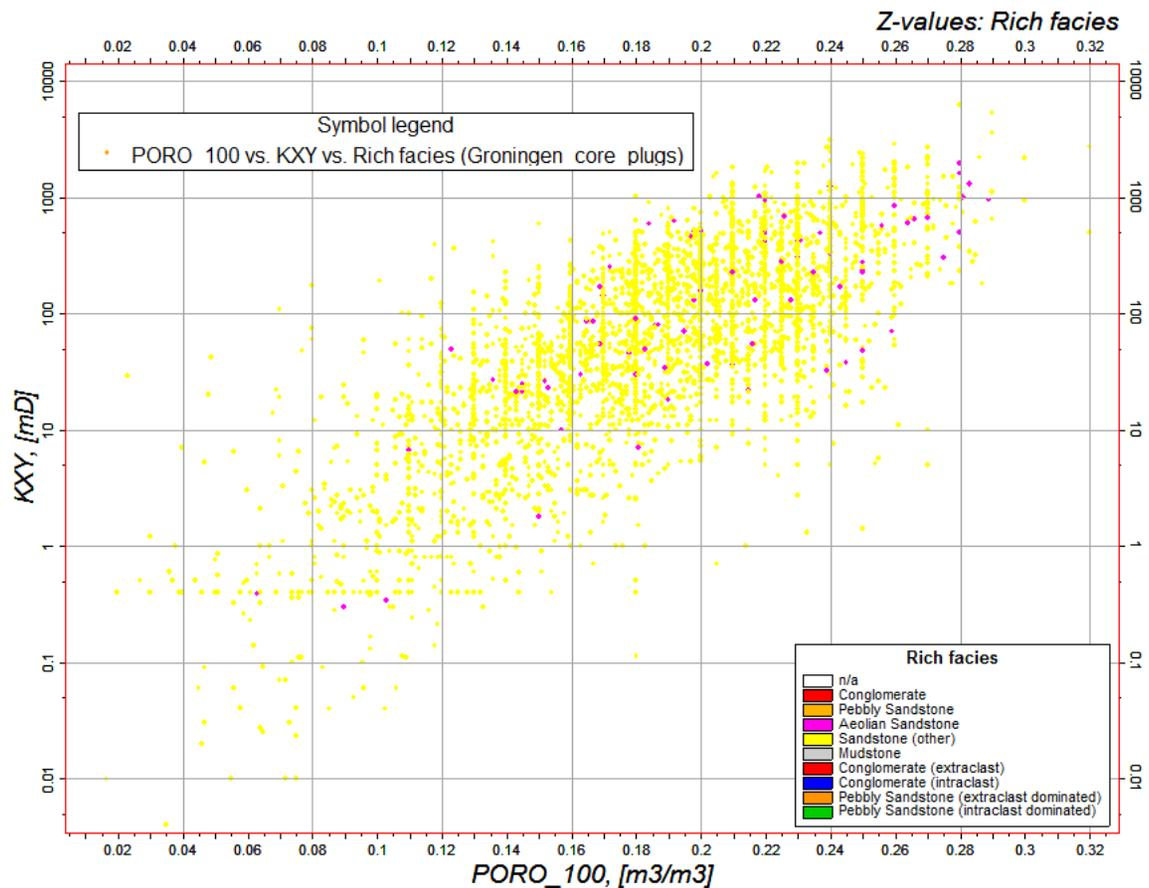
Fig. 11: Porosity-permeability cross-plot showing aeolian (purple) and undifferentiated (yellow) sandstone core plug data
