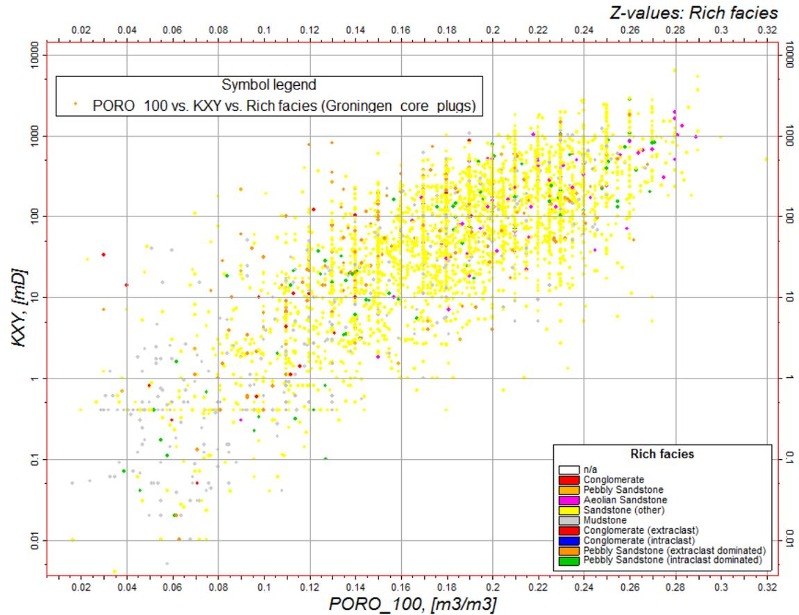
Fig. 10: Porosity-permeability cross-plot showing core plug data from 18 studied wells, grouped per lithofacies
