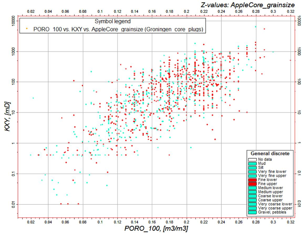
Fig. 21: Porosity-permeability cross-plot from core plug data, fine sandstone plugs coloured red
