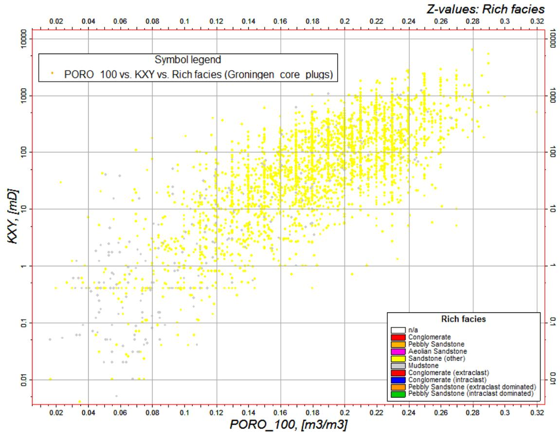
Fig. 16: Porosity-permeability cross-plot showing undifferentiated sandstone (yellow) and mudstone (grey) core plug data
