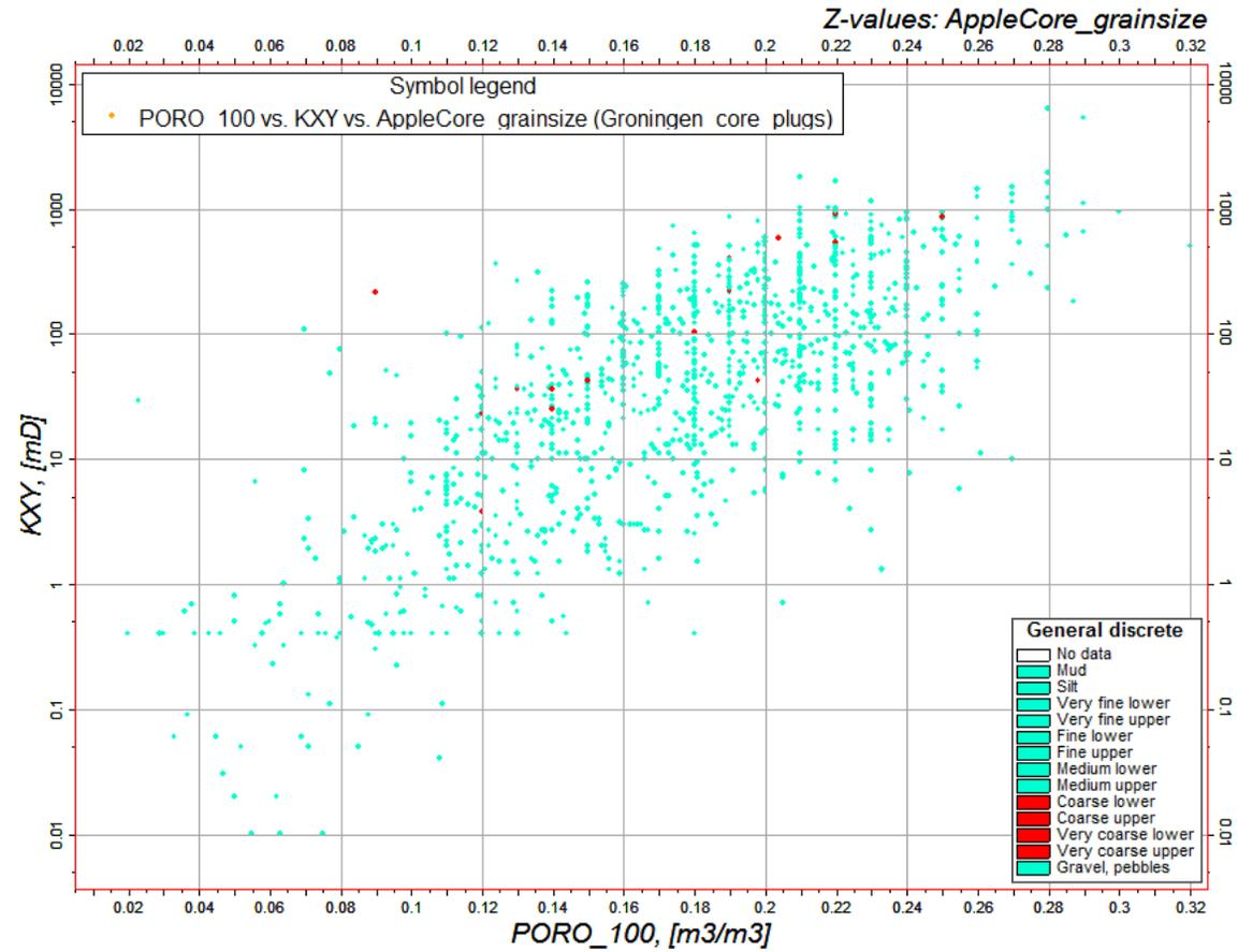
Fig. 23: Porosity-permeability cross-plot from core plug data, coarse to very coarse sandstone plugs coloured red
