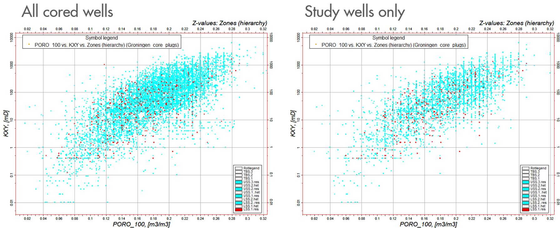
Fig. 30: Porosity-permeability cross-plot of core plug measurements, data points from LSS.1 res coloured red. Left-hand graph shows entire Groningen plug database, right-hand graph shows data for study wells only.
