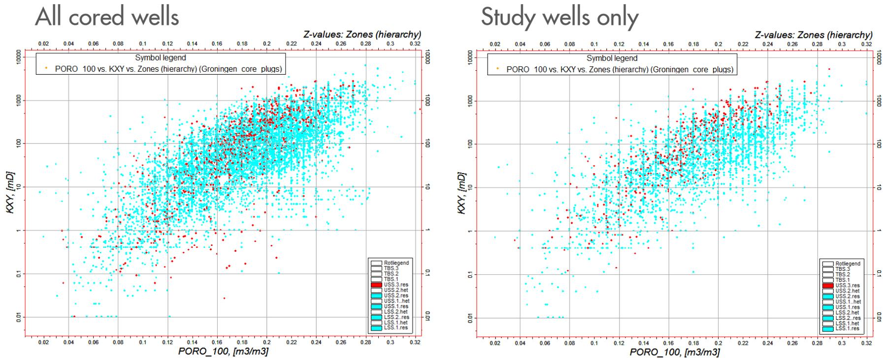
Fig. 34: Porosity-permeability cross-plot of core plug measurements, data points from USS.3res coloured red. Left-hand graph shows entire Groningen plug database, right-hand graph shows data for study wells only.
