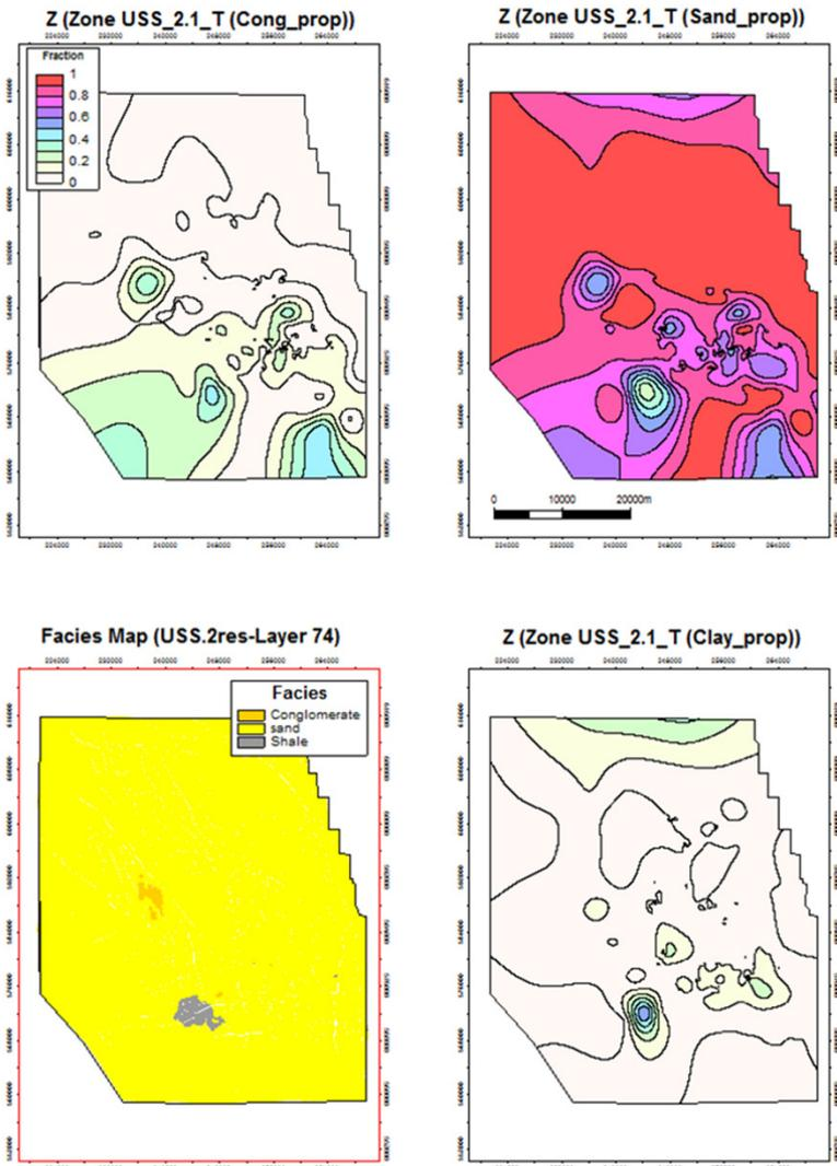
Fig. 28: Vertical proportion maps per electrofacies and one representative model layer for reservoir unit USS.2res
