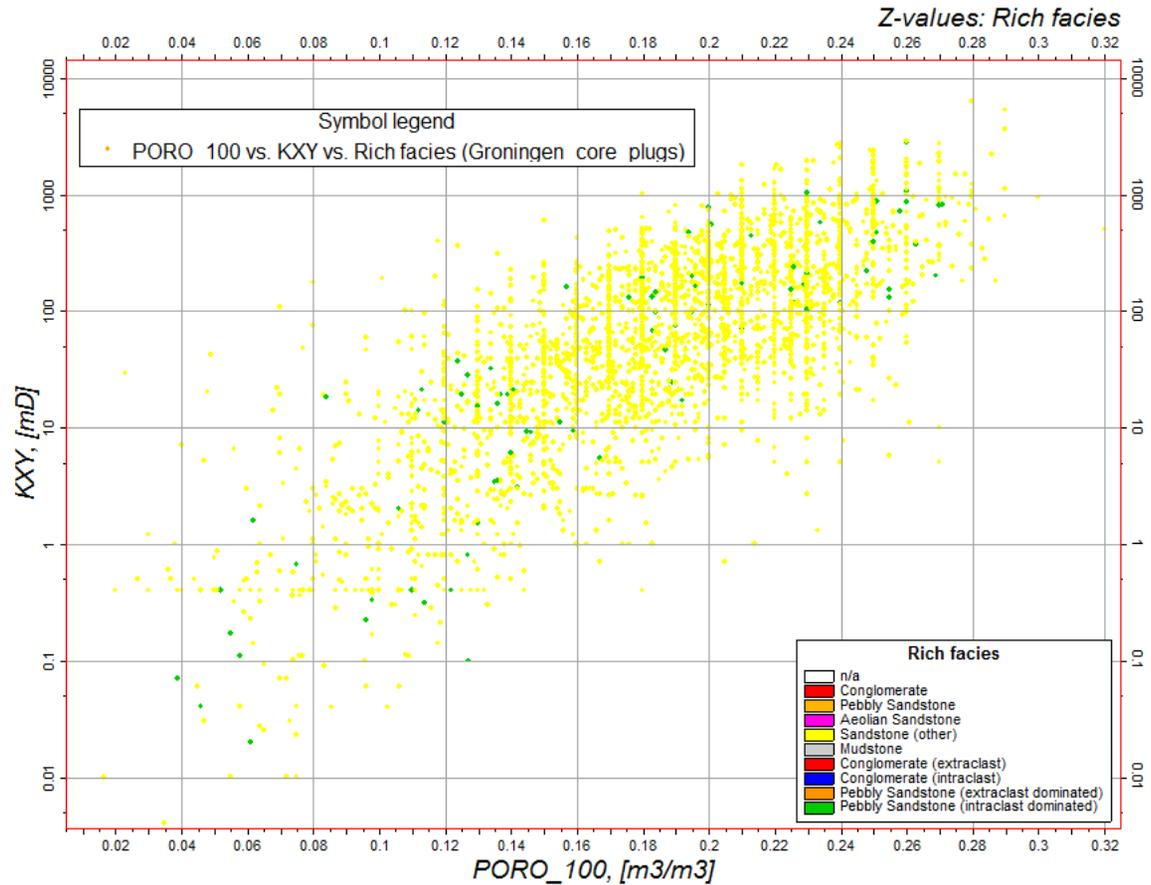
Fig. 14: Porosity-permeability cross-plot showing undifferentiated (yellow) and pebbly intraclast (green) sandstone core plug data
