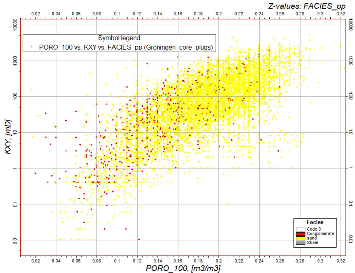
Fig. 15: Porosity-permeability cross-plot showing undifferentiated (yellow) and pebbly intraclast (green) sandstone core plug data
