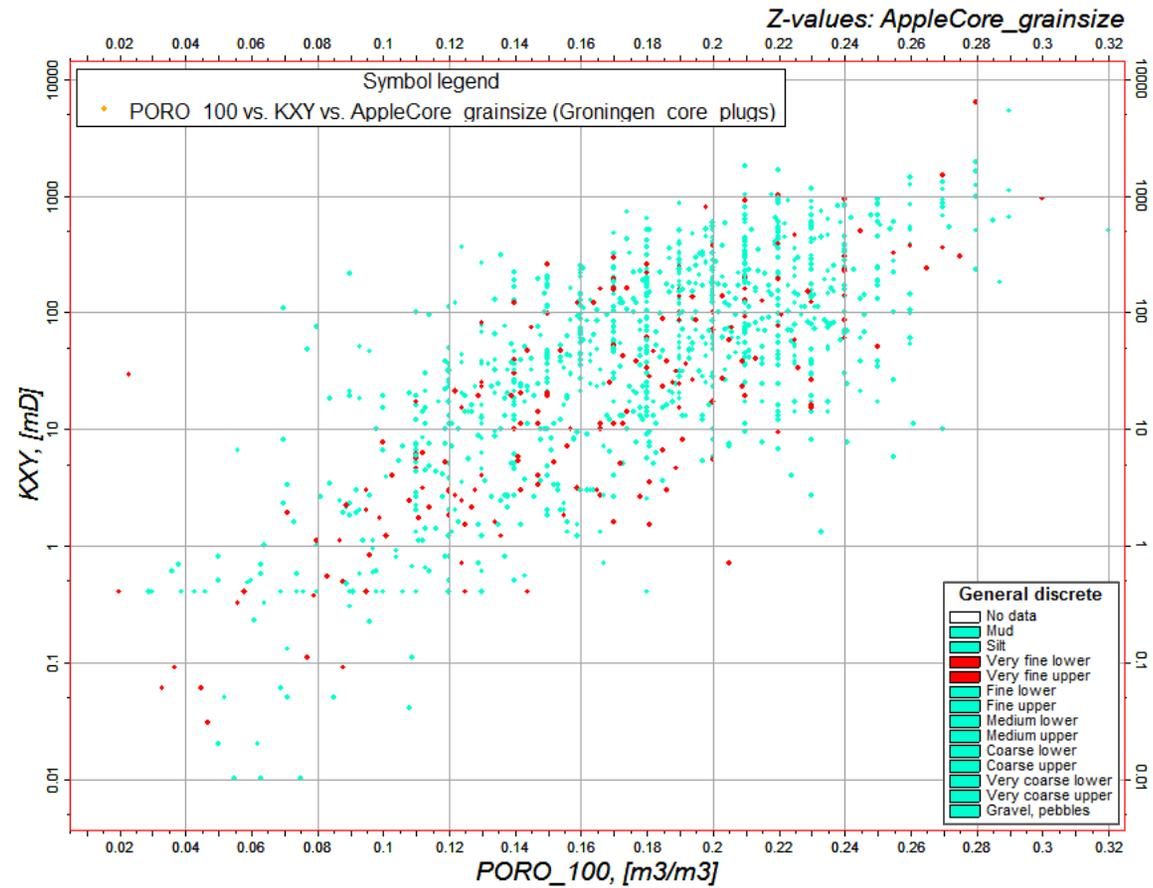
Fig. 20: Porosity-permeability cross-plot from core plug data, very fine sandstone plugs coloured red
