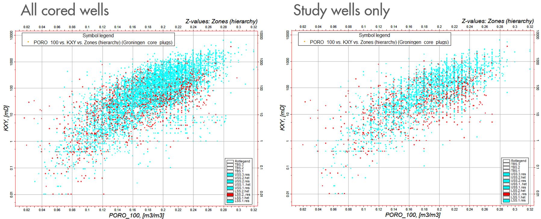
Fig. 31: Porosity-permeability cross-plot of core plug measurements, data points from LSS.2.res coloured red. Left-hand graph shows entire Groningen plug database, right-hand graph shows data for study wells only.
