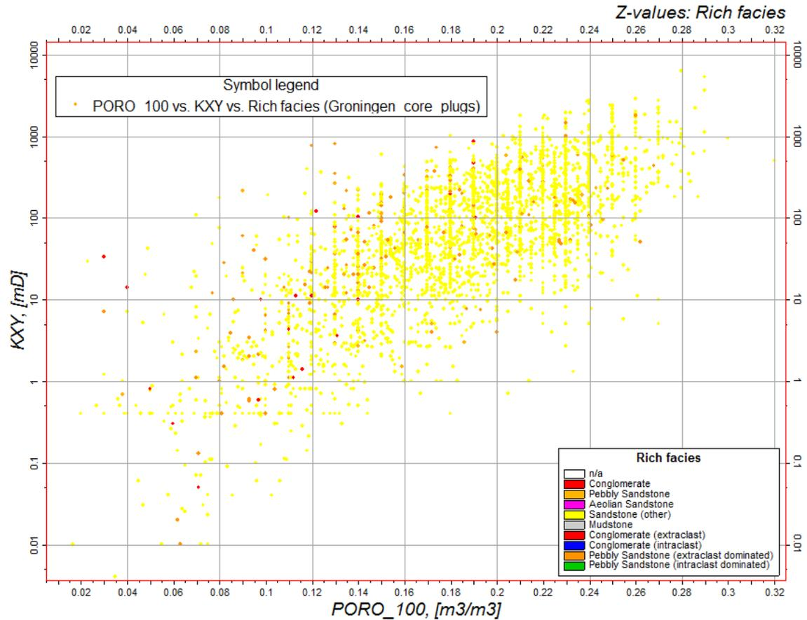
Fig. 13: Porosity-permeability cross-plot showing undifferentiated (yellow) and pebbly extraclast (shades of orange) sandstone core plug data
