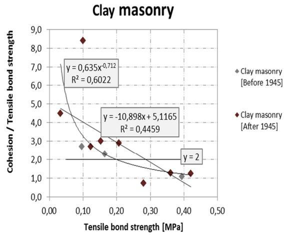
Figure 22 – Ratio between the cohesion and tensile bond strength of joints as a function of the tensile bond strength.
