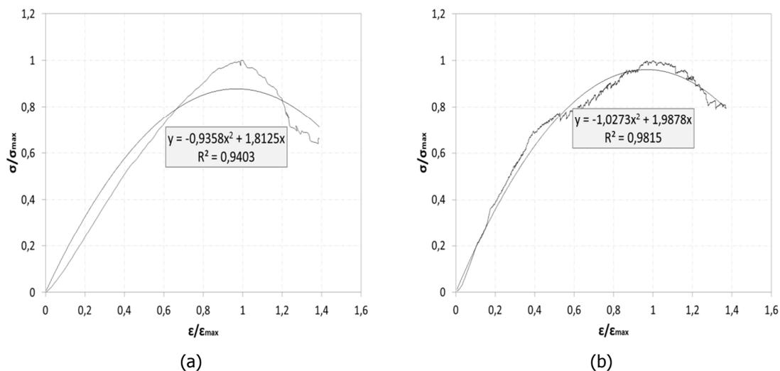
Figure 10 – Average of dimensionless normalised stress-strain curves and parabolic approximation: (a) vertical compression tests; (b) horizontal compression tests.
