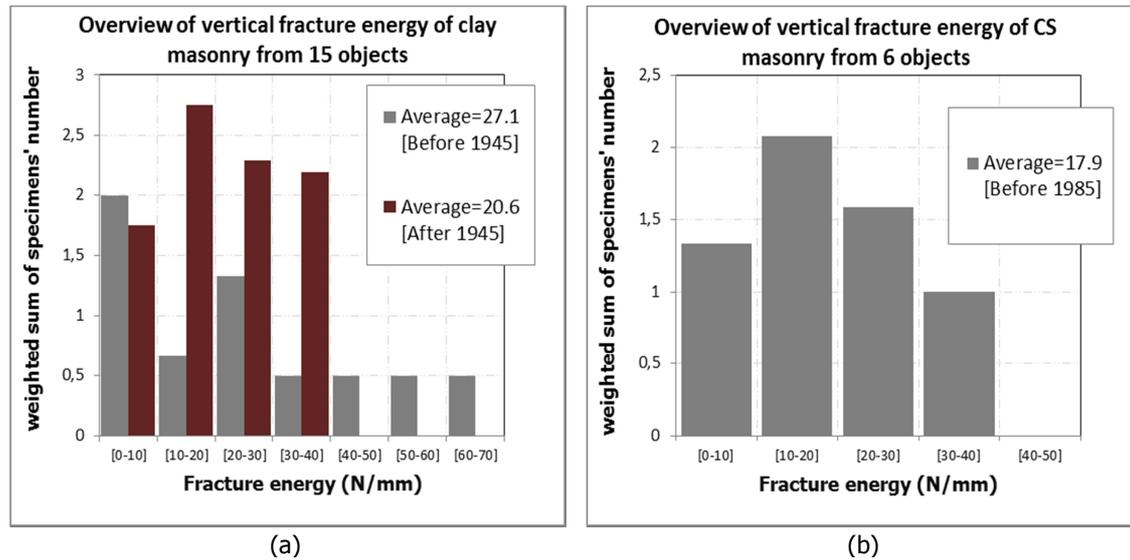
Figure 4 – Histograms of vertical compression fracture energy: (a) all types of clay masonry; (b) calcium silicate masonry.
