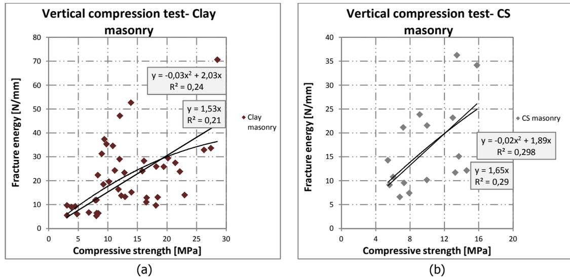
Figure 13 – Vertical fracture energy versus vertical compressive strength: (a) clay masonry; (b) calcium silicate masonry.
