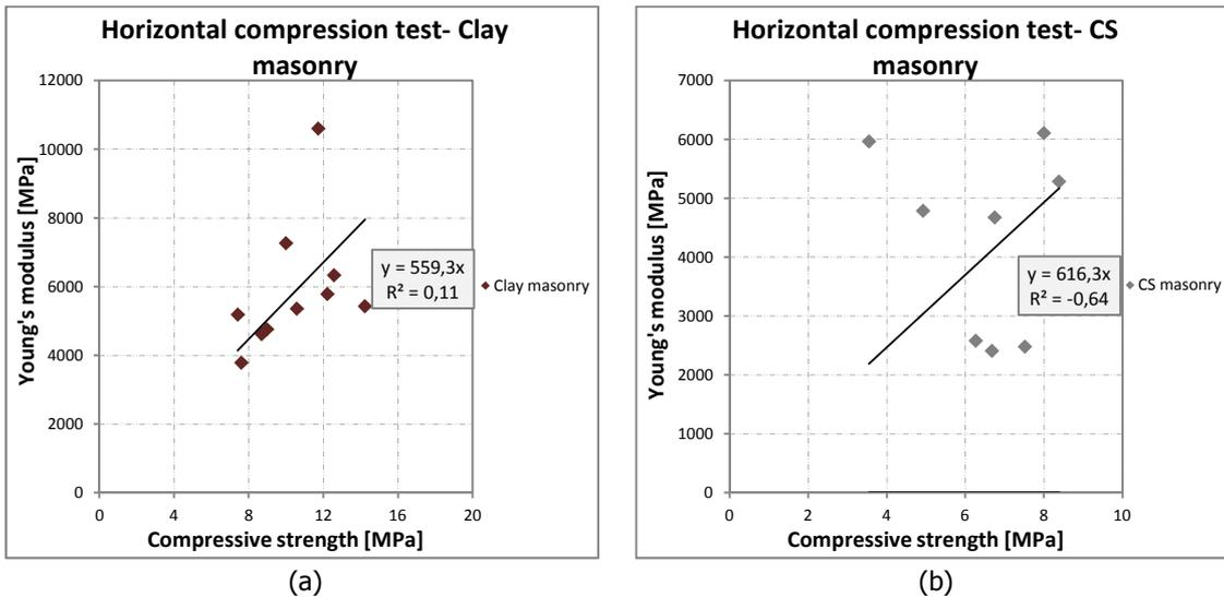
Figure 12 – Horizontal Young's modulus versus horizontal compressive strength: (a) clay masonry; (b) calcium silicate masonry.
