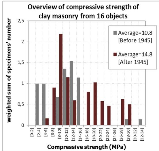
Figure 2 – Histograms of vertical compressive strength from the tests performed at TU Delft and TU/e .
