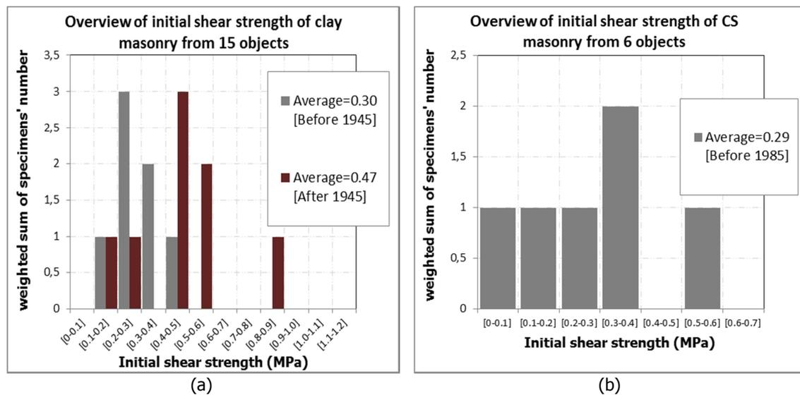
Figure 19 – Histograms of initial shear strength: (a) all types of clay masonry; (b) calcium silicate masonry.
