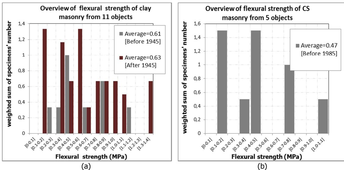
Figure 15 – Histograms of flexural strength from in-plane tests: (a) all types of clay masonry; (b) calcium silicate masonry.
