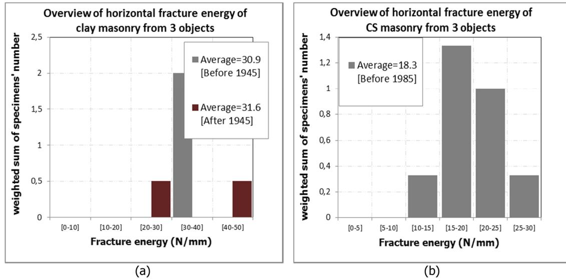
Figure 7 – Histograms of horizontal compression fracture energy: (a) all types of clay masonry; (b) calcium silicate masonry.
