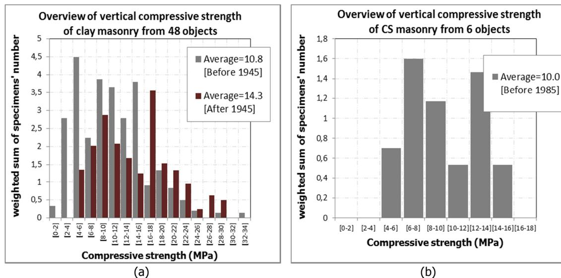
Figure 1 – Histograms of vertical compressive strength: (a) all types of clay masonry; (b) calcium silicate masonry.
