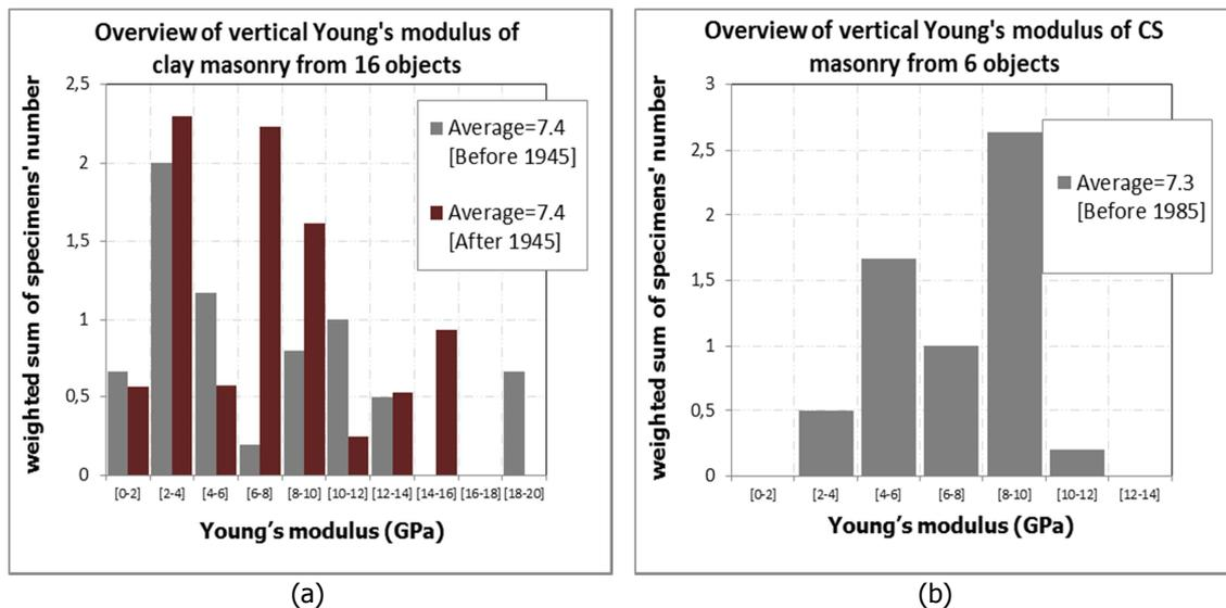
Figure 3 – Histograms of vertical Young’s modulus: (a) all types of clay masonry; (b) calcium silicate masonry.
