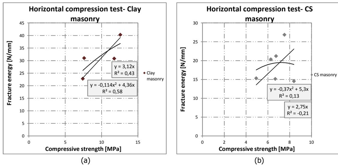
Figure 14 – Horizontal fracture energy versus horizontal compressive strength: (a) clay masonry; (b) calcium silicate masonry.
