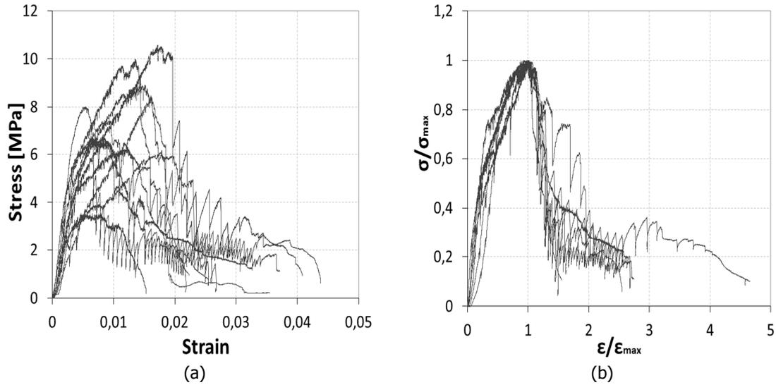
Figure 9 – (a) Stress-strain curves for masonry in horizontal compression tests; (b) dimensionless stress-strain curves for masonry in horizontal compression tests, normalized towards the peak.
