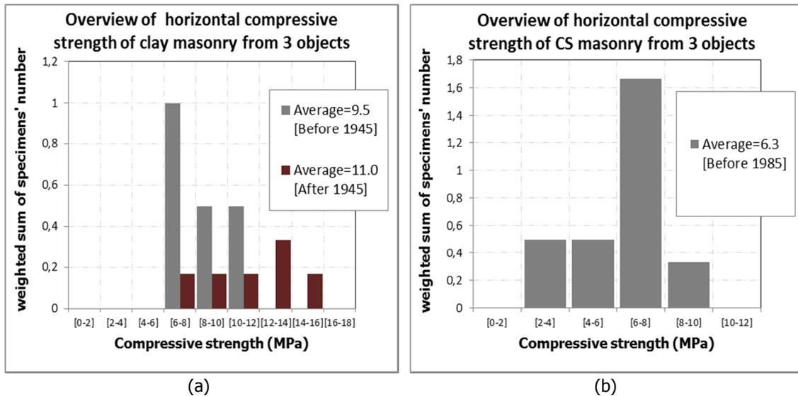
Figure 5 – Histograms of horizontal compressive strength: (a) all types of clay masonry; (b) calcium silicate masonry.
