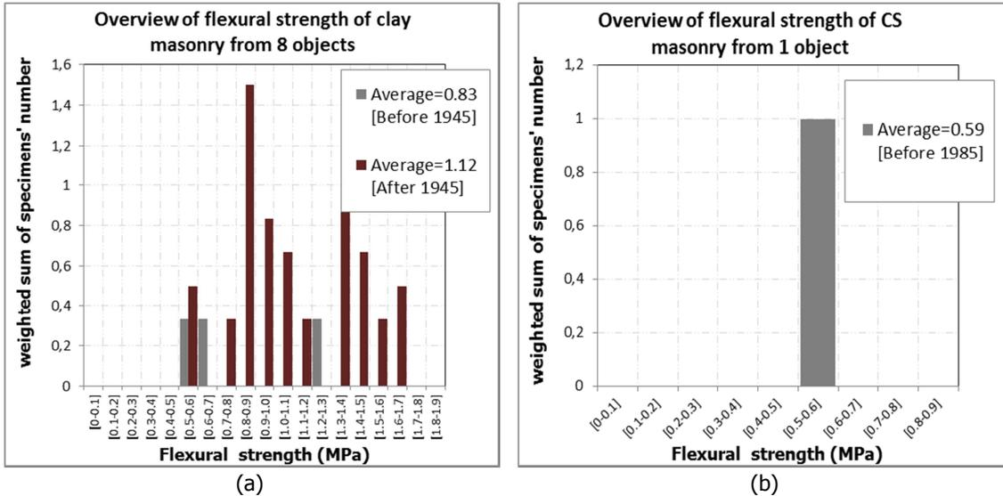
Figure 16 – Histograms of flexural strength from out-of-plane tests with vertical bending: (a) all types of clay masonry; (b) calcium silicate masonry.
