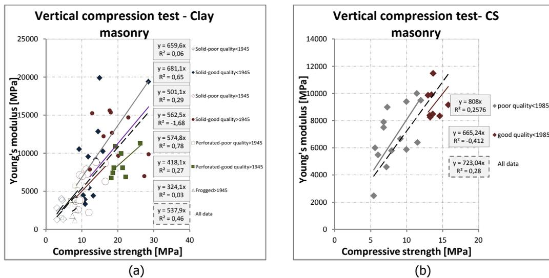
Figure 23 – Vertical Young's modulus versus vertical compressive strength: (a) clay masonry; (b) calcium silicate masonry.
