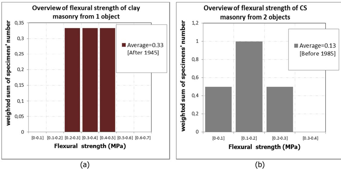
Figure 17 – Histograms of flexural strength from out-of-plane tests with horizontal bending: (a) all types of clay masonry; (b) calcium silicate masonry.
