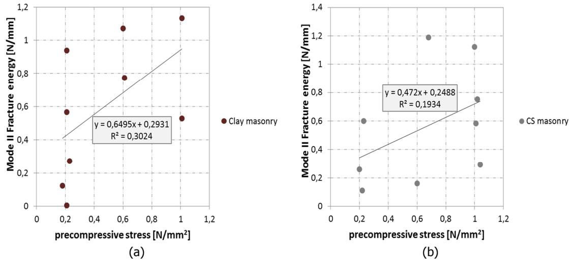
Figure 21 – Mode II fracture energy of specimens as a function of the normal stress: (a) clay masonry ;(b) calcium silicate masonry.
