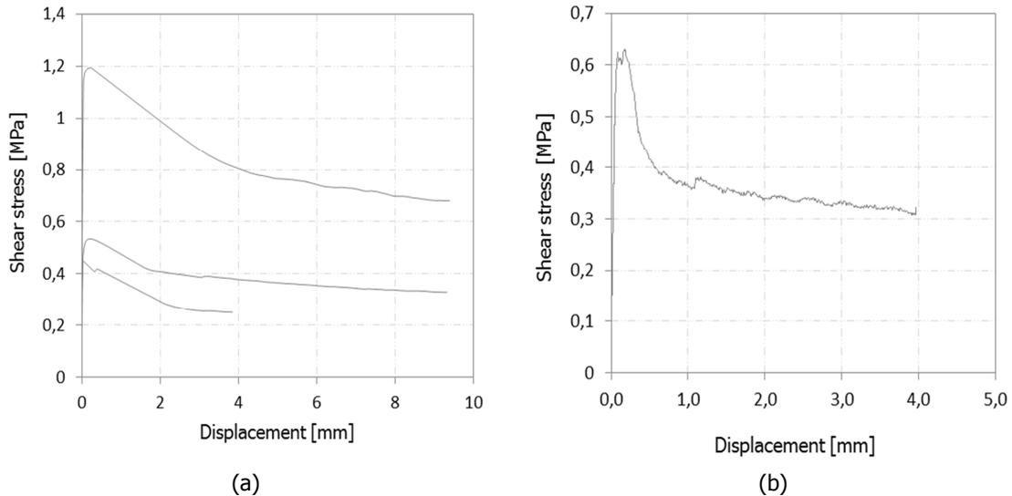
Figure 20 – Shear stress-displacement curves: (a) tests performed at TU/e at the different levels of confinement; (b) tests performed at TU Delft.
