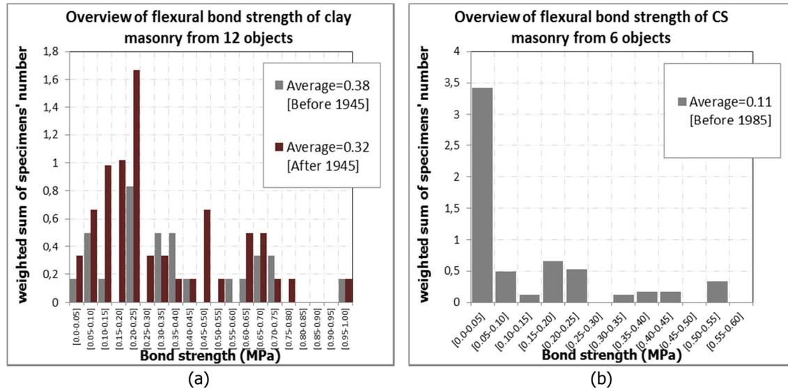
Figure 18 – Histograms of flexural bond tensile strength: (a) all types of clay masonry; (b) calcium silicate masonry.
