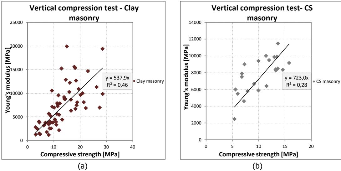
Figure 11 – Vertical Young's modulus versus vertical compressive strength: (a) clay masonry; (b) calcium silicate masonry.
