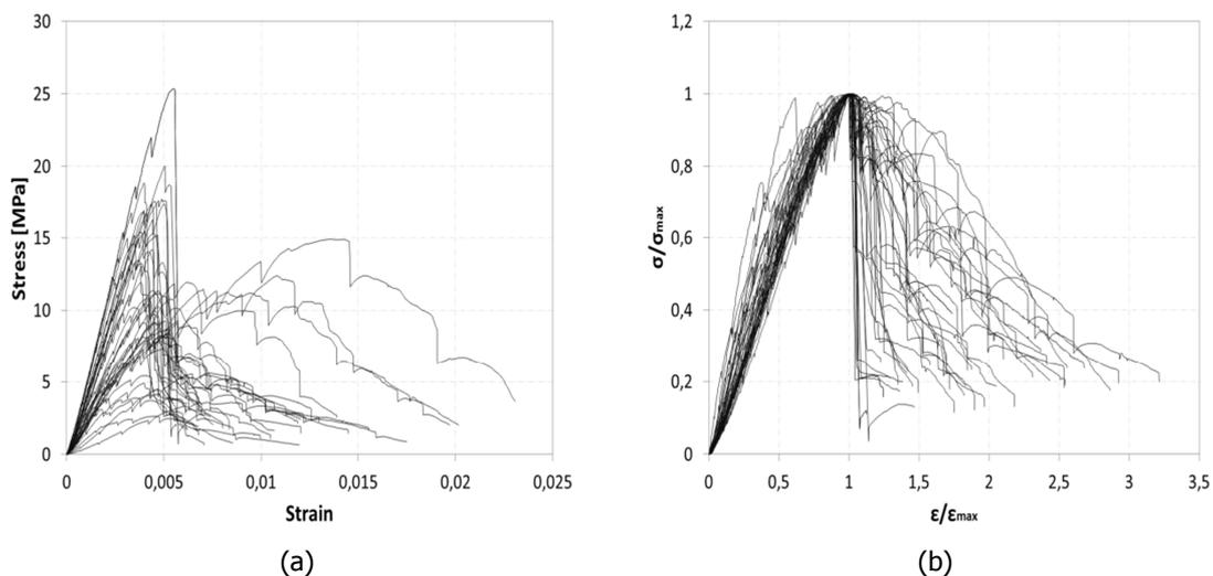
Figure 8 – (a) Stress-strain curves for masonry in vertical compression tests; (b) dimensionless stress-strain curves for masonry in vertical compression tests, normalized towards the peak.
