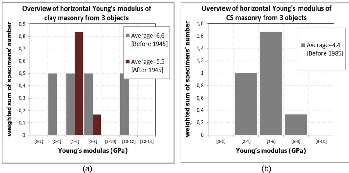
Figure 6 – Histograms of horizontal Young's modulus: (a) all types of clay masonry; (b) calcium silicate masonry.
