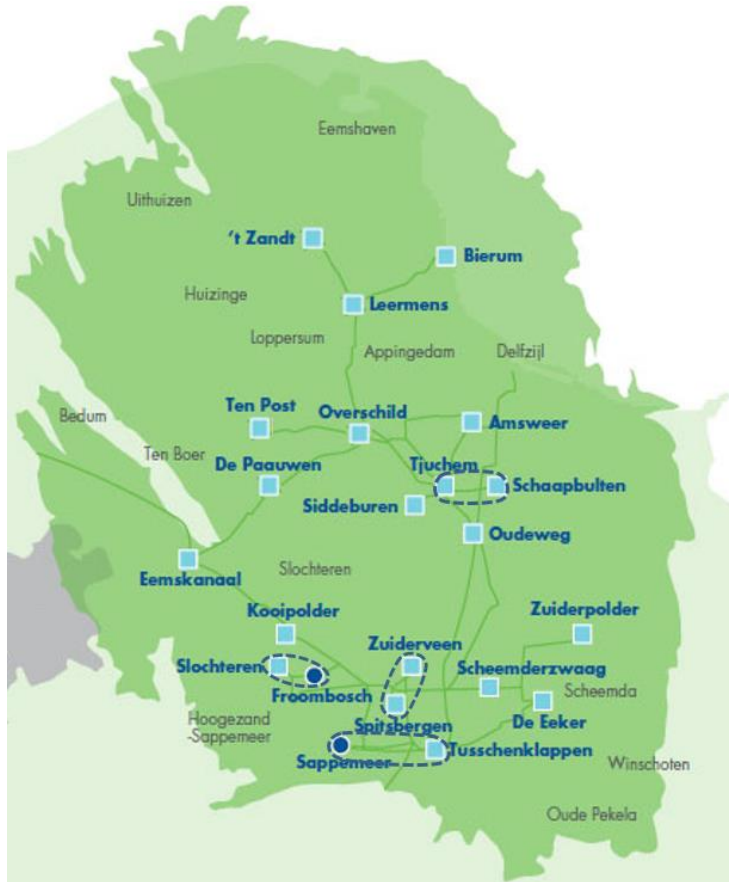
Figure 4-8: Model controls: 18 independent controls. Froombosch is a tie-back to Slochteren, and Sappemeer is a tie-back to Tussenklappen. Spitsbergen was merged with Zuiderveen, Tjuchem was merged with Schaapbulten.
