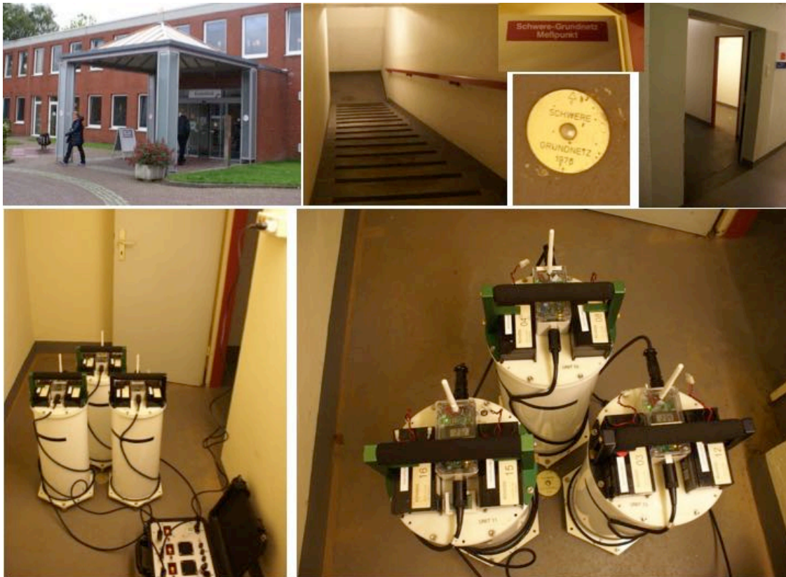
Figure 34: Pictures from the reference station 401 Aurich. A golden plate in the floor marks the site.
