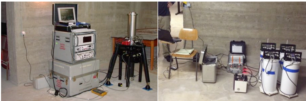
Figure 86: The basement of the St.-Michael Gymnasium in Monschau, Germany, with absolute measurement (left) and relative measurement (right).
