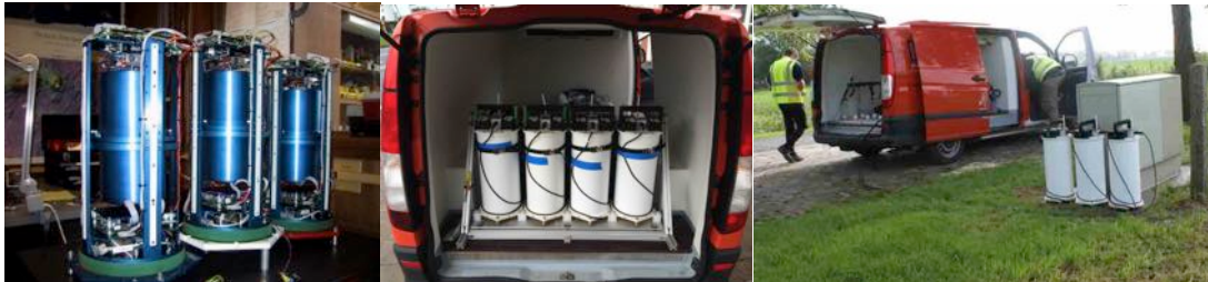
Figure 38: Left: Inside of gravimeter housing with gimbal frames and CG5 sensor cores. Middle: All four gravimeters fitted into the frame in the back of the survey car. Right: Three gravimeters on a seismic station (right).
