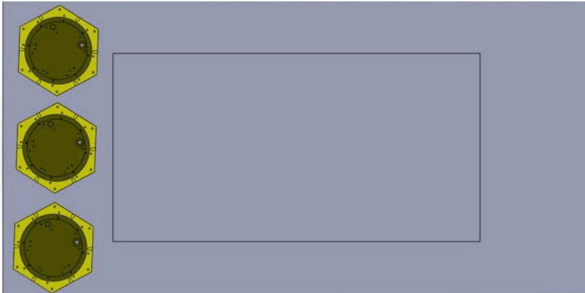
Figure 30: Sketch of how the three gravimeters are placed onto the short side of the concrete platform.
