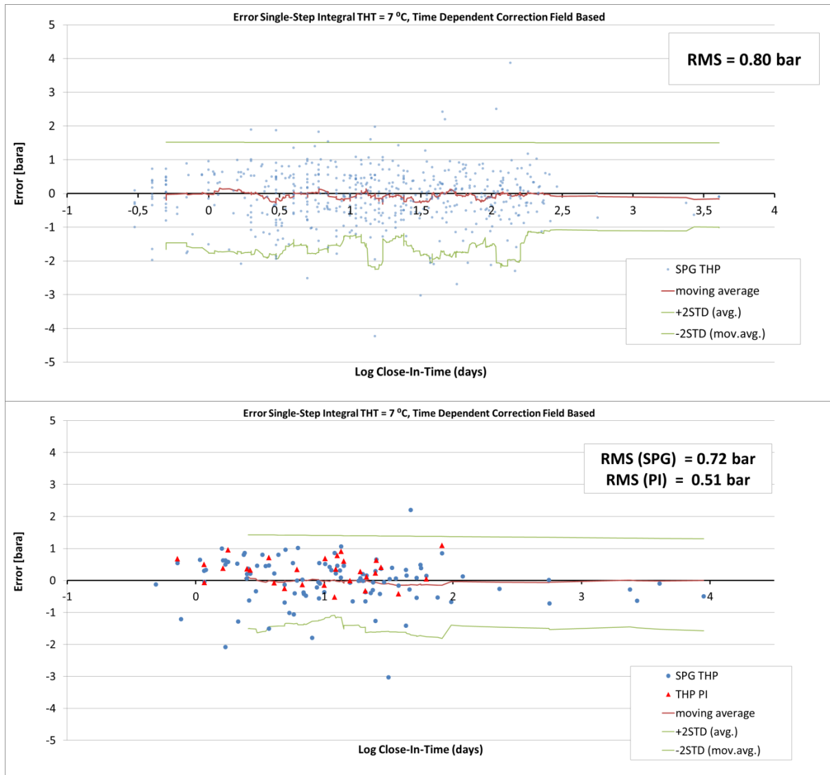
Figure 29: Error behavior of Field Based Time Corrected Single-Step integral conversion with THT = 7 degree C versus log (days shut-in time). Note that moving average and STD are only based on SPG data.
