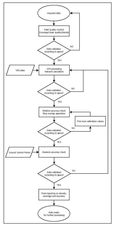
Figure 5: Processing flowchart
