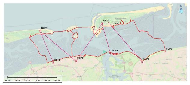
Figure 4: Overview of Ground Control Points
