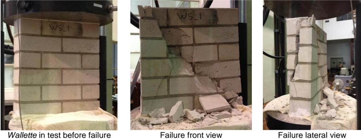
Figure 2.54 Calcium silicate block walette (WS\_1) during the test and after failure.
