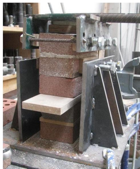
Figure 2.104 Test of the two connections in clay bricks using the same test device.
