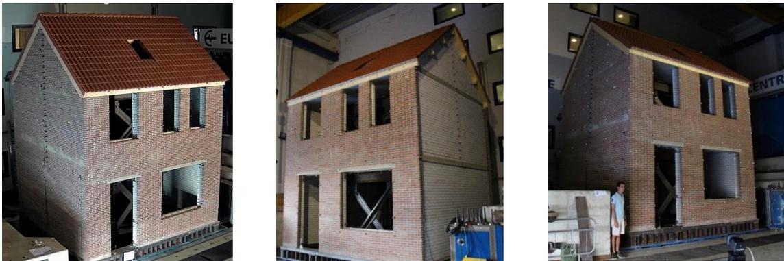
Figure 1.2 Views of the full-scale specimen built in Eucentre, Pavia, Italy.
