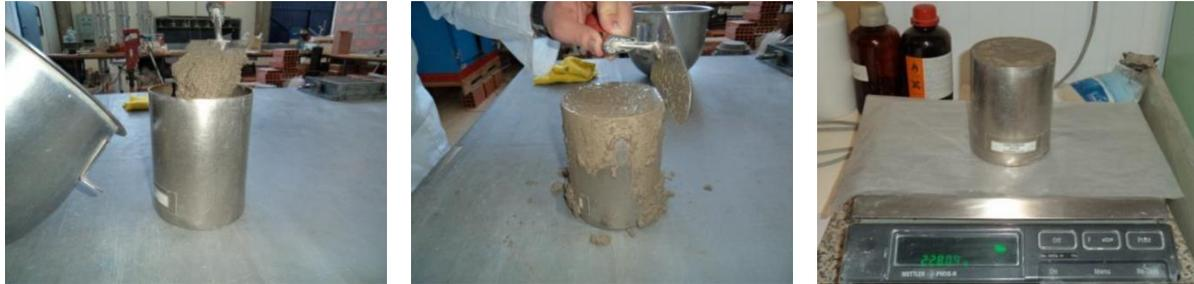
Figure 2.5 Carrying out the determination of bulk density of fresh mortar.
