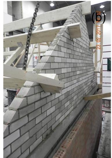
Figure 1.9 Details of the roof structure: (a) geometry of the timber diaphragm; (b) connection between the timber beams and the West gable.
