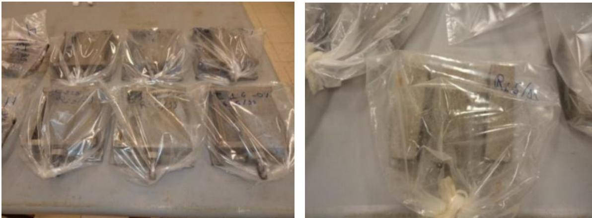
Figure 2.8 Curing conditions of mortar specimens.
