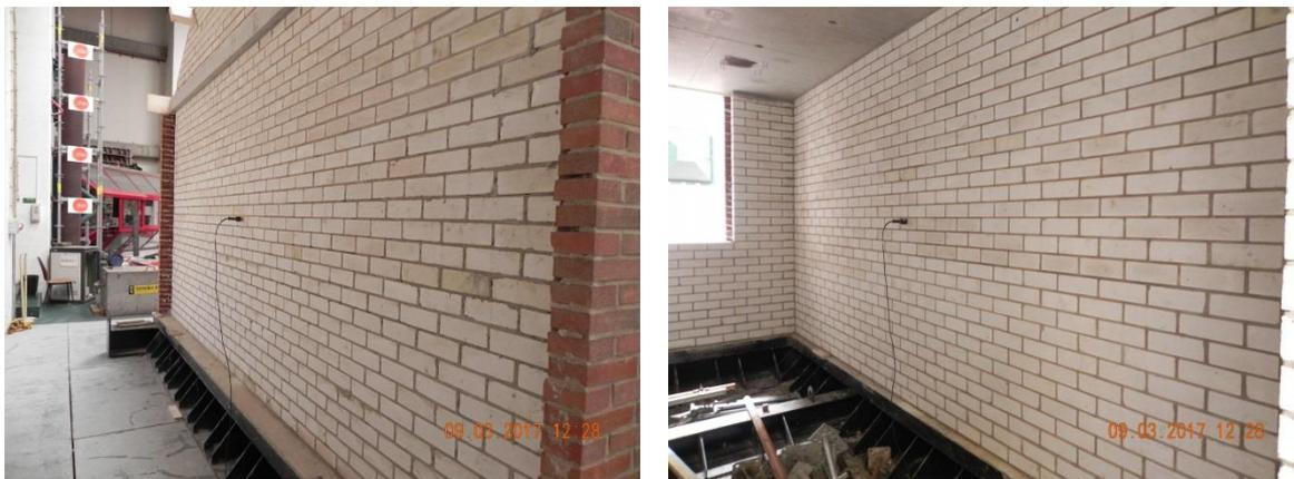
Figure 5.7 Accelerometers at the centre of the load-bearing walls.
