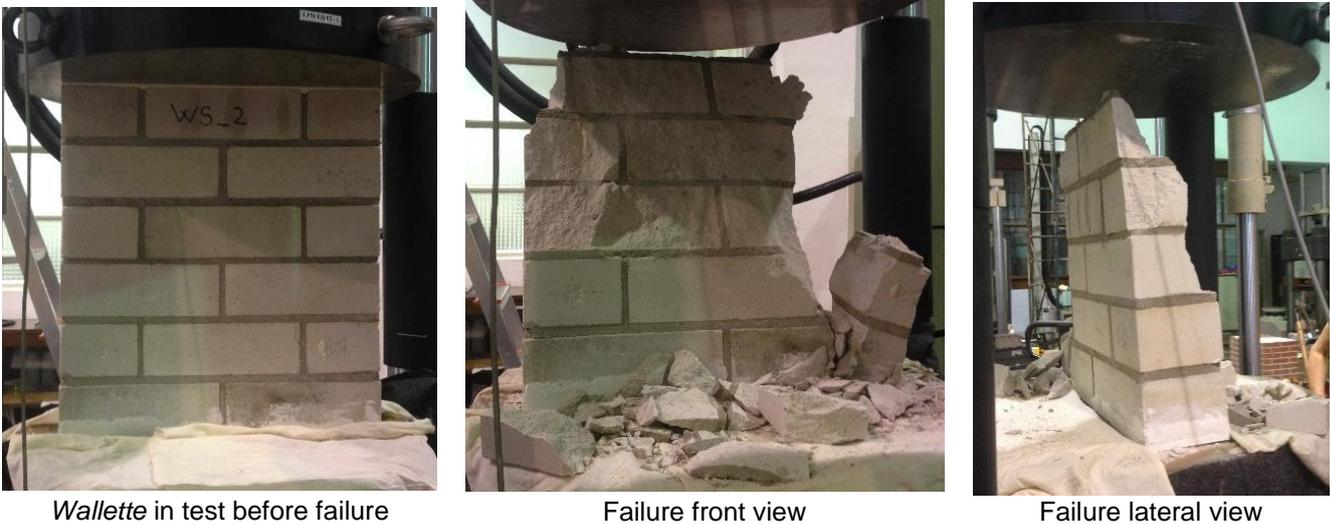
Figure 2.55 Calcium silicate block walette (WS\_2) during the test and after failure.
