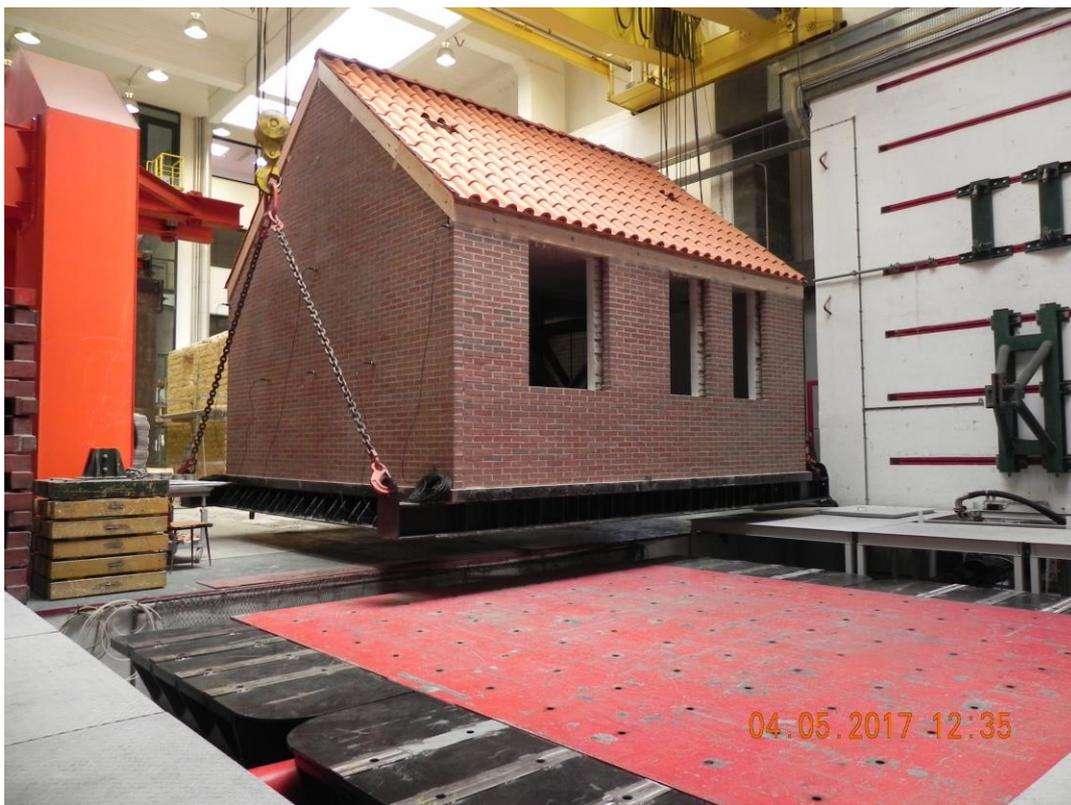
Figure 5.34 Specimen transportation to the shaking table.
