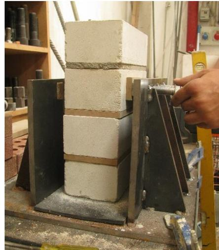
Figure 2.103 Test of the two connections in calcium silicate blocks using the same test device.
