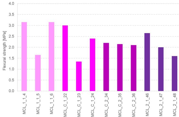
Figure 2.27 Flexural strength test results for bedding mortar specimens used with clay bricks (MCL) after 20 days of age.
