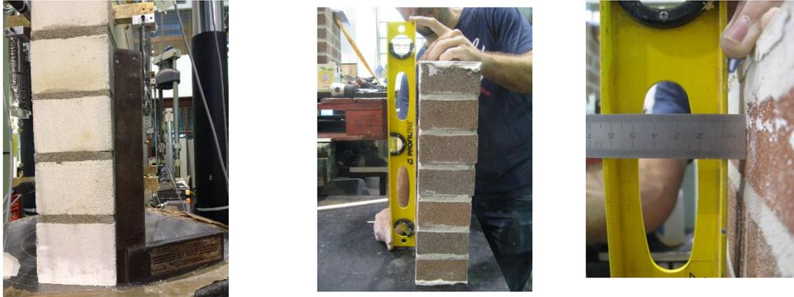
Figure 2.47 Lack of verticality in wallettes.
