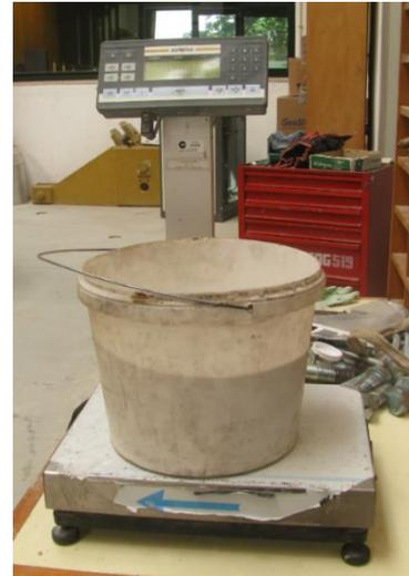
Figure 2.106 Measure of the weight of the top unit, its adherent mortar and sand volume leading to failure.
