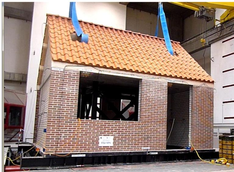
Figure 5.16 Test specimen on the shaking table.
