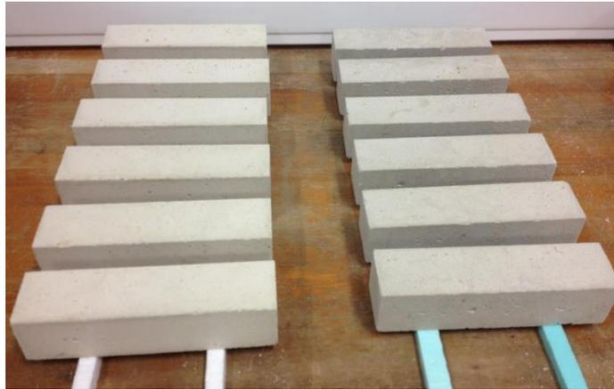
Figure 2.7 Part of mortar specimens.
