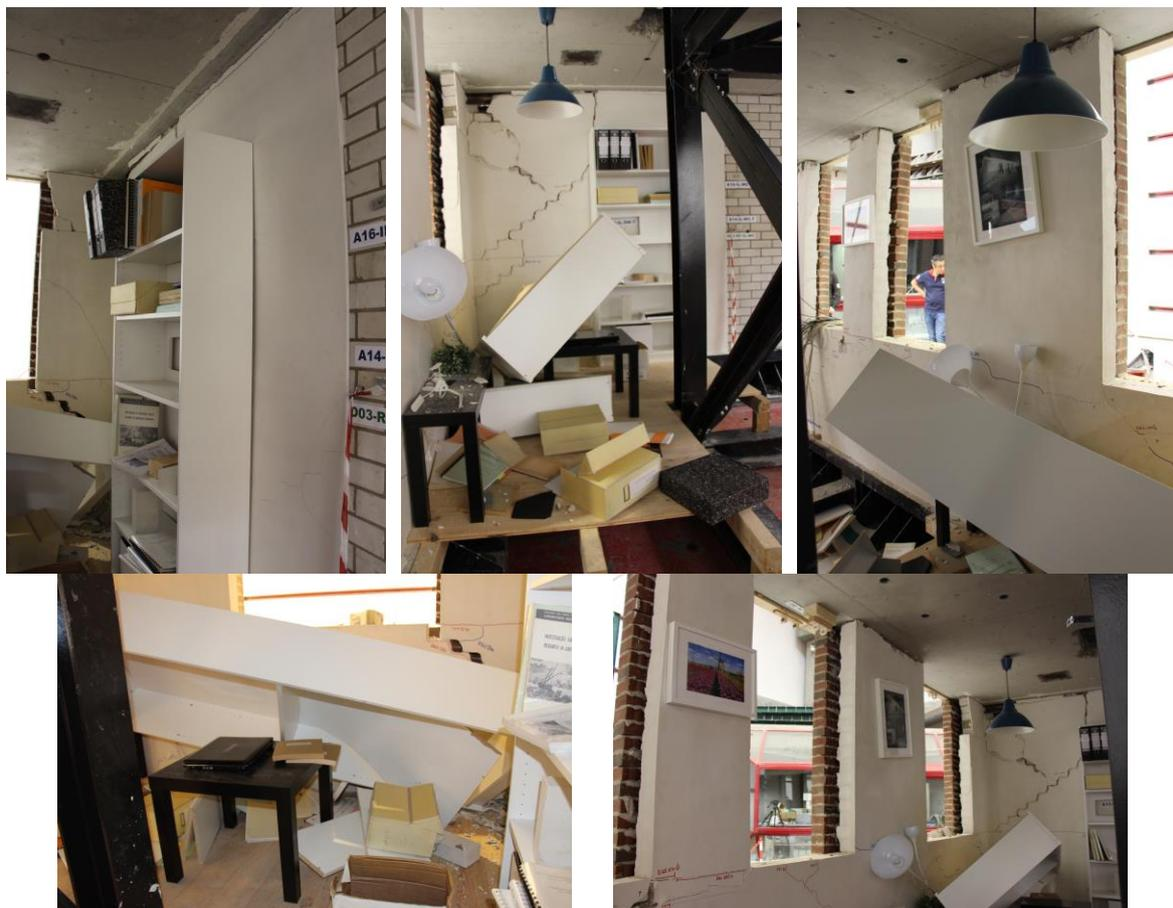
Figure 5.41 Pictures of the specimen at the end of test FEQ-300%.
