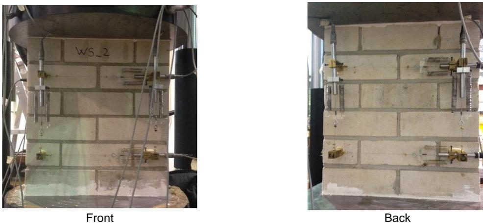
Figure 2.51 Instrumentation placed on each face of the calcium silicate wallettes.
