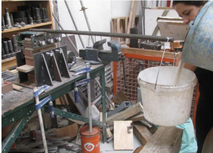
Figure 2.105 Application of vertical force until bond failure.
