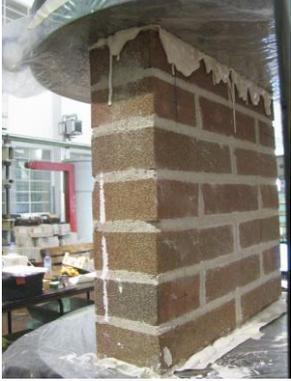
Figure 2.46 Final regularisation of the *wallettes* faces on top of the testing machine.
