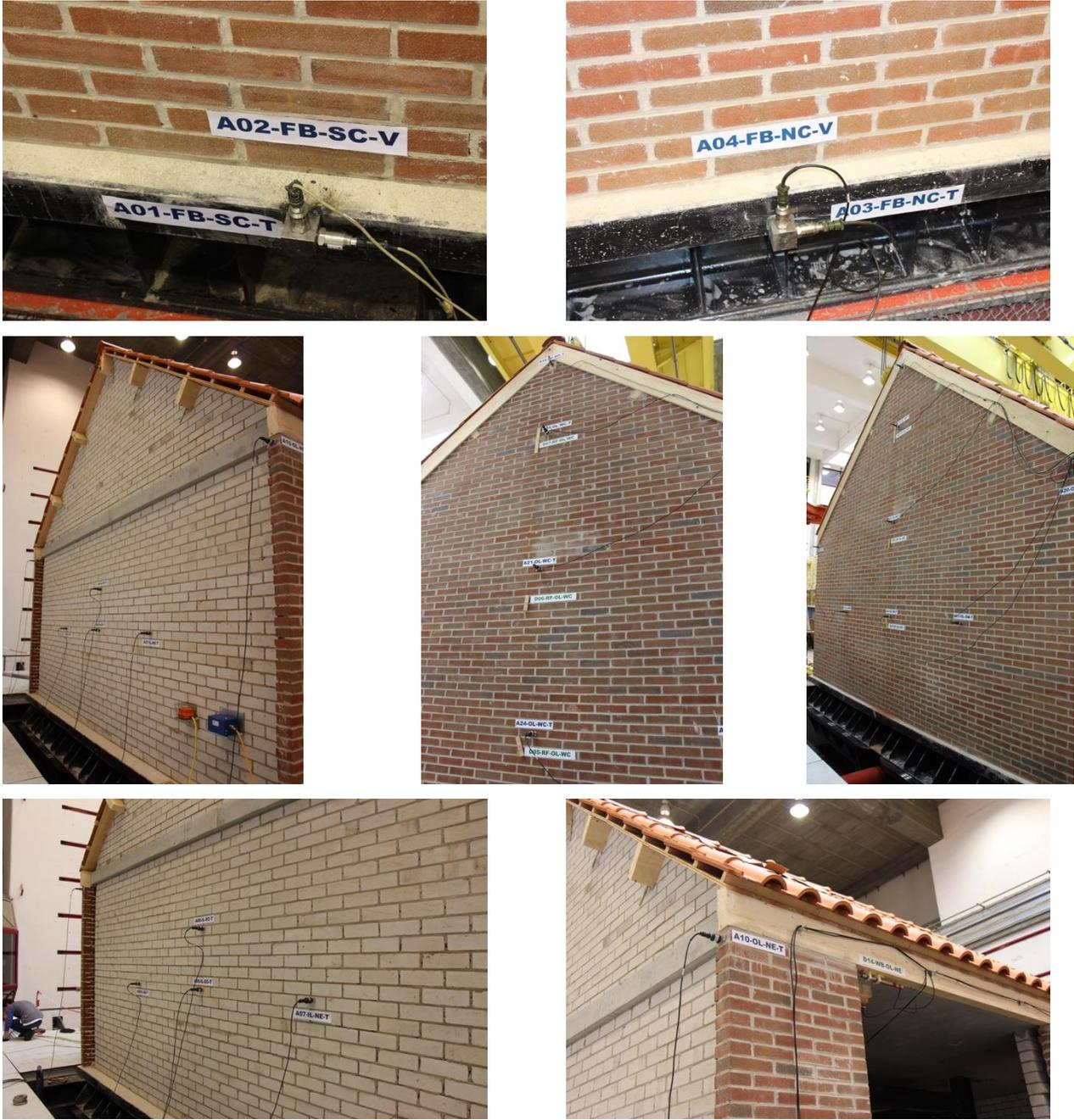
Figure 3.2 Pictures of the instrumentation.
