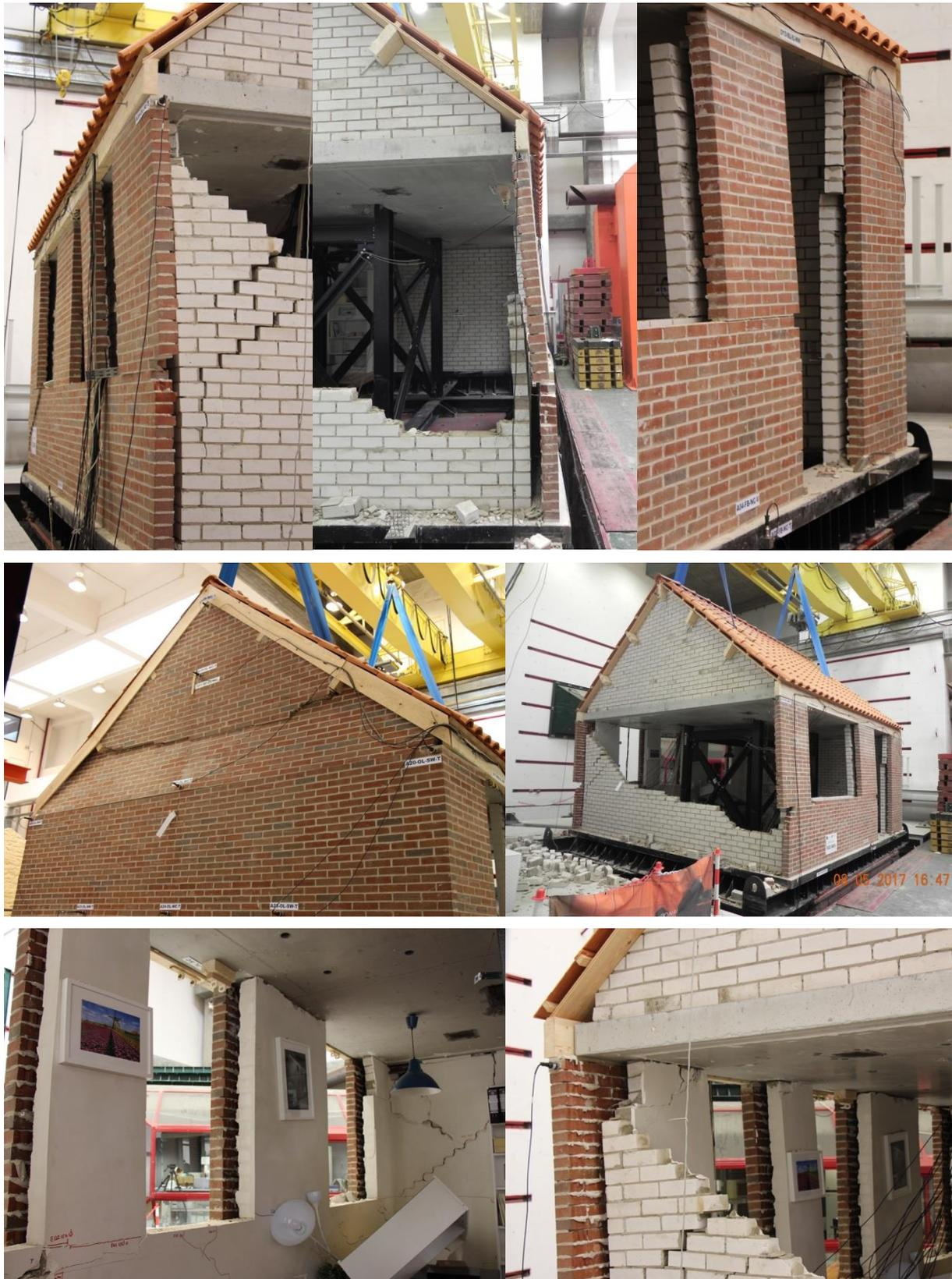
Figure 5.39 Pictures of the specimen at the end of the test FEQ-300%.
