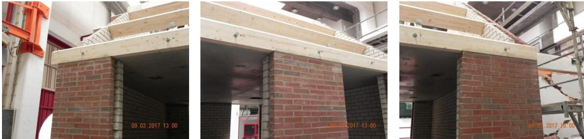
Figure 5.5 Joints filled with mortar.
