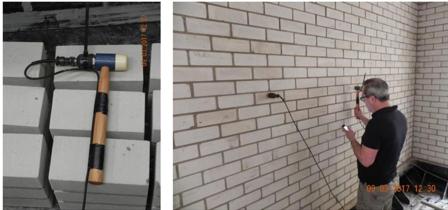
Figure 5.6 Instrumented hammer and application of periodic excitation pulses.
