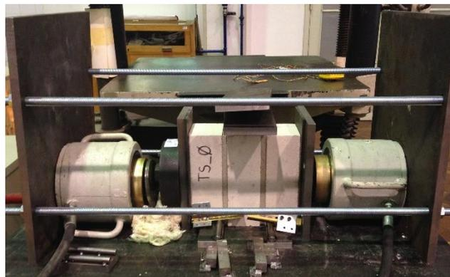
Figure 2.89 Final version of the shear strength test device.
