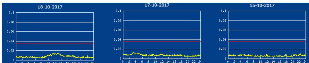
The ionospheric activity can also be expressed with the ionospheric noise index 195. The 195 values compute all corrections for the sattelites of all the station of the network with a timewindow of 1 hour. What happened is that the worst 5 % is rejected and the highest values left will be displayed in the graph. Figure 4.2 shows the 195 values for the 15<sup>th</sup>, 17<sup>th</sup> 18<sup>th</sup> of October, indicating a non-disturbed base station.
