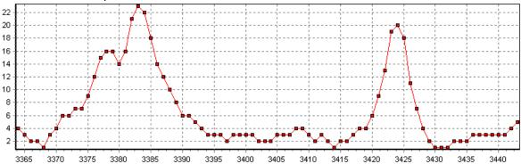
Figure 3.1 Discretized full waveform scanner output. On the x-axis the signal time is shown, on the y-axis the returning signal intensity is shown. The first peak represents the first pulse, the second peak shows the last pulse. In practice the first pulse will often represent vegetation and the last pulse the ground level.
