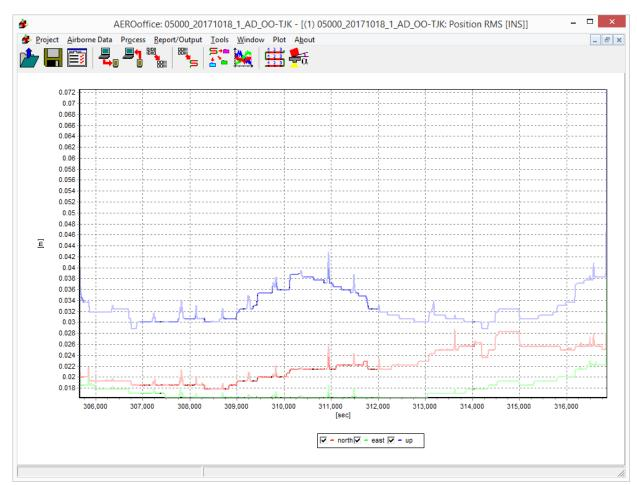
Estimated accuracy of the trajectory after combining the GPS solution with INS.
