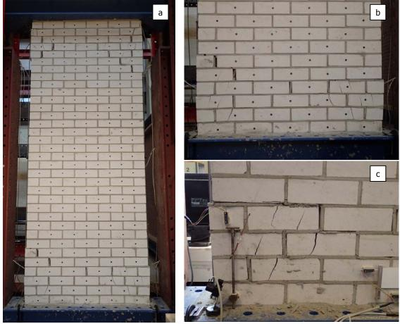
Figure 14. TUD\_COMP-0a: Crack pattern at end stage; general overview (a); detail of the bottom part of the wall (b) and of the toe crushing (c).
