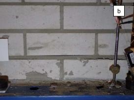
Figure 16. TUD\_COMP-1: Rocking cracks at the base of the wall: details of the left (a) and right (b) toes.
