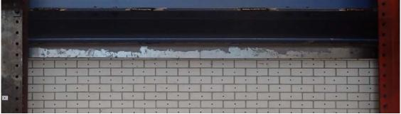
Figure 24. Detail of the repaired top bricklayer of TUD\_COMP-4.
