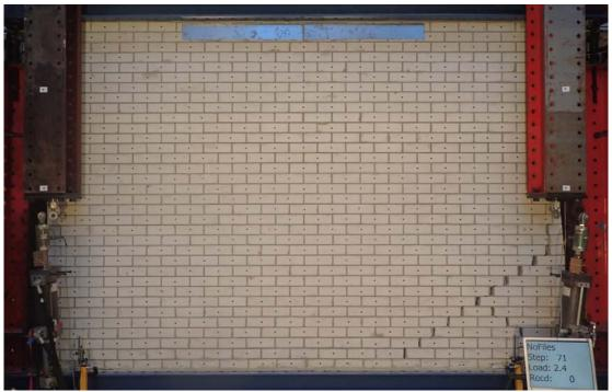
Figure 31. TUD\_COMP-5: crack pattern at end stage.
