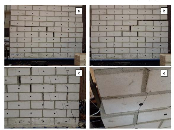
Figure 17. TUD\_COMP-1: Crack pattern at end stage for positive (a) and negative (b) drifts; details of the toe crushing (c) and sliding (d) at end stage.
